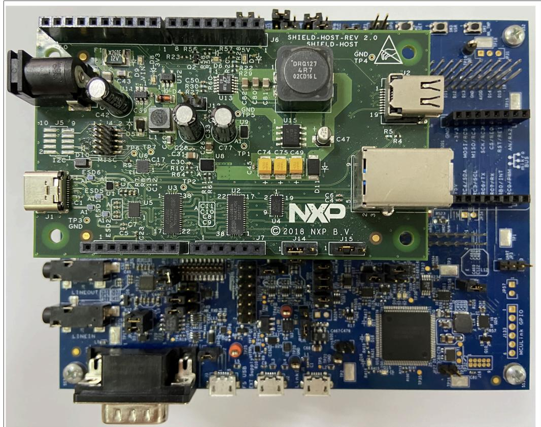
Figure 26. LPCXpresso55S36 connect shield board
