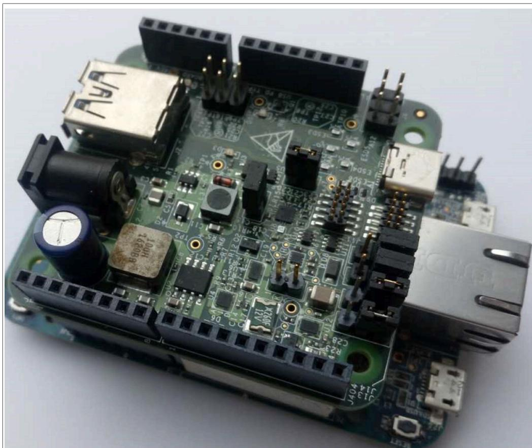
Figure 11. FRDM-K64F connect shield board
