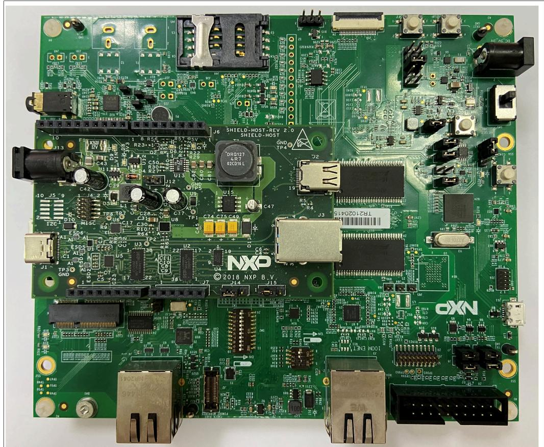
Figure 24. MIMXRT1160-EVK connect shield board
