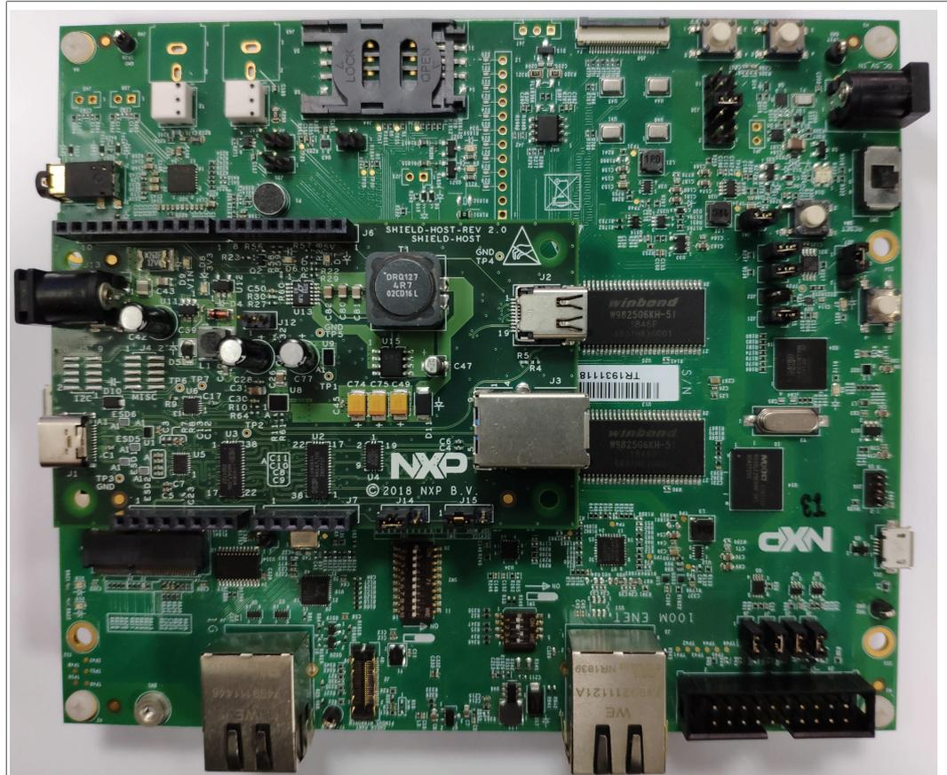
Figure 19. MIMXRT1170-EVK connect shield board
