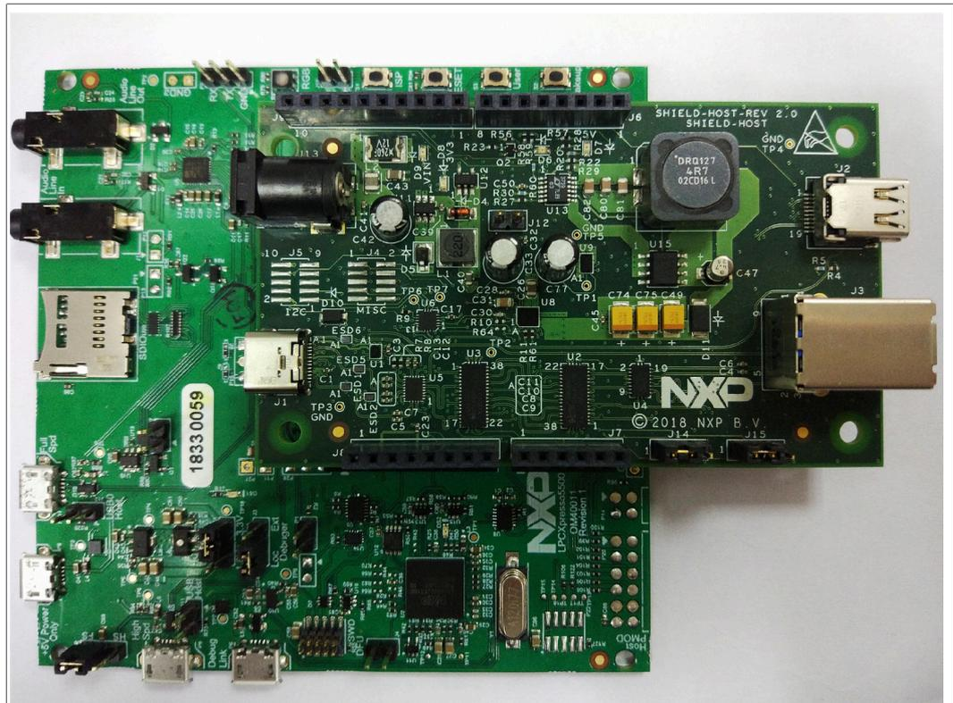
Figure 8. LPCxpresso55S69 connect shield board
