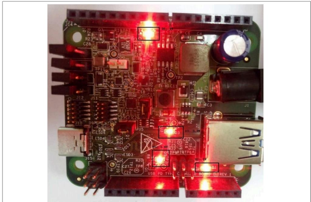
Figure 28. Shield board LEDs
