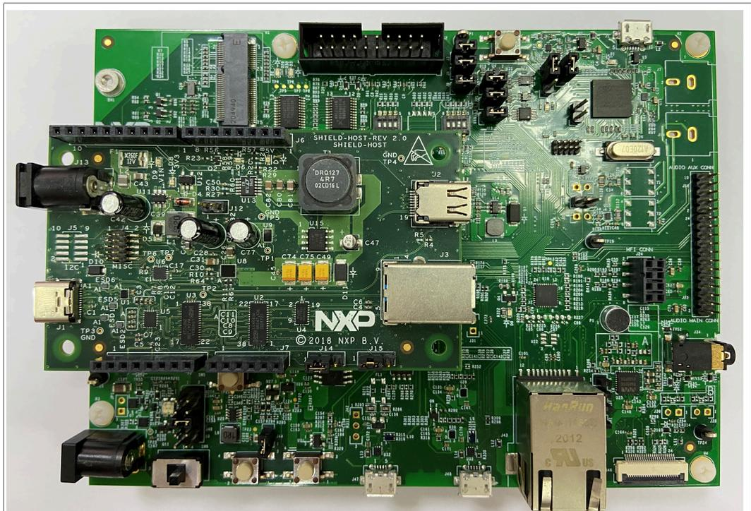
Figure 23. MIMXRT1060-EVKB connect shield board
