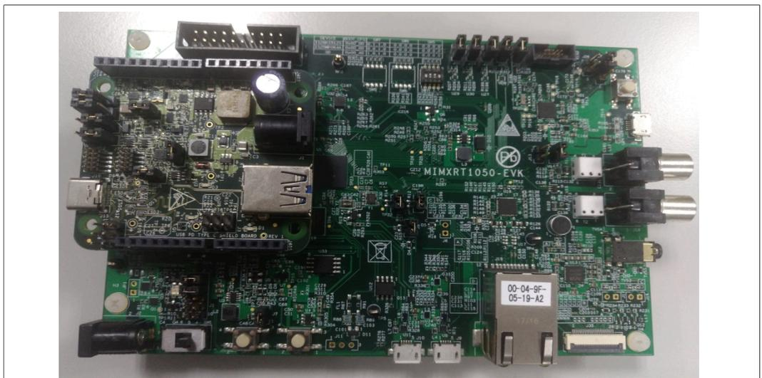
Figure 13. MIMXRT1050-EVK connect shield board
