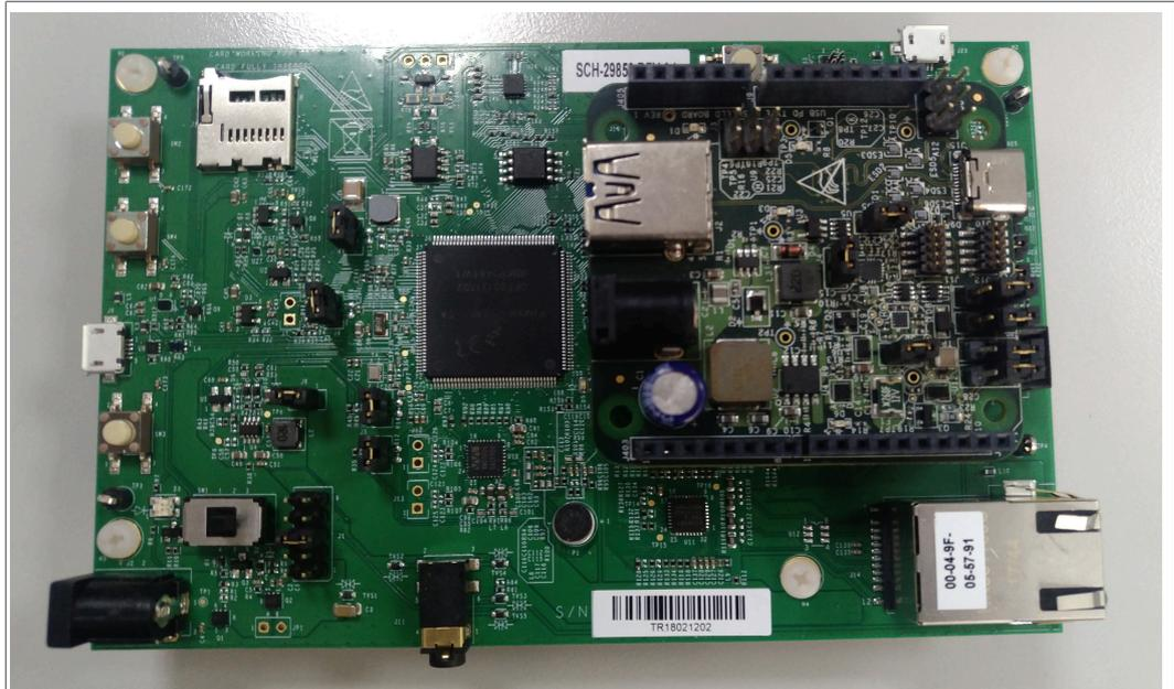
Figure 14. MIMXRT1020-EVK connect shield board
