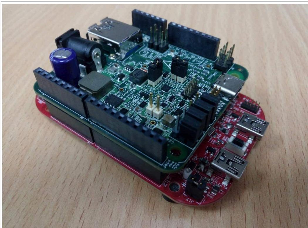
Figure 9. FRDM-KL27Z connect shield board
