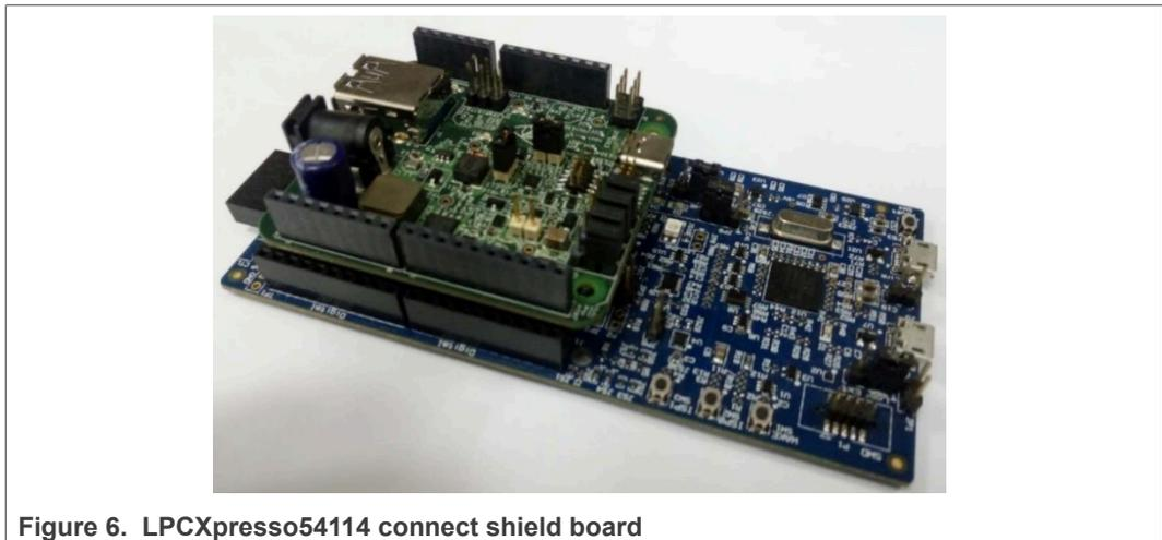
Figure 6. LPCXpresso54114 connect shield board
