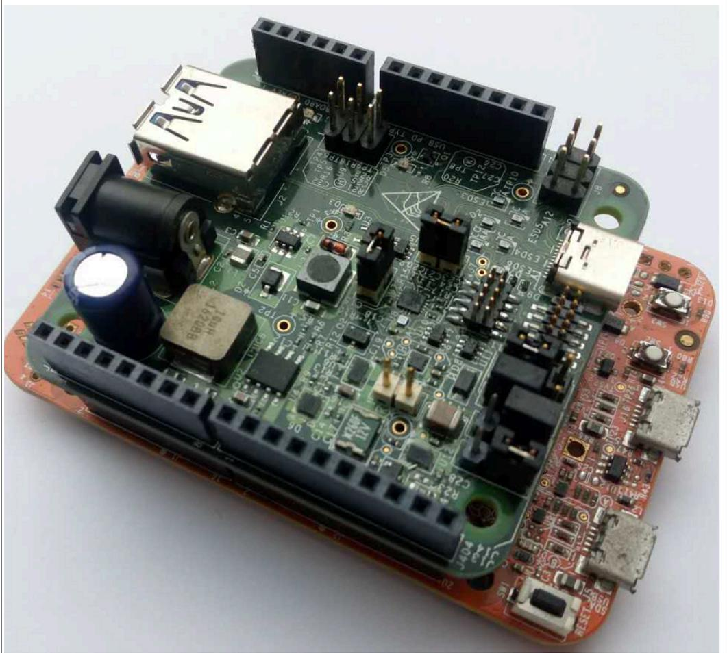
Figure 10. FRDM-K22F connect shield board
