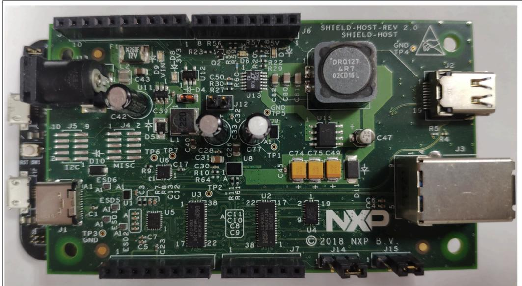
Figure 20. FRDM-KL32L2A4S connect shield board
