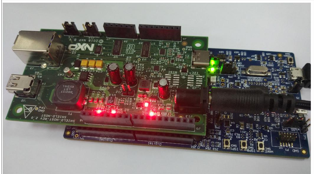
Figure 4. Hardware example - LPCXpresso54114 and shield host board om13790host
