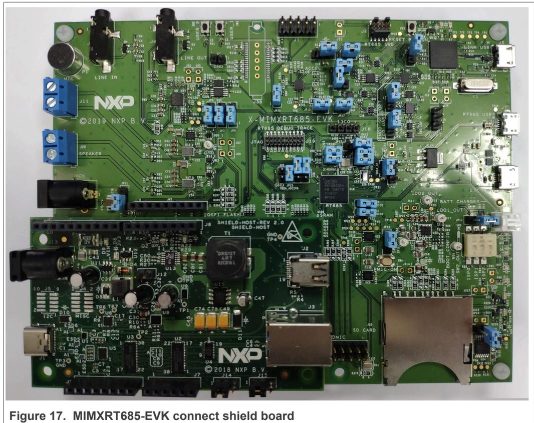
Figure 17. MIMXRT685-EVK connect shield board
