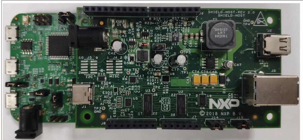
Figure 22. MC56F83000-EVK connect shield board
