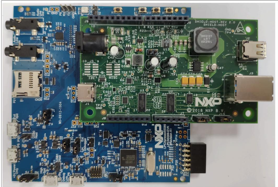
Figure 5. LPCXpresso55S28 connect shield board
