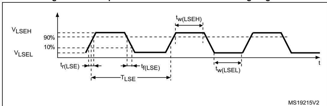
Table 48. Low-speed external user clock characteristics, bypass mode<sup>(1)</sup>
