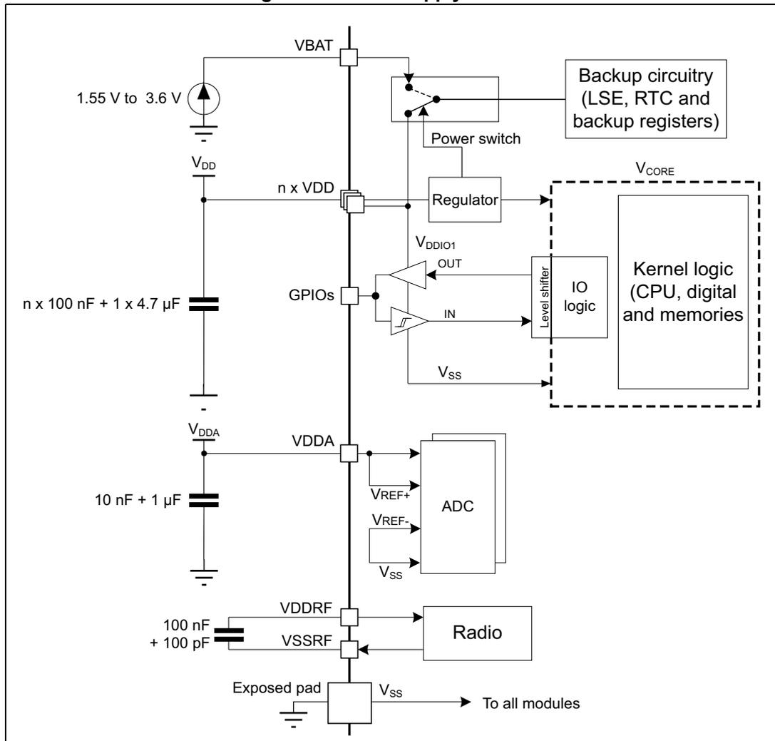
**Caution:** Each power supply pair (such as  $V_{\text{DD}} / V_{\text{SS}}$ ,  $V_{\text{DDA}} / V_{\text{SS}}$ ) must be decoupled with filtering ceramic capacitors as shown in Figure 11. These capacitors must be placed as close as possible to (or below) the appropriate pins on the underside of the PCB to ensure the good functionality of the device.
