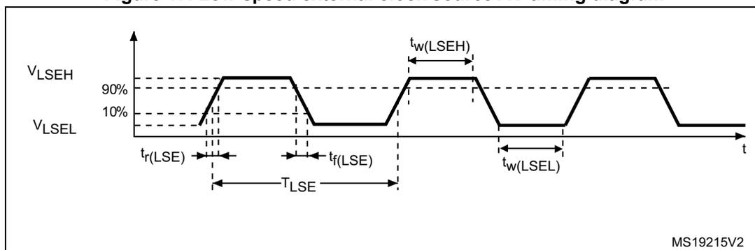
Table 51. Low-speed external user clock characteristics<sup>(1)</sup> – Bypass mode
