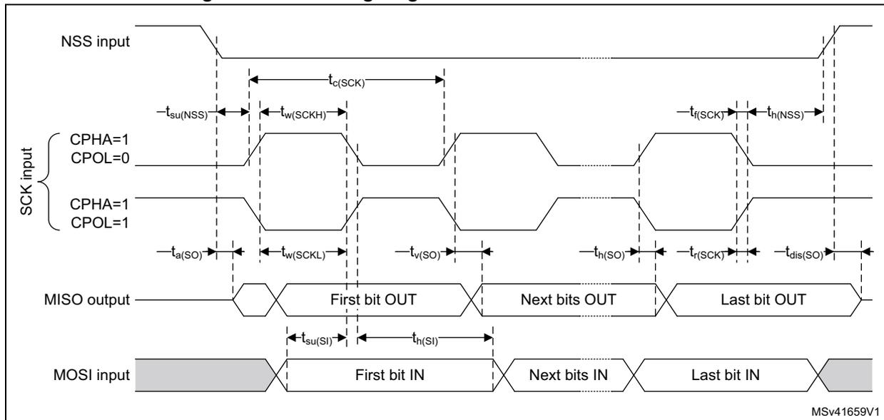
1. Measurement points are set at CMOS levels:  $0.3 V_{DD}$  and  $0.7 V_{DD}$ .
