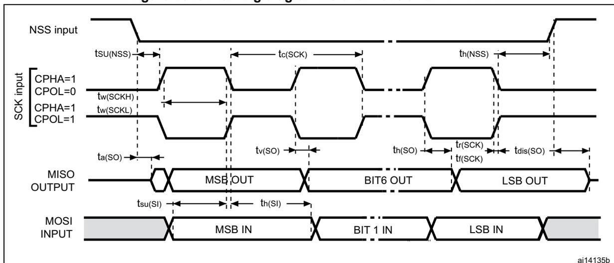
1. Measurement points are set at CMOS levels: 0.3  $V_{DD}$  and 0.7  $V_{DD}$ .
