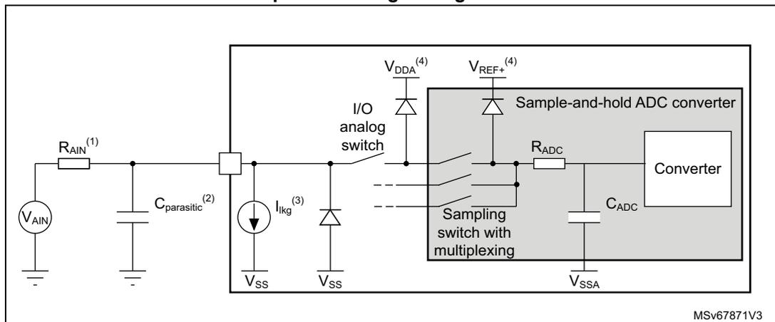
1. Refer to [Table 66: ADC characteristics](#) for the values of  $R_{AIN}$ ,  $R_{ADC}$  and  $C_{ADC}$ .
