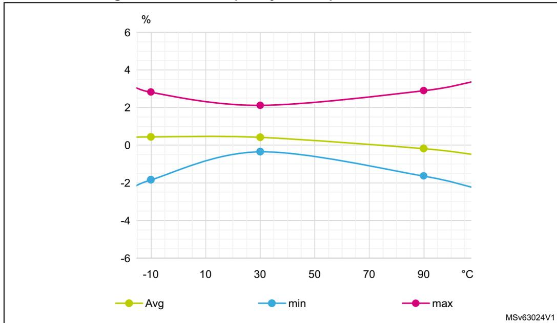
Low-speed internal (LSI) RC oscillator
