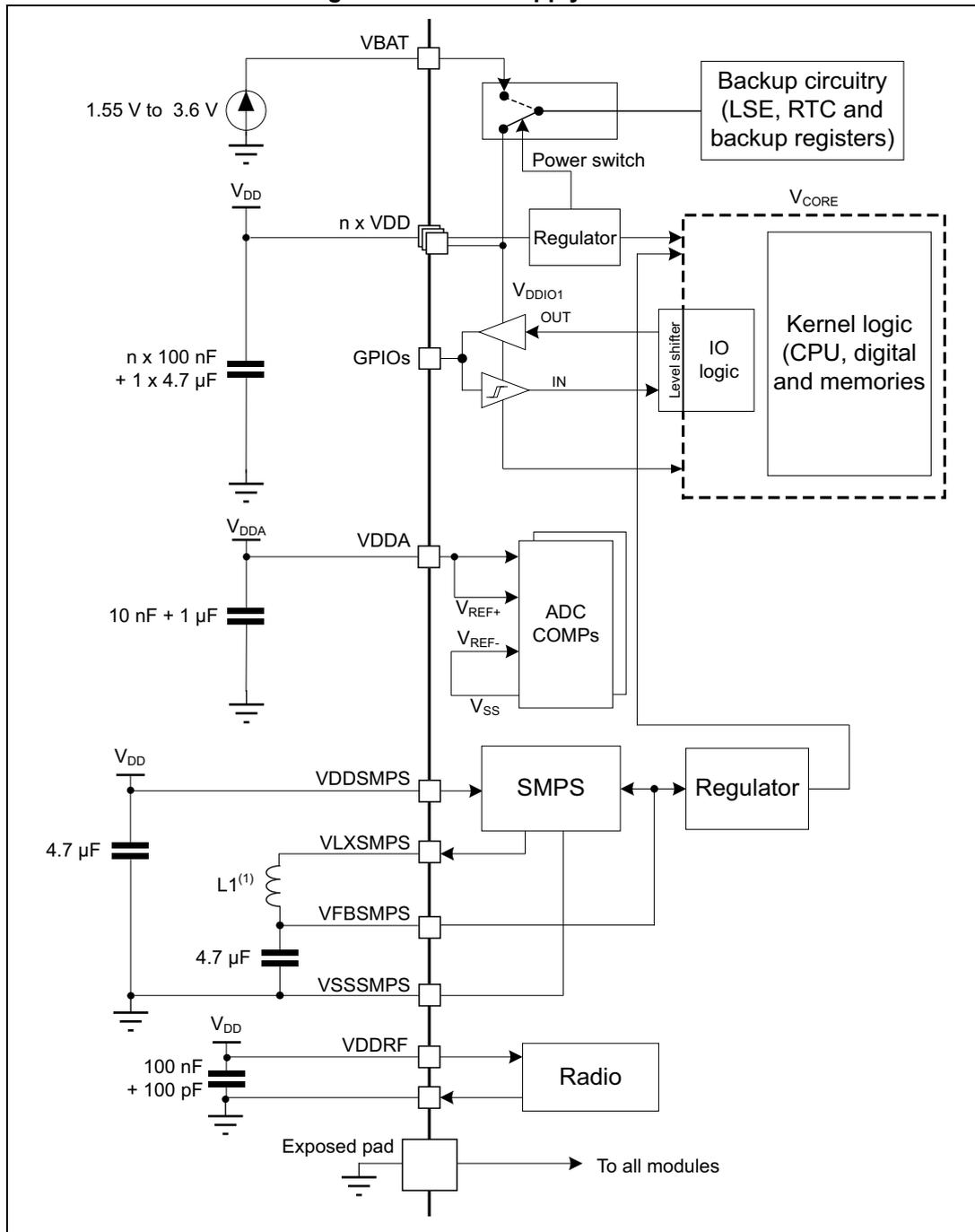
1. The value of L1 depends upon the frequency, as indicated in [Table 5: Power supply typical components](#).
