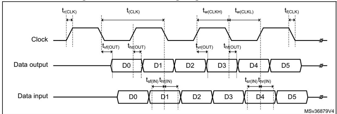
Figure 48. OCTOSPI hyperbus clock
