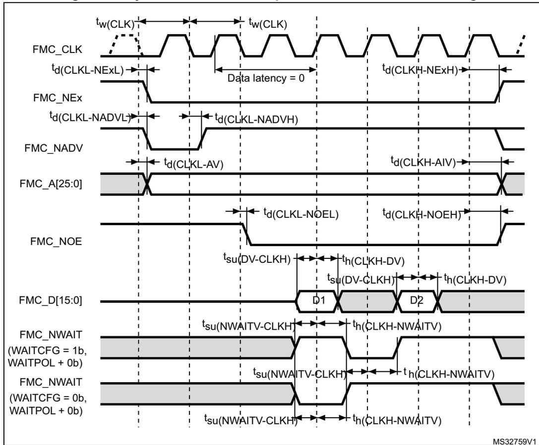
Table 77. Synchronous non-multiplexed NOR/PSRAM read timings<sup>(1)</sup>
