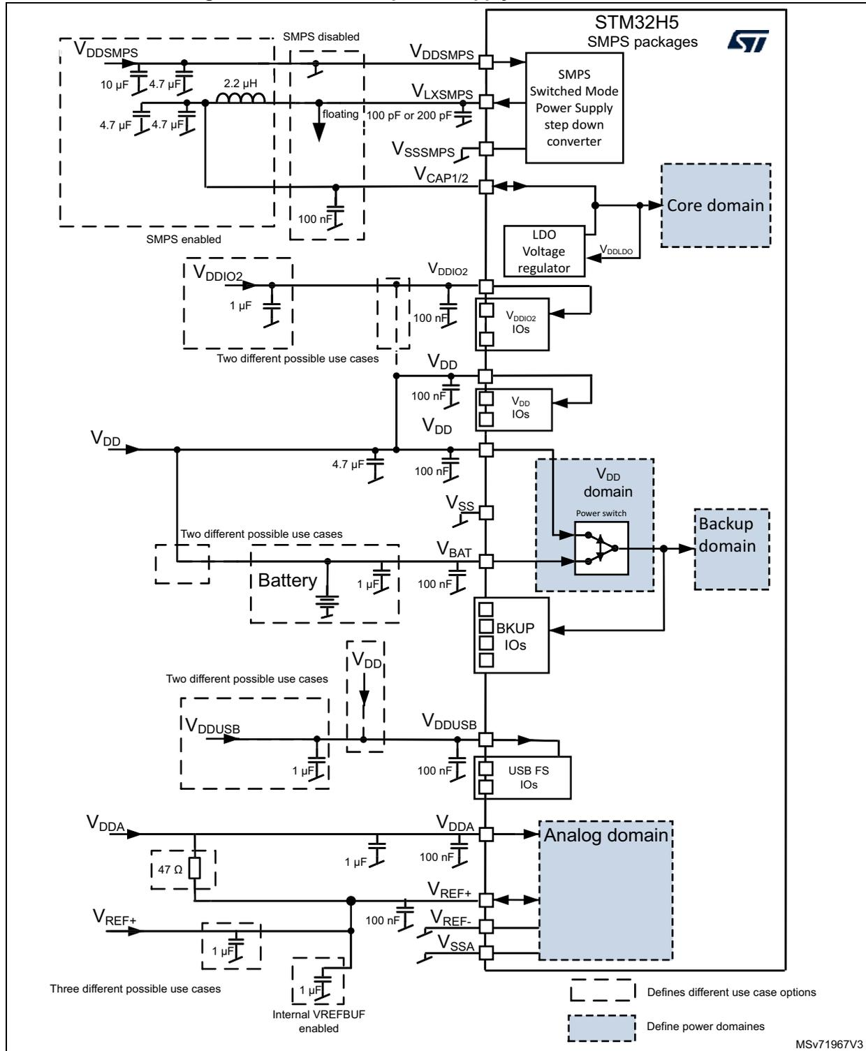
Figure 21. STM32H562/H563 power supply scheme with LDO
