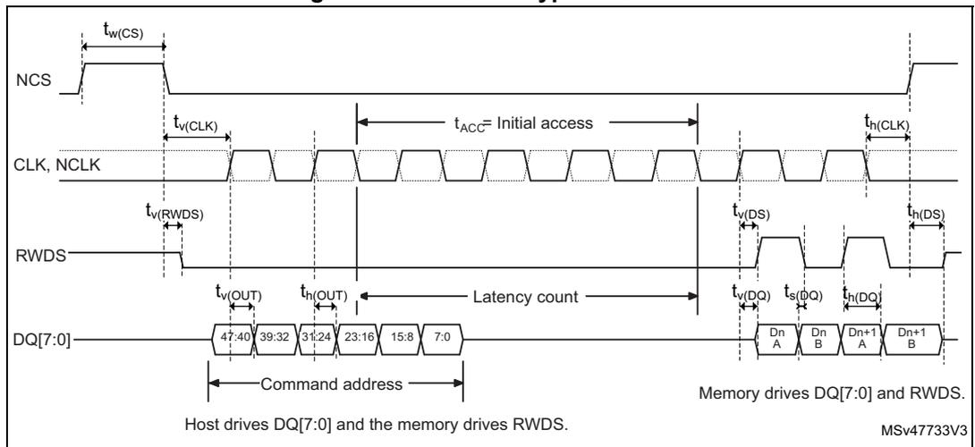
Figure 50. OCTOSPI hyperbus write
