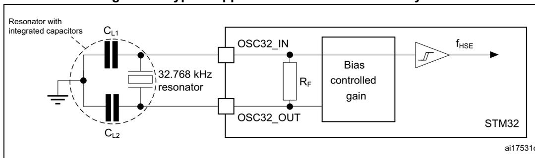
Note: An external resistor is not required between OSC32\_IN and OSC32\_OUT and it is forbidden to add one.
