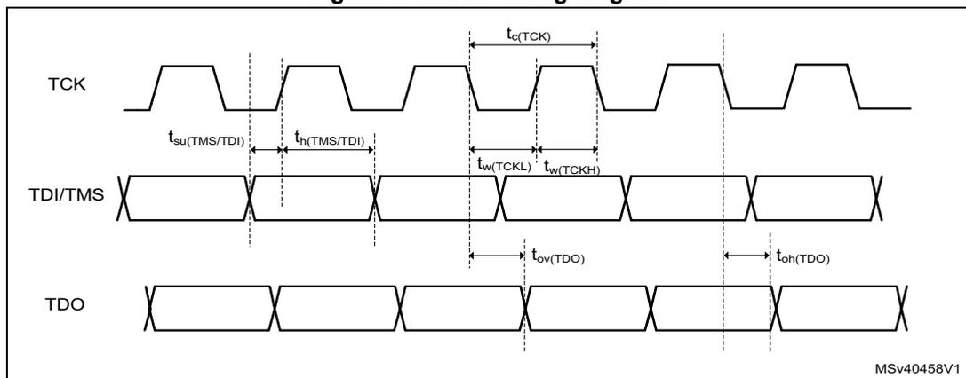
Figure 76. SWD timing diagram
