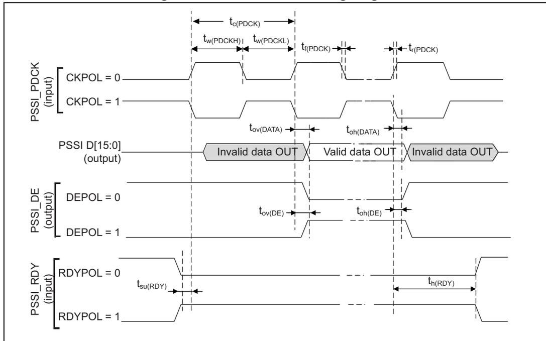
Figure 53. PSSI receive timing diagram
