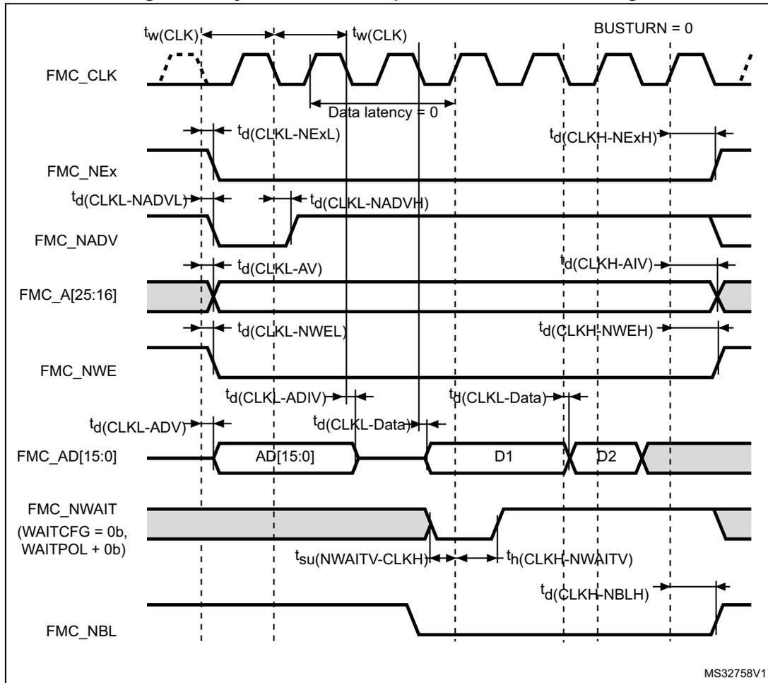
**Table 76. Synchronous multiplexed PSRAM write timings<sup>(1)</sup>**
