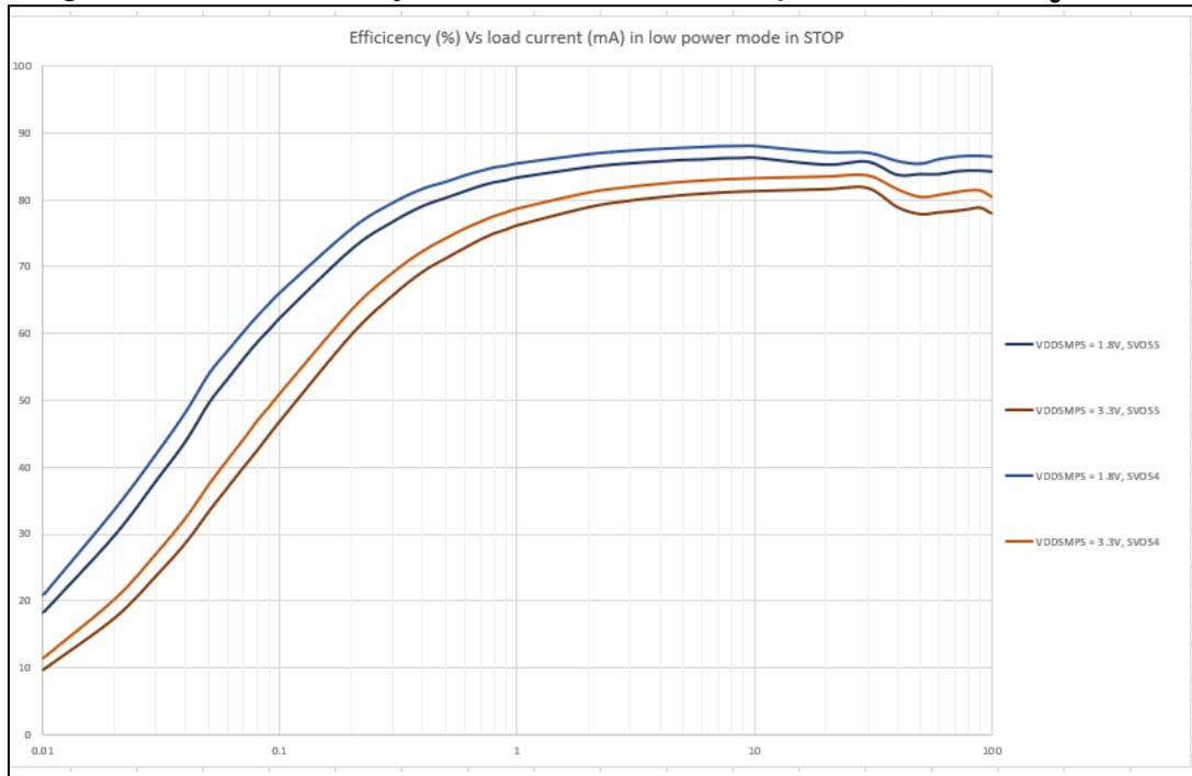
Figure 26. SMPS efficiency versus load current in stop SVOV4, SVOS5,  $T_J = 130\text{ }^\circ\text{C}$
