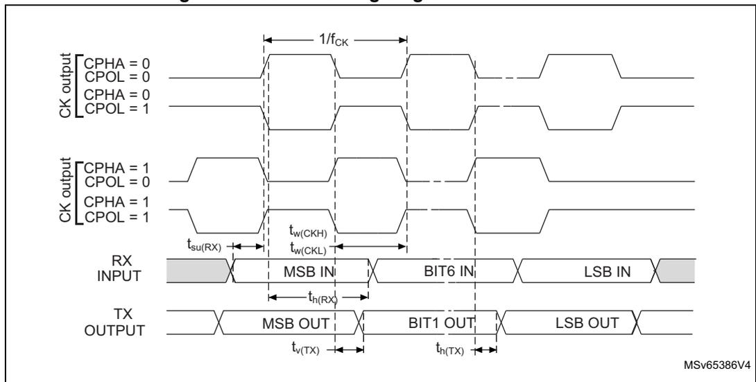
1. Measurement points are done at 0.5V<sub>DD</sub> and with external C<sub>L</sub> = 30 pF.
