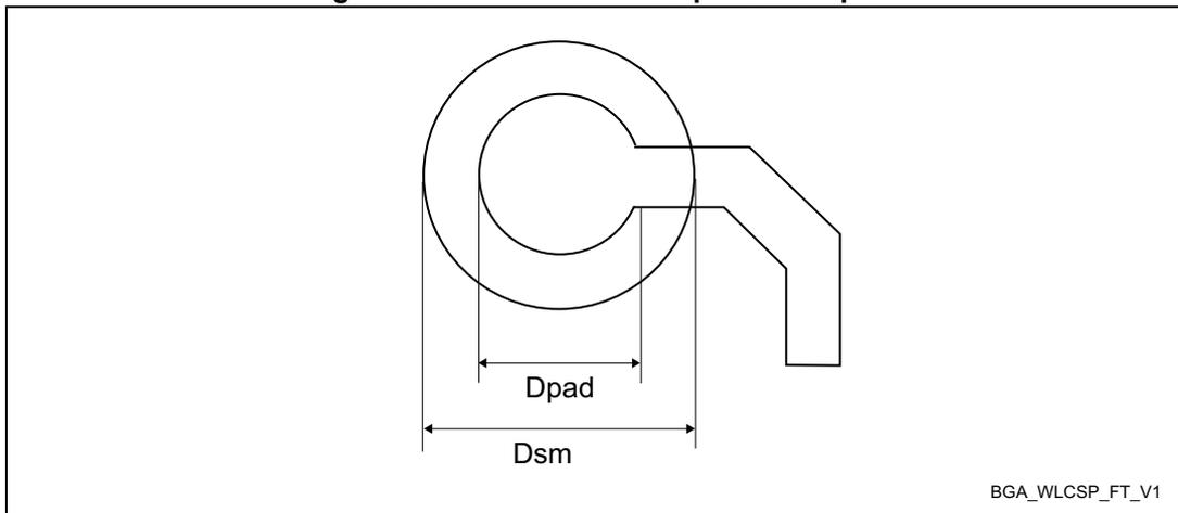
**Table 129. UFBGA169 - Example of PCB design rules (0.5 mm pitch BGA)**
