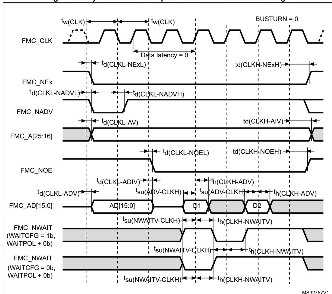
**Table 75. Synchronous multiplexed NOR/PSRAM read timings<sup>(1)</sup>**
