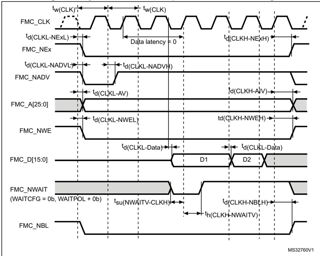
**Table 78. Synchronous non-multiplexed PSRAM write timings<sup>(1)</sup>**
