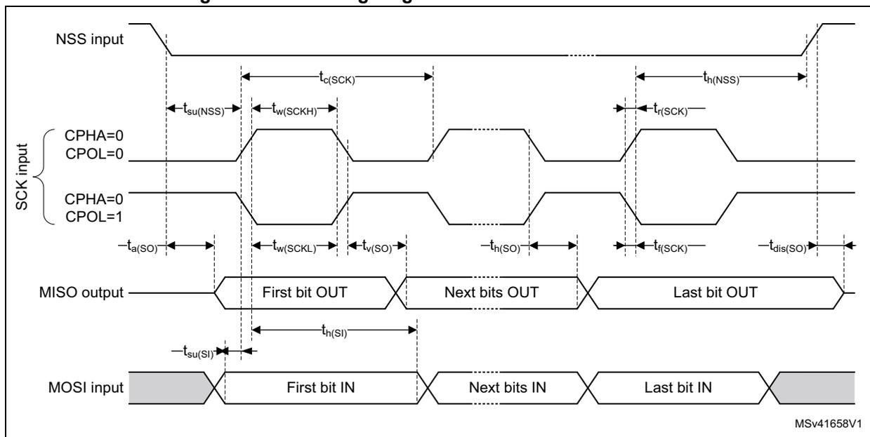
Figure 28. SPI timing diagram - slave mode and CPHA = 1<sup>(1)</sup>
