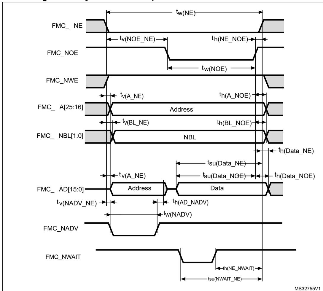
**Table 71. Asynchronous multiplexed PSRAM/NOR read timings<sup>(1)</sup>**
