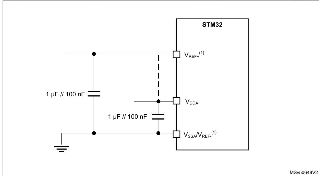
1.  $V_{REF+}$  input is not available on all packages (refer to [Table 14](#)),  $V_{REF-}$  is available only on UFBGA176+25, UFBGA169 with SMPS, LQFP100, UFBGA169, and UFBGA176+25 packages. When  $V_{REF-}$  is not available, it is internally connected to  $V_{SSA}$ .
