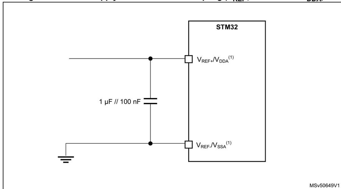
1.  $V_{REF+}$  input is not available on all packages (refer to [Table 14](#)),  $V_{REF-}$  is available only on UFBGA176+25, UFBGA169 with SMPS, LQFP100, UFBGA169, and UFBGA176+25 packages. When  $V_{REF-}$  is not available, it is internally connected to  $V_{SSA}$ . If  $V_{REF-}$  is available and connected to  $V_{DDA}$ , refer to [Figure 20](#) for more details.
