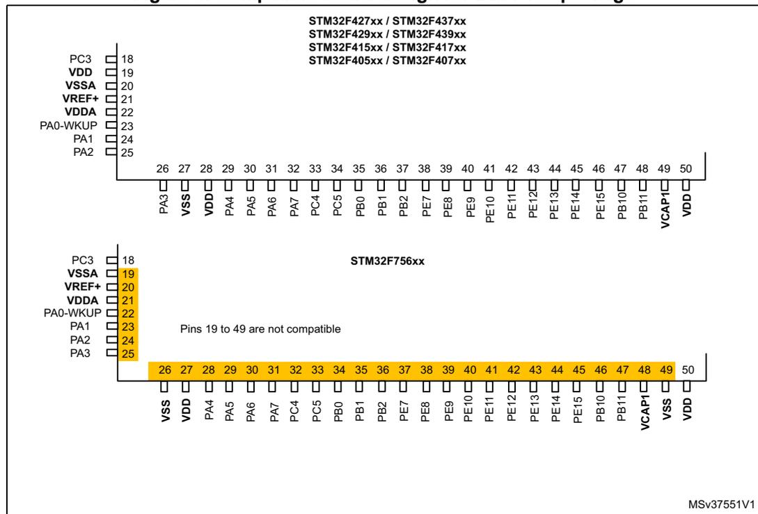
The STM32F756xx LQFP144, LQFP176, LQFP208, TFBGA216, UFBGA176, WLCSP143 packages are fully pin to pin compatible with STM32F4xxxx devices.
