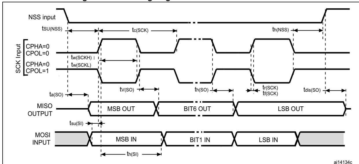
Figure 46. SPI timing diagram - slave mode and CPHA = 1<sup>(1)</sup>
