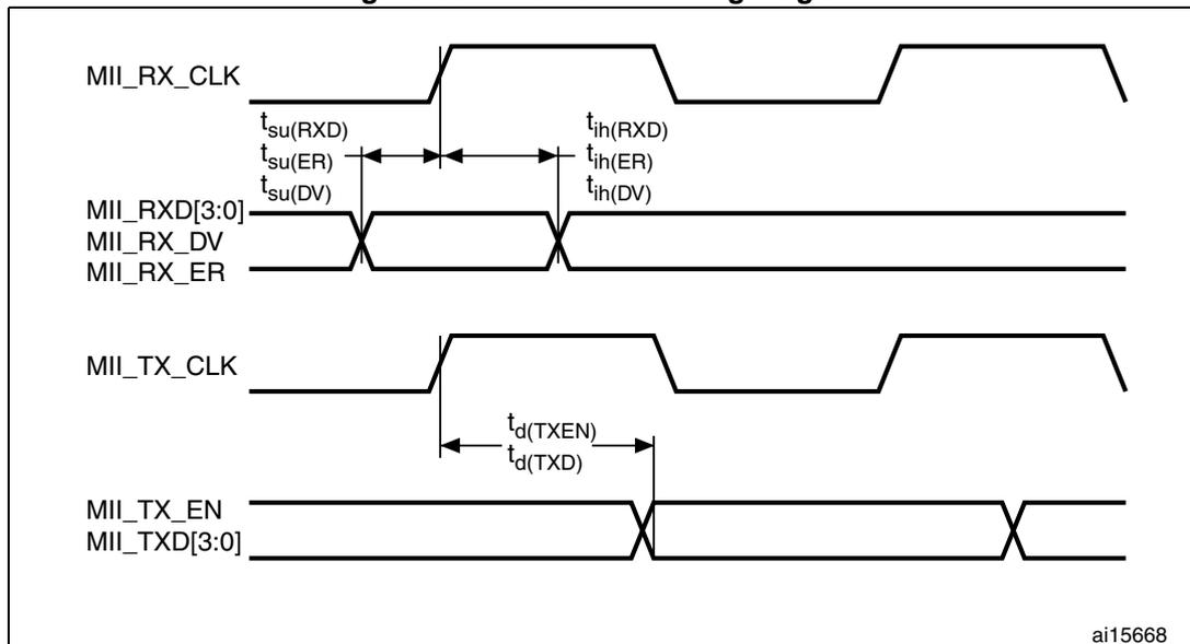
**Table 89. Dynamics characteristics: Ethernet MAC signals for MII<sup>(1)</sup>**
