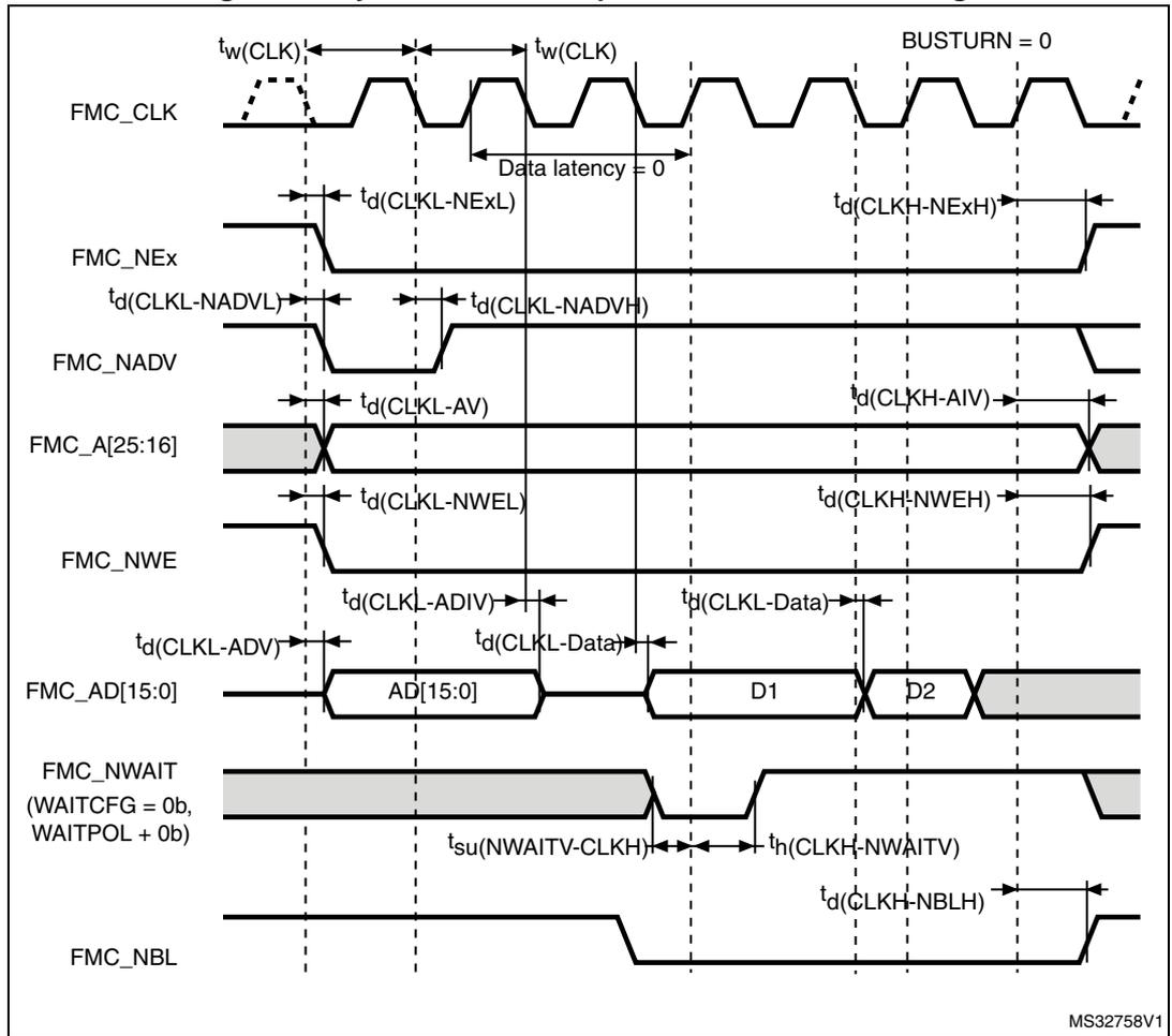
**Table 99. Synchronous multiplexed PSRAM write timings<sup>(1)</sup>**
