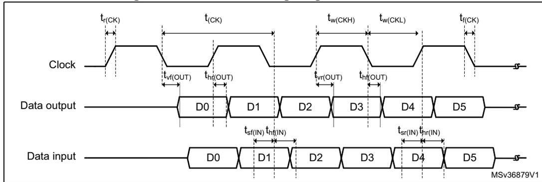
5.3.29 Camera interface (DCMI) timing specifications
