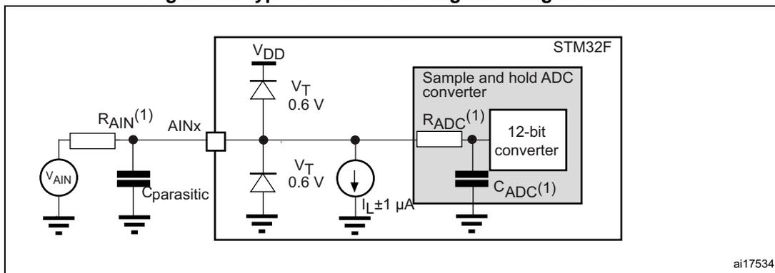
1. Refer to [Table 63](#) for the values of  $R_{AIN}$ ,  $R_{ADC}$  and  $C_{ADC}$ .
