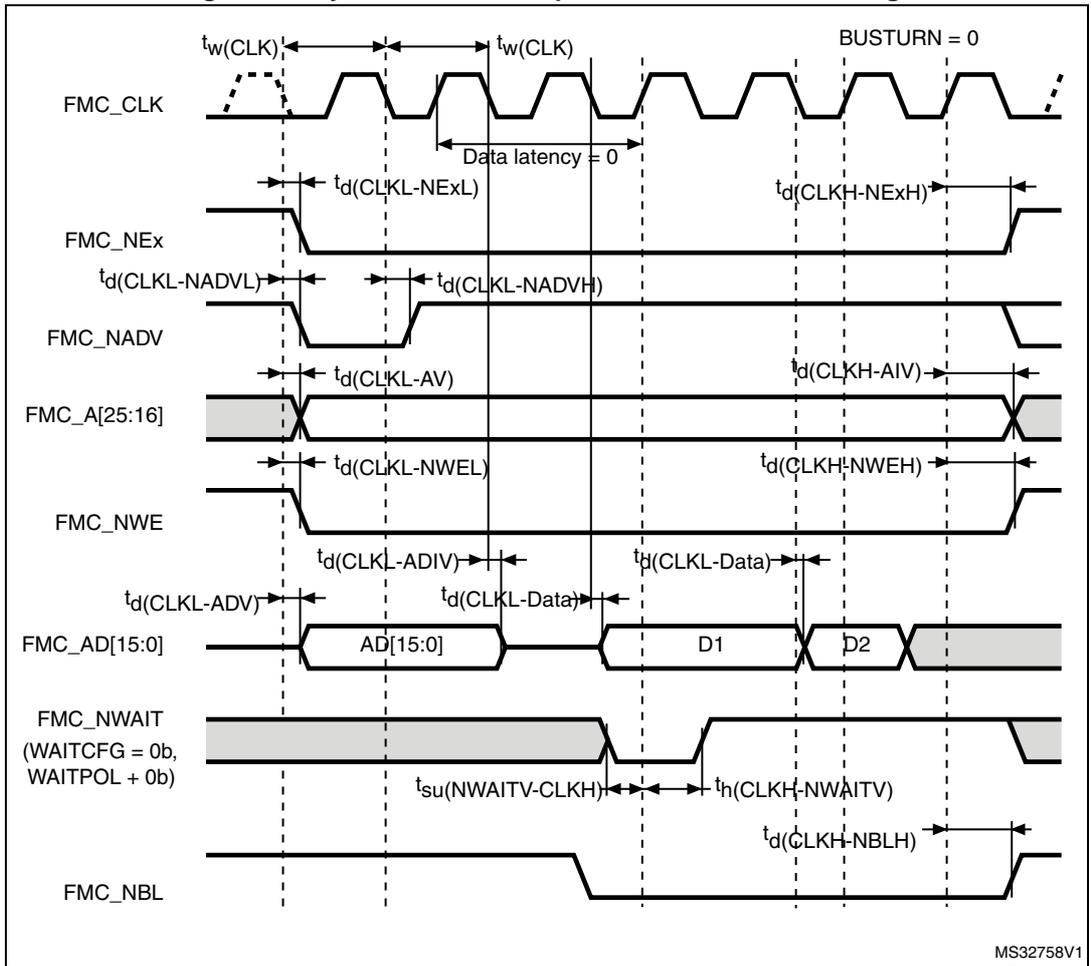
**Table 99. Synchronous multiplexed PSRAM write timings<sup>(1)</sup>**
