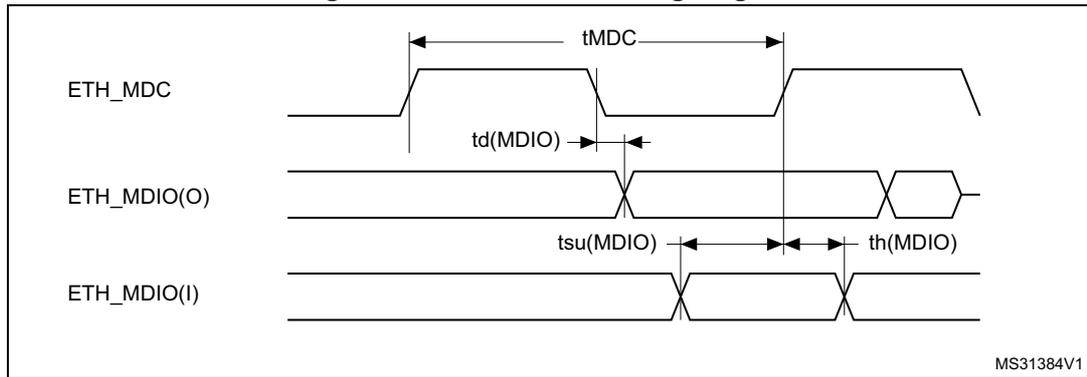
Table 87. Dynamics characteristics: Ethernet MAC signals for SMI<sup>(1)</sup>
