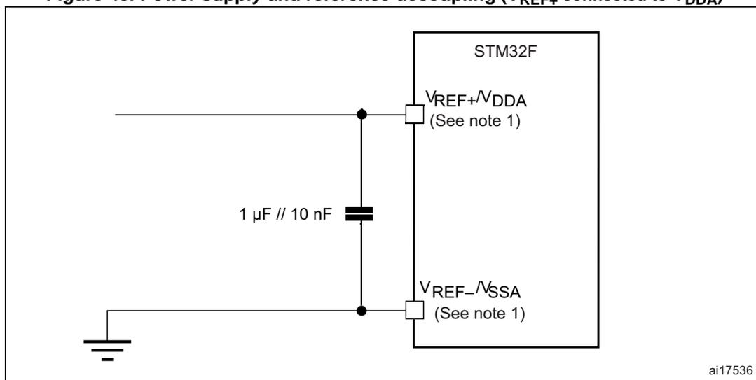
1.  $V_{REF+}$  input is available on all package whereas the  $V_{REF-}$  is available only on UFBGA176 and TFBGA216. When  $V_{REF-}$  is not available, it is internally connected to  $V_{DDA}$  and  $V_{SSA}$ .
