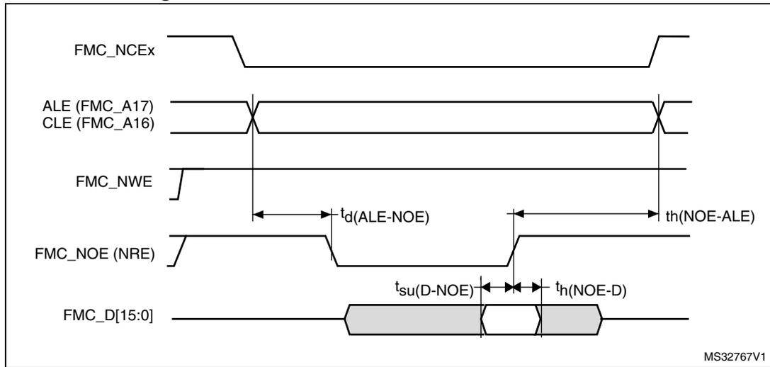
Figure 66. NAND controller waveforms for write access
