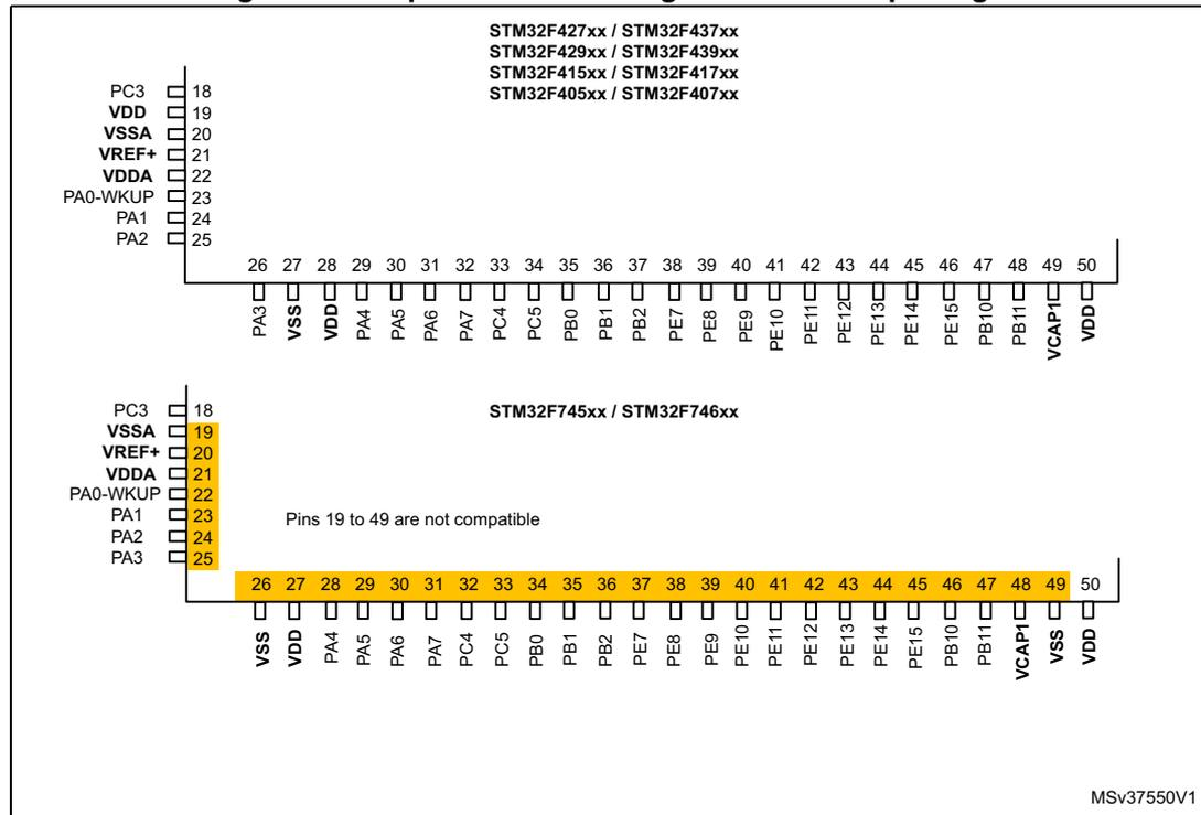
The STM32F745xx and STM32F746xx LQFP144, LQFP176, LQFP208, TFBGA216, UFBGA176, WLCSP143 packages are fully pin to pin compatible with STM32F4xxxx devices.
