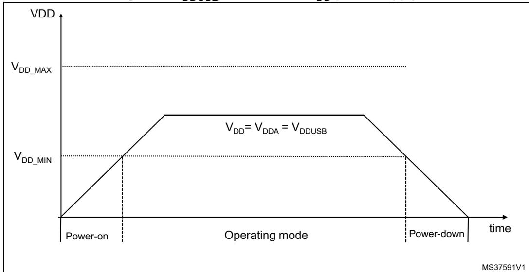
Figure 5.  $V_{DDUSB}$  connected to external power supply
