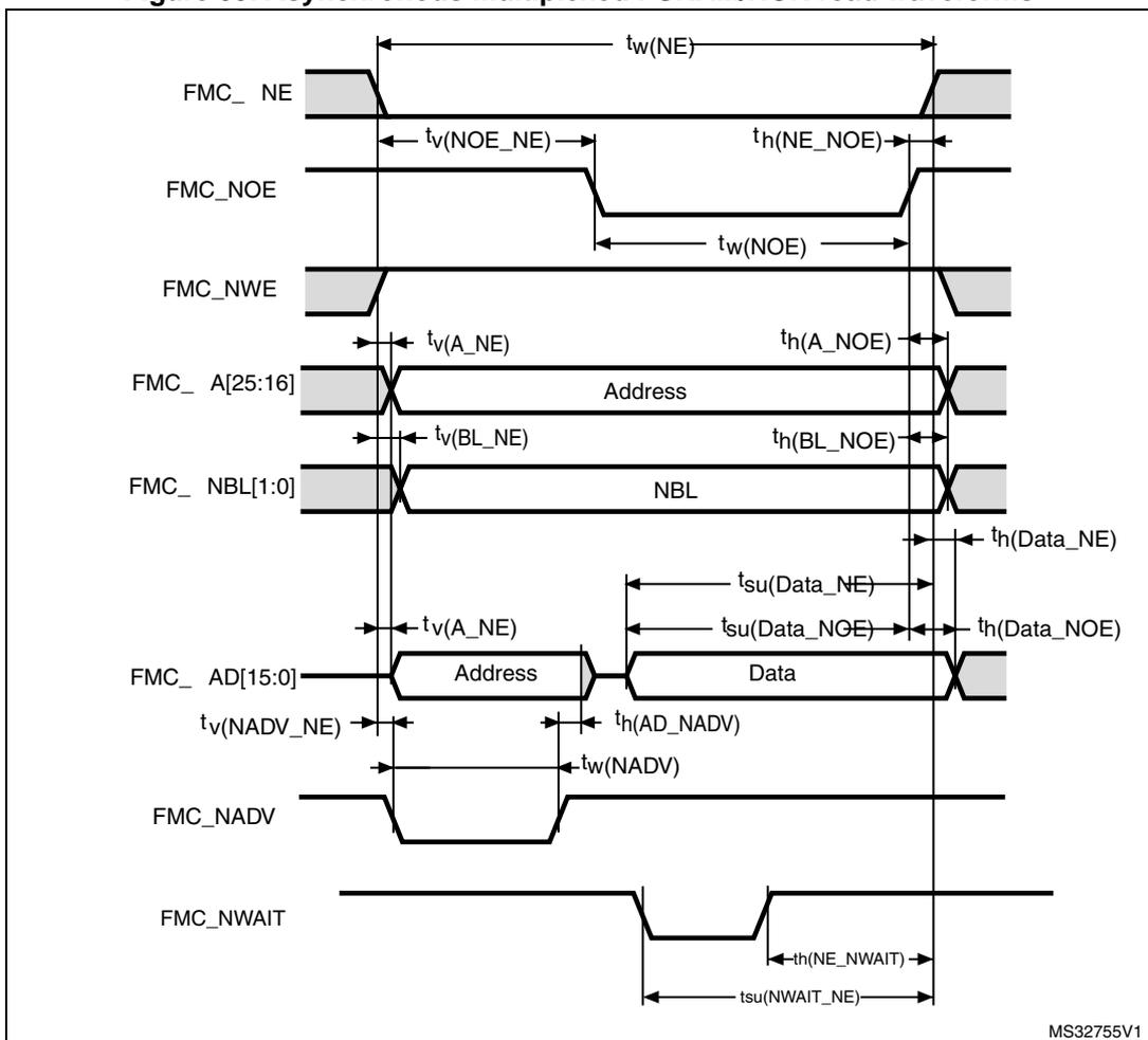
**Table 94. Asynchronous multiplexed PSRAM/NOR read timings<sup>(1)</sup>**
