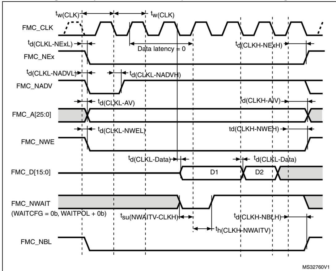
Table 101. Synchronous non-multiplexed PSRAM write timings<sup>(1)</sup>
