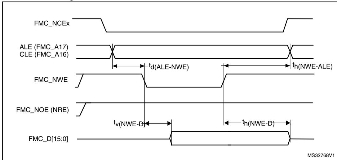
Figure 67. NAND controller waveforms for common memory read access
