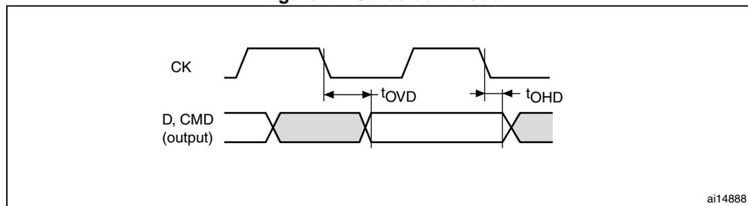
Table 112. Dynamic characteristics: SD / MMC characteristics,  $V_{DD}=2.7V$  to  $3.6V^{(1)}$
