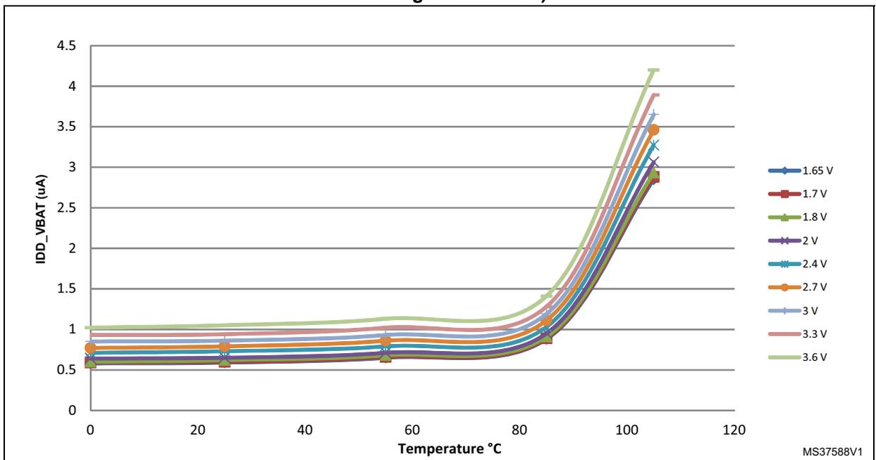
Figure 28. Typical  $V_{BAT}$  current consumption (RTC ON/BKP SRAM OFF and LSE in high medium drive mode)
