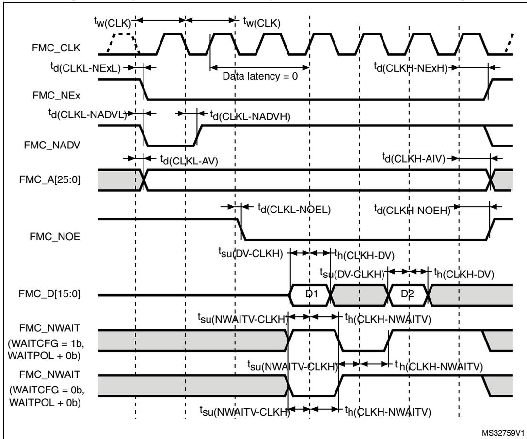
Table 100. Synchronous non-multiplexed NOR/PSRAM read timings<sup>(1)</sup>
