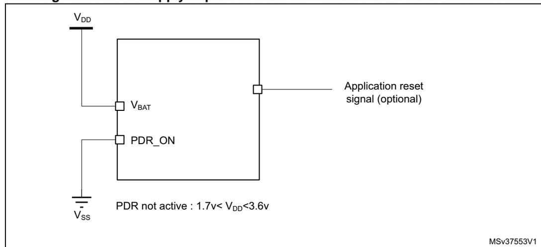
The  $V_{DD}$  specified threshold, below which the device must be maintained under reset, is 1.7 V (see [Figure 7](#)).
