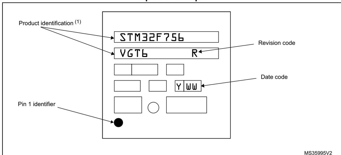
1. Parts marked as “ES”, “E” or accompanied by an Engineering Sample notification letter, are not yet qualified and therefore not yet ready to be used in production and any consequences deriving from such usage will not be at ST charge. In no event, ST will be liable for any customer usage of these engineering samples in production. ST Quality has to be contacted prior to any decision to use these Engineering samples to run qualification activity.
