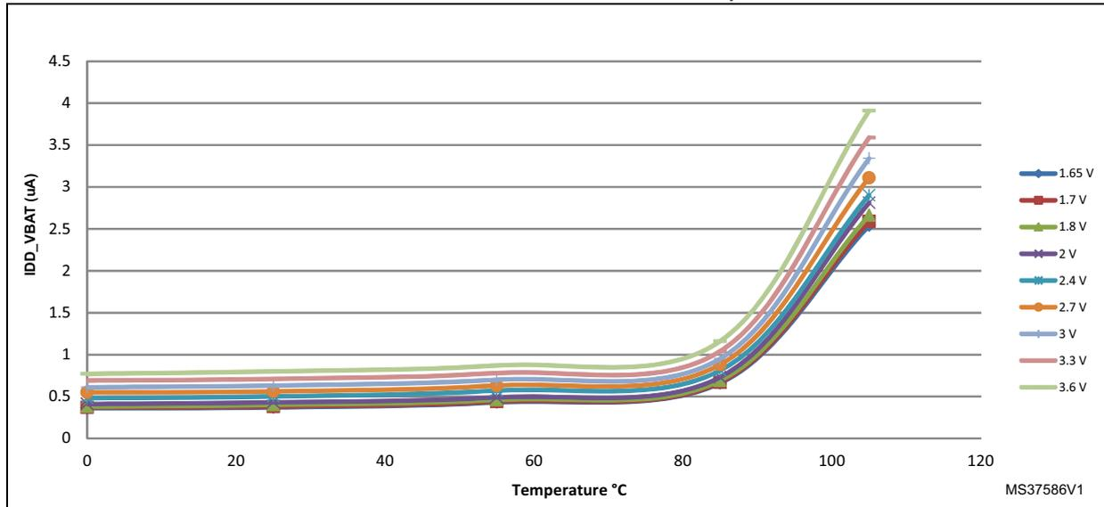
Figure 26. Typical  $V_{BAT}$  current consumption (RTC ON/BKP SRAM OFF and LSE in medium high drive mode)
