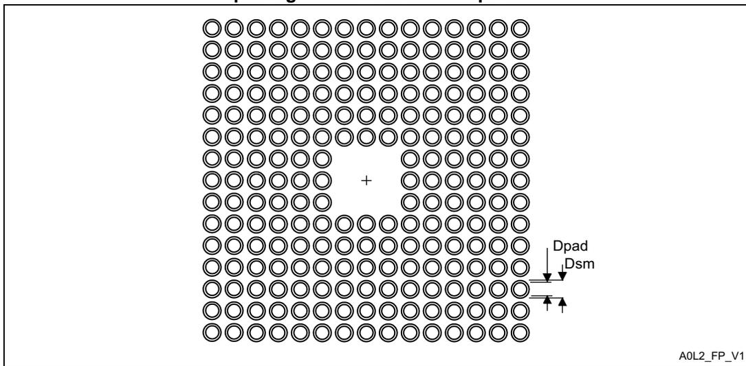
**Table 123. TFBGA216 recommended PCB design rules (0.8 mm pitch BGA)**
