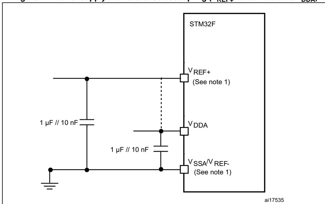
1.  $V_{REF+}$  input is available on all package whereas the  $V_{REF-}$  is available only on UFBGA176 and TFBGA216. When  $V_{REF-}$  is not available, it is internally connected to  $V_{DDA}$  and  $V_{SSA}$ .
