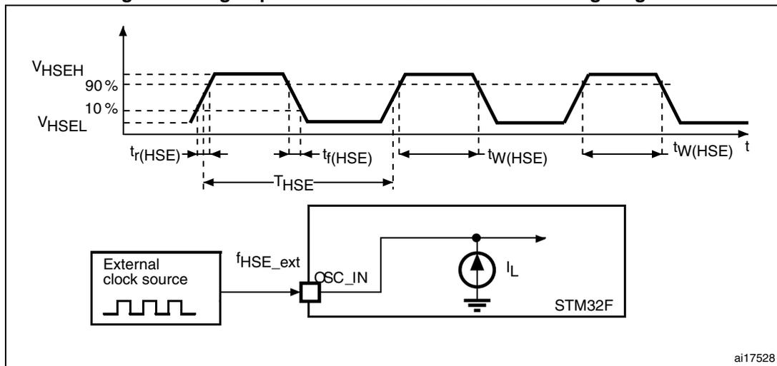
Figure 30. Low-speed external clock source AC timing diagram
