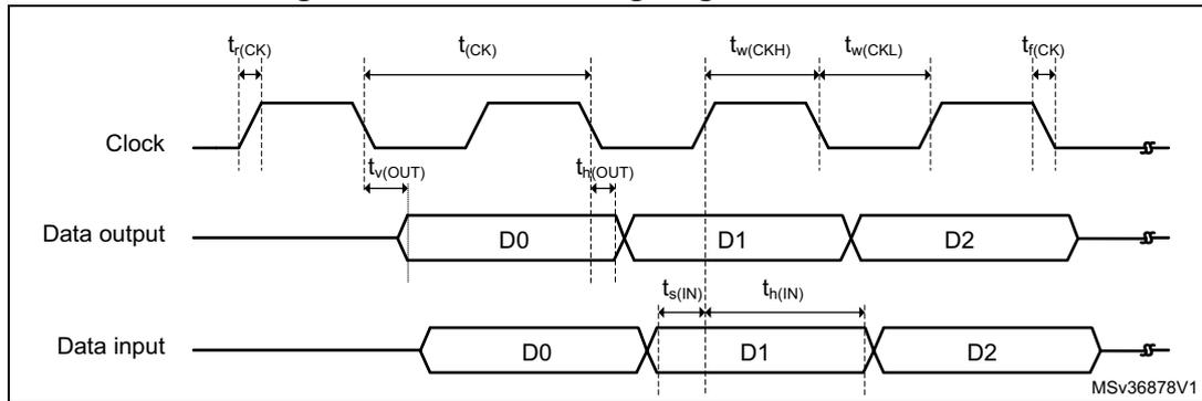
Figure 72. Quad SPI timing diagram - DDR mode
