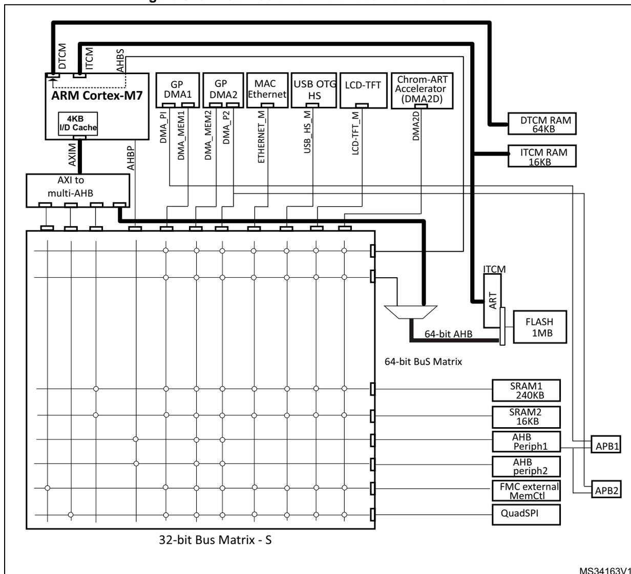
1. The above figure has large wires for 64-bits bus and thin wires for 32-bits bus.
