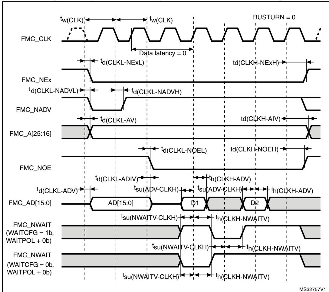
Table 98. Synchronous multiplexed NOR/PSRAM read timings<sup>(1)</sup>
