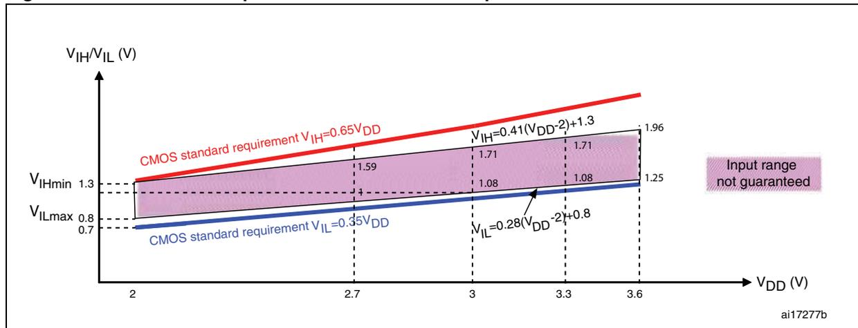
Figure 19. Standard I/O input characteristics - TTL port
