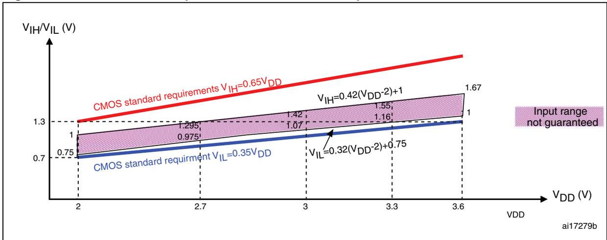
Figure 25. 5 V tolerant I/O input characteristics - TTL port
