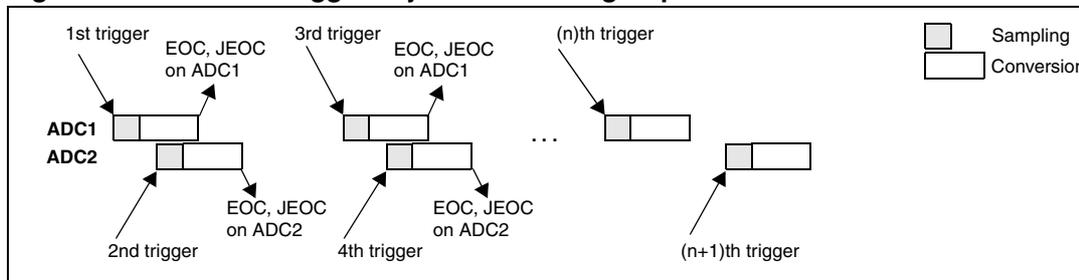
If the injected discontinuous mode is enabled for both ADC1 and ADC2:
