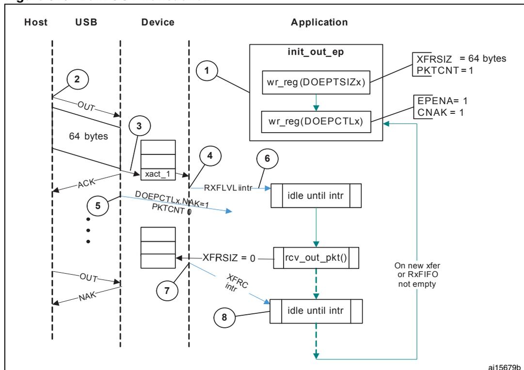
After a SetConfiguration/SetInterface command, the application initializes all OUT endpoints by setting CNAK = 1 and EPENA = 1 (in OTG\_FS\_DOEPCTLx), and setting a suitable XFRSIZ and PKTCNT in the OTG\_FS\_DOEPSIZx register.
