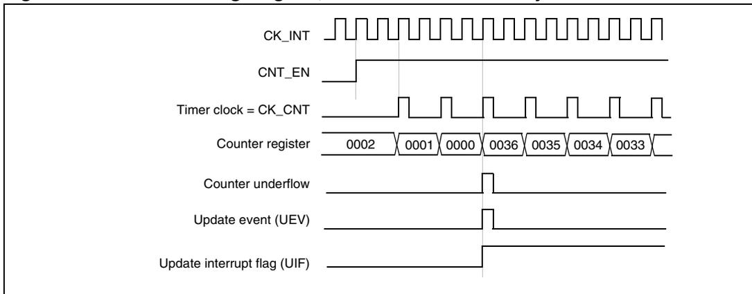
**Figure 111. Counter timing diagram, internal clock divided by 4**
