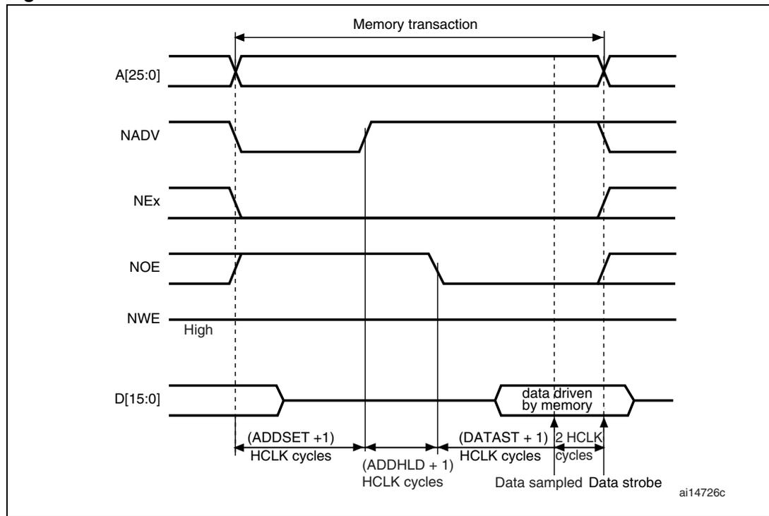
**ModeD write accesses** The differences with mode1 are the toggling of NADV, NOE that
