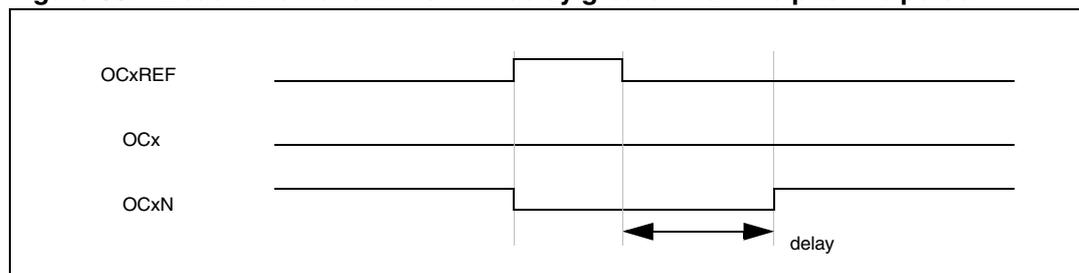
The dead-time delay is the same for each of the channels and is programmable with the DTG bits in the TIMx\_BDTR register. Refer to [Section 14.4.18: TIM1&TIM8 break and dead-time register \(TIMx\\_BDTR\) on page 344](#) for delay calculation.
