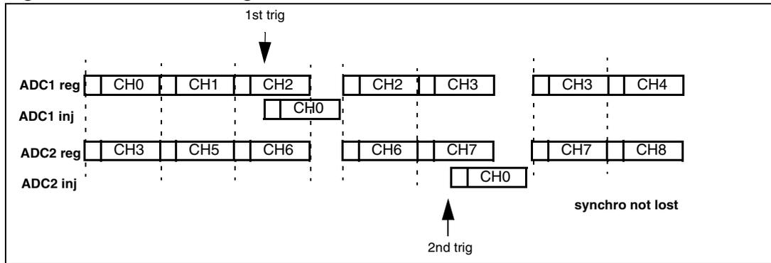
If a trigger occurs during an injected conversion that has interrupted a regular conversion, it will be ignored. [Figure 37](#) shows the behavior in this case (2nd trig is ignored).
