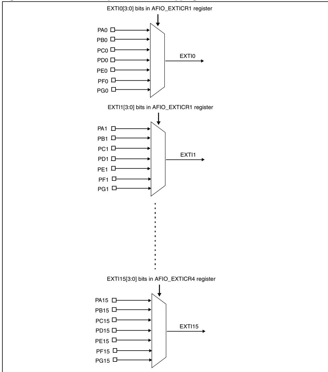
1. To configure the AFIO\_EXTICRx for the mapping of external interrupt/event lines onto GPIOs, the AFIO clock should first be enabled. Refer to [Section 7.3.7: APB2 peripheral clock enable register \(RCC\\_APB2ENR\)](#) for low-, medium-, high- and XL-density devices and, to [Section 8.3.7: APB2 peripheral clock enable register \(RCC\\_APB2ENR\)](#) for connectivity line devices.
