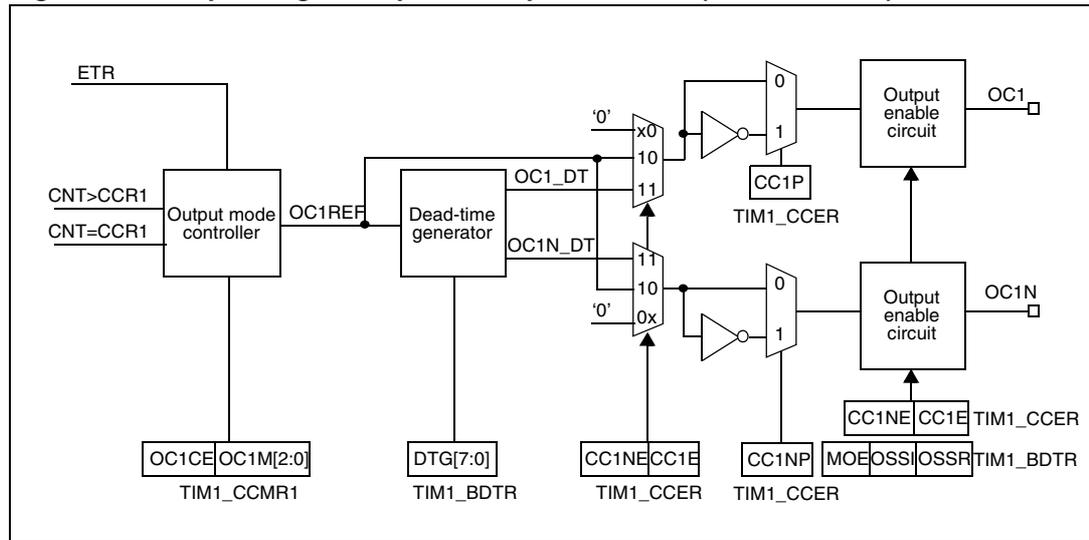
Figure 81. Output stage of capture/compare channel (channel 4)
