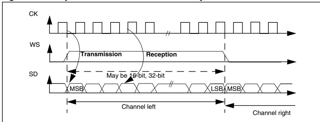
**Figure 258. LSB Justified 24-bit frame length with CPOL = 0**
