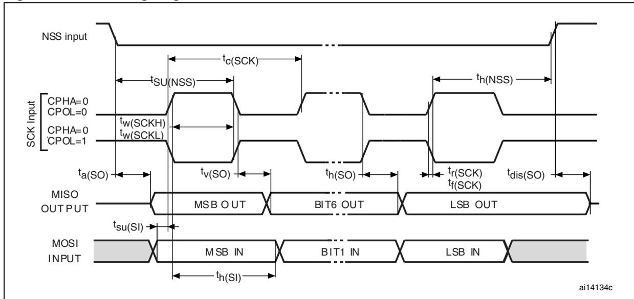
Figure 30. SPI timing diagram - slave mode and CPHA = 1<sup>(1)</sup>
