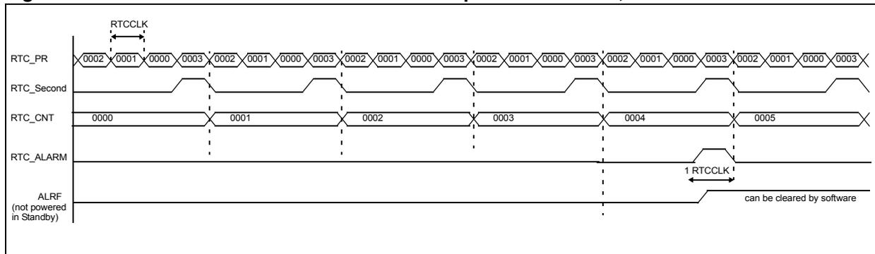
**Figure 181. RTC Overflow waveform example with PR=0003**
