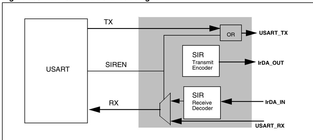
Figure 294. IrDA data modulation (3/16) -normal mode
