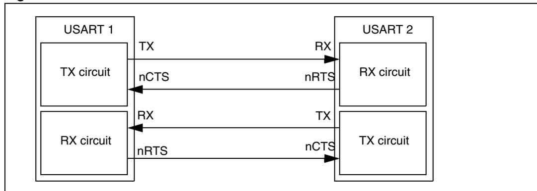
RTS and CTS flow control can be enabled independently by writing respectively RTSE and CTSE bits to 1 (in the USART\_CR3 register).
