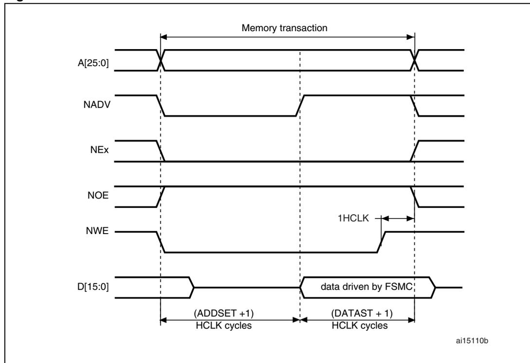
The differences with mode1 are the toggling of NADV and the independent read and write timings when extended mode is set (Mode B).
