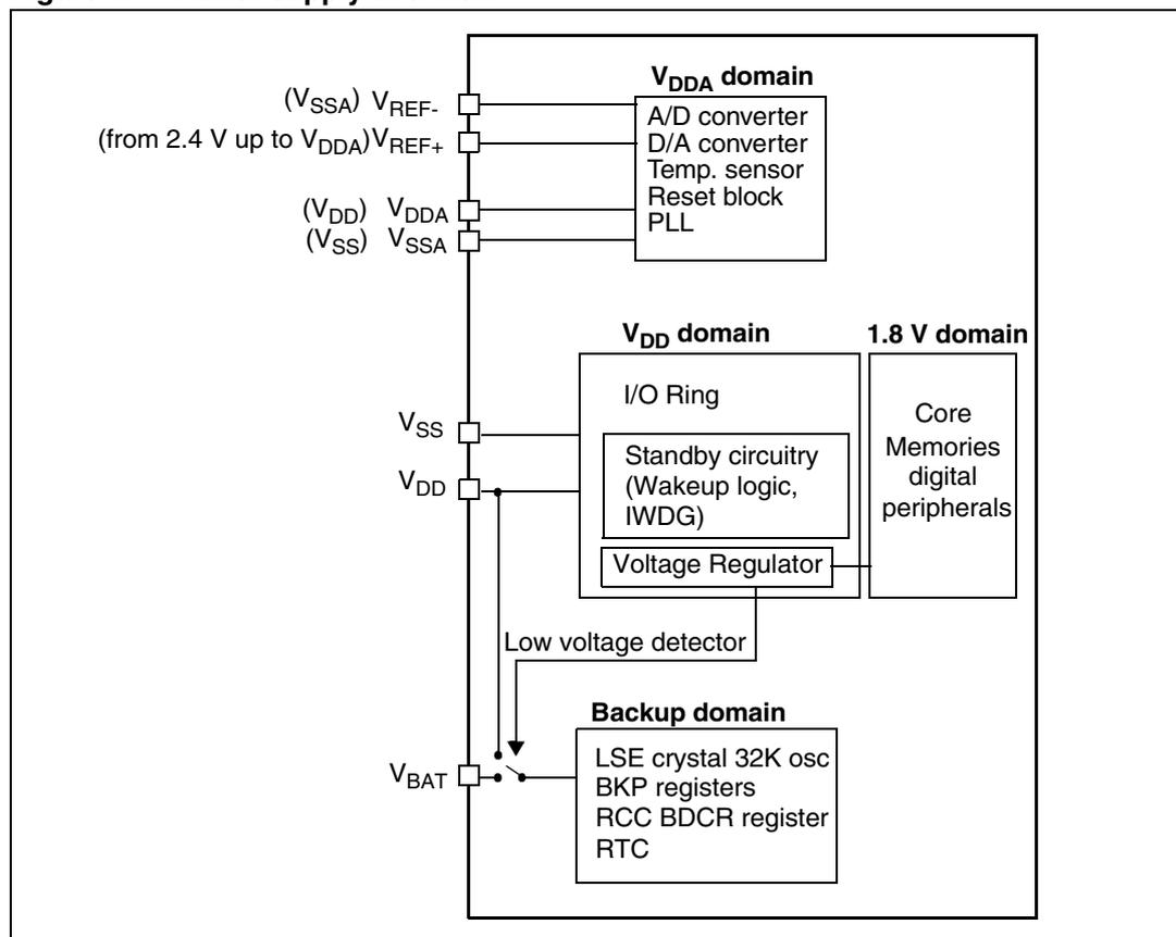
Note: 1  $V_{DDA}$  and  $V_{SSA}$  must be connected to  $V_{DD}$  and  $V_{SS}$ , respectively.
