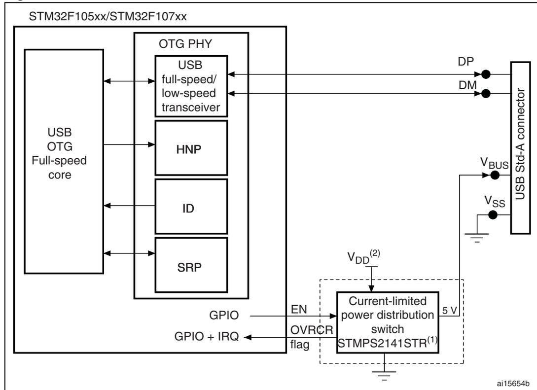
1. STMP2141STR needed only if the application has to support bus-powered devices.
