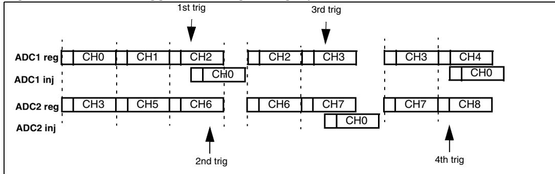
**11.9.9 Combined injected simultaneous + interleaved**
