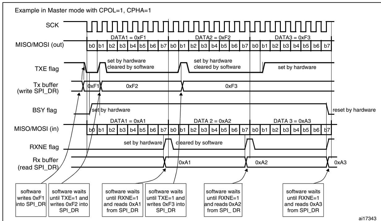
**Figure 240. TXE/RXNE/BSY behavior in Slave / full-duplex mode (BIDIMODE=0, RXONLY=0) in the case of continuous transfers**
