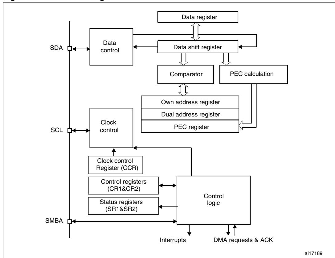
1. SMBA is an optional signal in SMBus mode. This signal is not applicable if SMBus is disabled.
