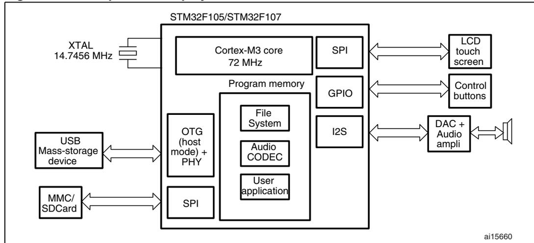
*Figure 54* shows storage media to audio Codec/amplifier streaming with SOF synchronization of input/output audio streaming using a hardware Codec.
