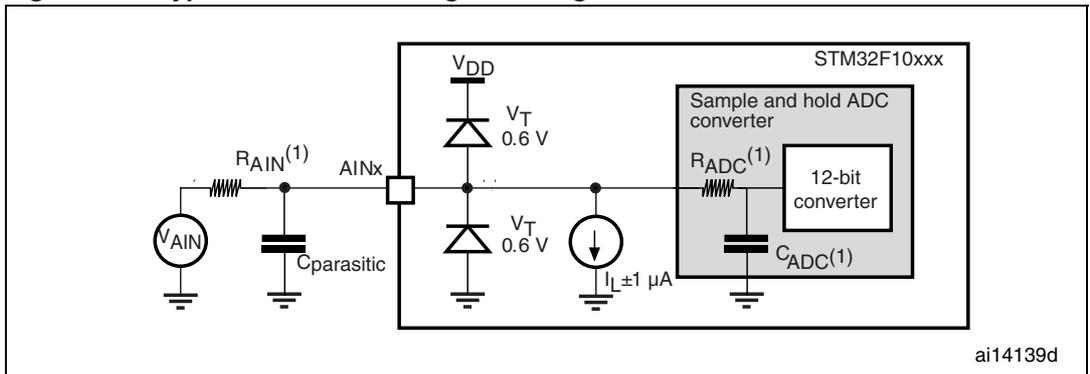
1. Refer to [Table 52](#) for the values of  $R_{\text{AIN}}$ ,  $R_{\text{ADC}}$  and  $C_{\text{ADC}}$ .
