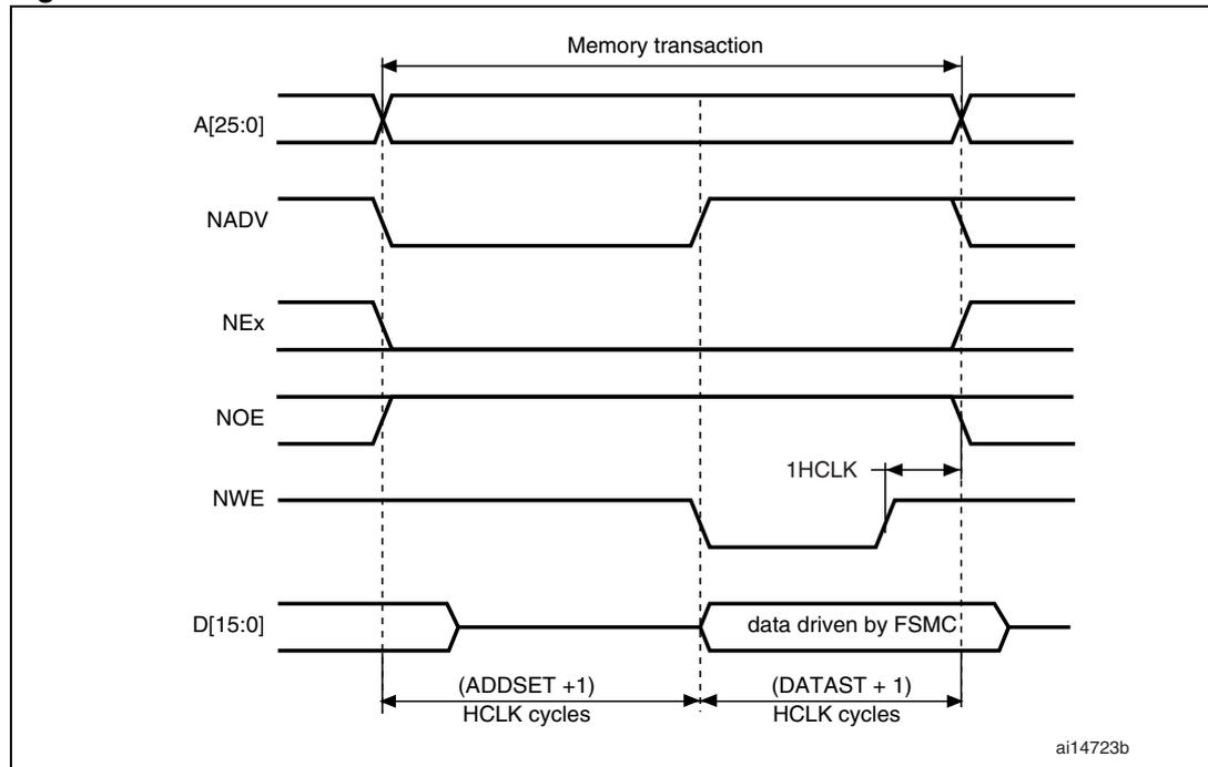
The differences compared with mode1 are the toggling of NOE and NADV and the independent read and write timings.
