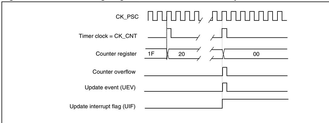
**Figure 59. Counter timing diagram, update event when ARPE=0 (TIMx\_ARR not preloaded)**
