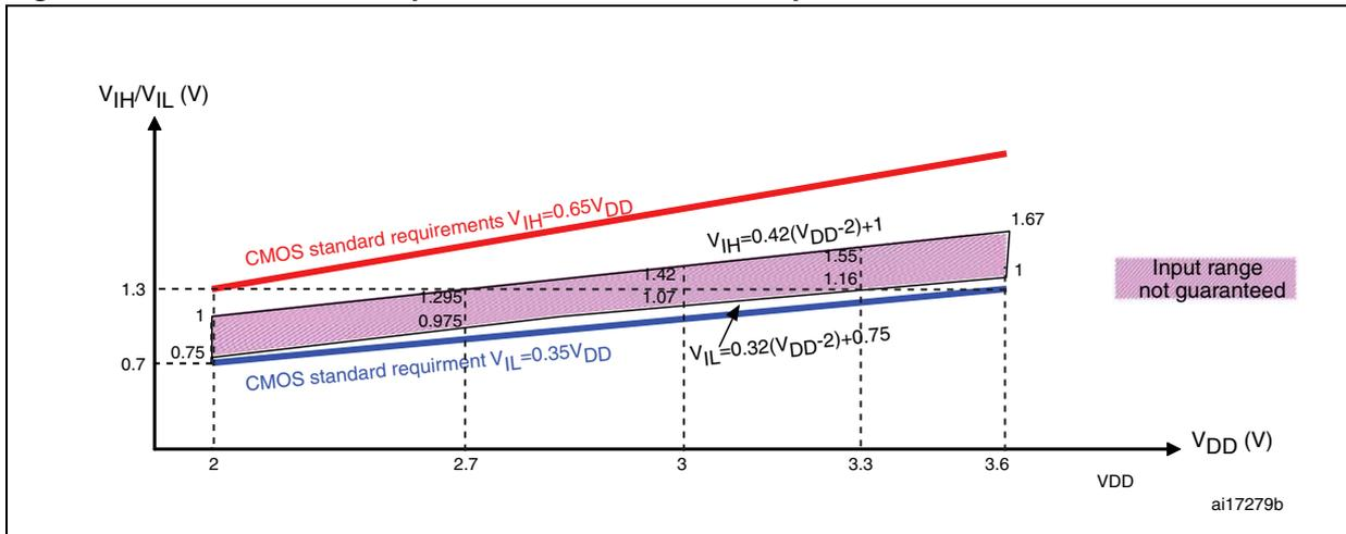
Figure 29. 5 V tolerant I/O input characteristics - TTL port
