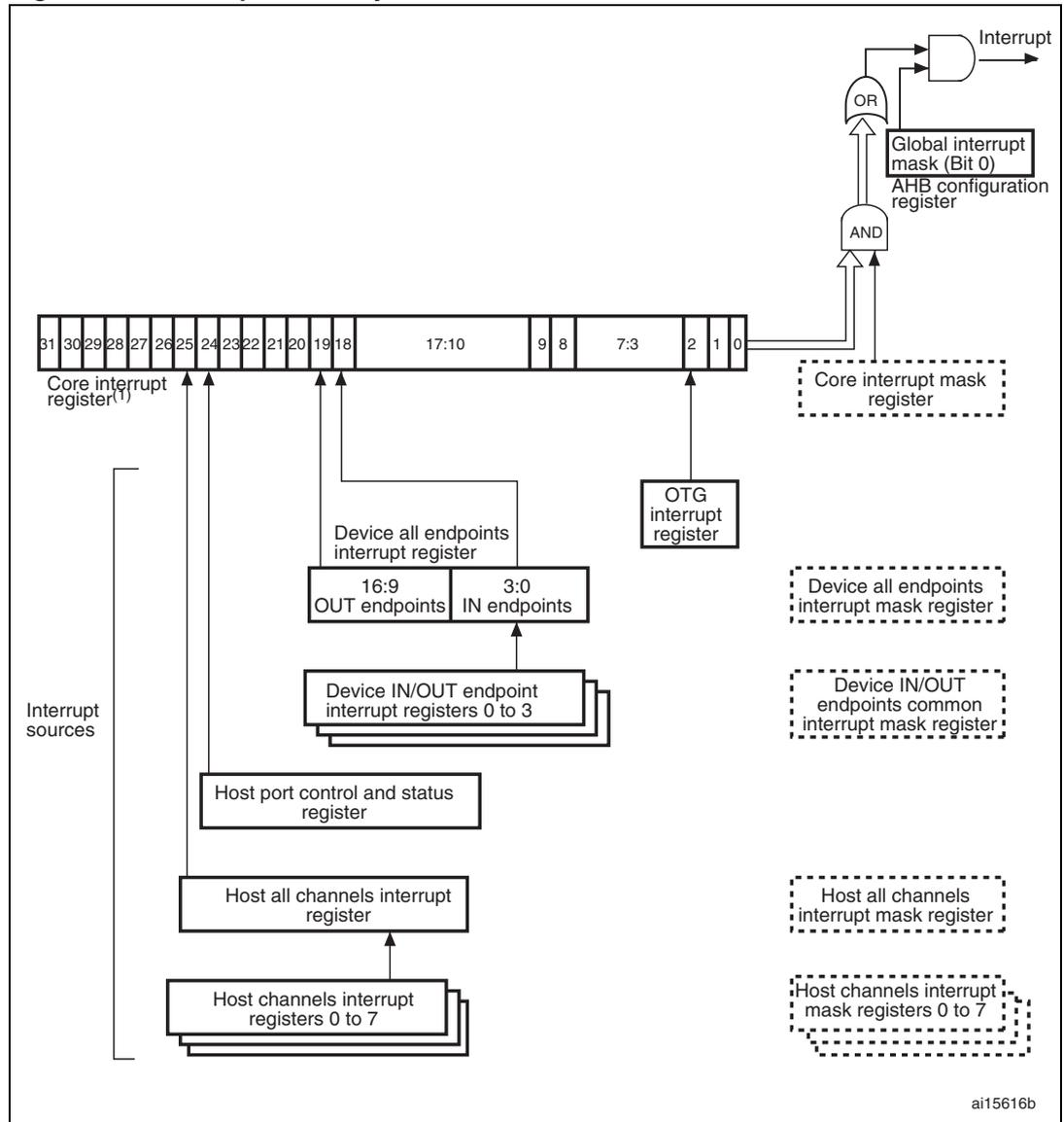
1. The core interrupt register bits are shown in *OTG\_FS core interrupt register (OTG\_FS\_GINTSTS)* on page 838.
