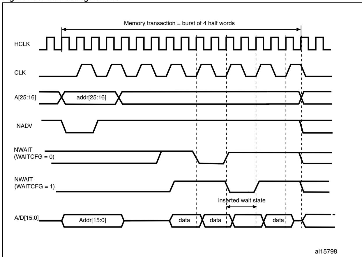
Figure 202. Synchronous multiplexed read mode - NOR, PSRAM (CRAM)
