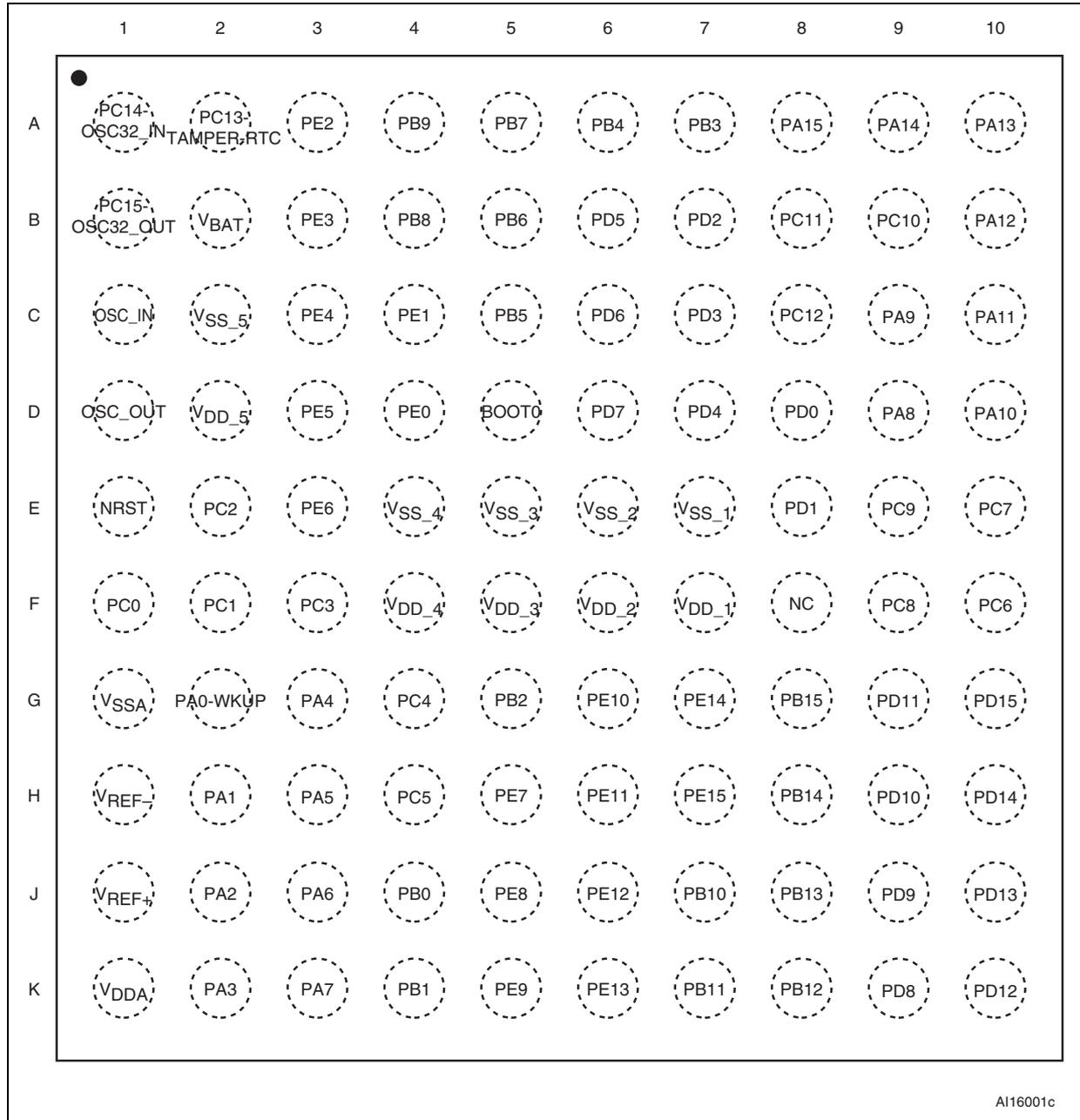
Figure 3. STM32F105xxx and STM32F107xxx connectivity line LQFP100 pinout
