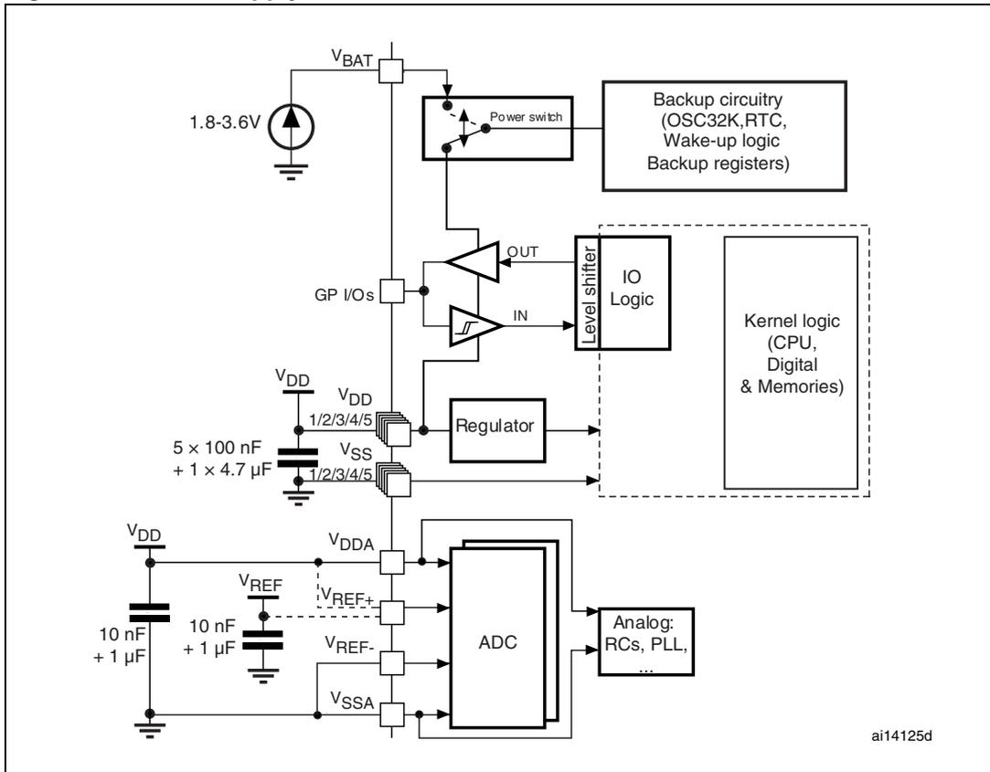
**Caution:** In [Figure 14](#), the 4.7 μF capacitor must be connected to V<sub>DD3</sub>.
