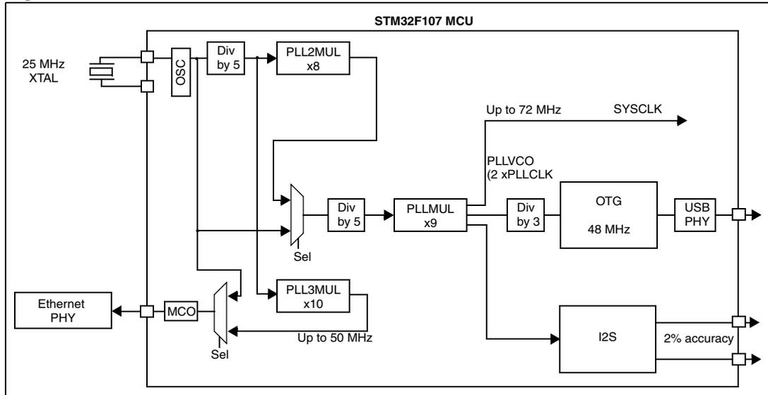
With the clock tree implemented on the STM32F107xx, only one crystal is required to work with both the USB (host/device/OTG) and the I<sup>2</sup>S (Audio) interfaces. *Figure 56* illustrate the solution.
