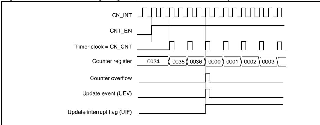
**Figure 105. Counter timing diagram, internal clock divided by 4**
