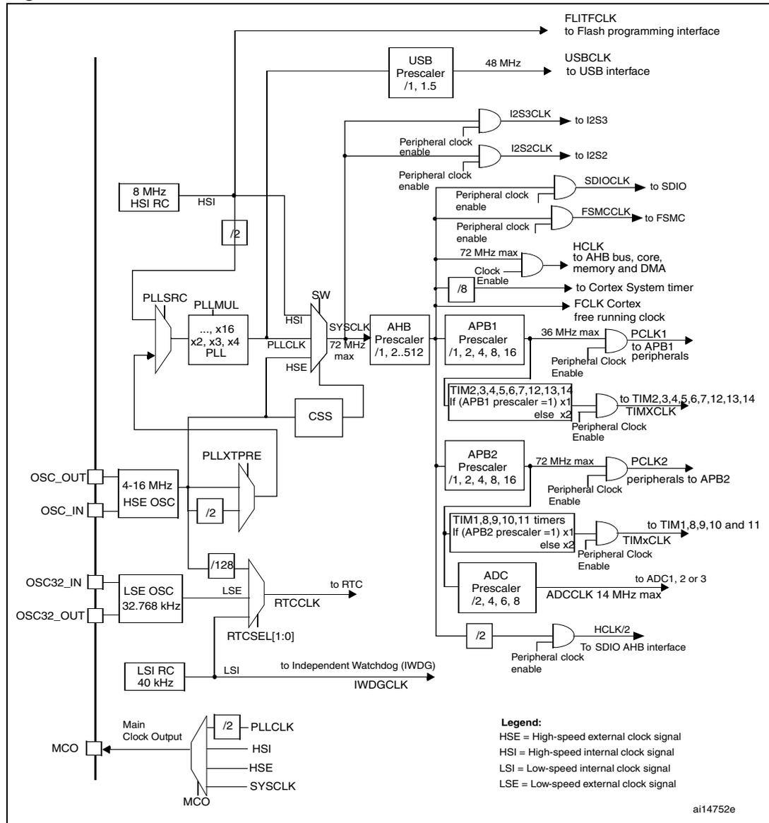
1. When the HSI is used as a PLL clock input, the maximum system clock frequency that can be achieved is 64 MHz.
