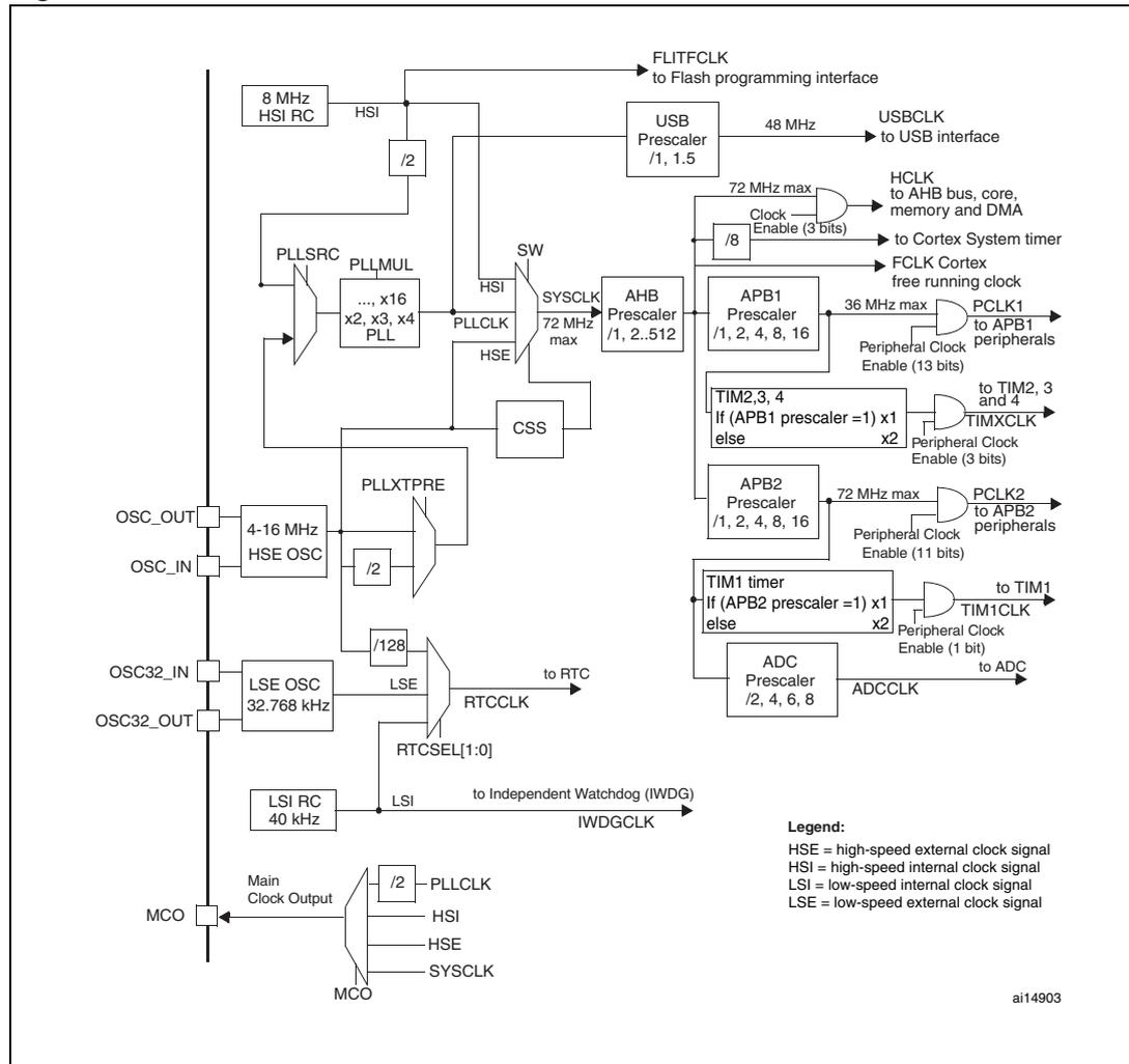
1. When the HSI is used as a PLL clock input, the maximum system clock frequency that can be achieved is 64 MHz.
