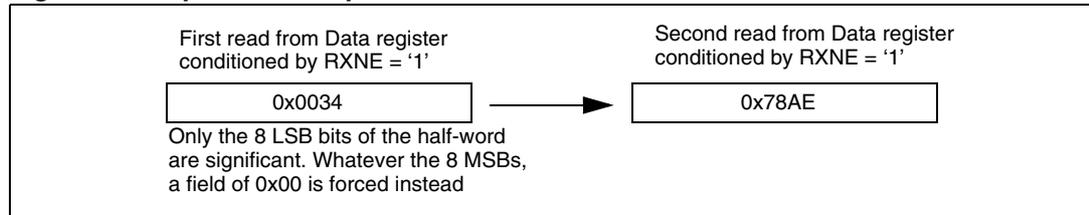
**Figure 261. LSB Justified 16-bit extended to 32-bit packet frame with CPOL = 0**
