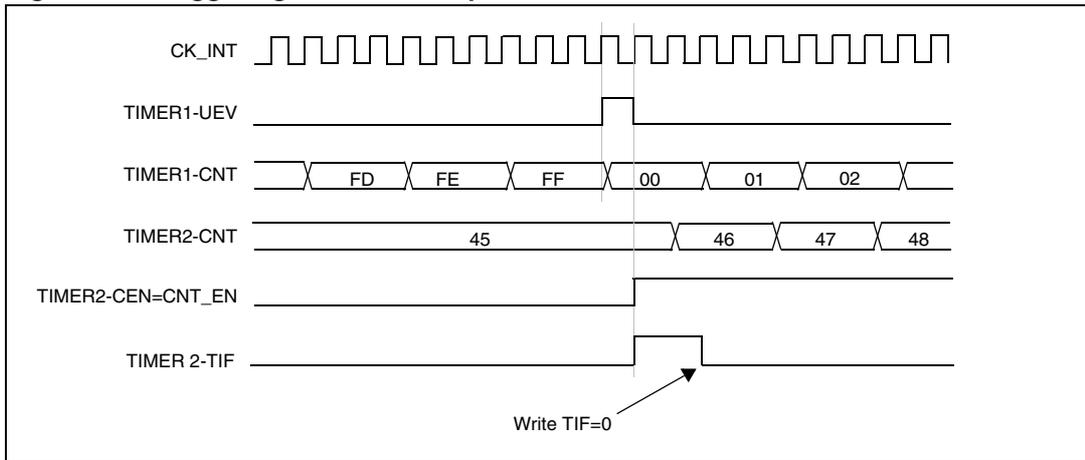
As in the previous example, you can initialize both counters before starting counting. [Figure 144](#) shows the behavior with the same configuration as in [Figure 143](#) but in trigger mode instead of gated mode (SMS=110 in the TIM2\_SMCR register).
