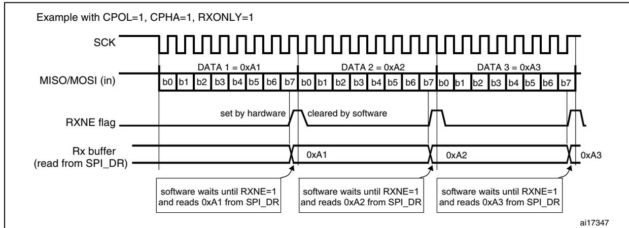
**Bidirectional receive procedure (BIDIMODE=1 and BIDIOE=0)**
