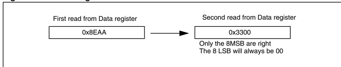
**Figure 252. I<sup>2</sup>S Phillips standard (16-bit extended to 32-bit packet frame with CPOL = 0)**
