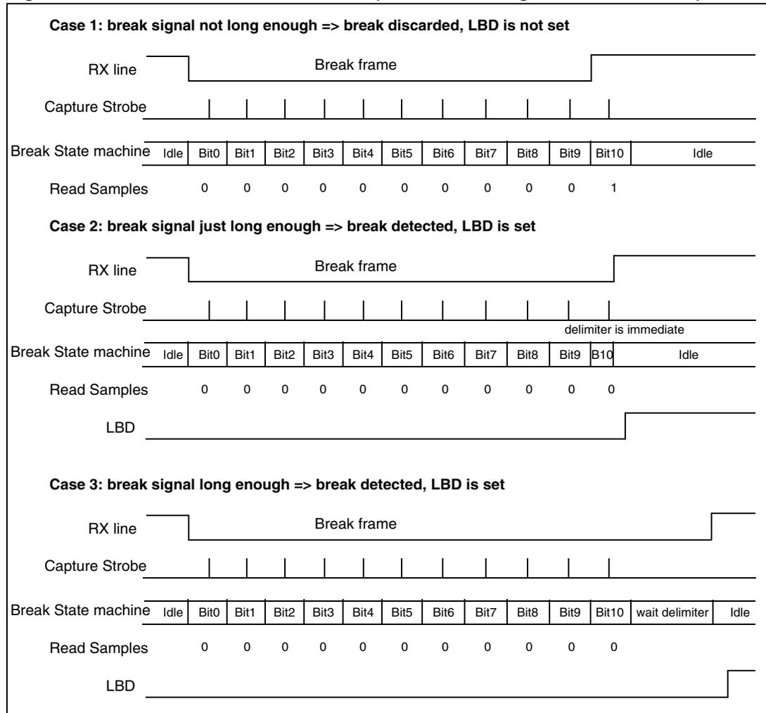
**Figure 286. Break detection in LIN mode vs. Framing error detection**
