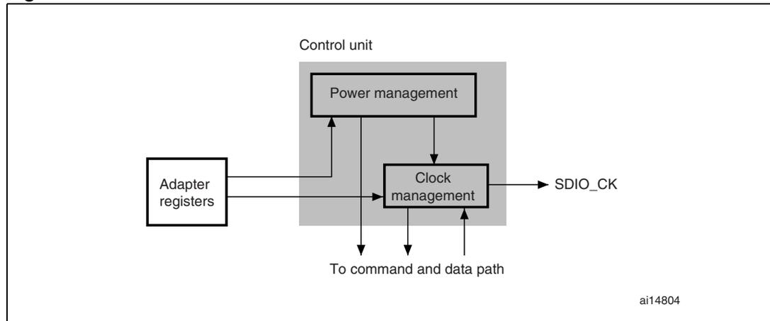
The control unit is illustrated in [Figure 213](#). It consists of a power management subunit and a clock management subunit.
