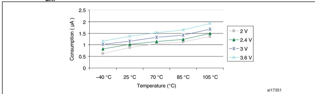
Figure 19. Typical current consumption in Stop mode with regulator in Run mode versus temperature at  $V_{DD} = 3.3\text{ V}$  and  $3.6\text{ V}$
