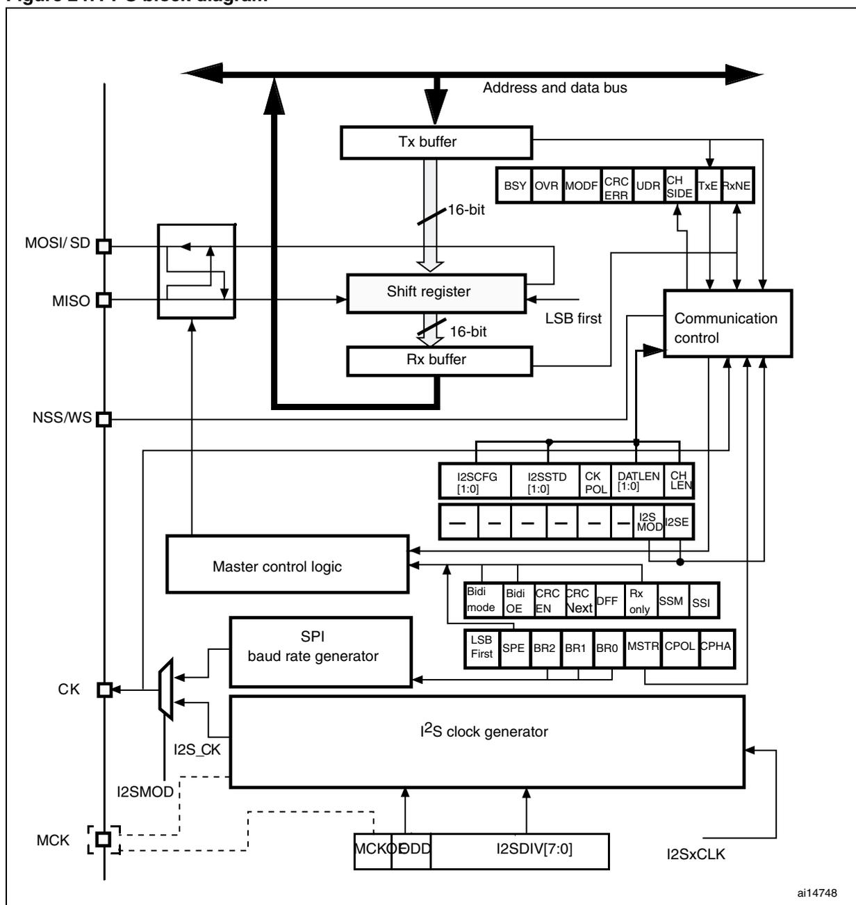
The SPI could function as an audio I<sup>2</sup>S interface when the I<sup>2</sup>S capability is enabled (by setting the I2SMOD bit in the SPI\_I2SCFGR register). This interface uses almost the same pins, flags and interrupts as the SPI.
