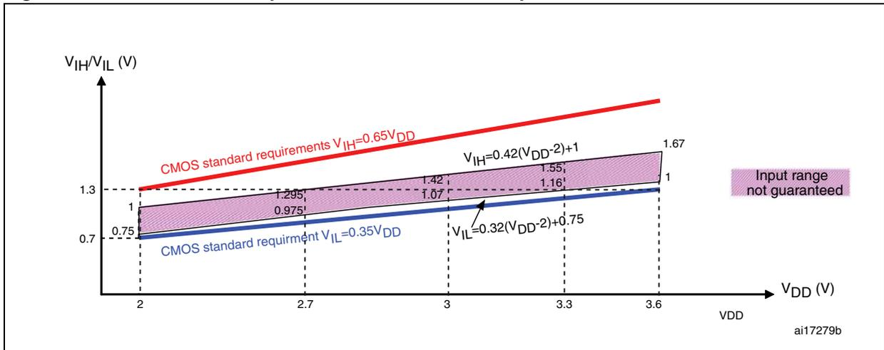
Figure 21. 5 V tolerant I/O input characteristics - TTL port
