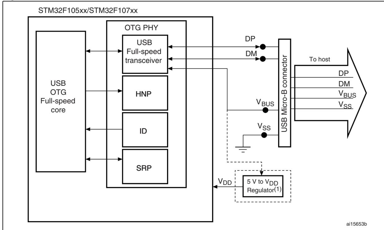
1. Use a regulator if you want to build a bus-powered device.
