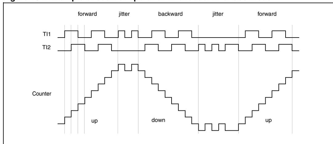
Figure 135 gives an example of counter behavior when TI1FP1 polarity is inverted (same configuration as above except CC1P=1).
