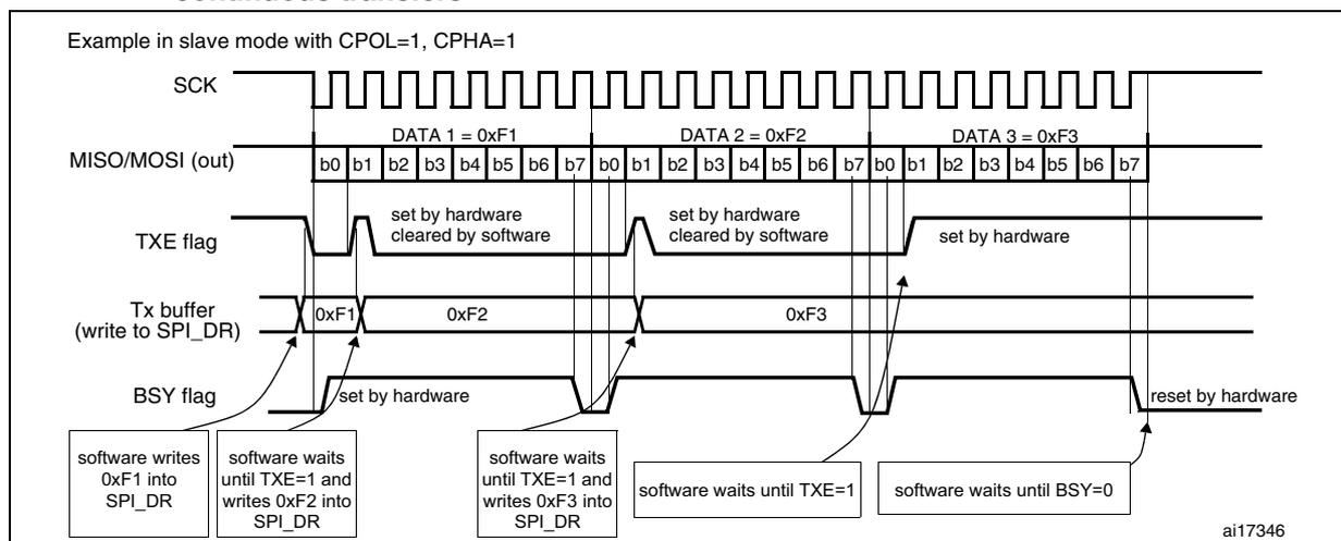
**Bidirectional transmit procedure (BIDIMODE=1 and BIDIOE=1)**
