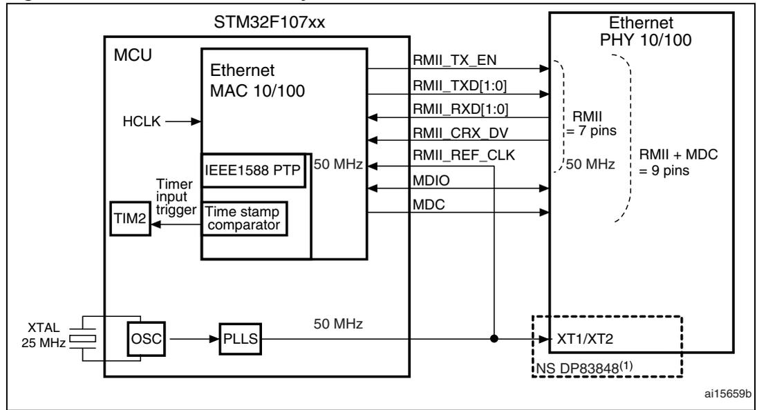
1. The NS DP83848 is recommended as the input jitter requirement of this PHY. It is compliant with the output jitter specification of the MCU.
