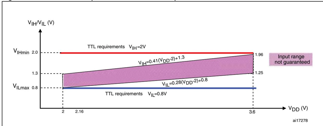
Figure 28. 5 V tolerant I/O input characteristics - CMOS port
