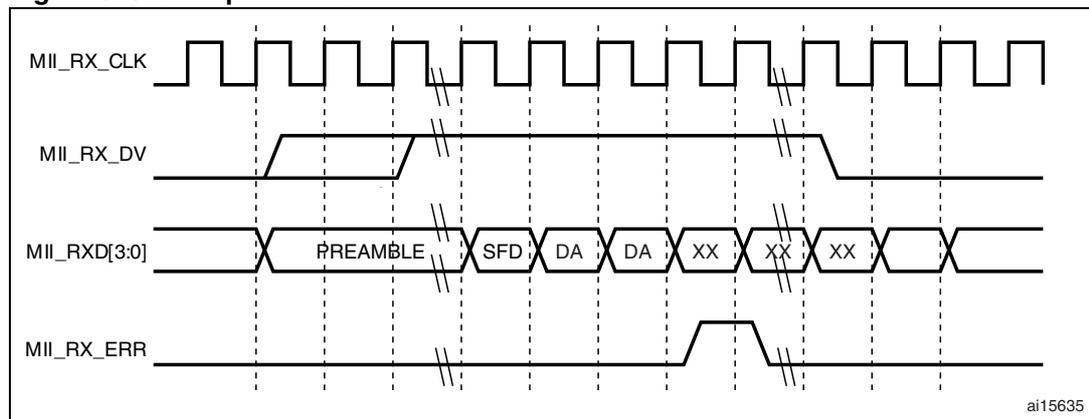
Figure 344. Reception with false carrier indication
