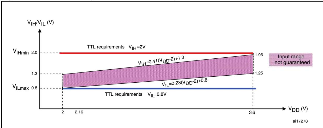
Figure 20. 5 V tolerant I/O input characteristics - CMOS port
