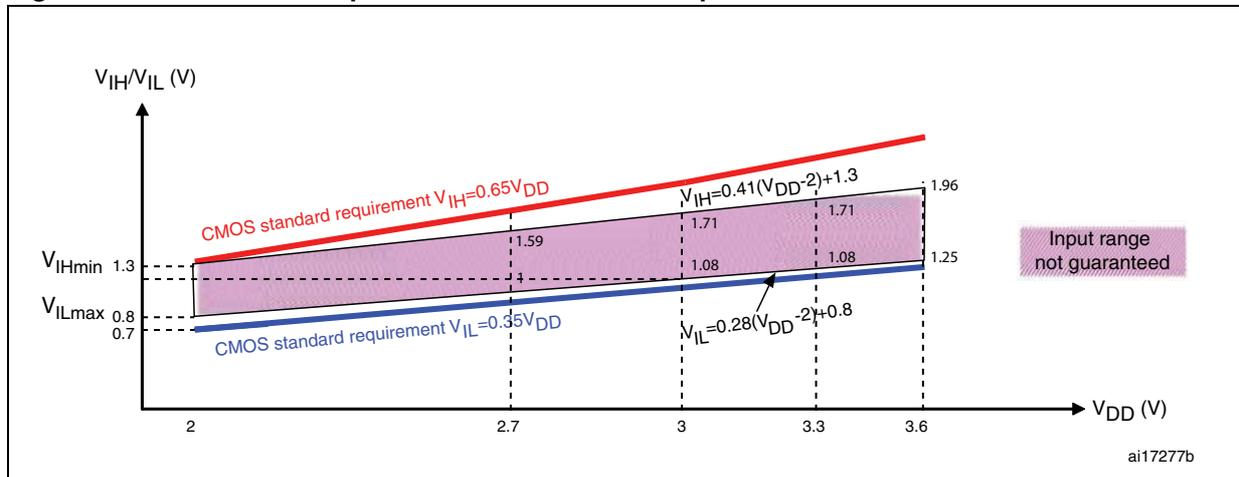
**Figure 27. Standard I/O input characteristics - TTL port**
