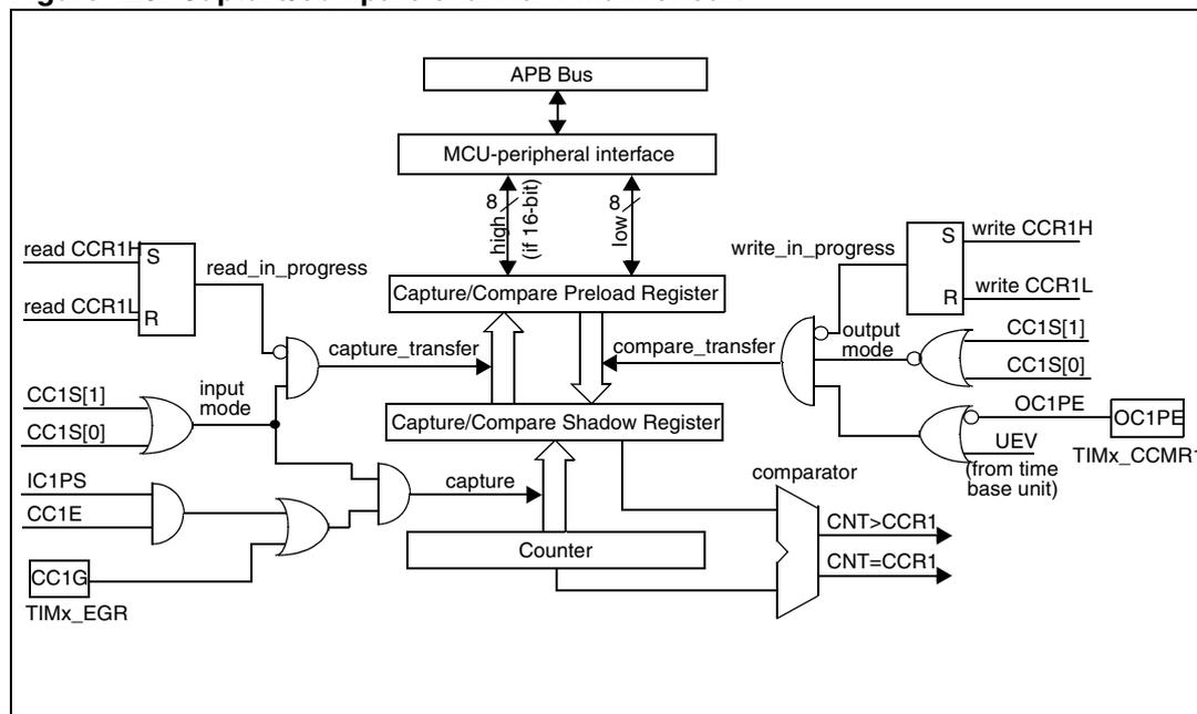
Figure 127. Output stage of capture/compare channel (channel 1)
