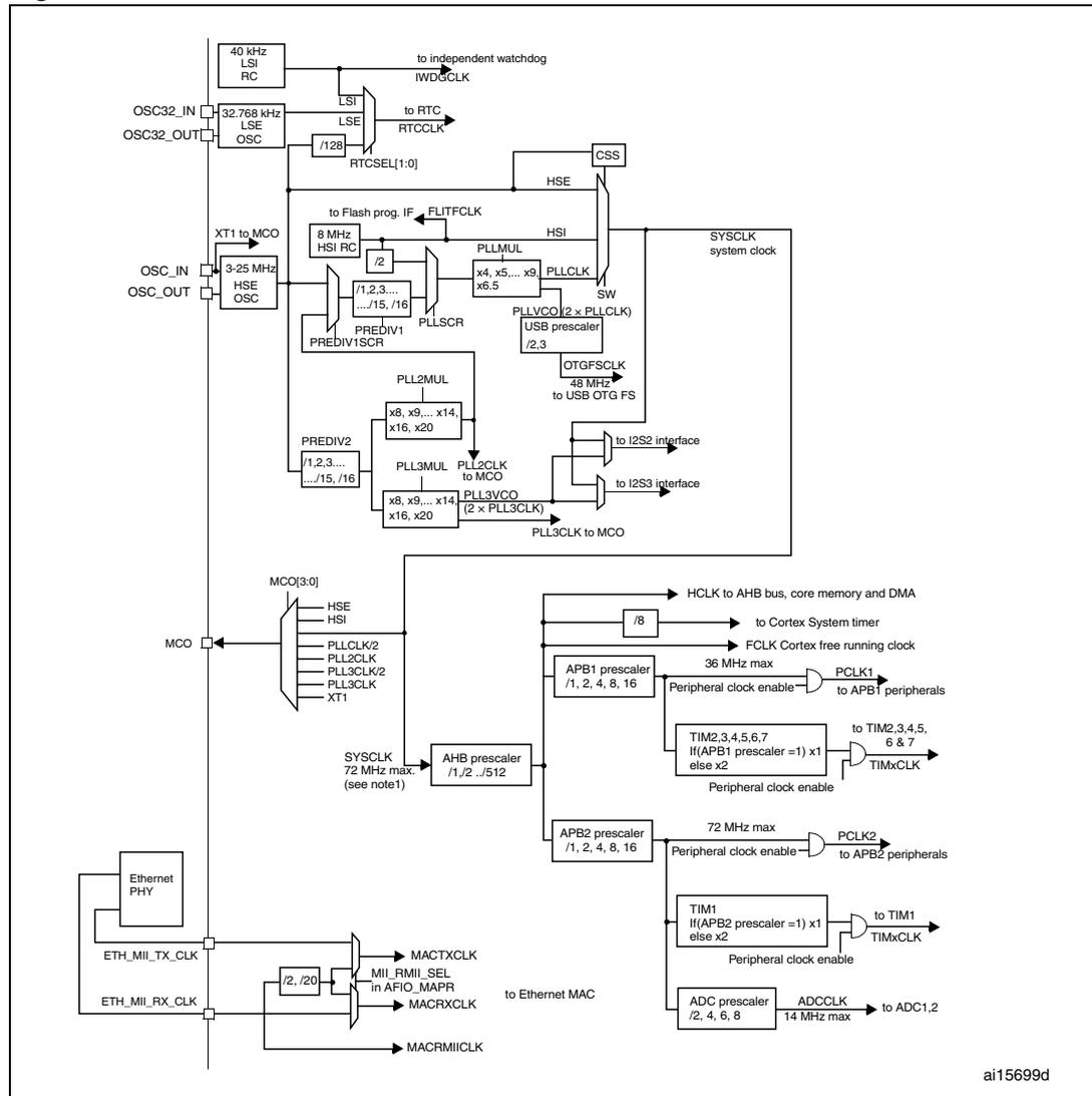
1. When the HSI is used as a PLL clock input, the maximum system clock frequency that can be achieved is 36 MHz.
