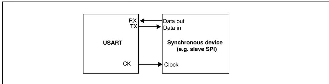
Figure 288. USART data clock timing diagram (M=0)
