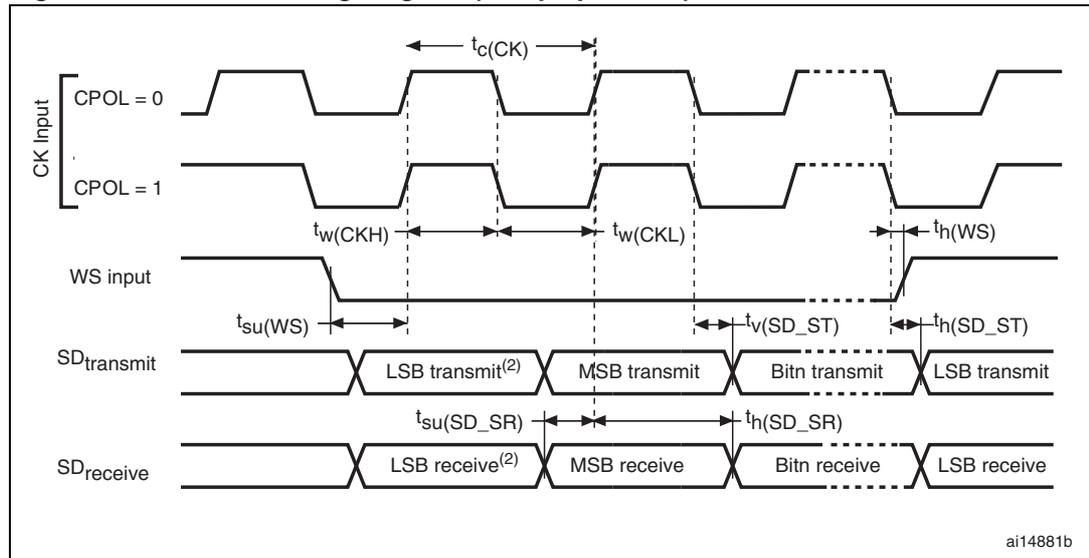
1. Measurement points are done at CMOS levels:  $0.3 \times V_{DD}$  and  $0.7 \times V_{DD}$ .
