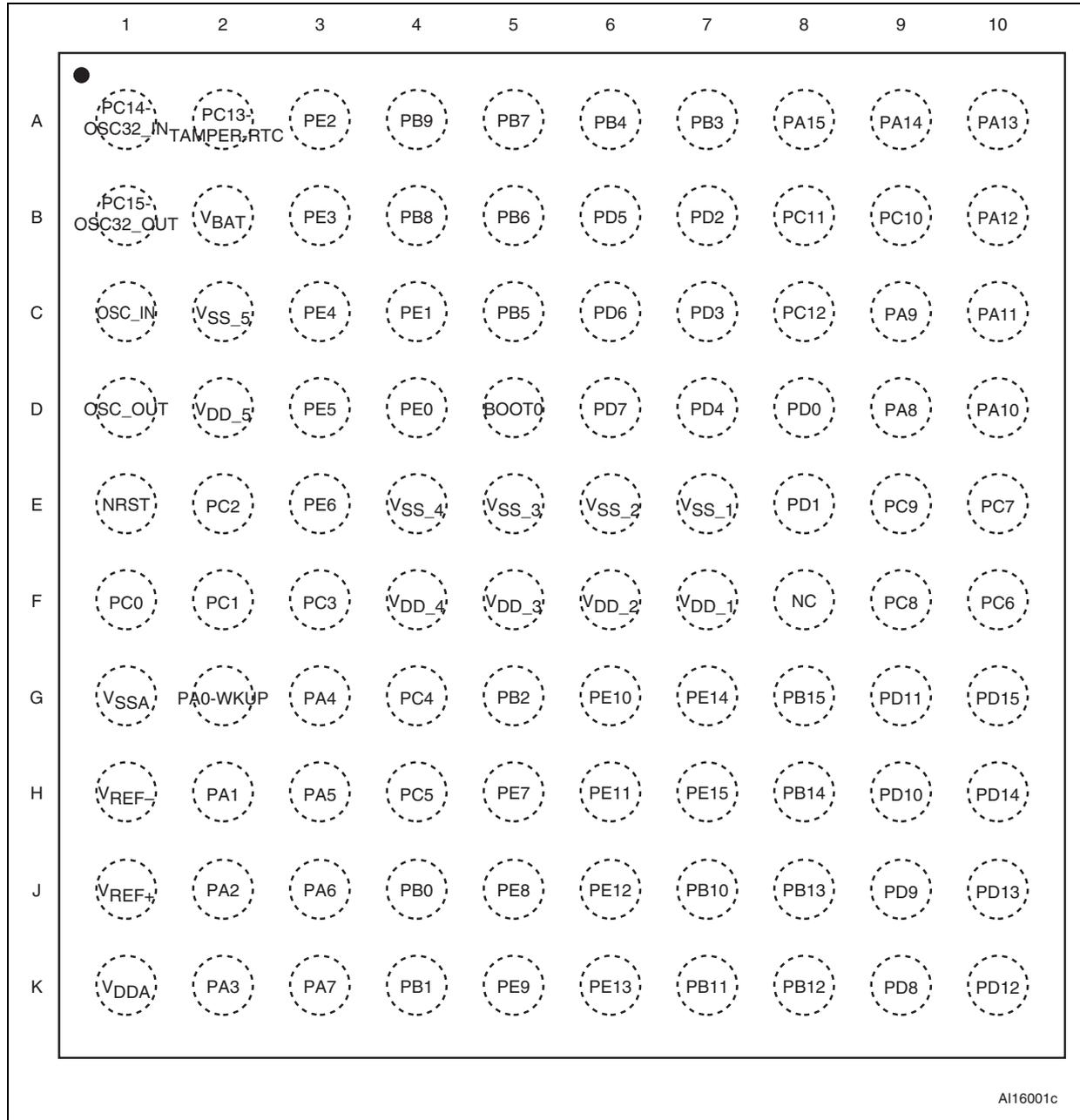
Figure 4. STM32F103xx performance line LQFP100 pinout
