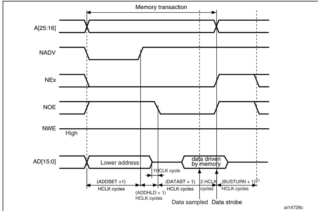
1. The bus turnaround delay (BUSTURN + 1) and the delay between side-by-side transactions overlap, so BUSTURN ≤ 5 has not impact.
