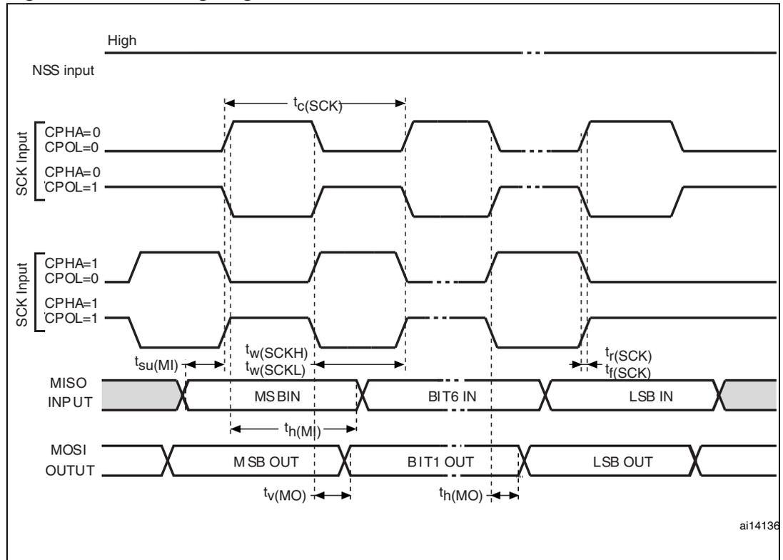
1. Measurement points are done at CMOS levels:  $0.3V_{DD}$  and  $0.7V_{DD}$ .
