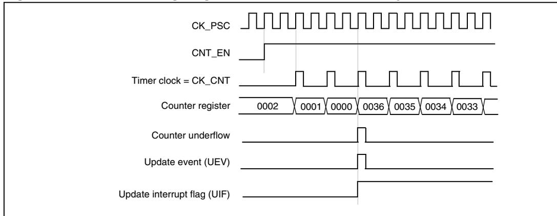
**Figure 63. Counter timing diagram, internal clock divided by 4**
