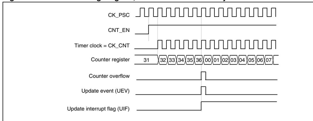
**Figure 151. Counter timing diagram, internal clock divided by 2**
