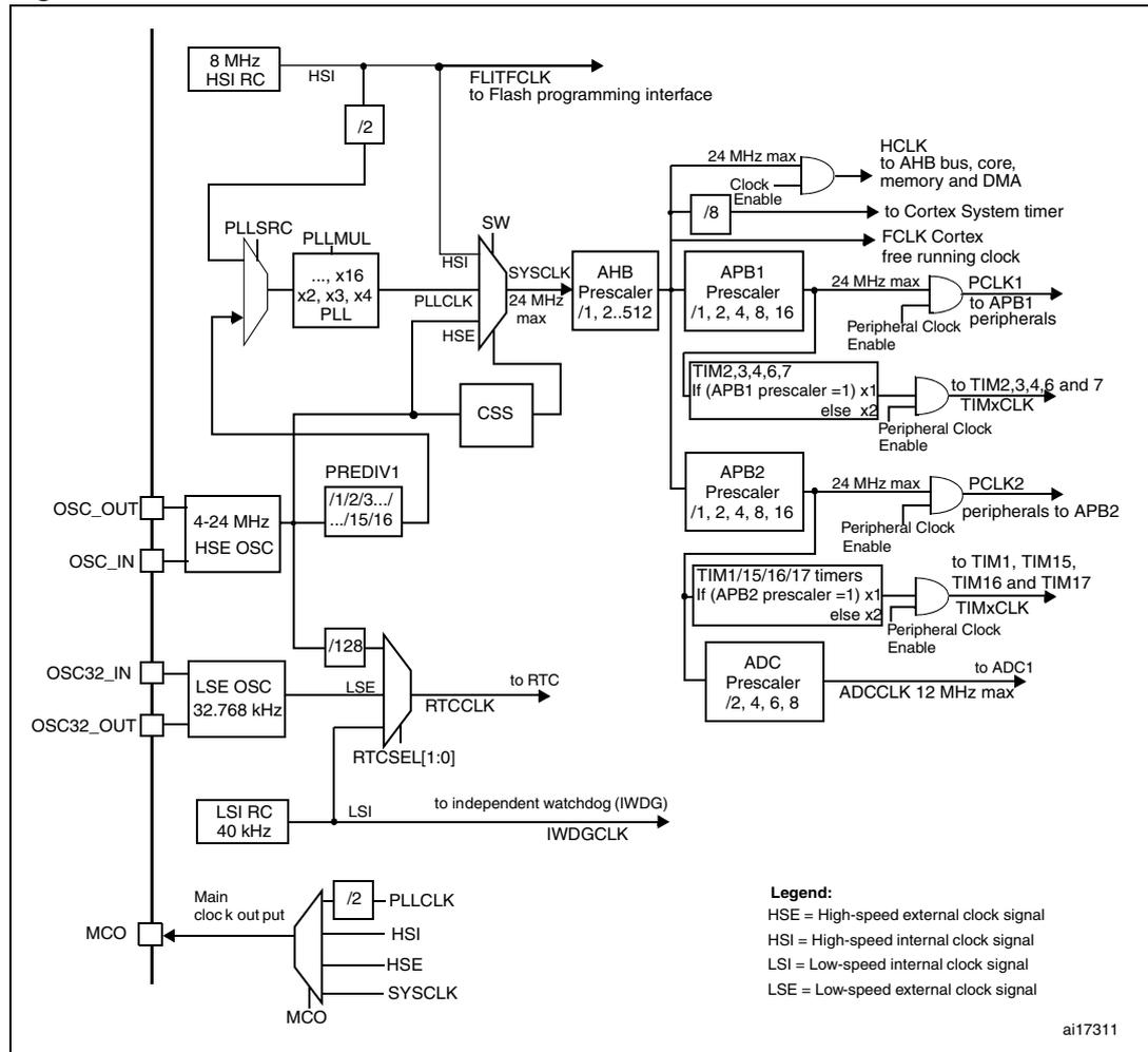
4. To have an ADC conversion time of 1.2  $\mu$ s, APB2 must be at 24 MHz.
