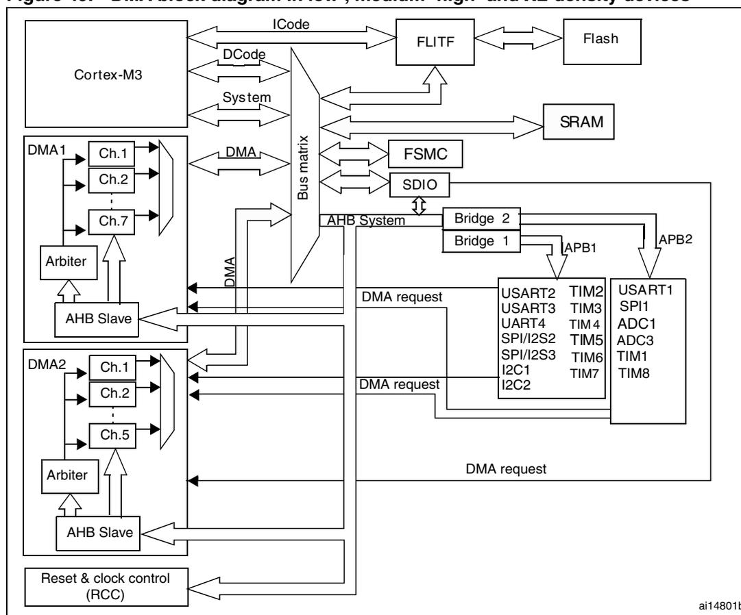
1. The DMA2 controller is available only in high-density and XL-density devices.
