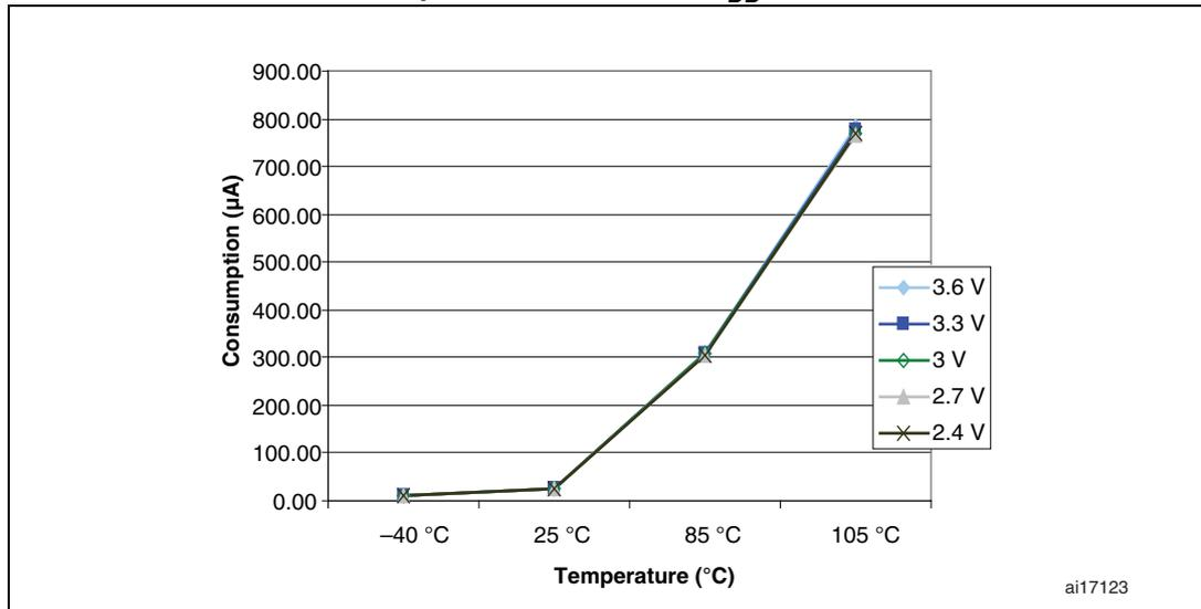
**Figure 13. Typical current consumption in Standby mode versus temperature at different V<sub>DD</sub> values**
