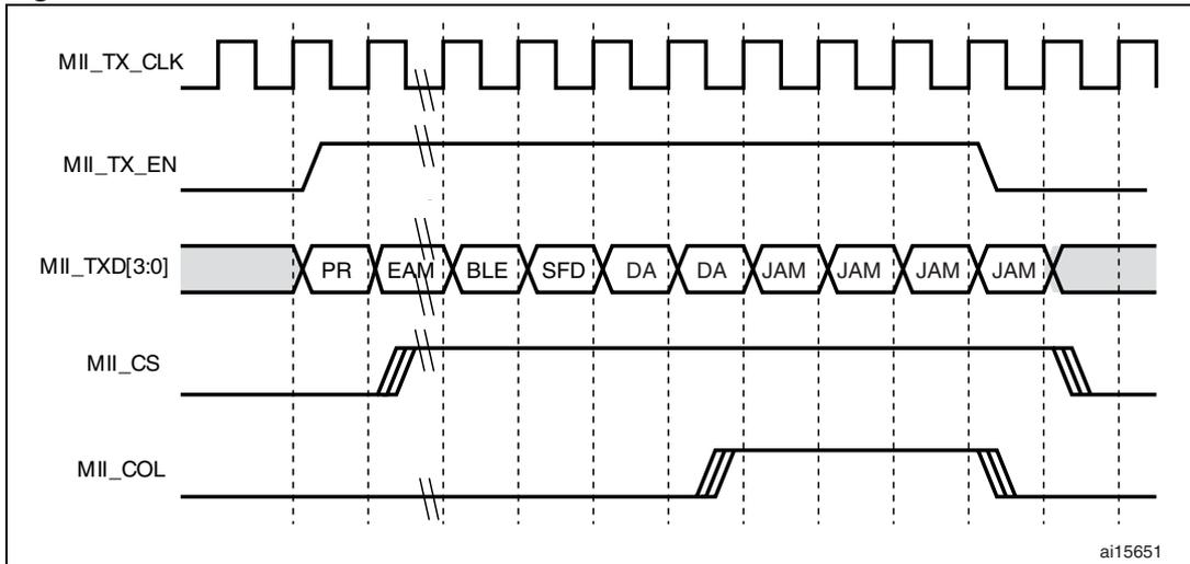
Figure 340 shows a frame transmission in MII and RMII.
