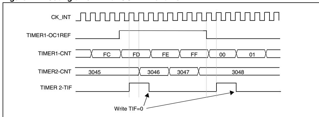
In the example in [Figure 141](#), the Timer 2 counter and prescaler are not initialized before being started. So they start counting from their current value. It is possible to start from a given value by resetting both timers before starting Timer 1. You can then write any value you want in the timer counters. The timers can easily be reset by software using the UG bit in the TIMx\_EGR registers.
