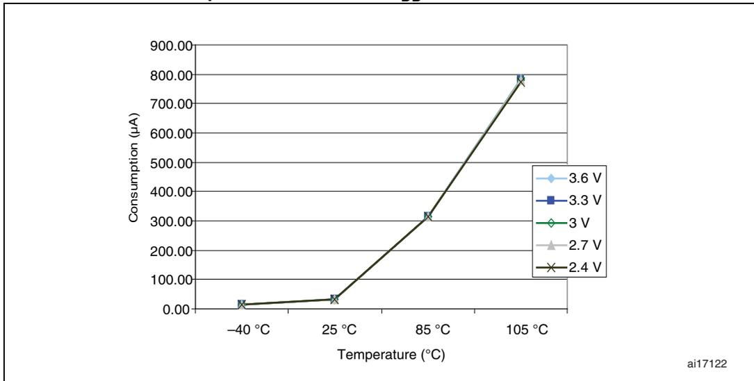
**Figure 12. Typical current consumption in Stop mode with regulator in Low-power mode versus temperature at different V<sub>DD</sub> values**
