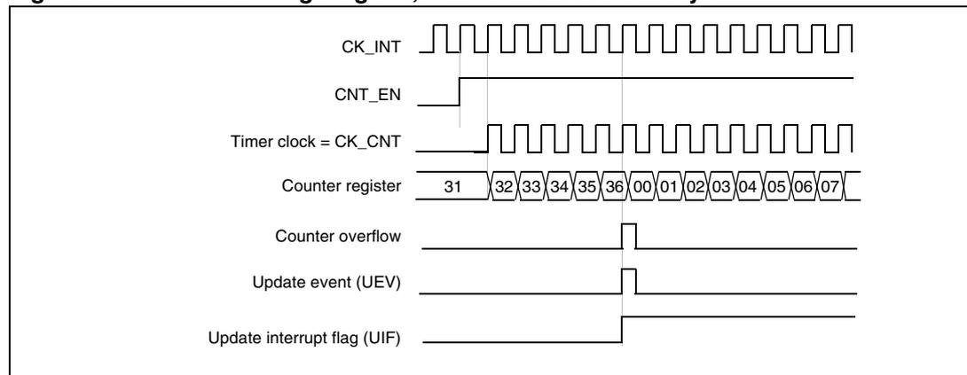
**Figure 173. Counter timing diagram, internal clock divided by 2**
