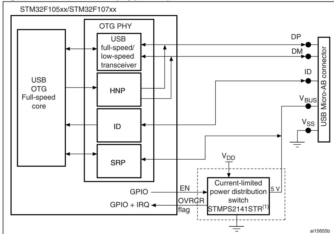
1. STMPS2141STR needed only if the application has to support bus-powered devices.
