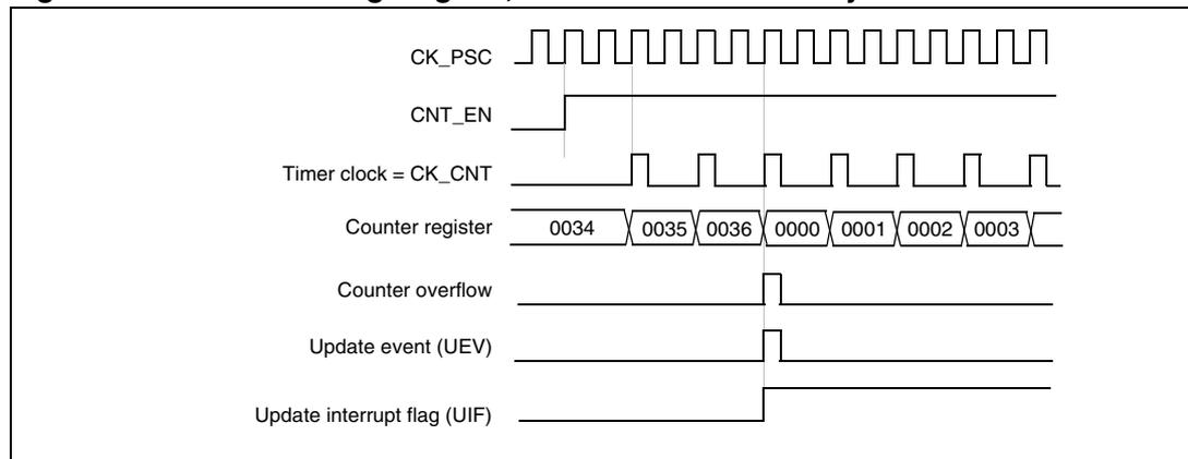
**Figure 152. Counter timing diagram, internal clock divided by 4**
