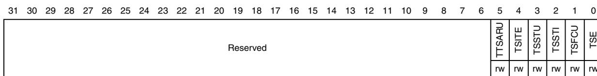
**Ethernet PTP subsecond increment register (ETH\_PTPSSIR)**
