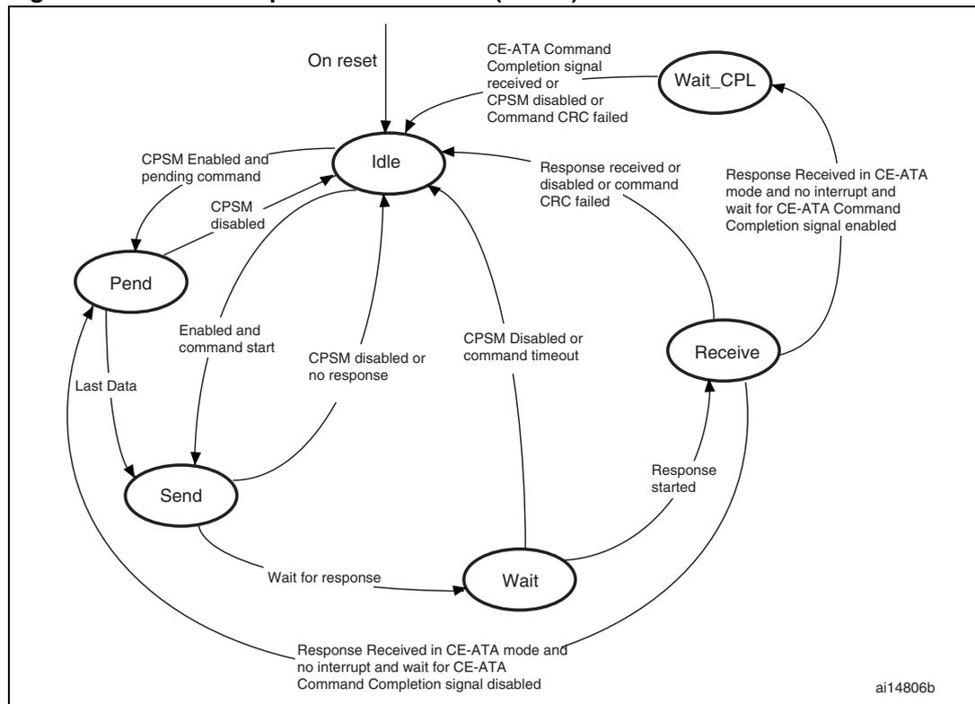
When the Wait state is entered, the command timer starts running. If the timeout is reached before the CPSM moves to the Receive state, the timeout flag is set and the Idle state is entered.
