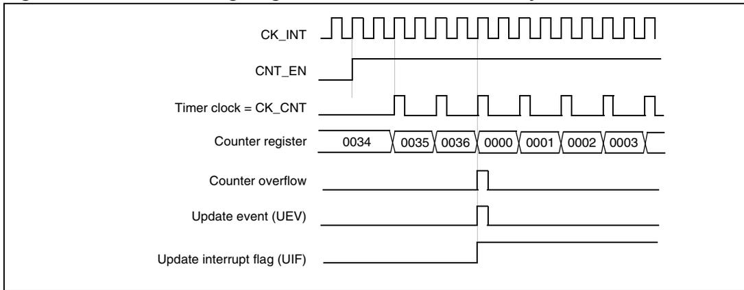
**Figure 174. Counter timing diagram, internal clock divided by 4**
