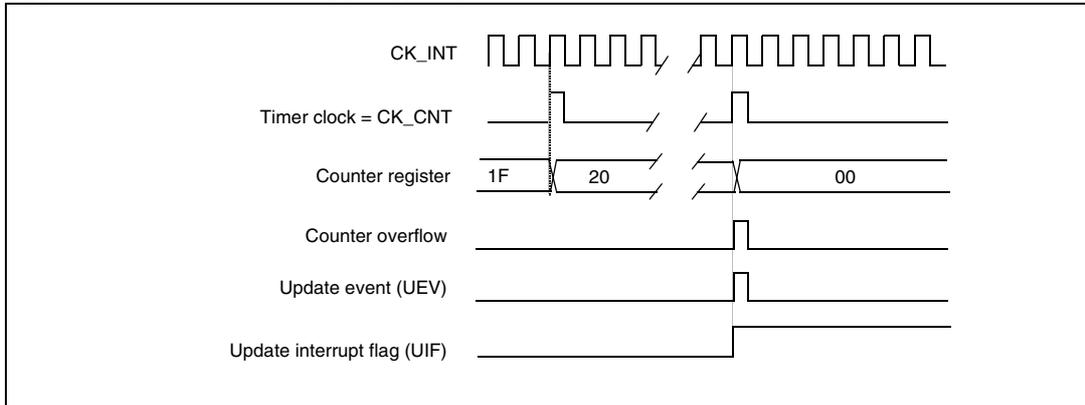
**Figure 176. Counter timing diagram, update event when ARPE = 0 (TIMx\_ARR not preloaded)**
