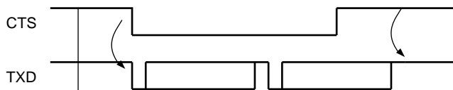
Figure 36-28. Transmitter Behavior when Operating with Hardware Handshaking
