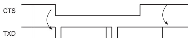
Figure 43-27. Transmitter Behavior when Operating with Hardware Handshaking
