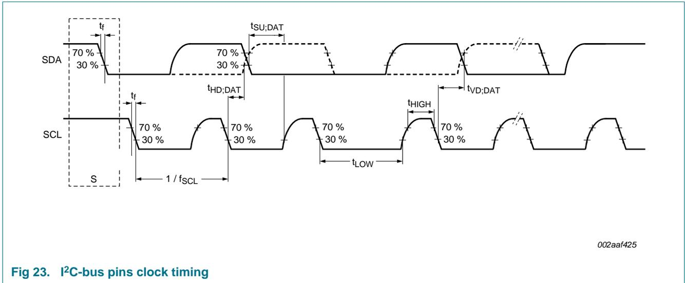
Fig 23. I<sup>2</sup>C-bus pins clock timing
