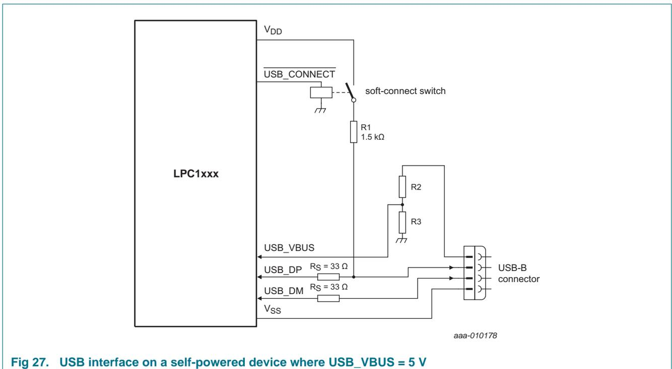
Fig 27. USB interface on a self-powered device where USB\_VBUS = 5 V
