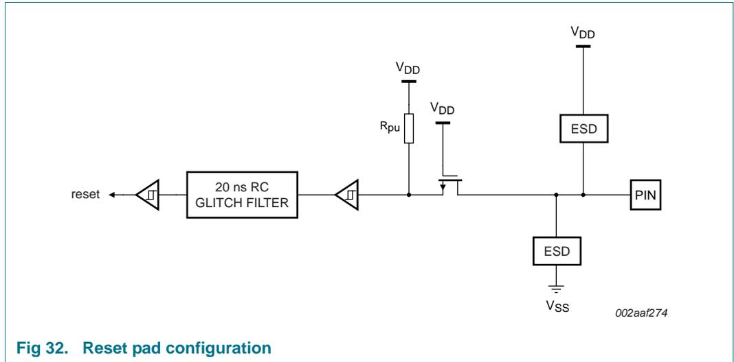
Fig 32. Reset pad configuration
