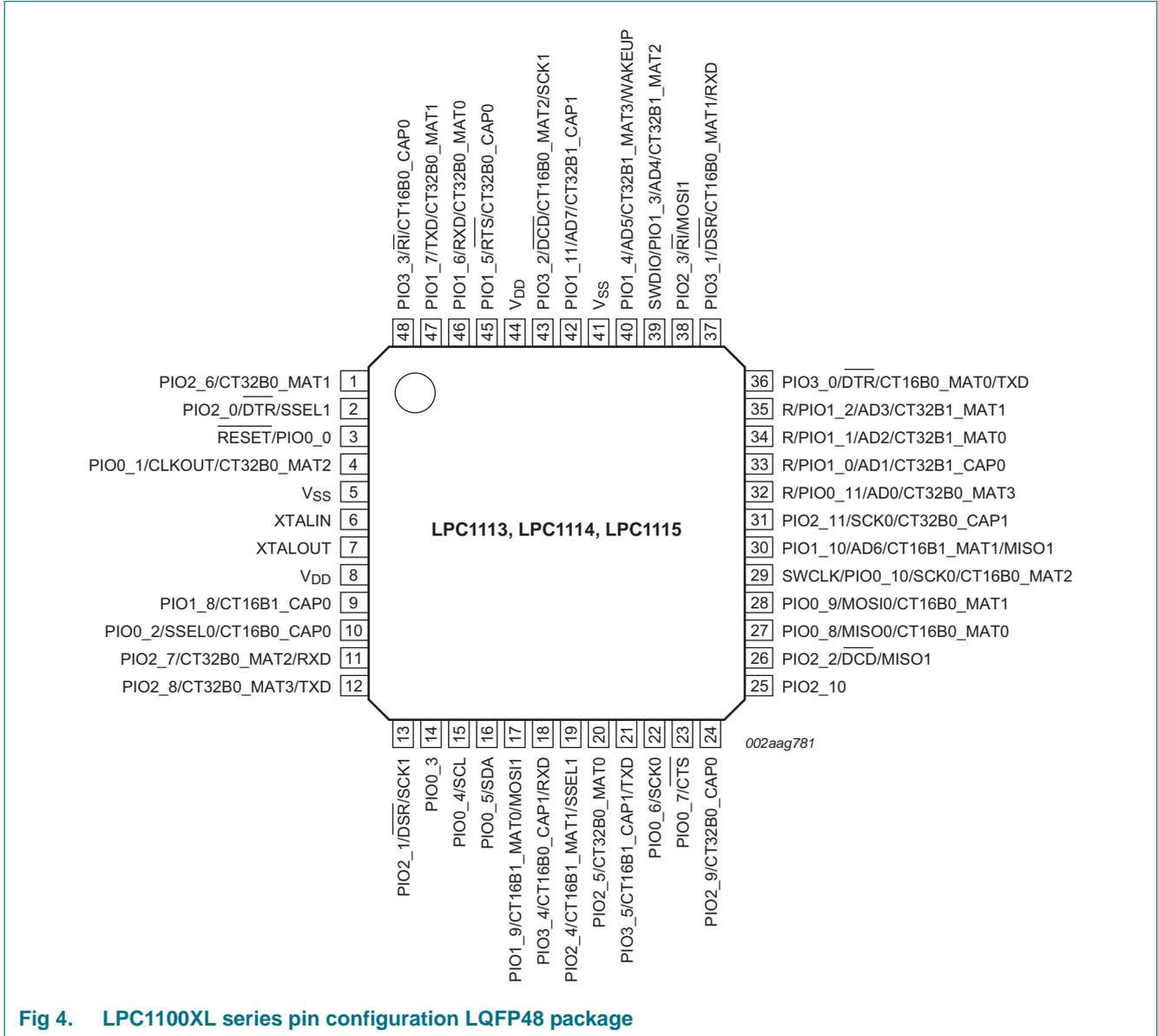
Fig 4. LPC1100XL series pin configuration LQFP48 package
