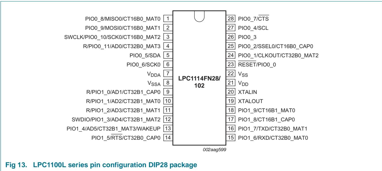
**Fig 13. LPC1100L series pin configuration DIP28 package**
