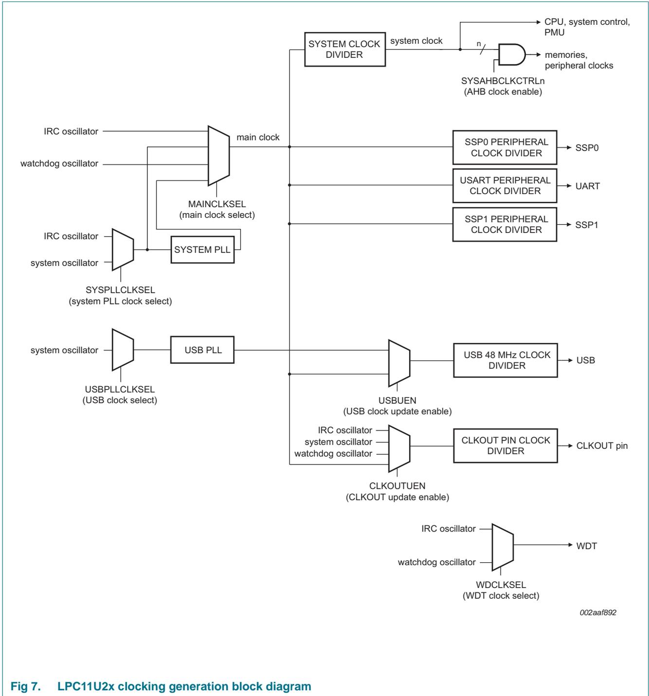
Fig 7. LPC11U2x clocking generation block diagram
