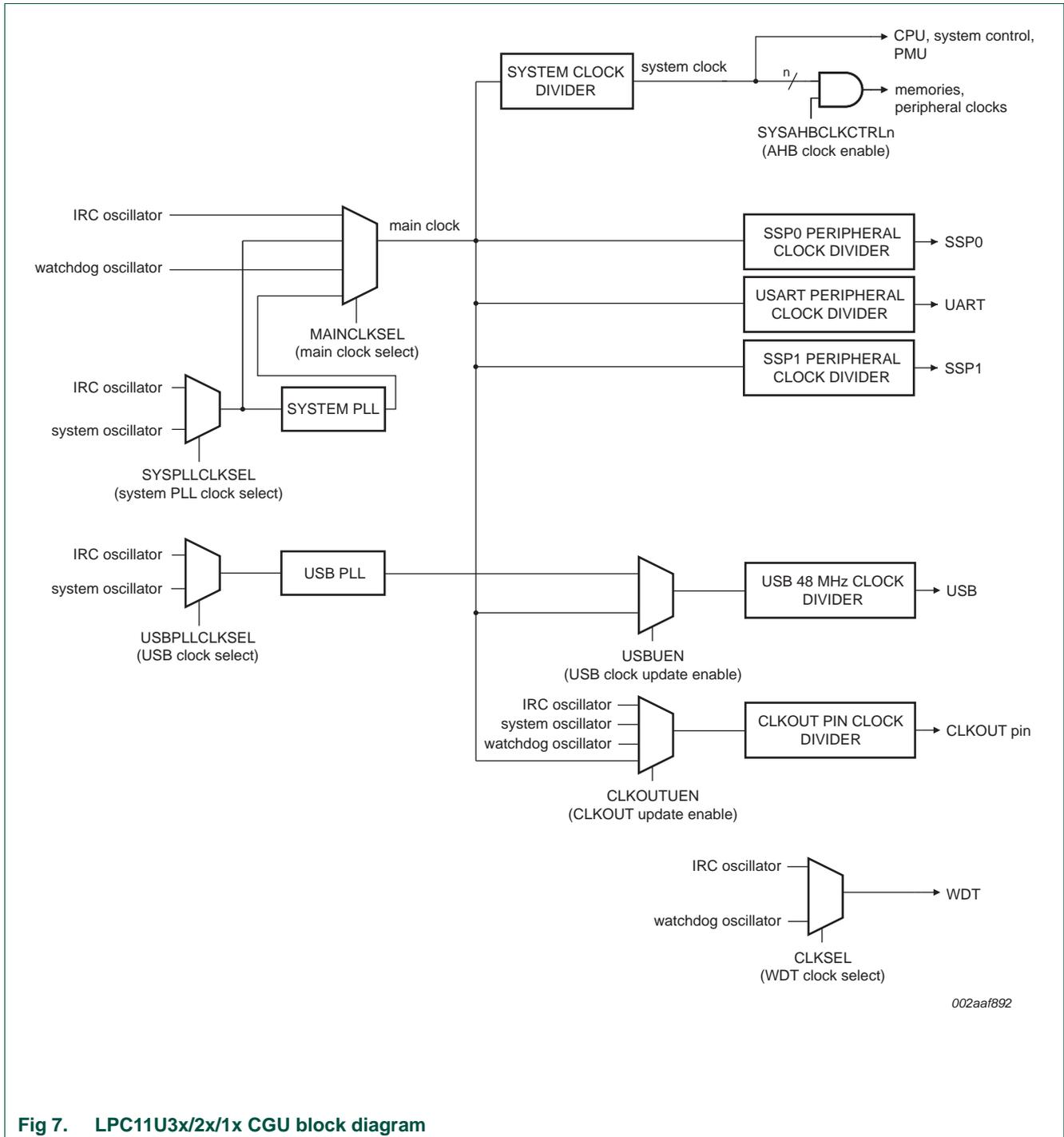
Fig 7. LPC11U3x/2x/1x CGU block diagram
