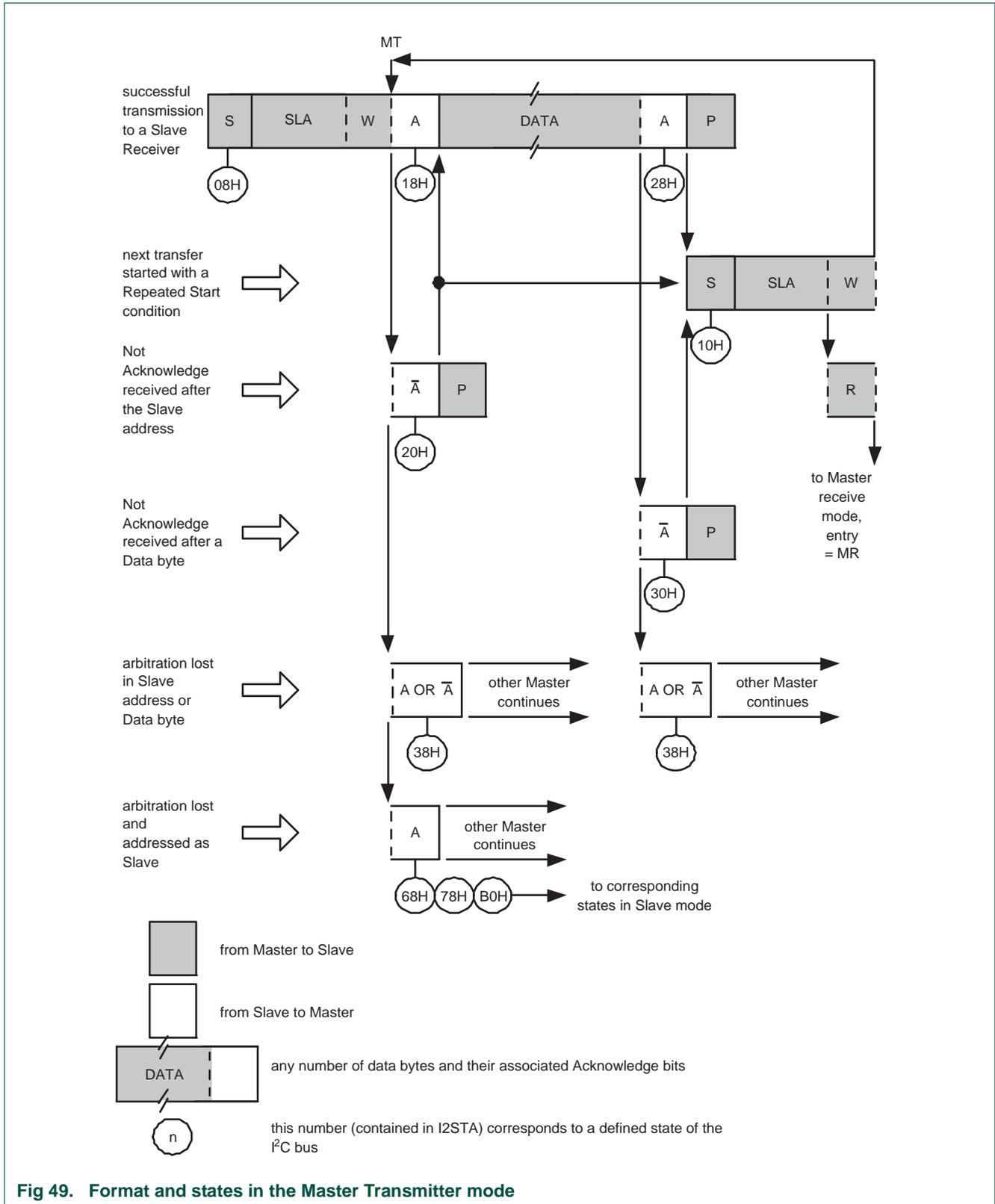
Fig 49. Format and states in the Master Transmitter mode
