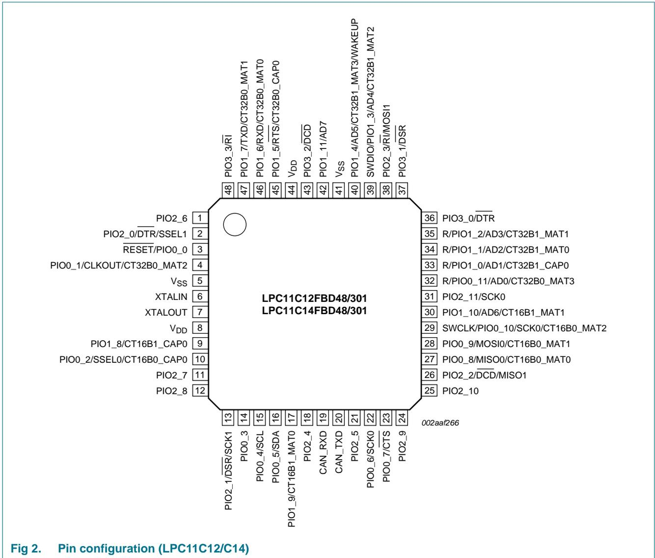
Fig 2. Pin configuration (LPC11C12/C14)
