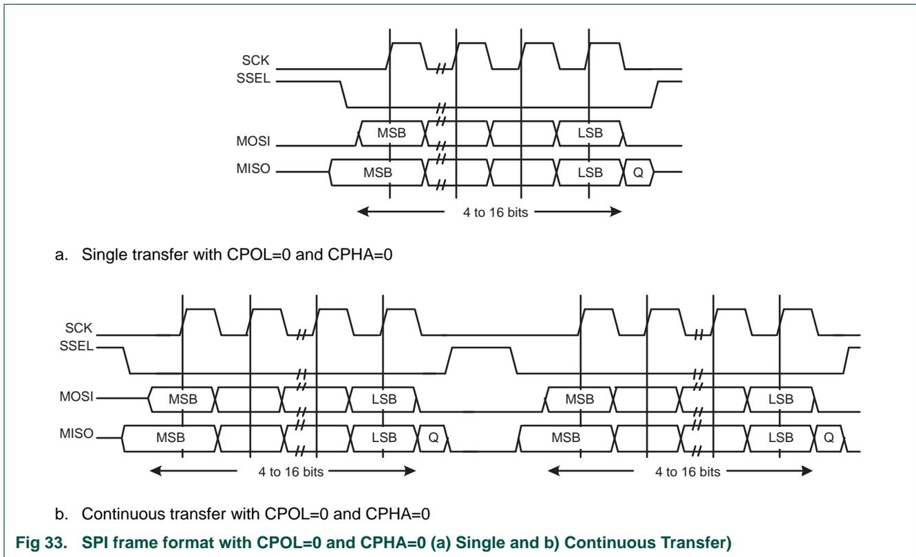
**Fig 33. SPI frame format with CPOL=0 and CPHA=0 (a) Single and b) Continuous Transfer)**
