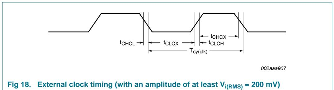
**Fig 18. External clock timing (with an amplitude of at least  $V_{i(RMS)} = 200\text{ mV}$ )**
