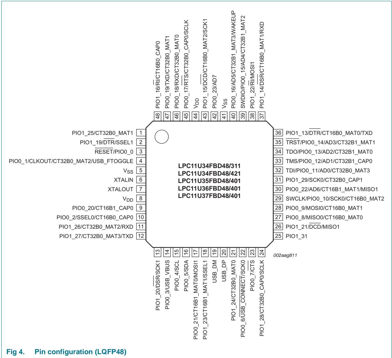
Fig 4. Pin configuration (LQFP48)
