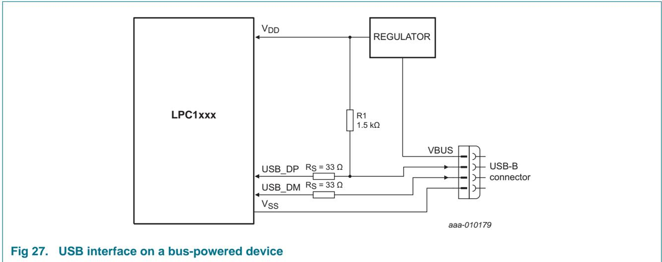
Fig 27. USB interface on a bus-powered device
