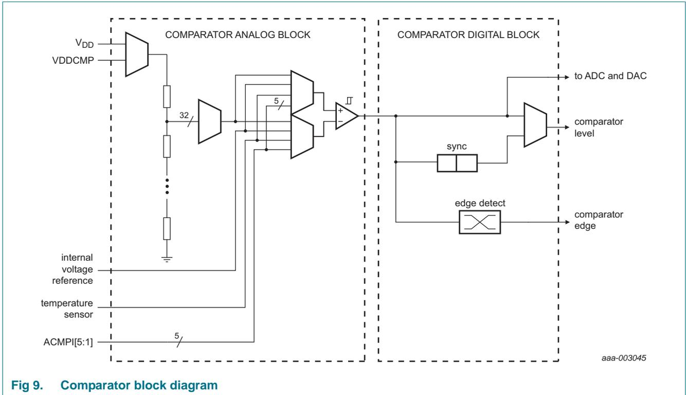
Fig 9. Comparator block diagram
