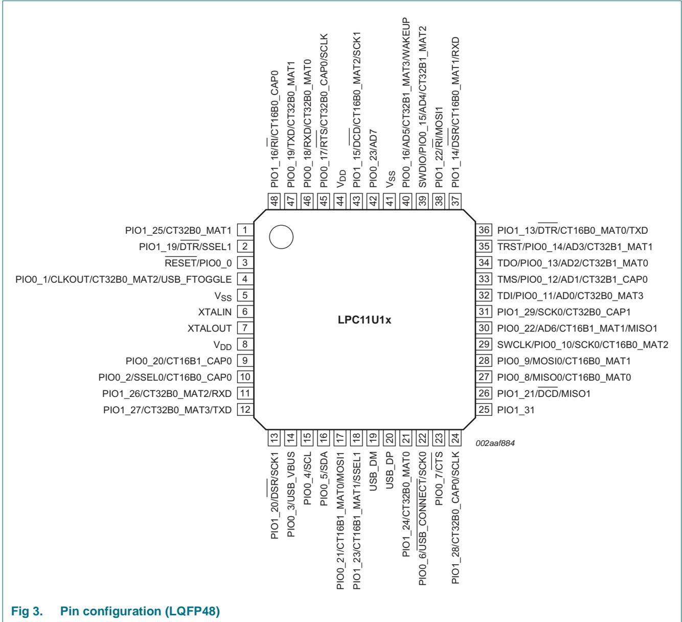
Fig 3. Pin configuration (LQFP48)
