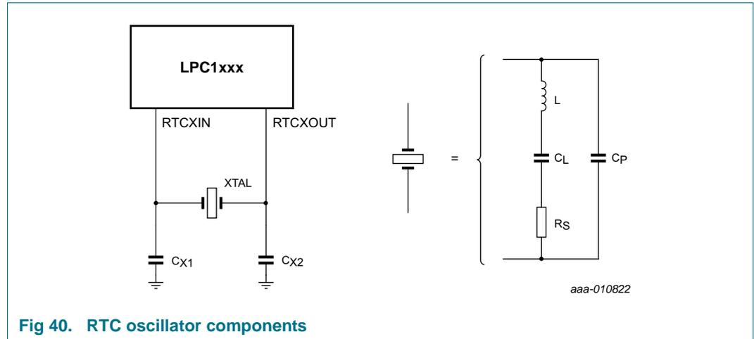
Fig 40. RTC oscillator components
