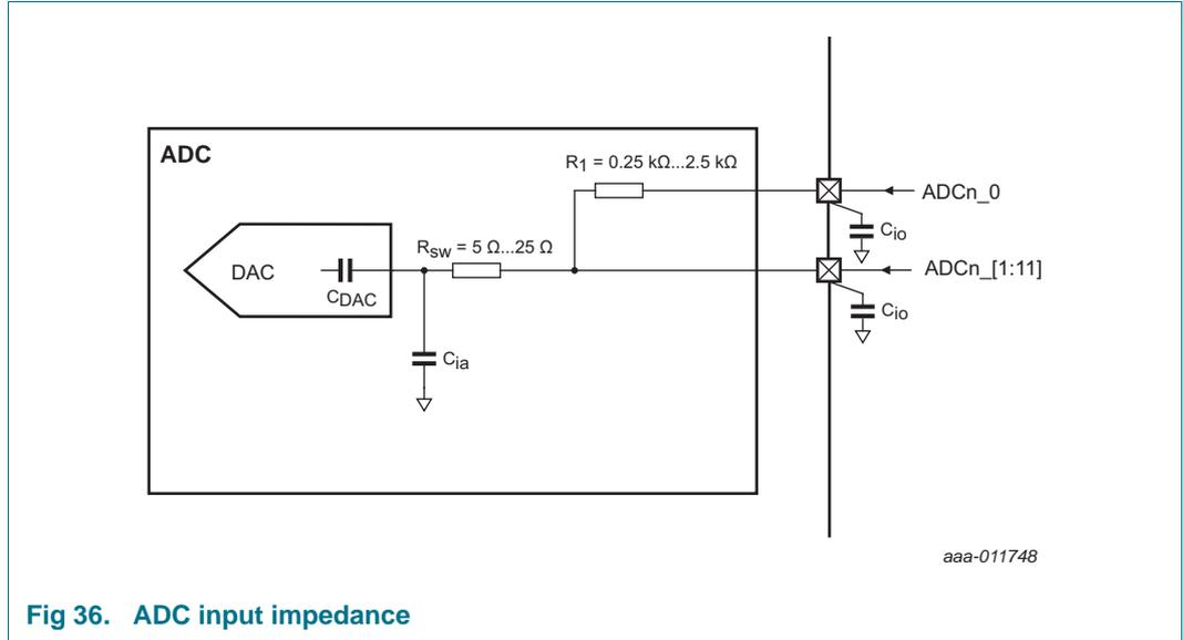
Fig 36. ADC input impedance
