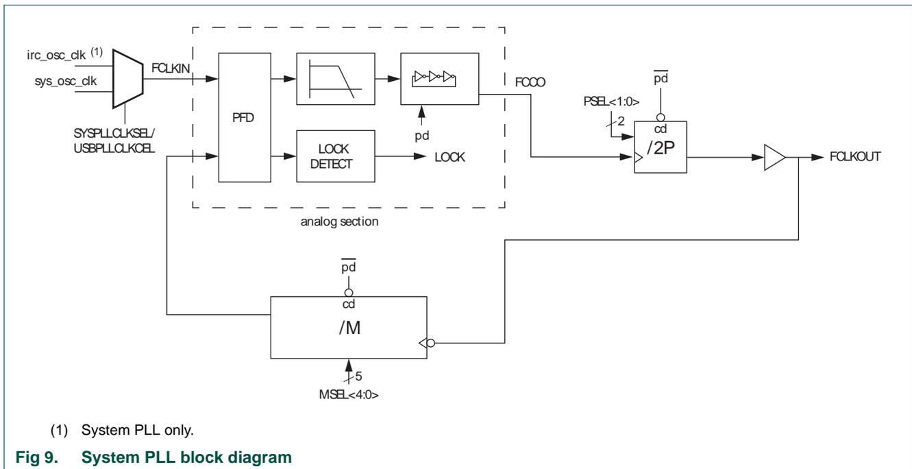
The block diagram of this PLL is shown in Figure 9. The input frequency range is 10 MHz to 25 MHz. The input clock is fed directly to the Phase-Frequency Detector (PFD). This block compares the phase and frequency of its inputs, and generates a control signal when phase and/ or frequency do not match. The loop filter filters these control signals and drives the current controlled oscillator (CCO), which generates the main clock and
