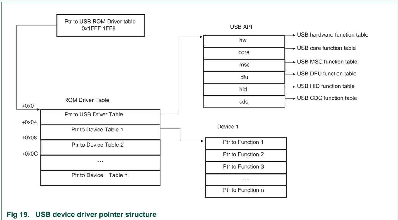
Fig 19. USB device driver pointer structure
