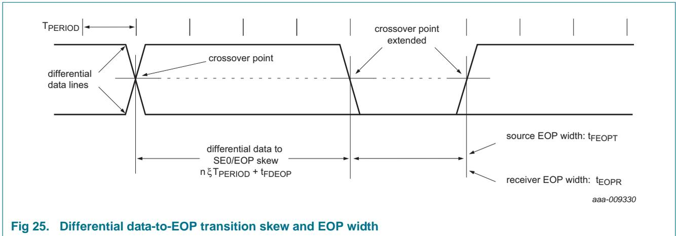
Fig 25. Differential data-to-EOP transition skew and EOP width
