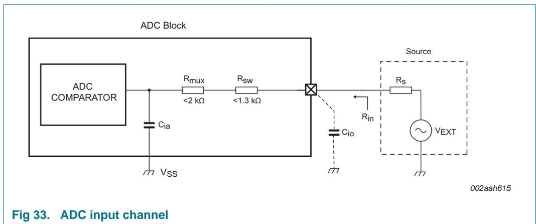
Fig 33. ADC input channel
