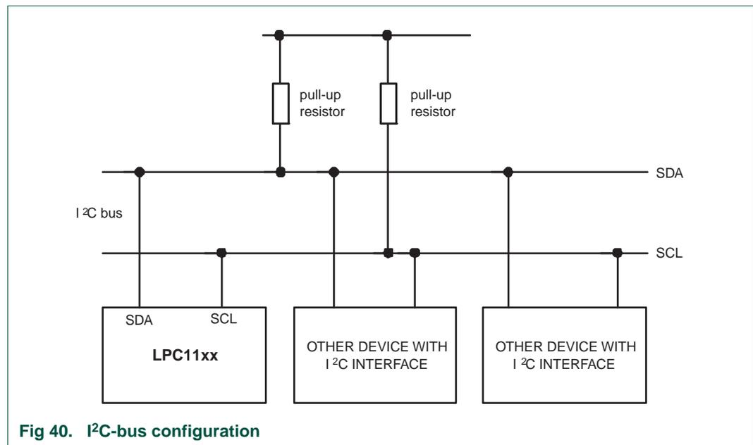
Fig 40. I<sup>2</sup>C-bus configuration
