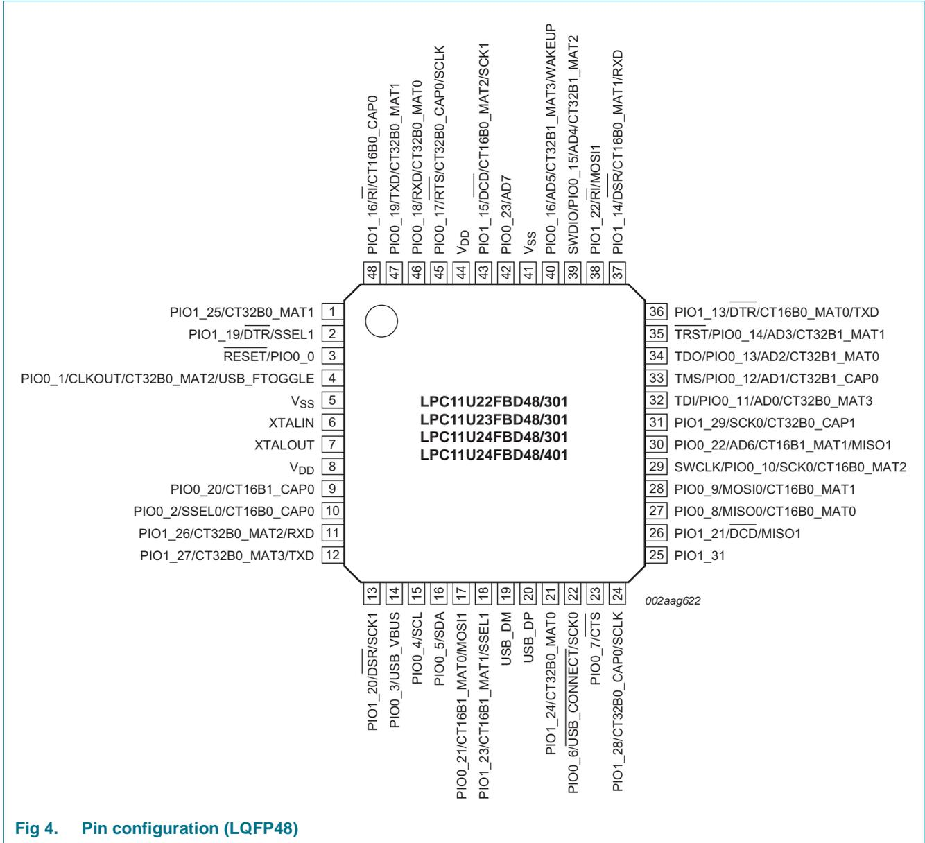
Fig 4. Pin configuration (LQFP48)
