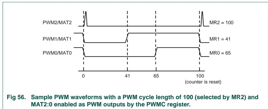
**Fig 56. Sample PWM waveforms with a PWM cycle length of 100 (selected by MR2) and MAT2:0 enabled as PWM outputs by the PWMC register.**
