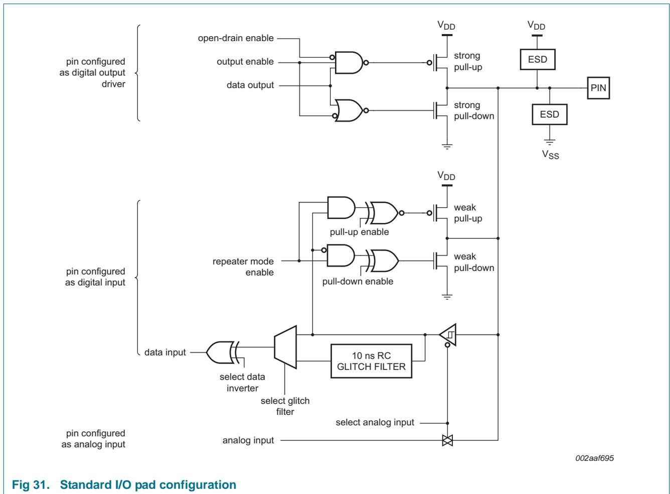
Fig 31. Standard I/O pad configuration
