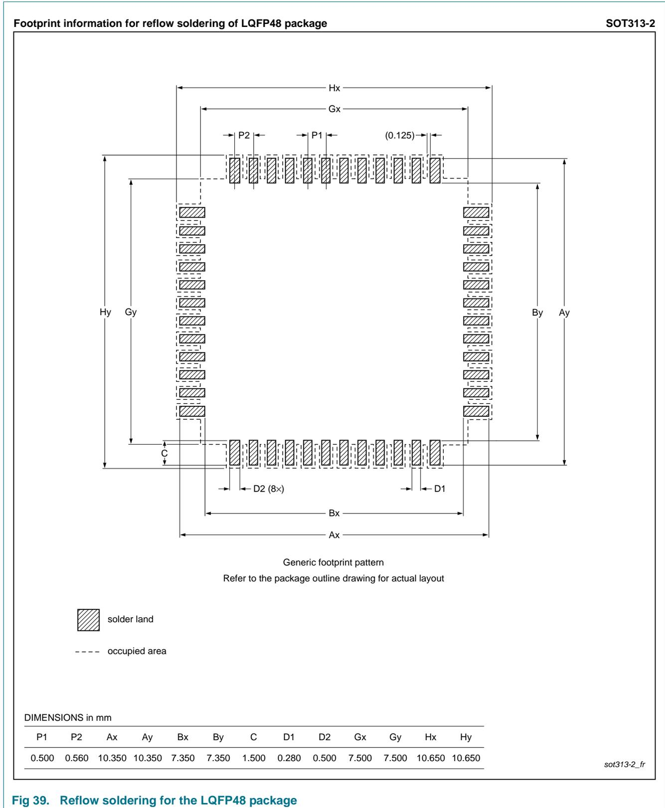
**Fig 39. Reflow soldering for the LQFP48 package**
