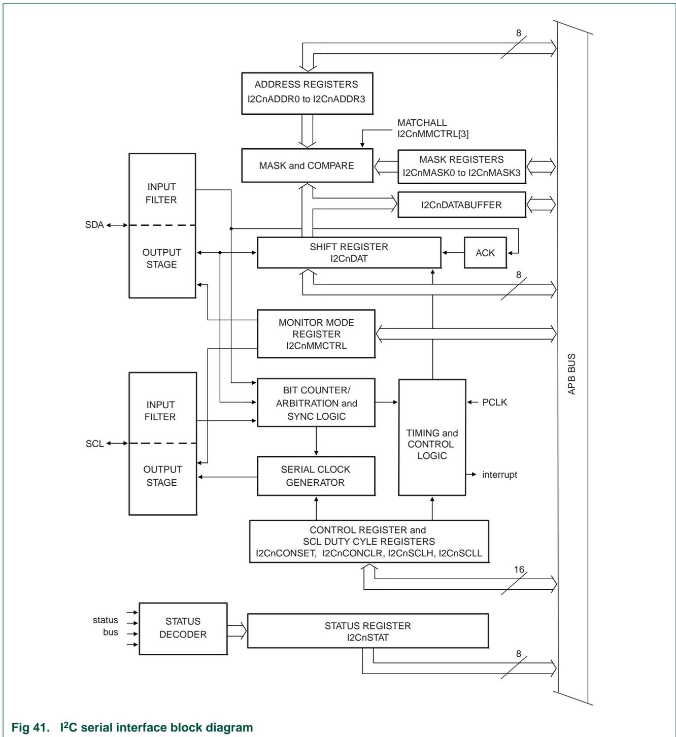
Fig 41. I2C serial interface block diagram
