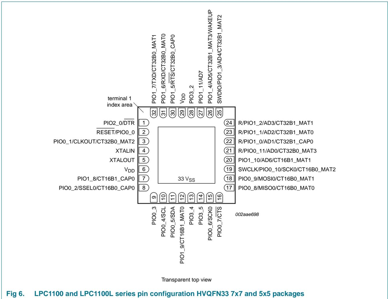
**Fig 6. LPC1100 and LPC1100L series pin configuration HVQFN33 7x7 and 5x5 packages**
