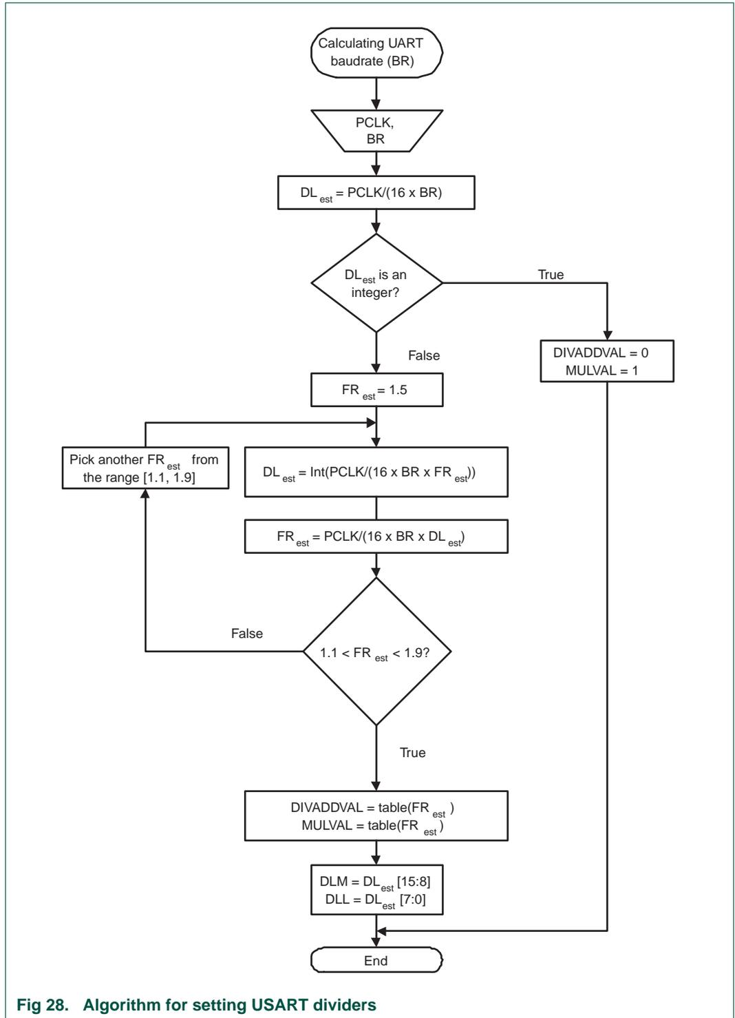
Fig 28. Algorithm for setting USART dividers
