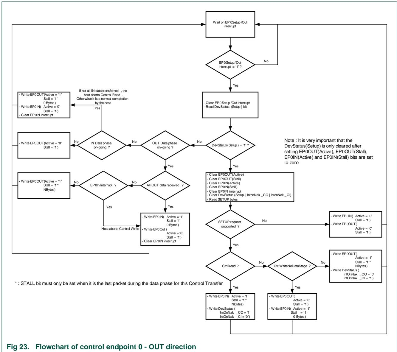
Fig 23. Flowchart of control endpoint 0 - OUT direction
