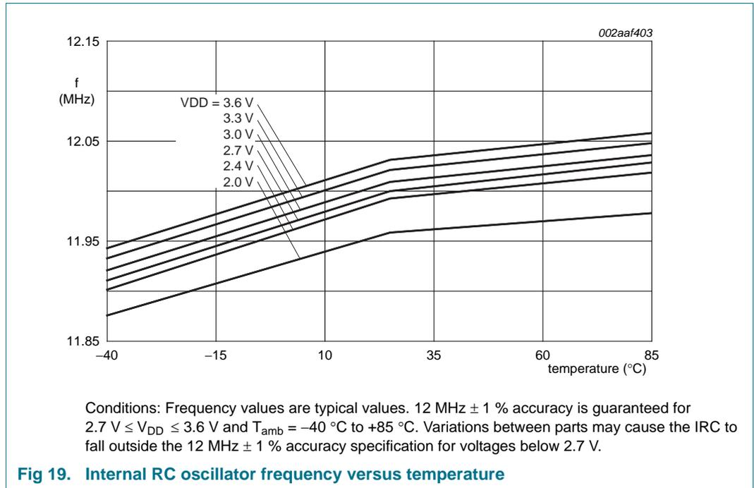
**Fig 19. Internal RC oscillator frequency versus temperature**
