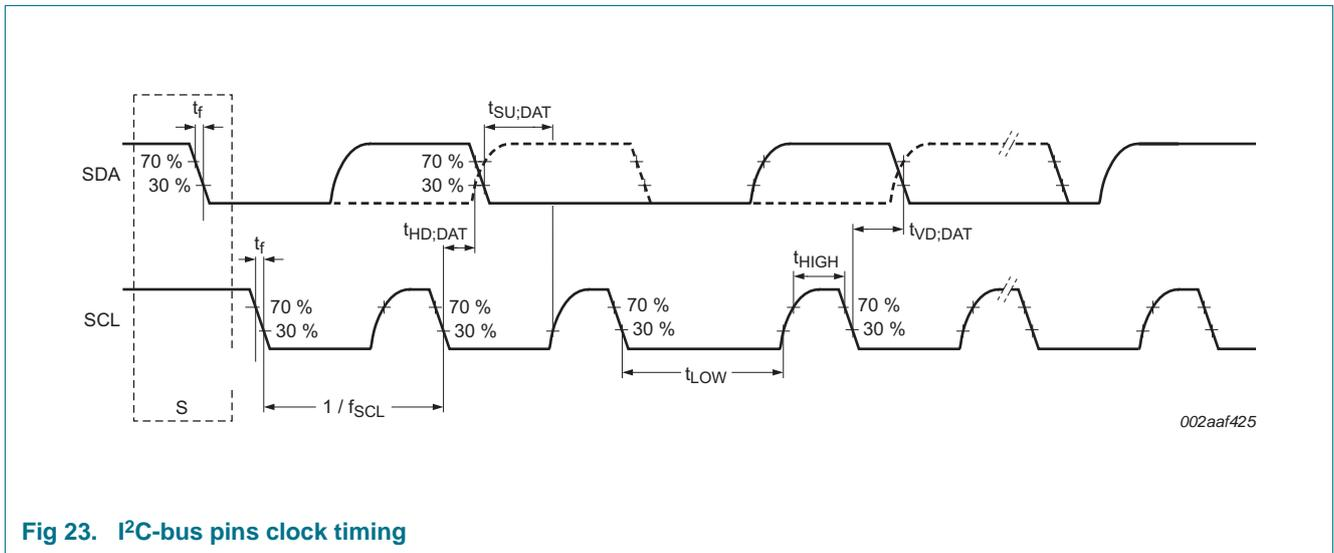
Fig 23. I<sup>2</sup>C-bus pins clock timing
