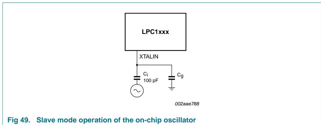
**Fig 49. Slave mode operation of the on-chip oscillator**
