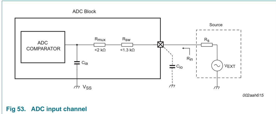
Fig 53. ADC input channel
