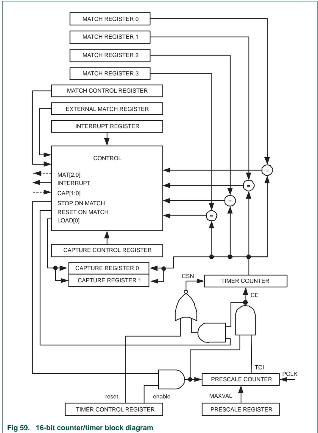
Fig 59. 16-bit counter/timer block diagram
