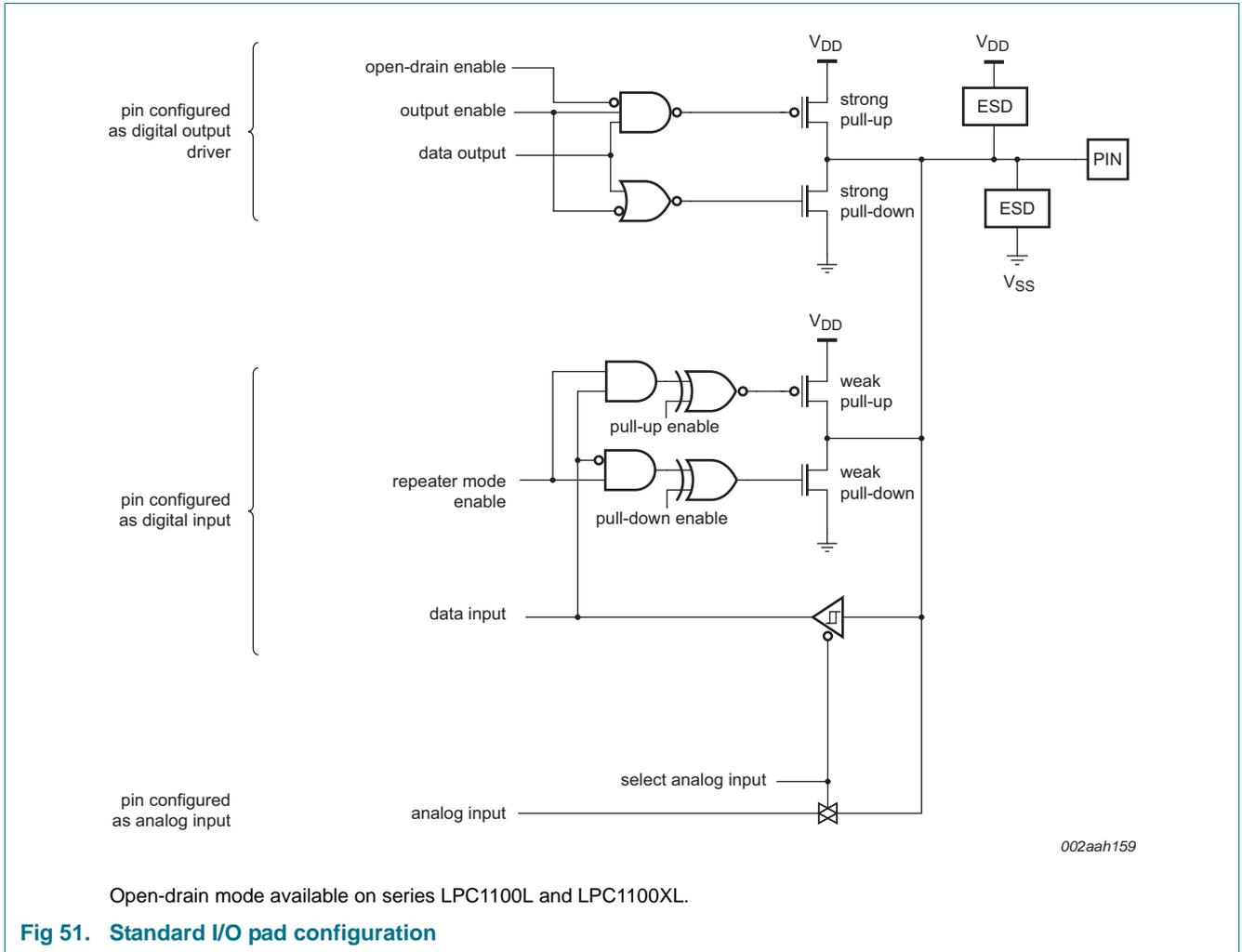
Fig 51. Standard I/O pad configuration
