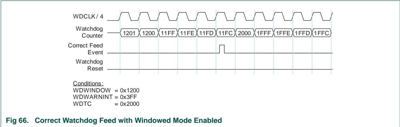
Fig 66. Correct Watchdog Feed with Windowed Mode Enabled
