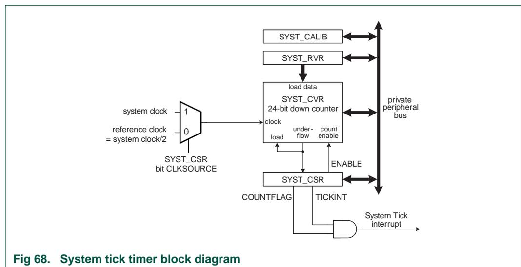
Fig 68. System tick timer block diagram
