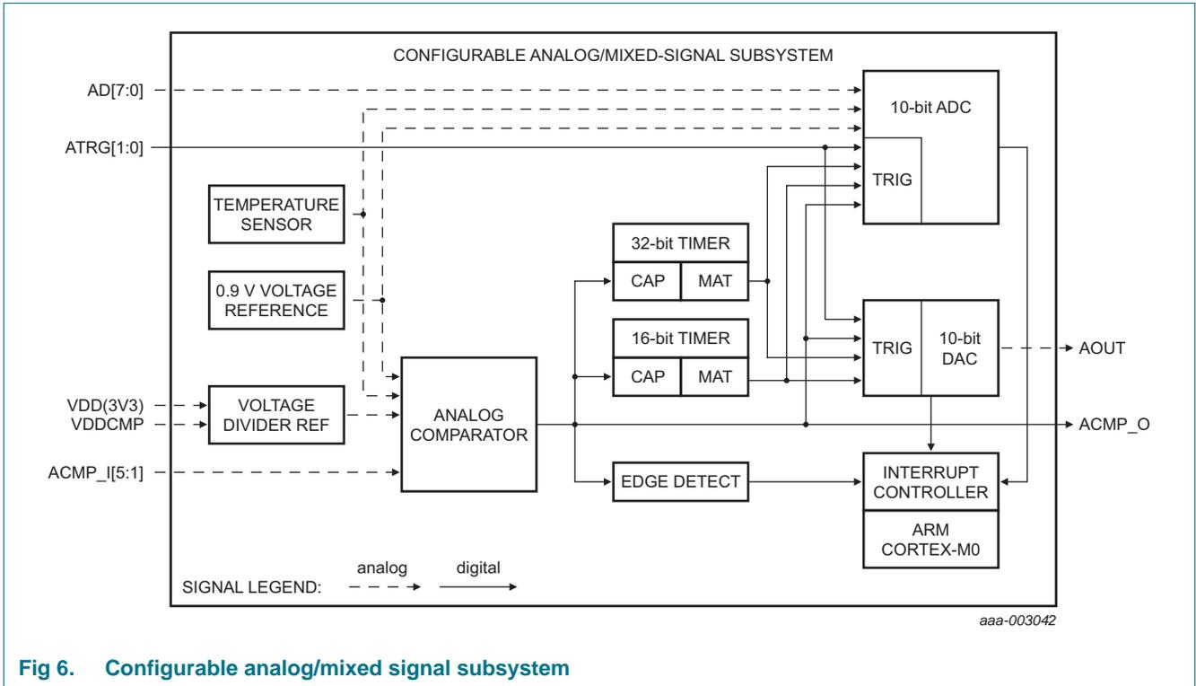
Fig 6. Configurable analog/mixed signal subsystem
