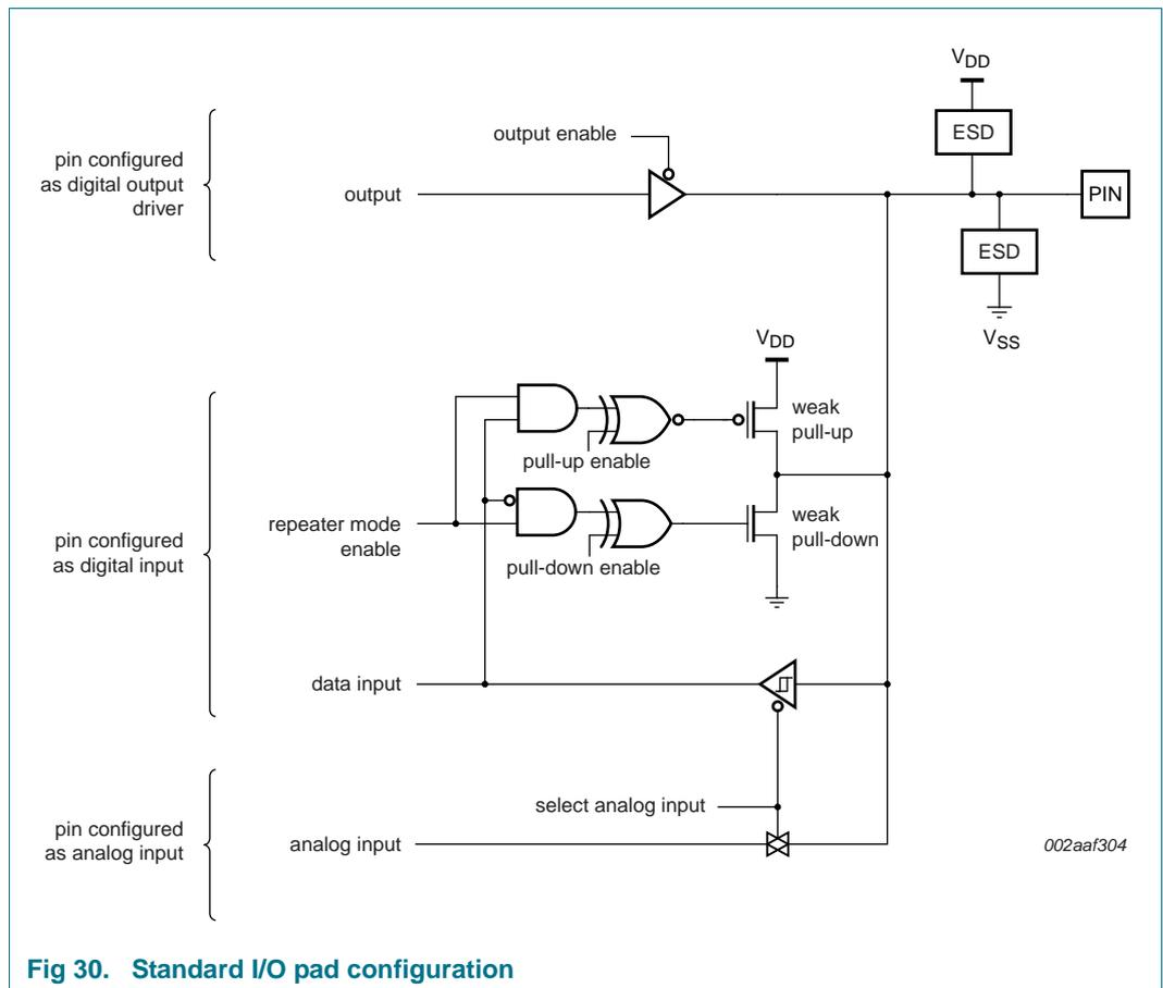
Fig 30. Standard I/O pad configuration
