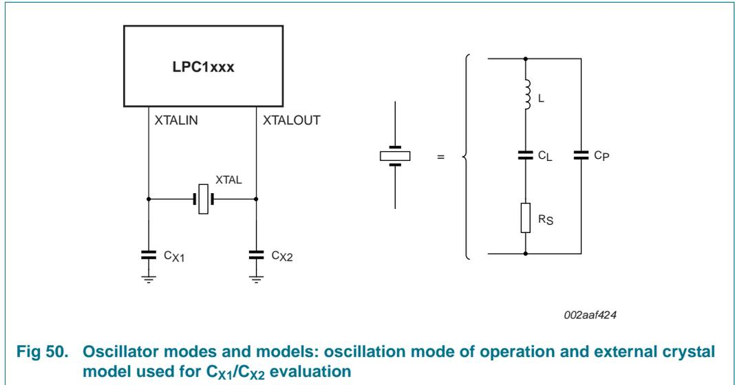
**Fig 50. Oscillator modes and models: oscillation mode of operation and external crystal model used for  $C_{X1}/C_{X2}$  evaluation**
