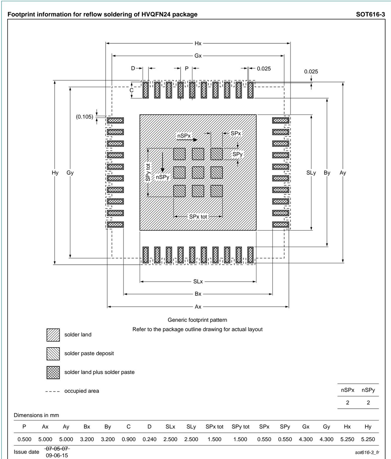
**Fig 66. Reflow soldering of the HVQFN24 package**
