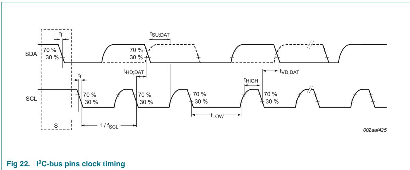
Fig 22. I<sup>2</sup>C-bus pins clock timing
