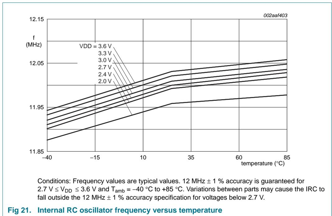
**Fig 21. Internal RC oscillator frequency versus temperature**
