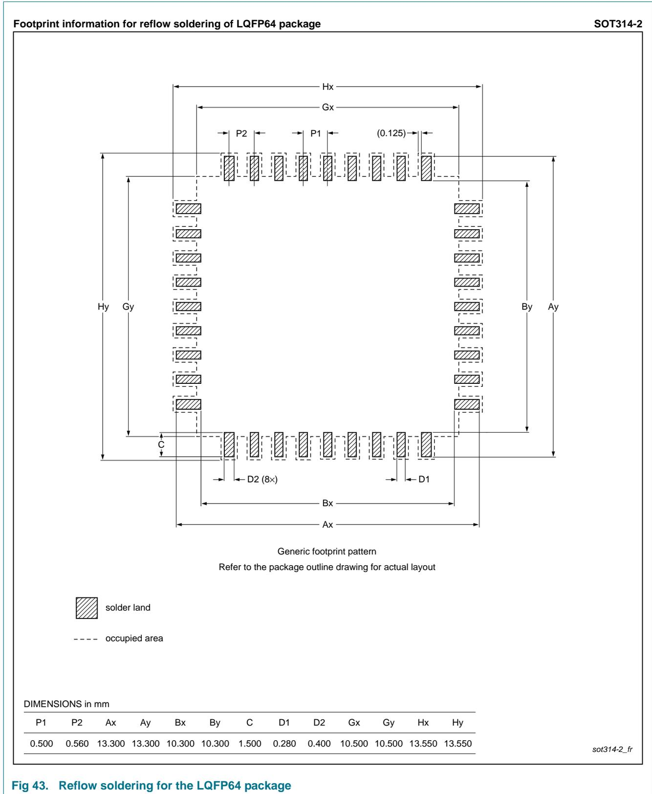
**Fig 43. Reflow soldering for the LQFP64 package**
