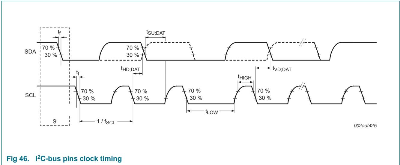
Fig 46. I<sup>2</sup>C-bus pins clock timing
