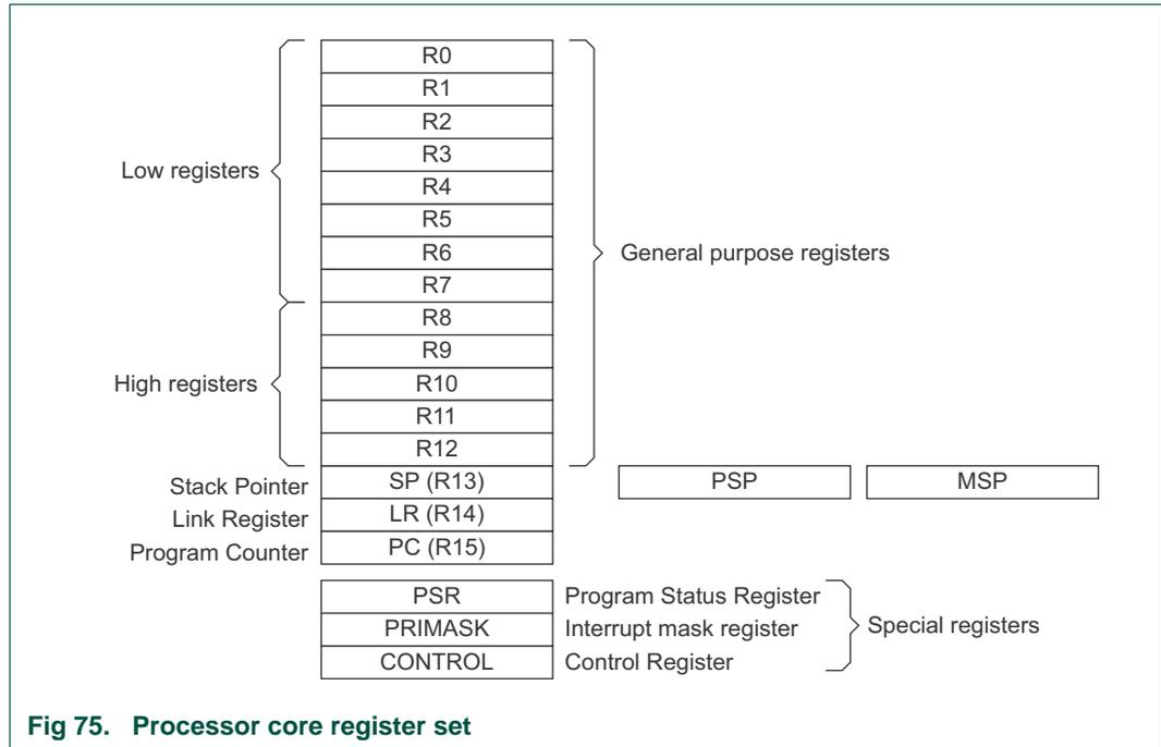
Fig 75. Processor core register set
