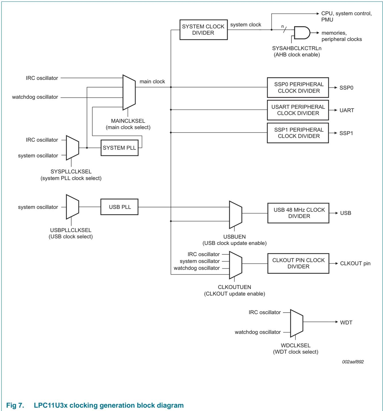
Fig 7. LPC11U3x clocking generation block diagram
