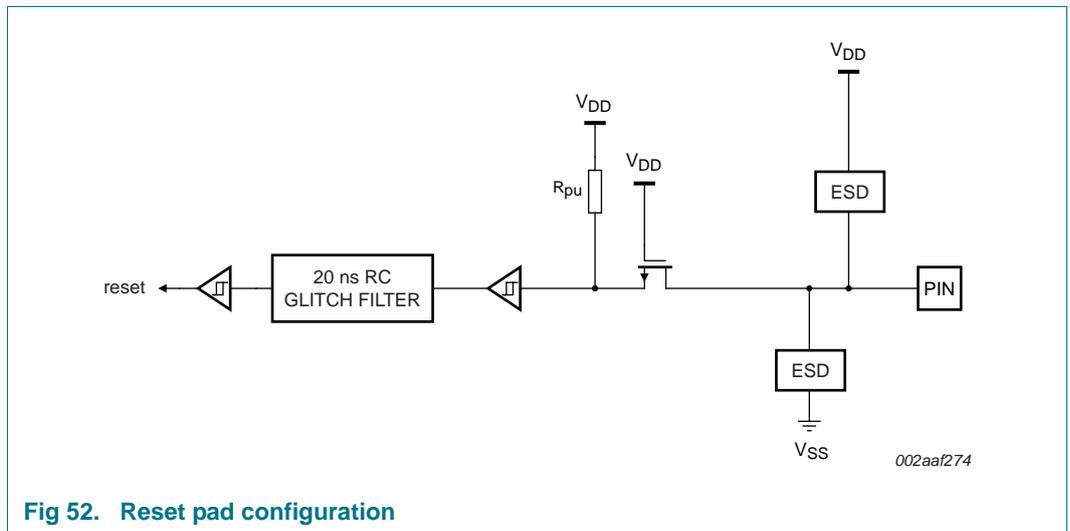
Fig 52. Reset pad configuration
