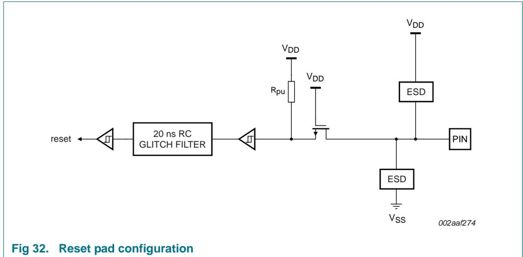
Fig 32. Reset pad configuration
