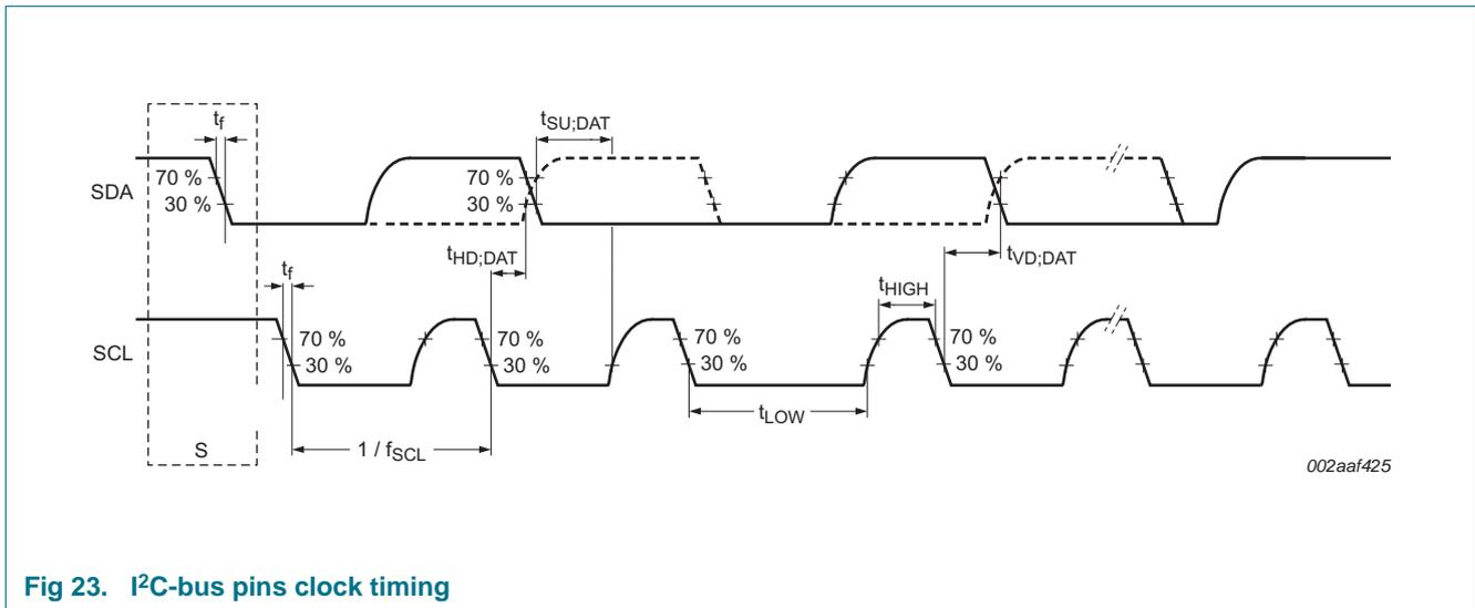
Fig 23. I<sup>2</sup>C-bus pins clock timing
