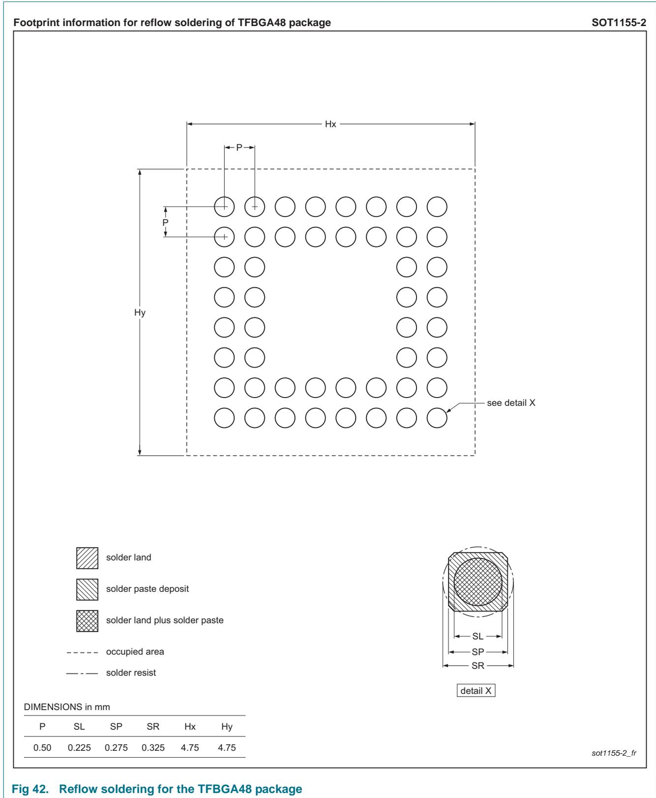
**Fig 42. Reflow soldering for the TFBGA48 package**
