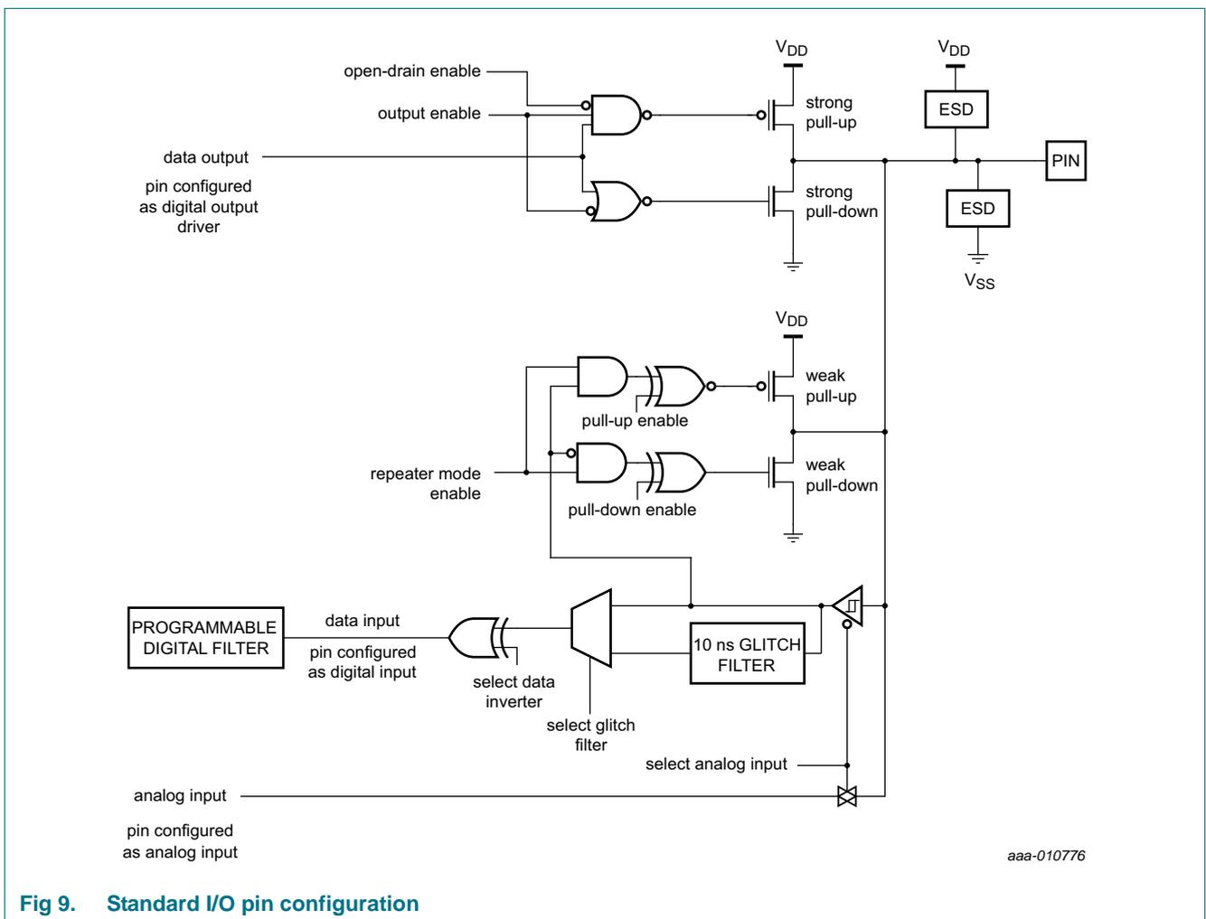
**Fig 9. Standard I/O pin configuration**
