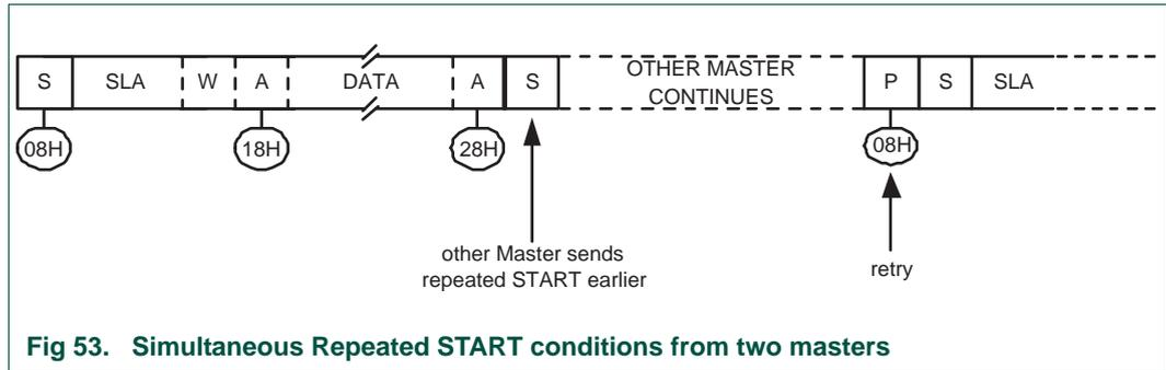
Fig 53. Simultaneous Repeated START conditions from two masters
