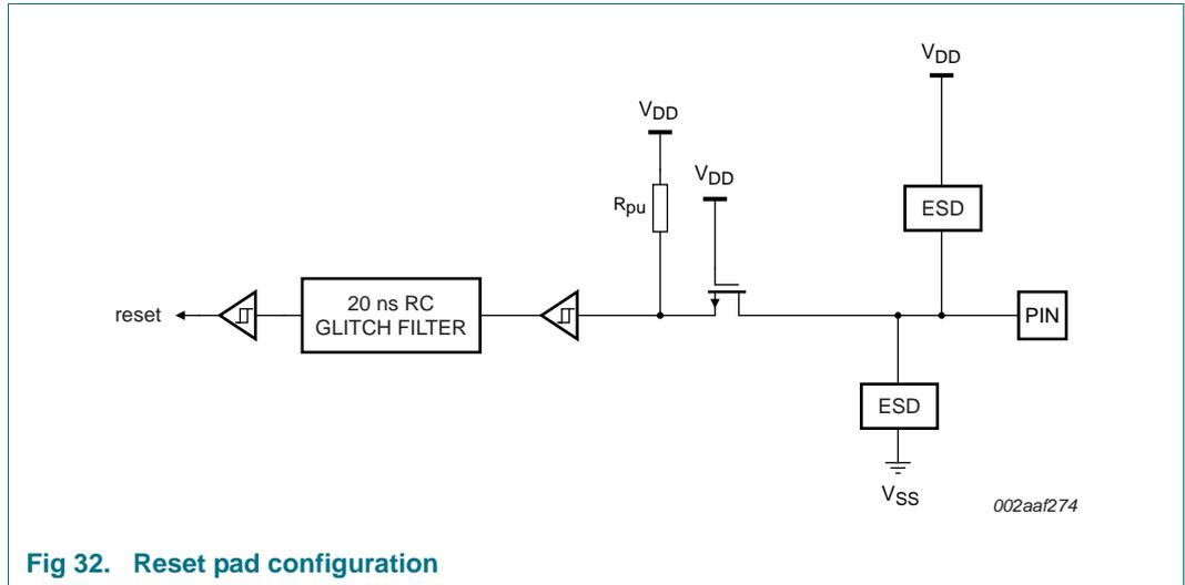
Fig 32. Reset pad configuration
