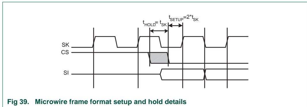
**Fig 39. Microwire frame format setup and hold details**
