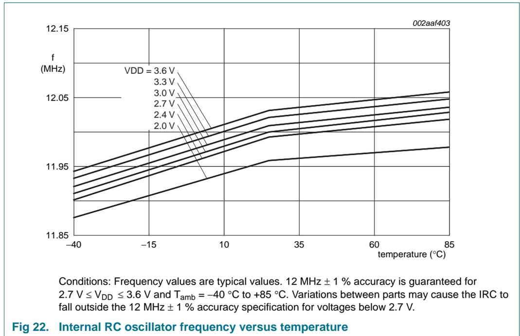
Conditions: Frequency values are typical values.  $12\text{ MHz} \pm 1\%$  accuracy is guaranteed for  $2.7\text{ V} \leq V_{DD} \leq 3.6\text{ V}$  and  $T_{amb} = -40\text{ }^{\circ}\text{C}$  to  $+85\text{ }^{\circ}\text{C}$ . Variations between parts may cause the IRC to fall outside the  $12\text{ MHz} \pm 1\%$  accuracy specification for voltages below 2.7 V.
