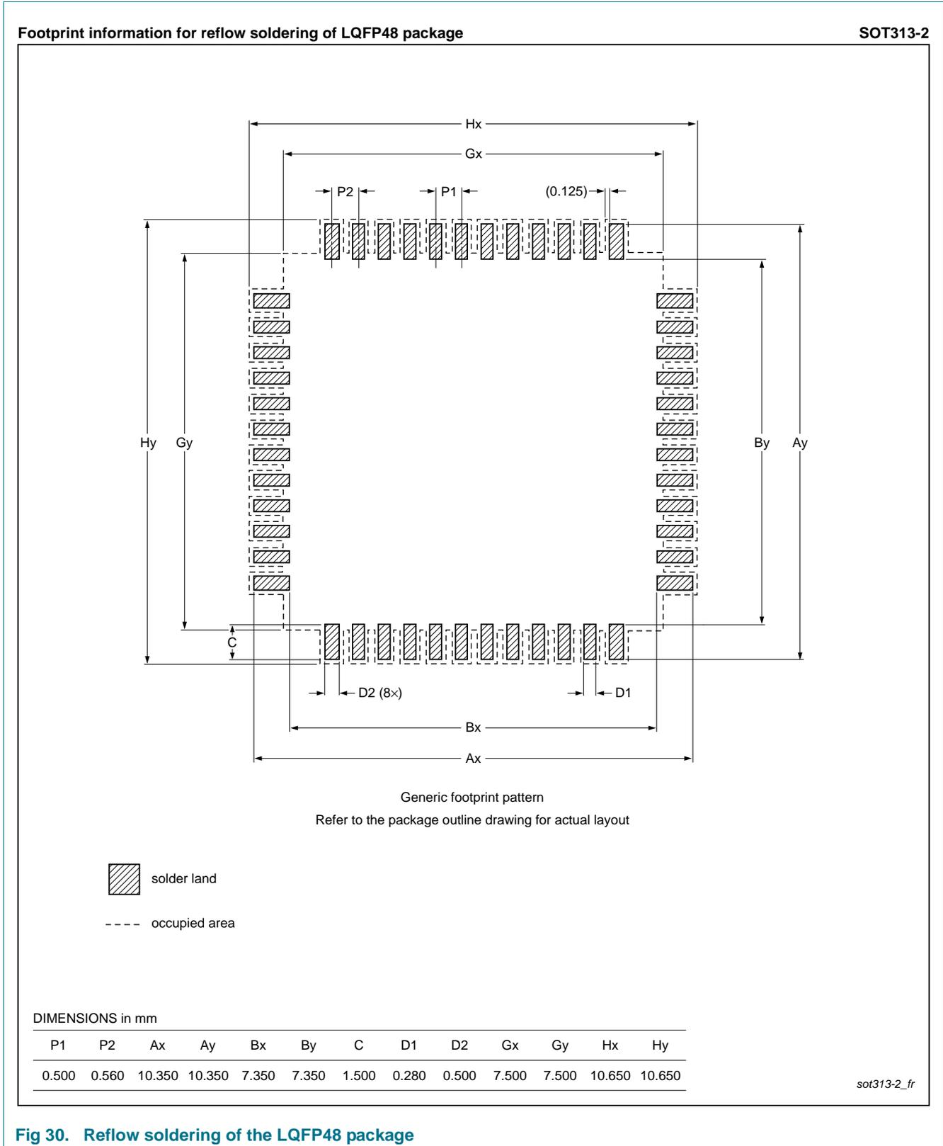
Fig 30. Reflow soldering of the LQFP48 package
