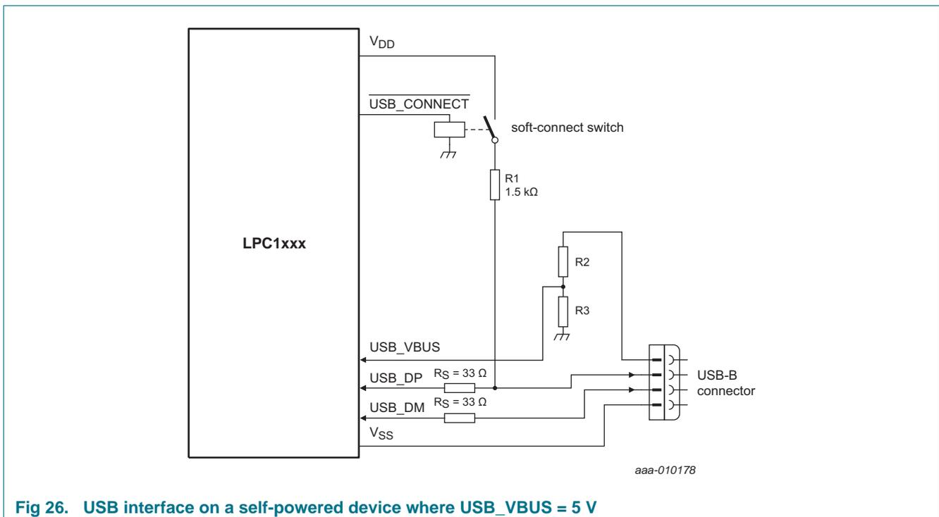
Fig 26. USB interface on a self-powered device where  $USB\_VBUS = 5 \text{ V}$
