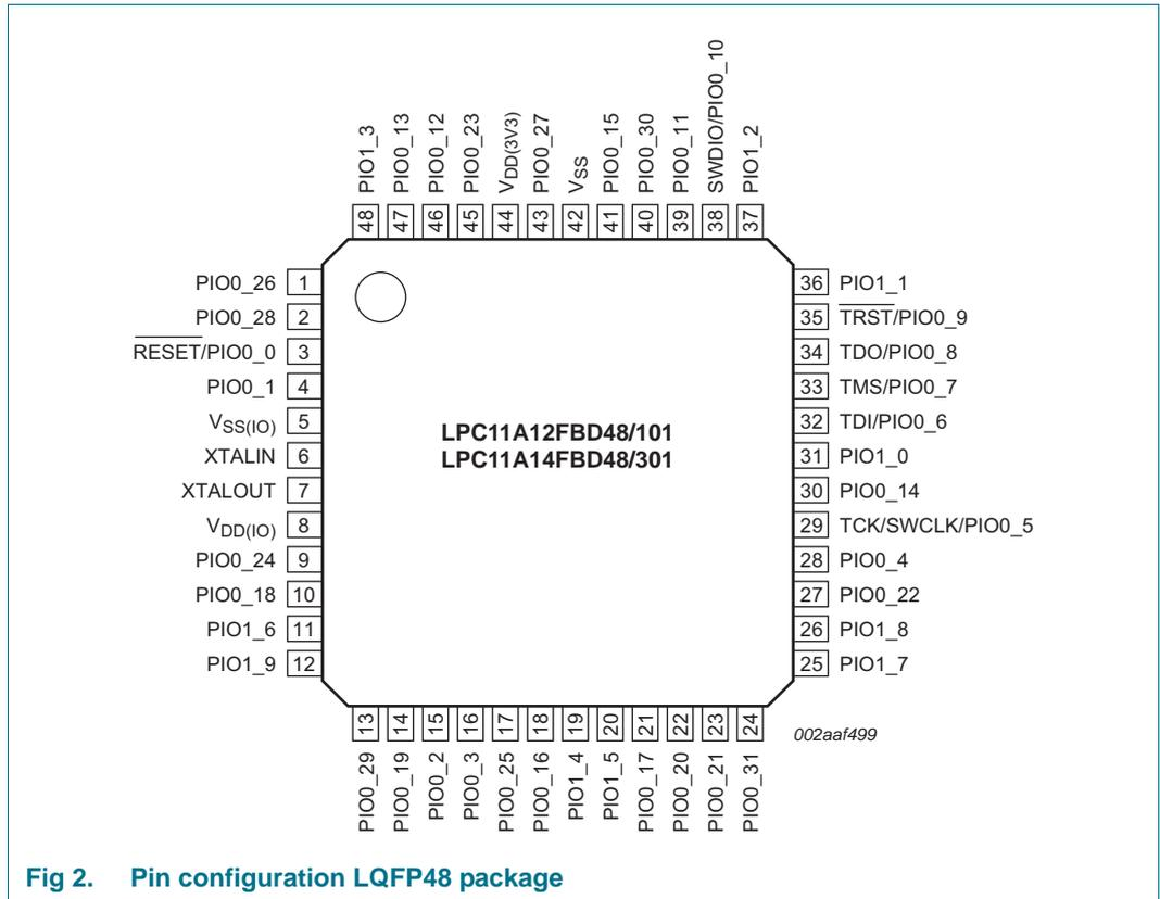
Fig 2. Pin configuration LQFP48 package
