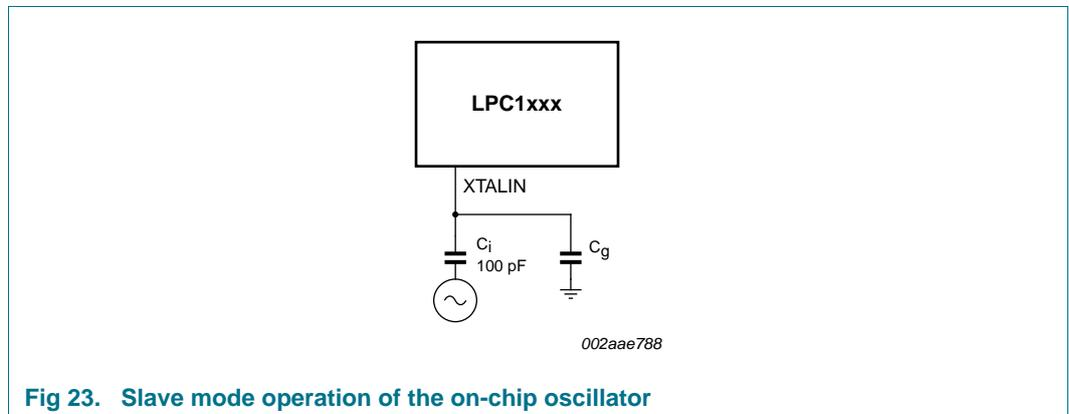
**Fig 23. Slave mode operation of the on-chip oscillator**
