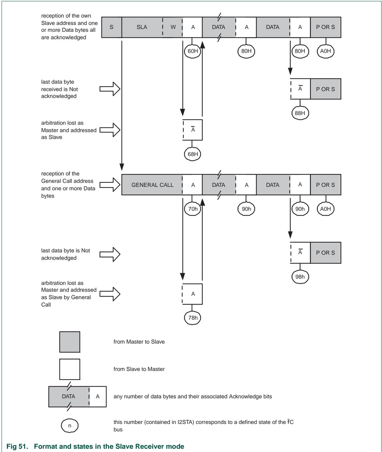
Fig 51. Format and states in the Slave Receiver mode
