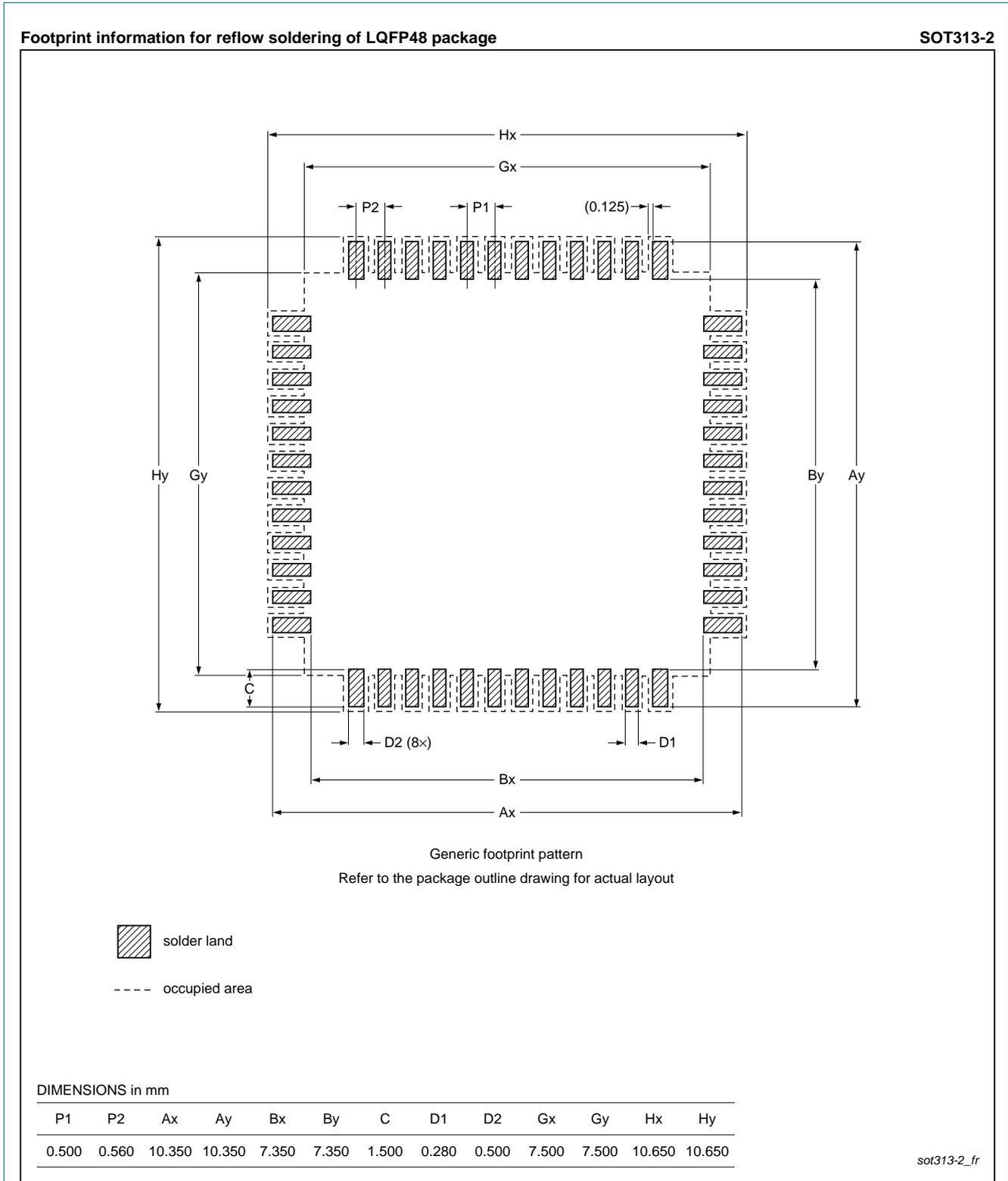
**Fig 69. Reflow soldering of the LQFP48 package**
