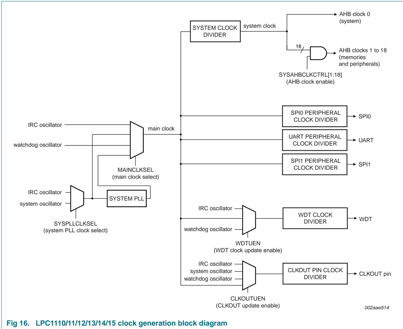
Fig 16. LPC1110/11/12/13/14/15 clock generation block diagram
