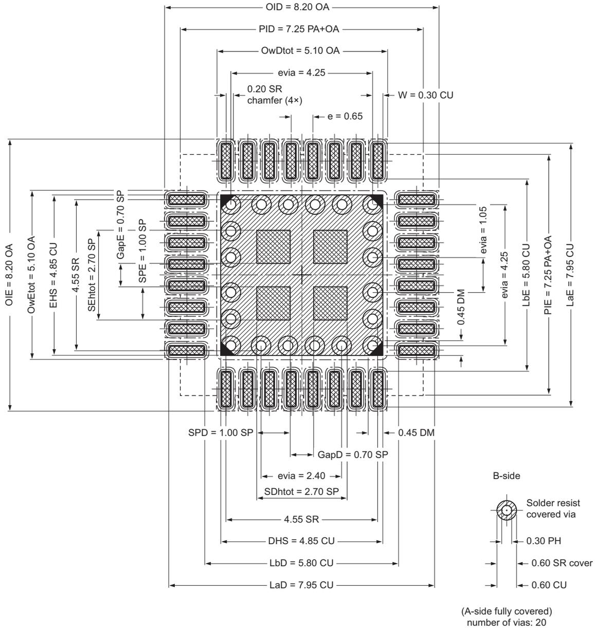
Fig 39. Reflow soldering of the HVQFN33(7x7) package
