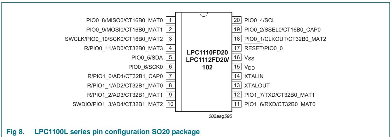
Fig 8. LPC1100L series pin configuration SO20 package
