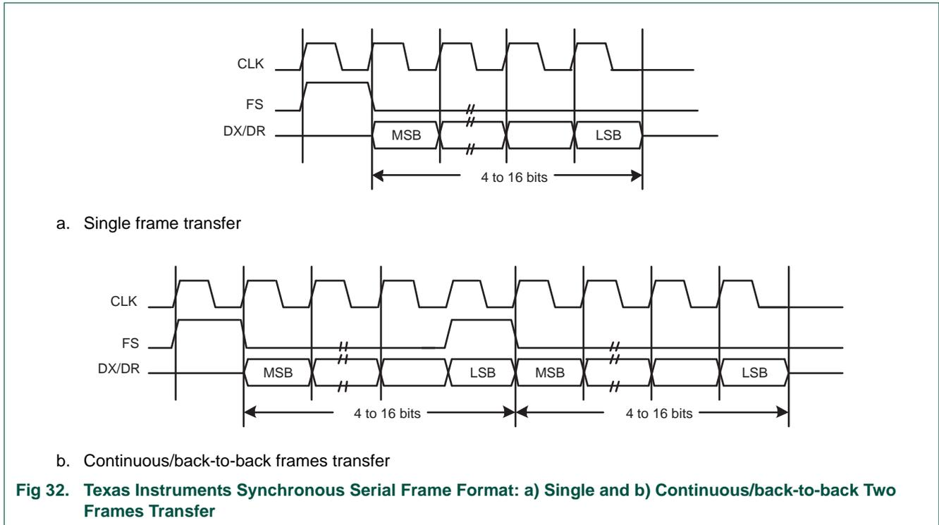
**Fig 32. Texas Instruments Synchronous Serial Frame Format: a) Single and b) Continuous/back-to-back Two Frames Transfer**
