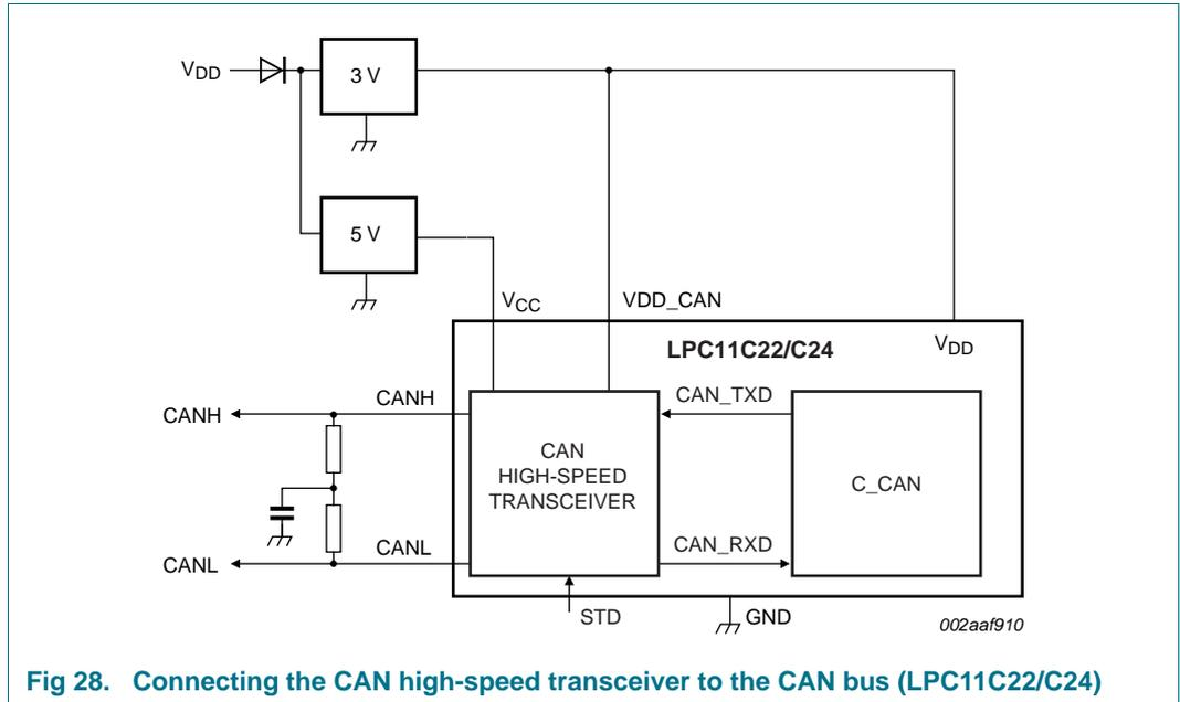
Fig 28. Connecting the CAN high-speed transceiver to the CAN bus (LPC11C22/C24)
