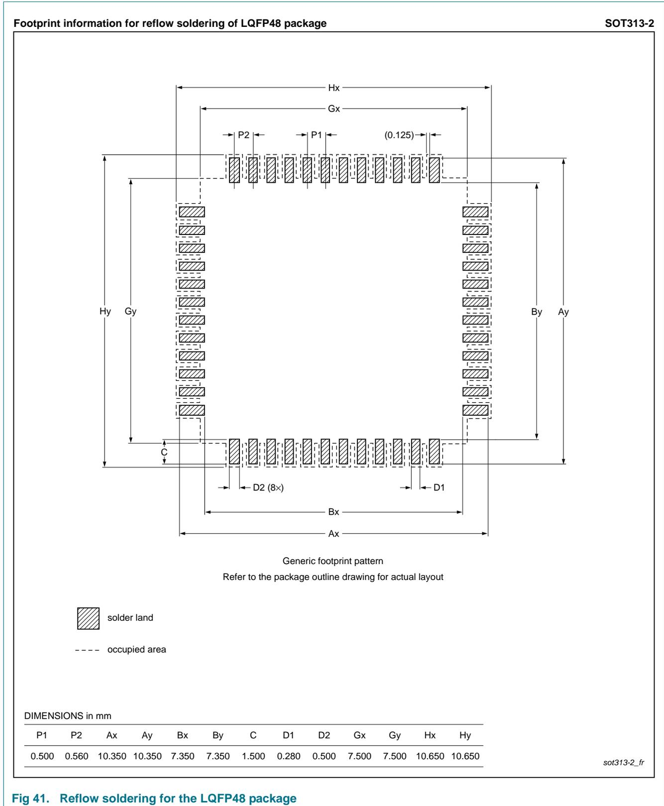
**Fig 41. Reflow soldering for the LQFP48 package**
