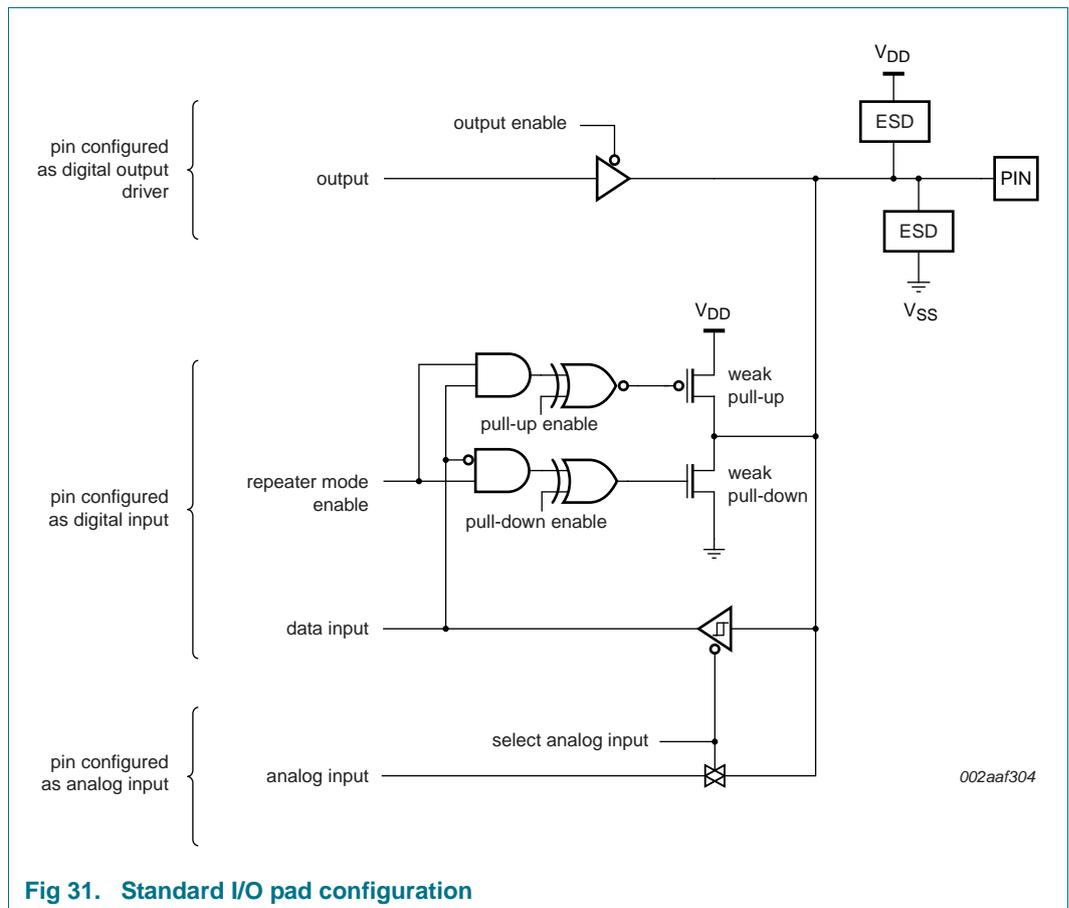
Fig 31. Standard I/O pad configuration
