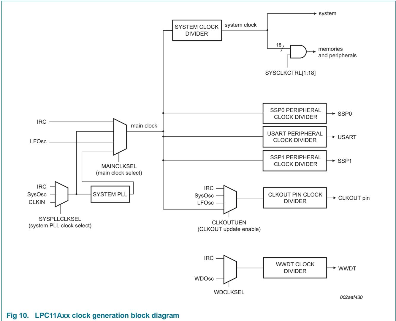
Fig 10. LPC11Axx clock generation block diagram
