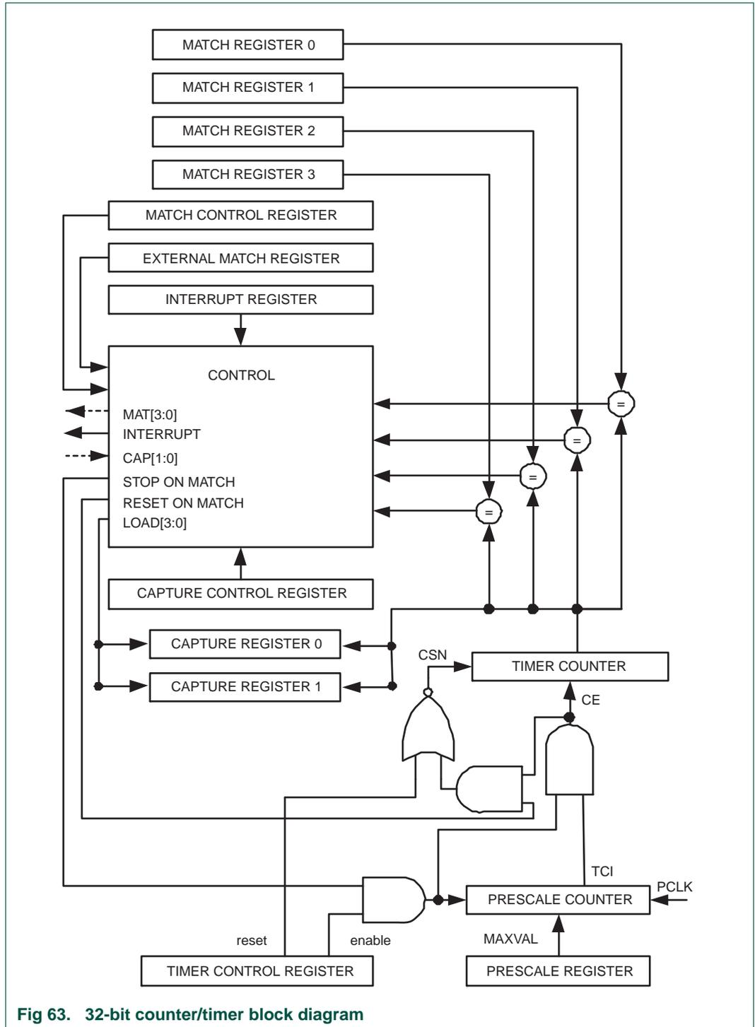
Fig 63. 32-bit counter/timer block diagram
