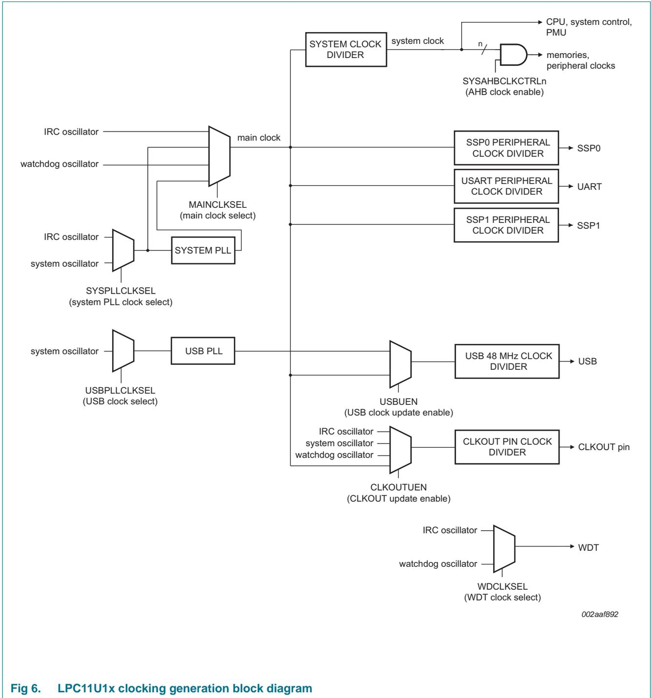
Fig 6. LPC11U1x clocking generation block diagram
