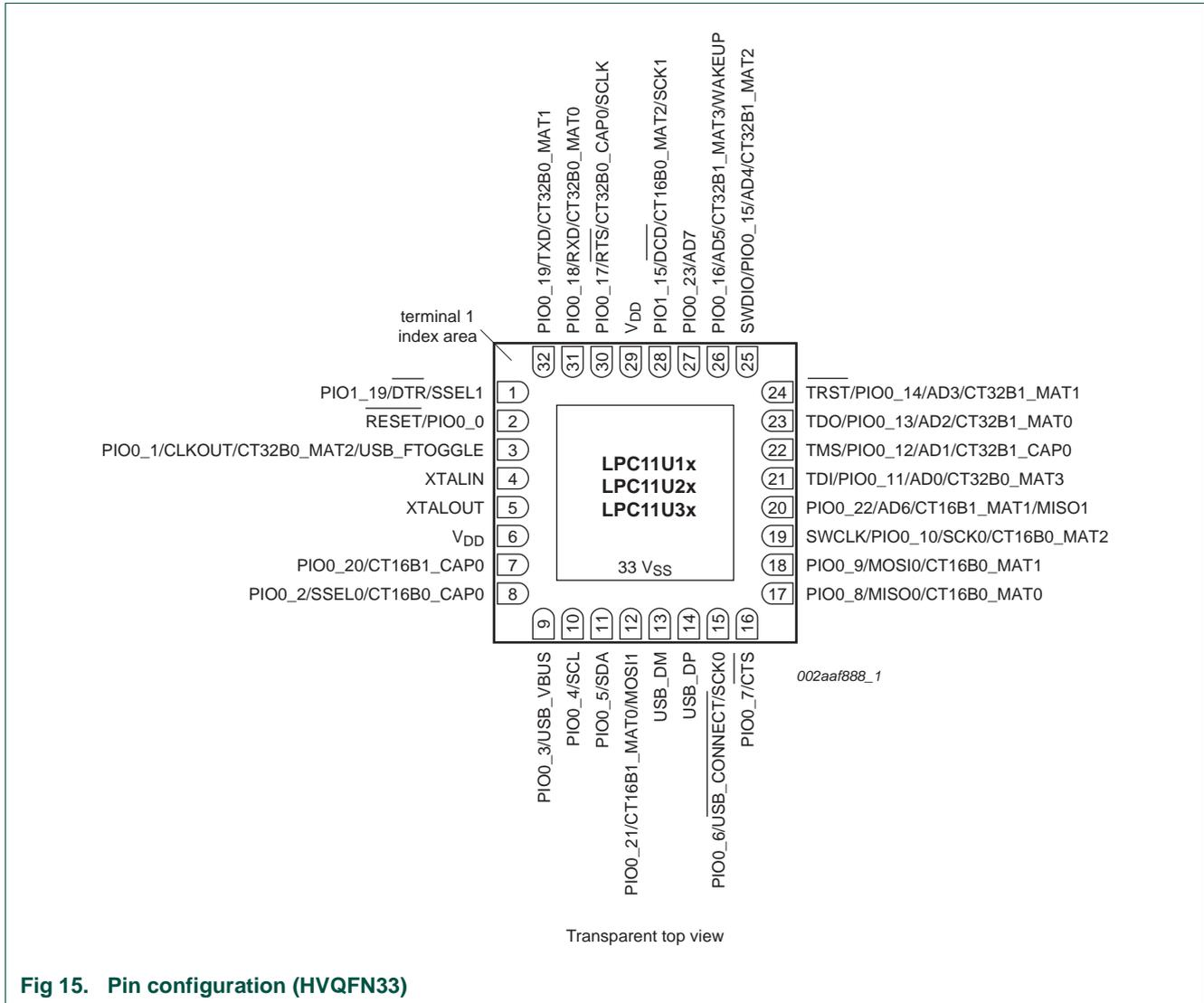
Fig 15. Pin configuration (HVQFN33)
