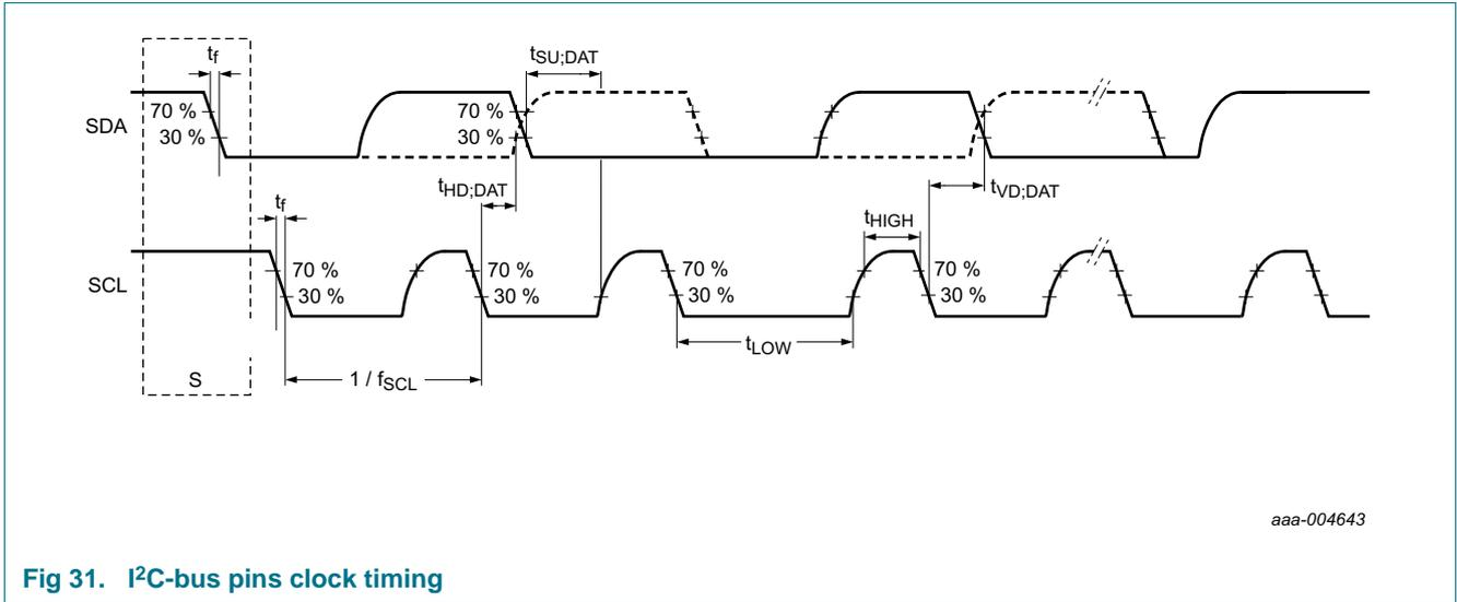
Fig 31. I<sup>2</sup>C-bus pins clock timing
