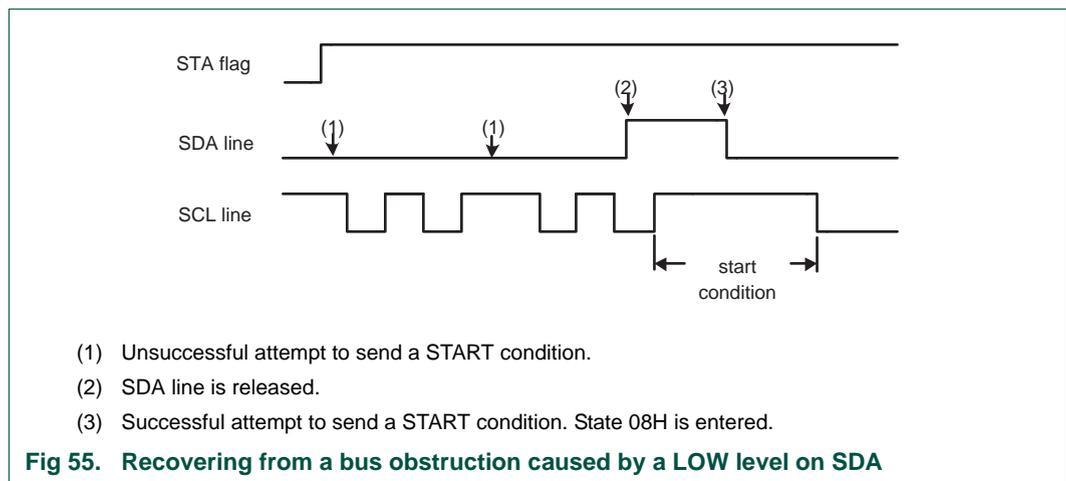
**Fig 55. Recovering from a bus obstruction caused by a LOW level on SDA**
