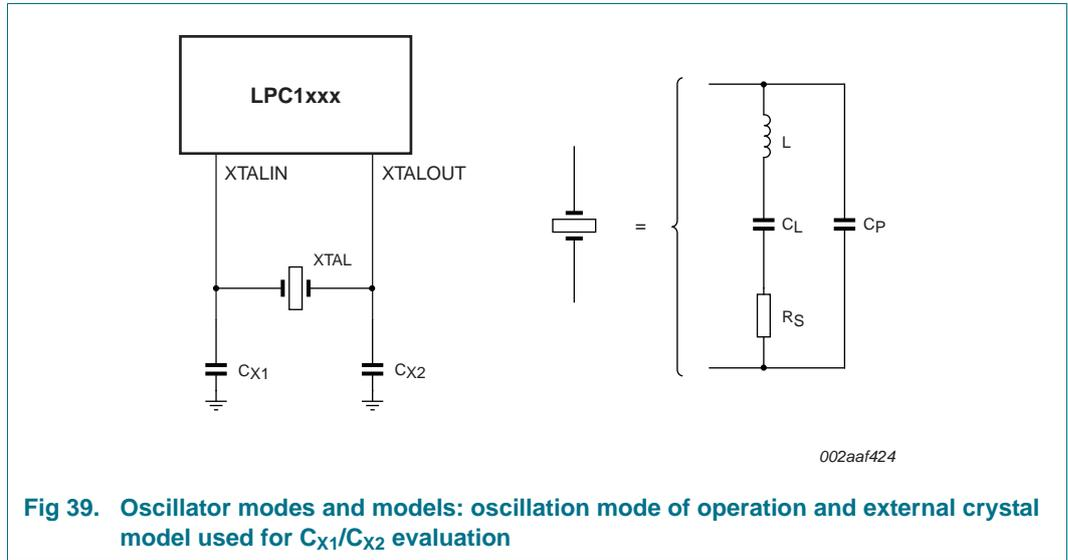
Fig 39. Oscillator modes and models: oscillation mode of operation and external crystal model used for  $C_{X1}/C_{X2}$  evaluation
