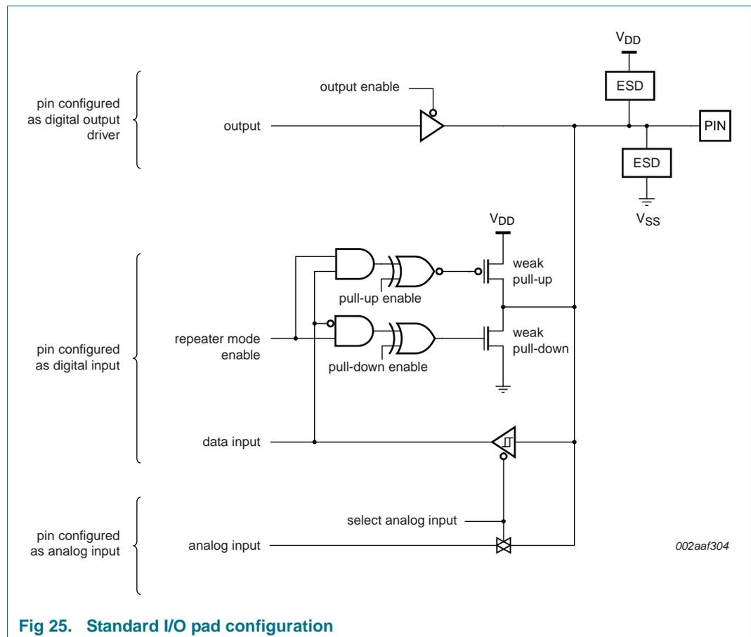
Fig 25. Standard I/O pad configuration
