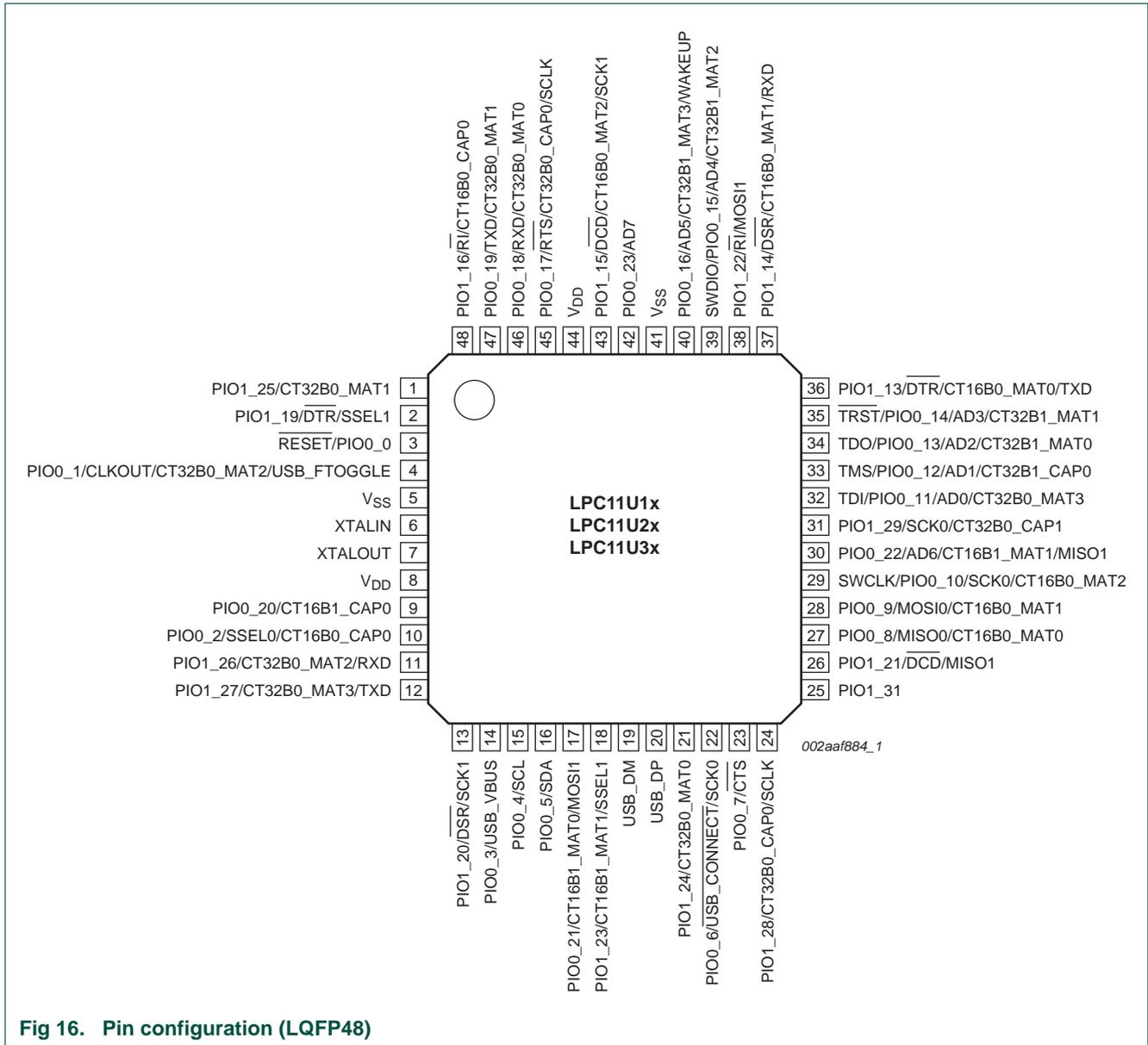
Fig 16. Pin configuration (LQFP48)
