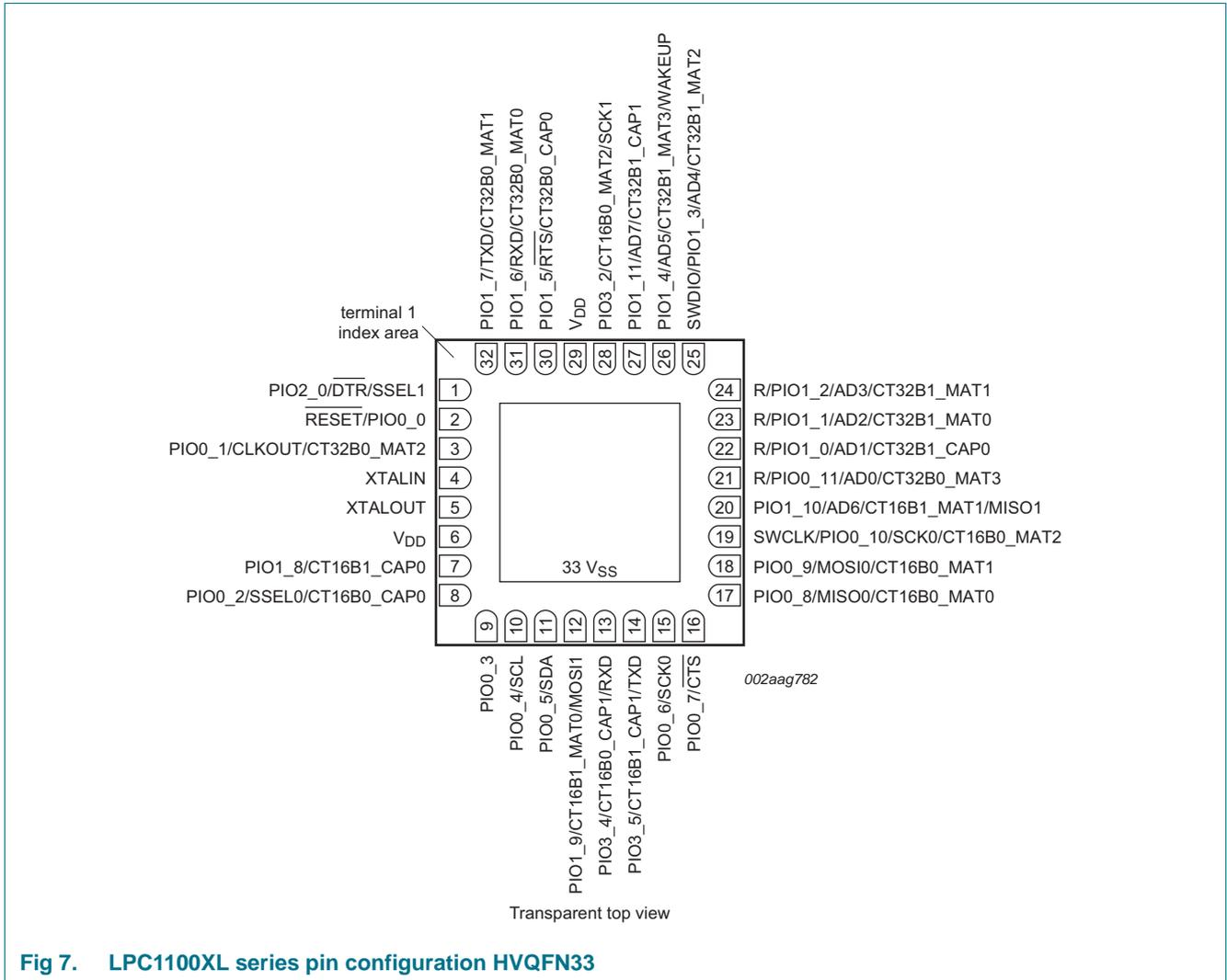
Fig 7. LPC1100XL series pin configuration HVQFN33
