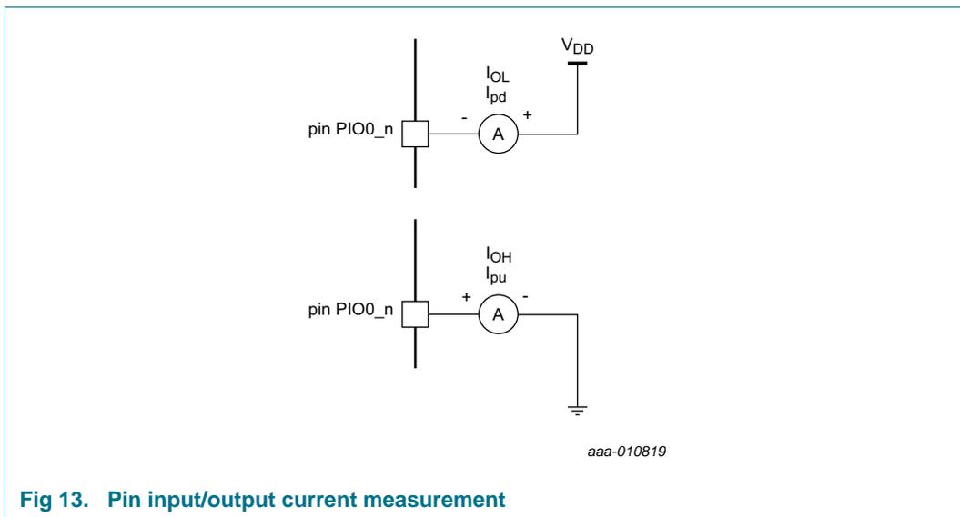
**Fig 13. Pin input/output current measurement**
