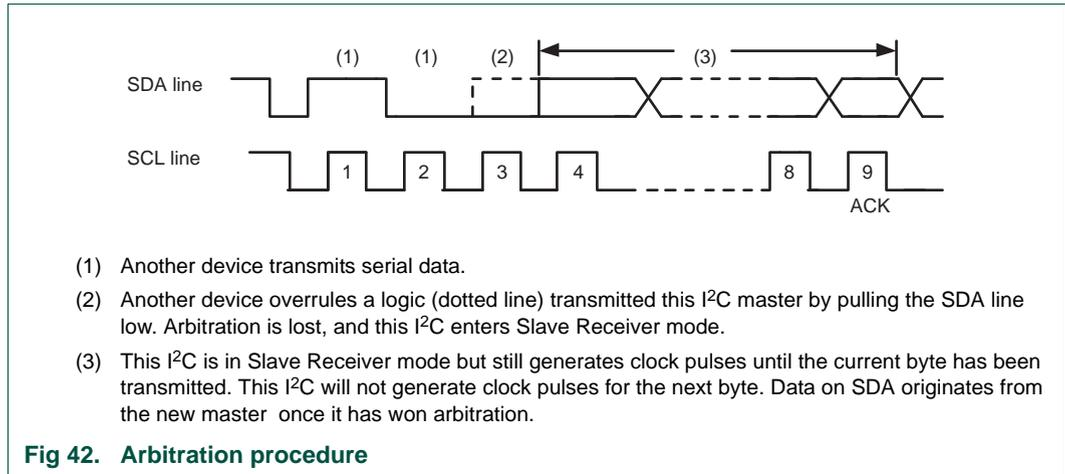
The synchronization logic will synchronize the serial clock generator with the clock pulses on the SCL line from another device. If two or more master devices generate clock pulses, the “mark” duration is determined by the device that generates the shortest “marks,” and the “space” duration is determined by the device that generates the longest “spaces”. [Figure 43](#) shows the synchronization procedure.
