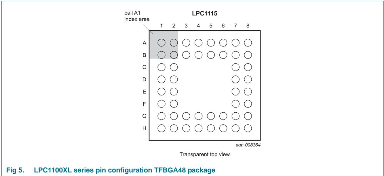
**Fig 5. LPC1100XL series pin configuration TFBGA48 package**
