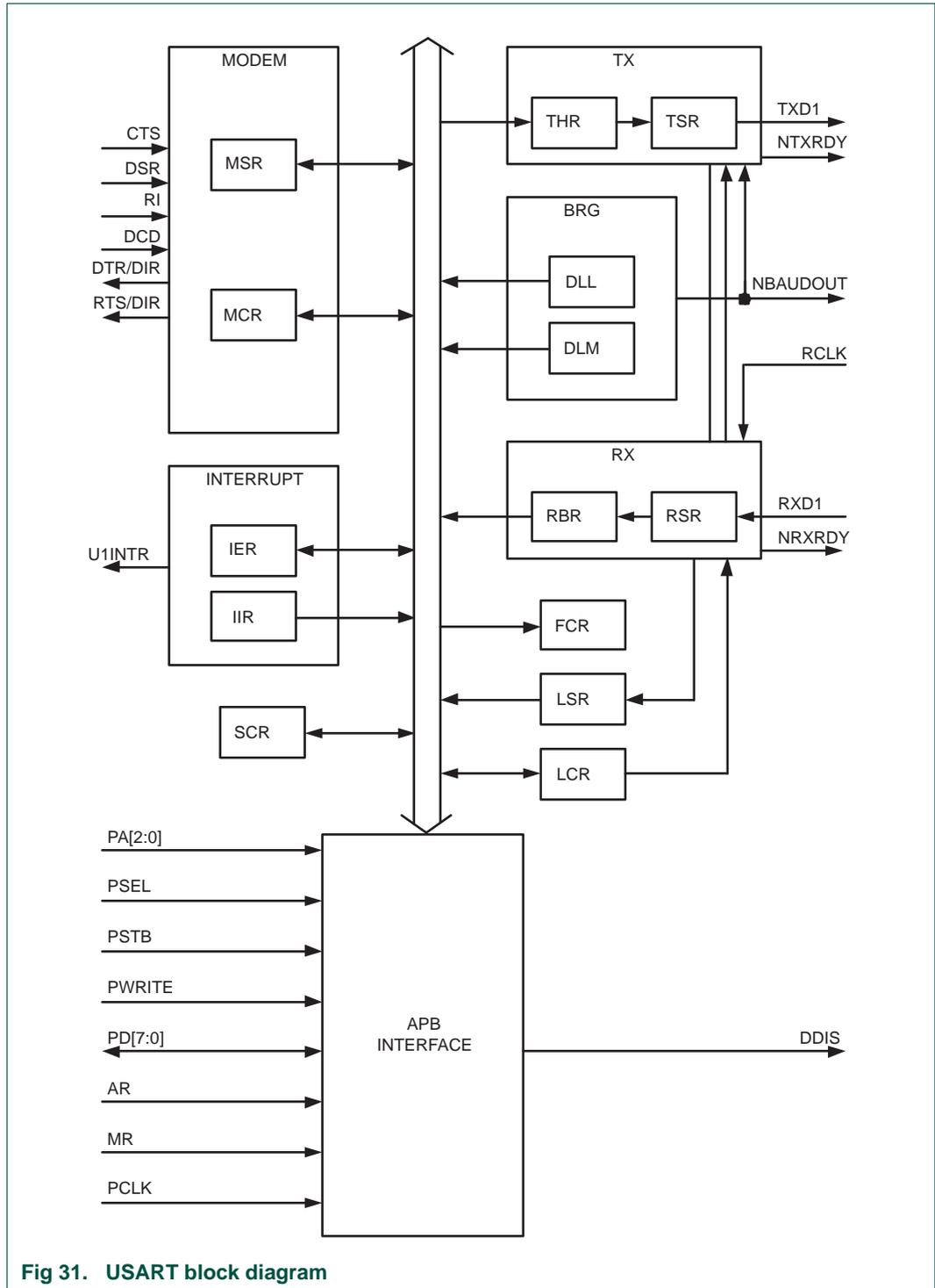
Fig 31. USART block diagram
