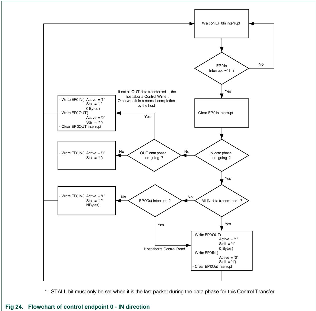
Fig 24. Flowchart of control endpoint 0 - IN direction
