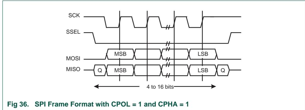
Fig 36. SPI Frame Format with CPOL = 1 and CPHA = 1
