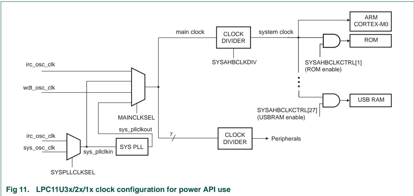
Fig 11. LPC11U3x/2x/1x clock configuration for power API use
