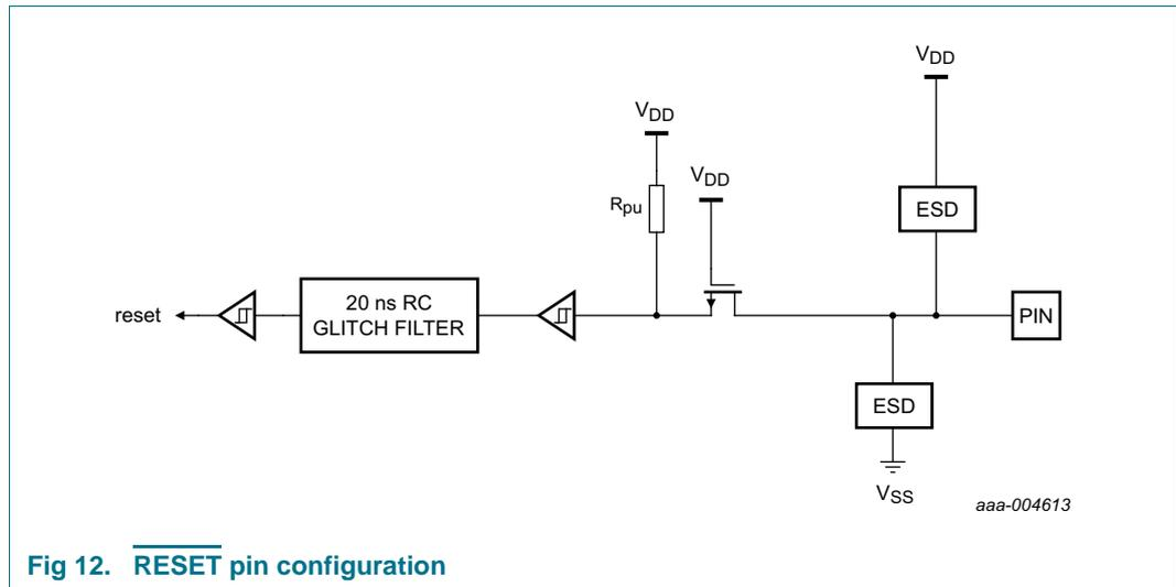
Fig 12. **RESET** pin configuration
