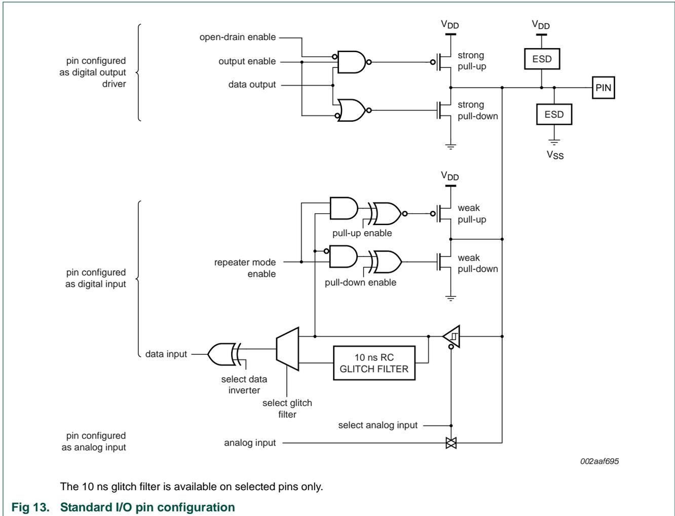
Fig 13. Standard I/O pin configuration
