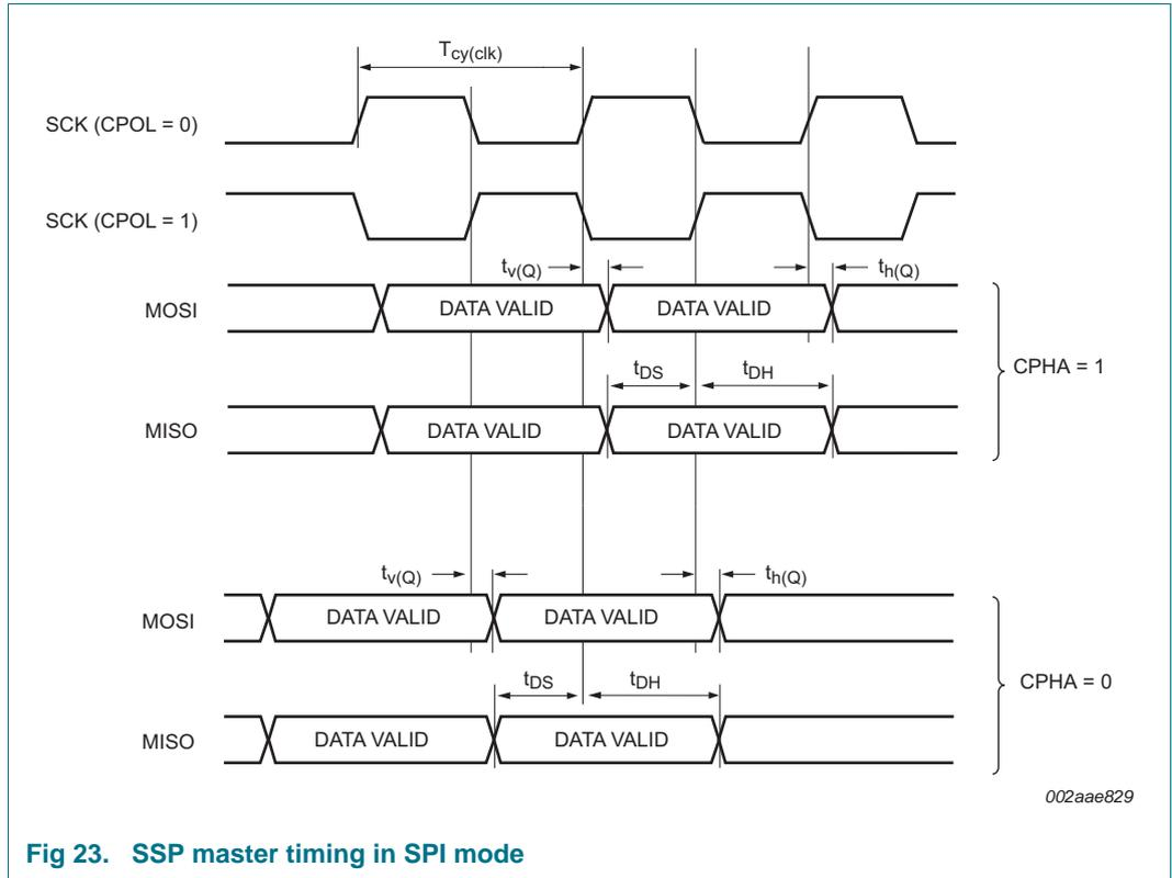
Fig 23. SSP master timing in SPI mode
