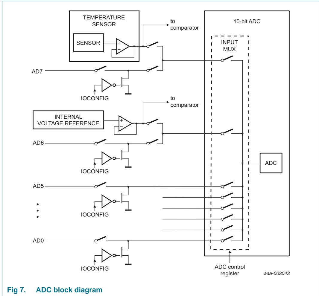
Fig 7. ADC block diagram
