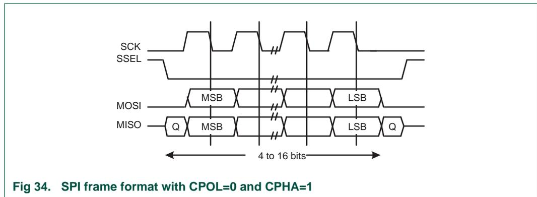
**Fig 34. SPI frame format with CPOL=0 and CPHA=1**
