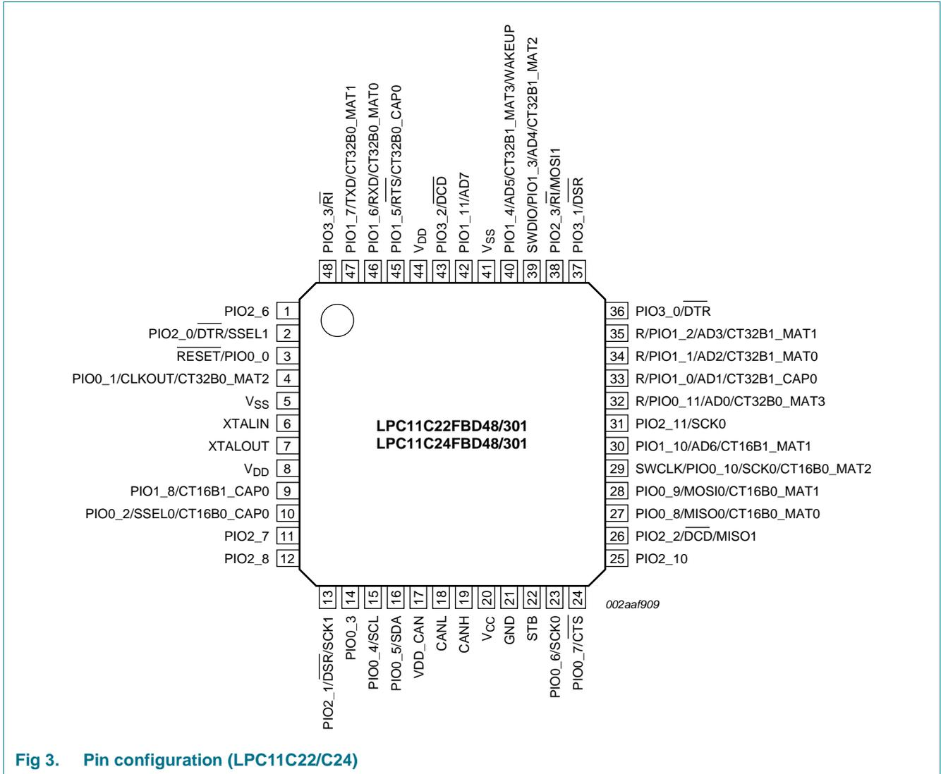
Fig 3. Pin configuration (LPC11C22/C24)
