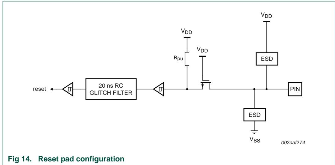
Fig 14. Reset pad configuration
