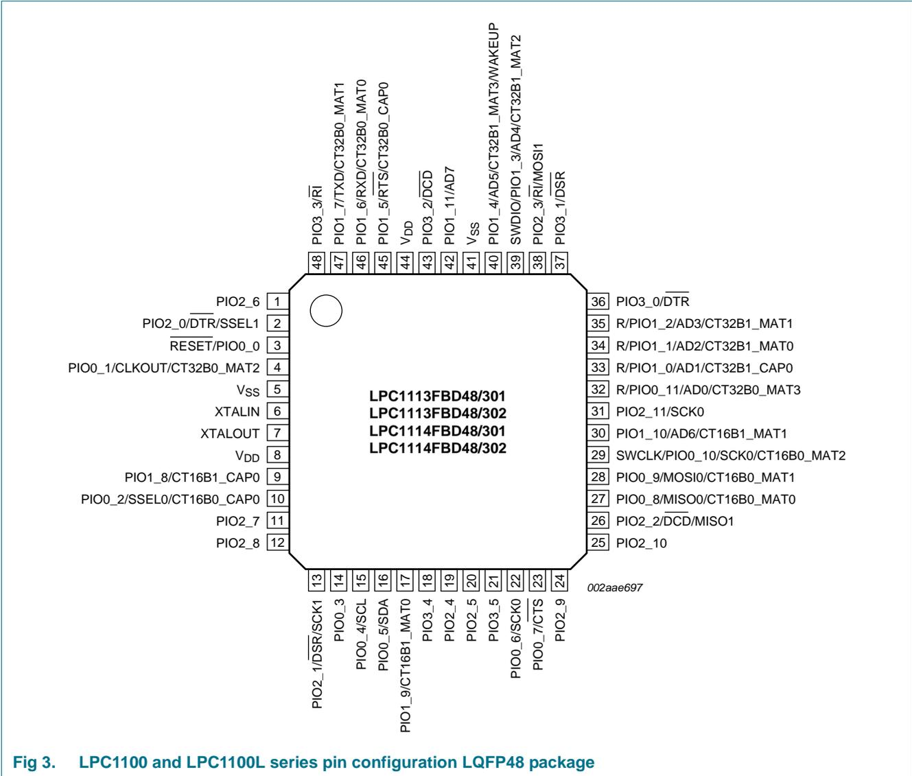
**Fig 3. LPC1100 and LPC1100L series pin configuration LQFP48 package**
