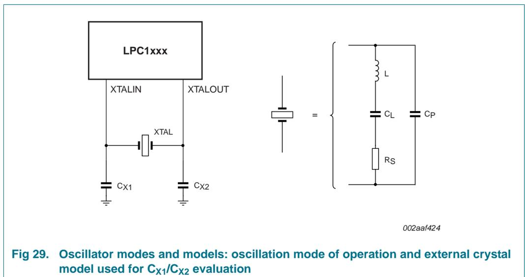
**Fig 29. Oscillator modes and models: oscillation mode of operation and external crystal model used for  $C_{X1}/C_{X2}$  evaluation**
