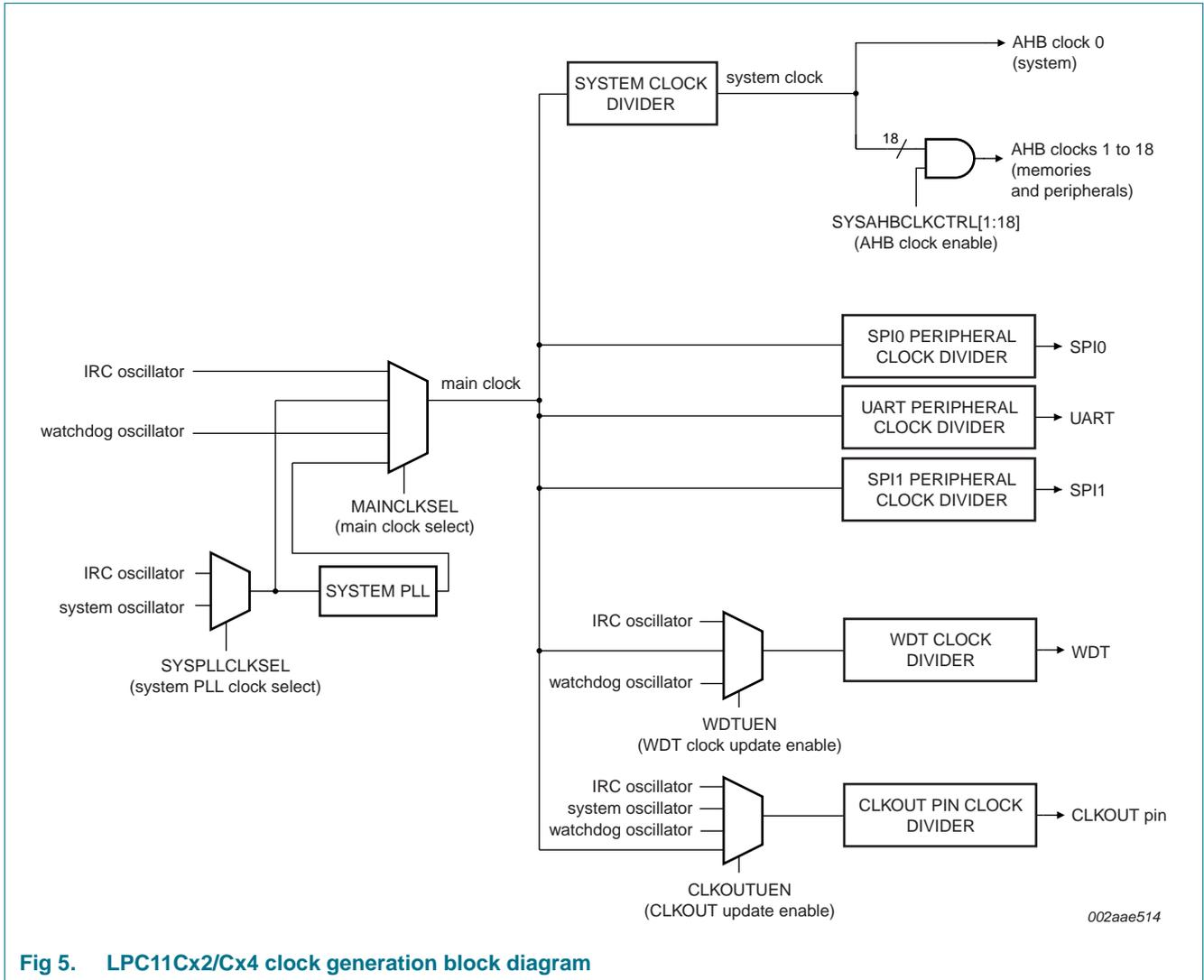
Fig 5. LPC11Cx2/Cx4 clock generation block diagram
