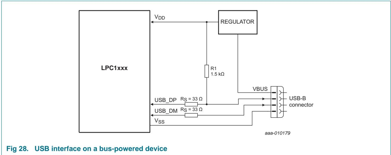
Fig 28. USB interface on a bus-powered device
