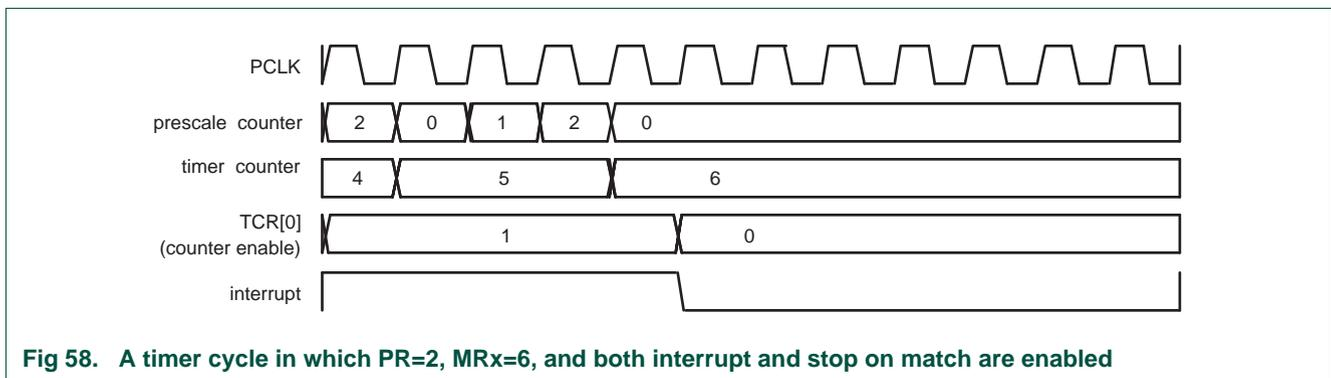
Fig 58. A timer cycle in which PR=2, MRx=6, and both interrupt and stop on match are enabled
