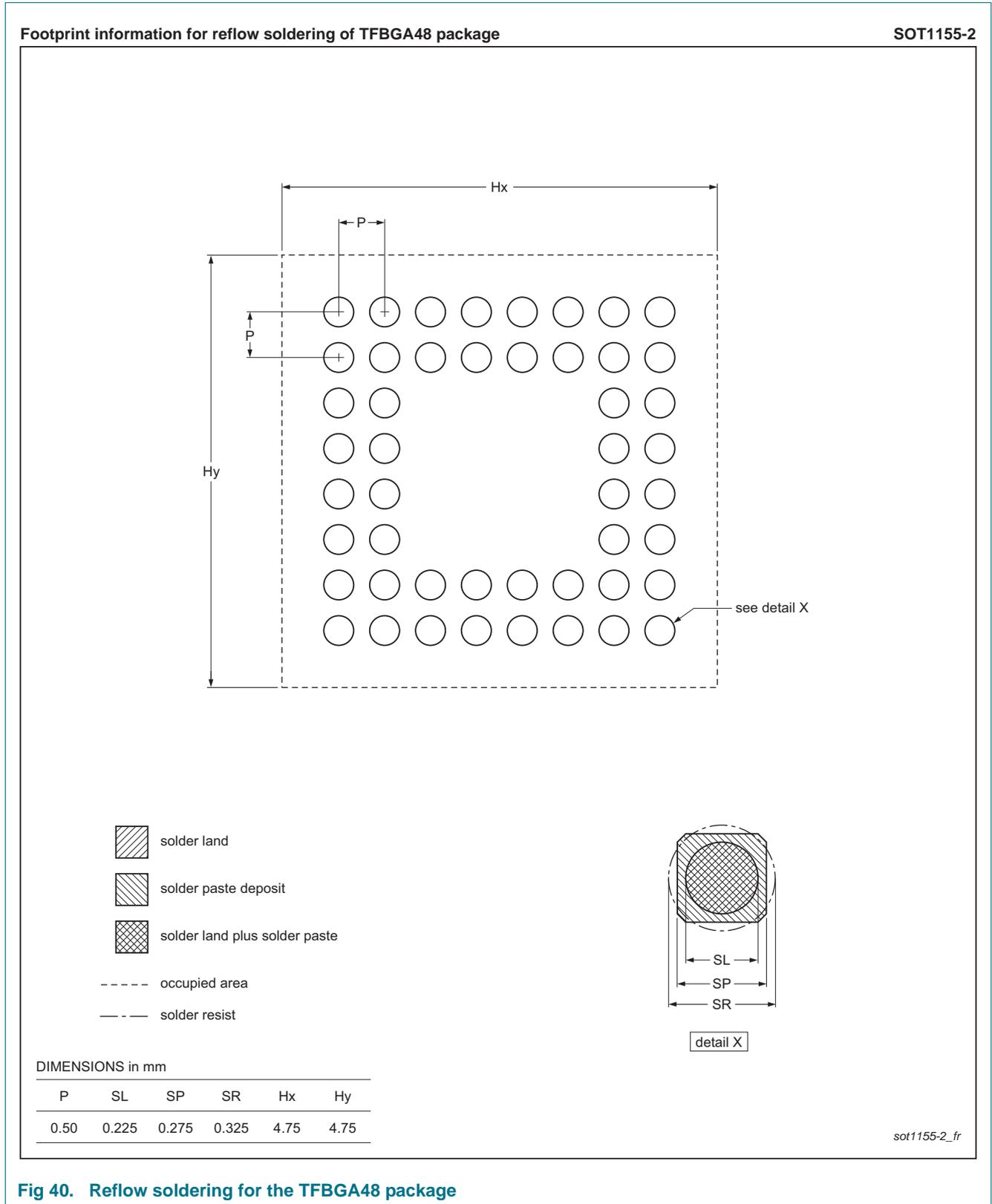
**Fig 40. Reflow soldering for the TFBGA48 package**
