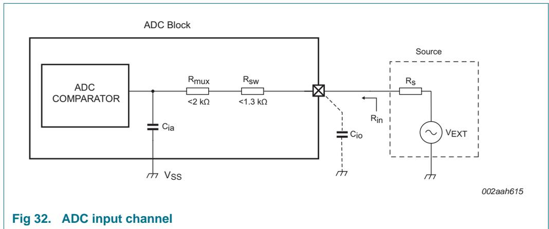
Fig 32. ADC input channel
