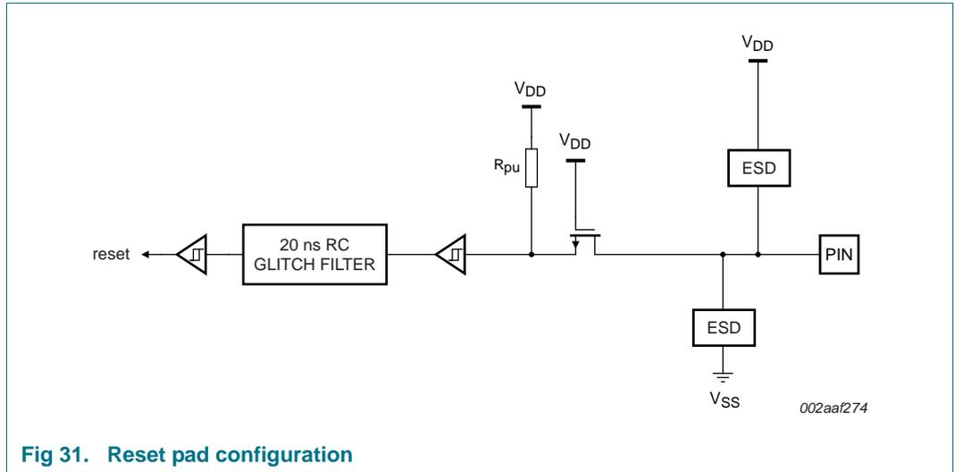
Fig 31. Reset pad configuration
