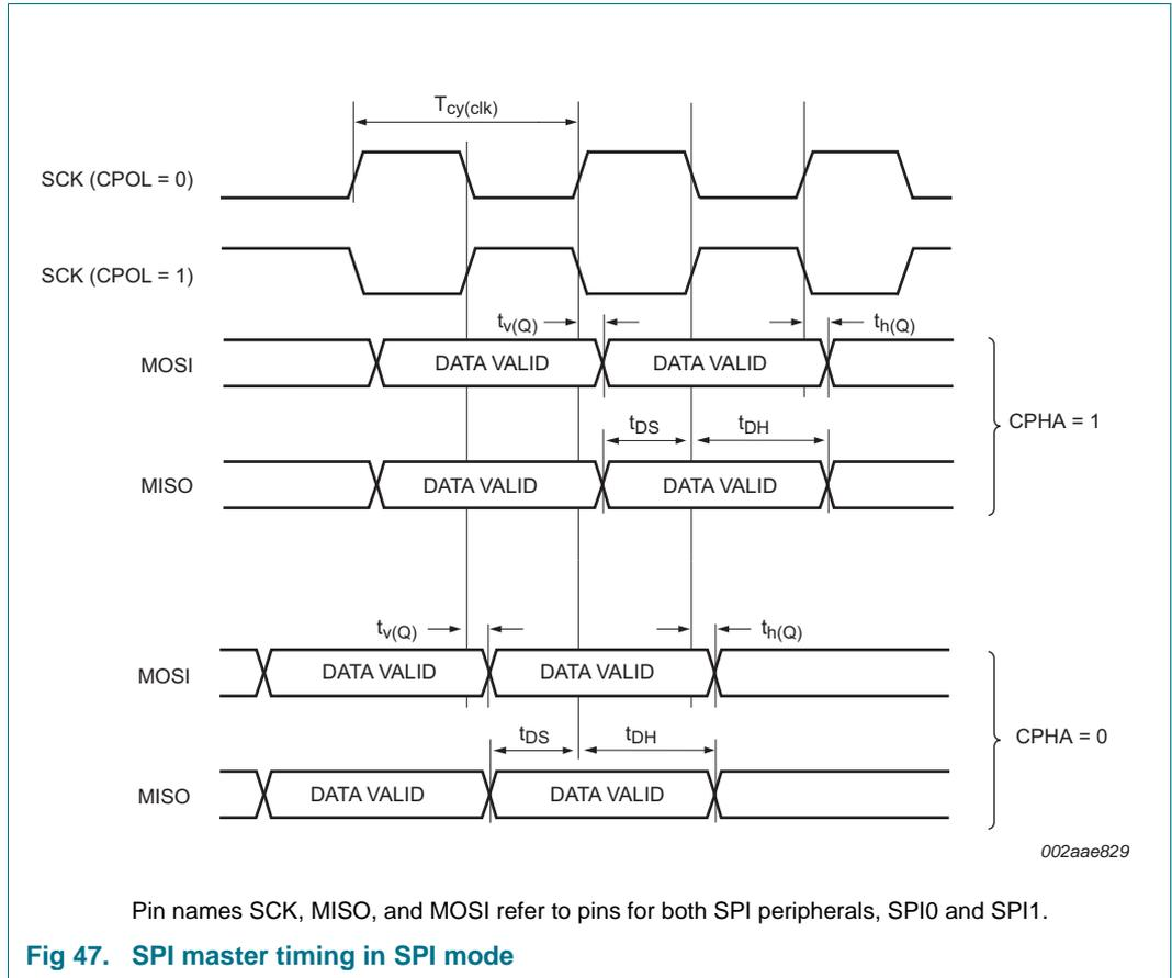
Fig 47. SPI master timing in SPI mode
