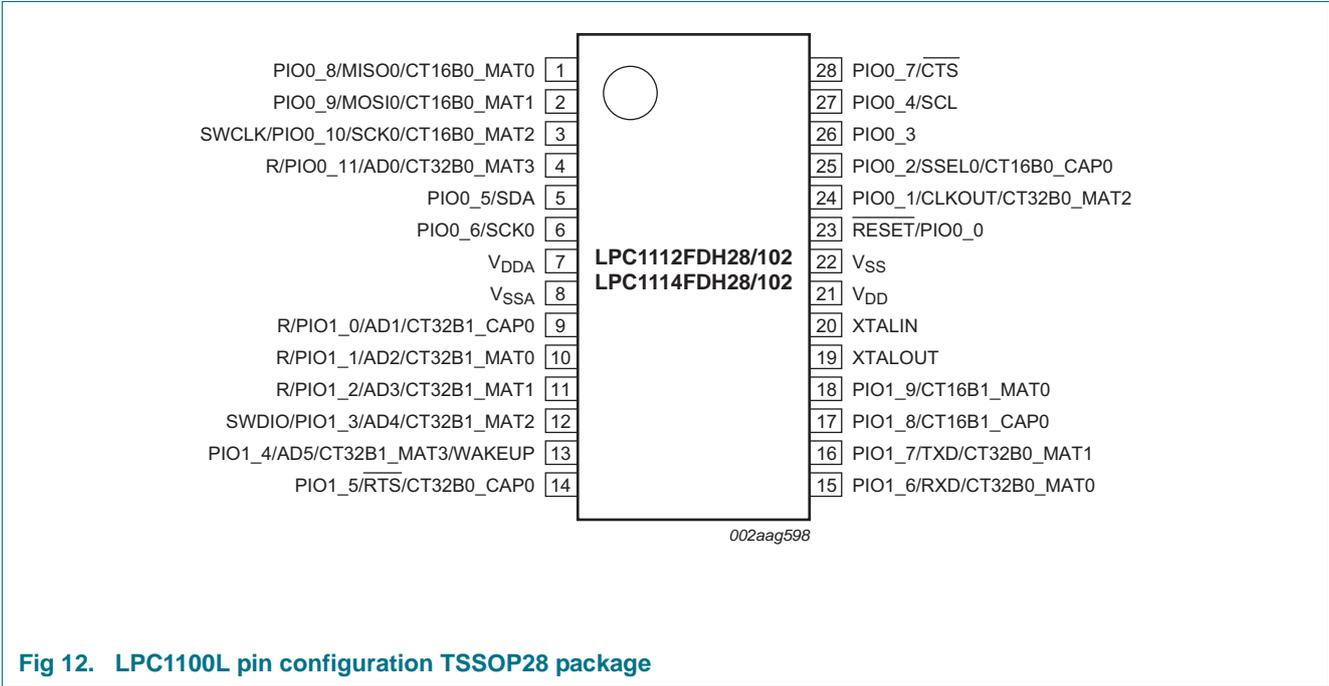
**Fig 12. LPC1100L pin configuration TSSOP28 package**
