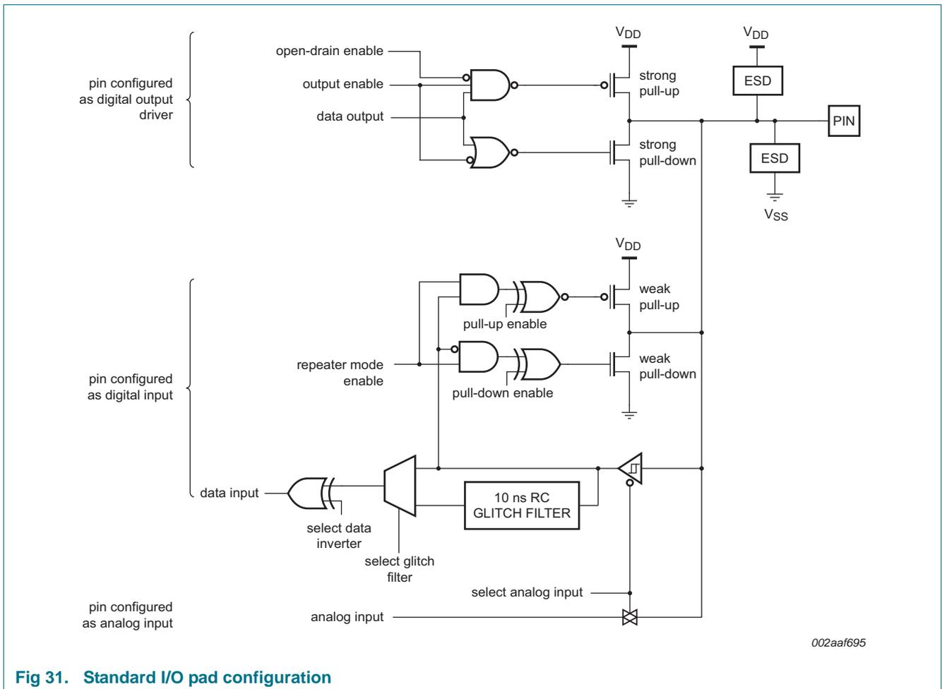
Fig 31. Standard I/O pad configuration
