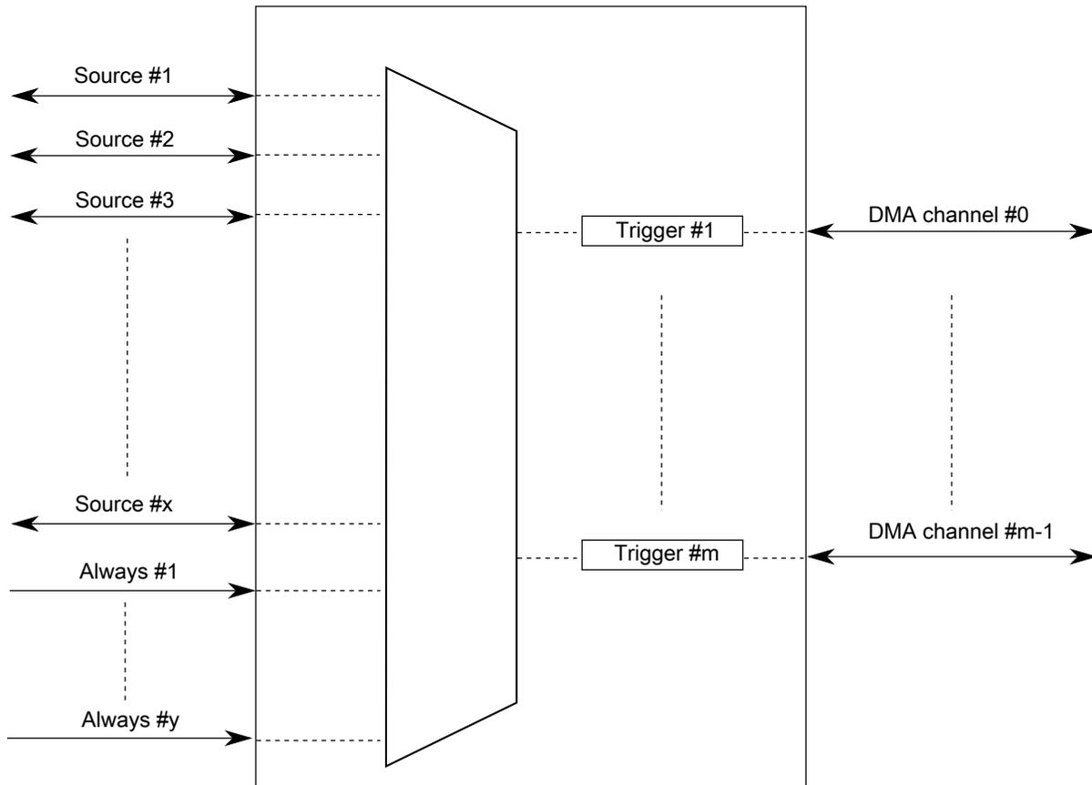
Figure 27-2. DMAMUX triggered channels
