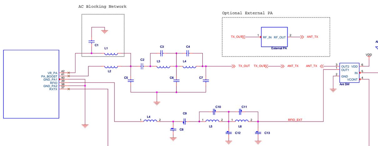
Figure 4-6. Dual Port RF Schematic (+17dBm to 1W)
