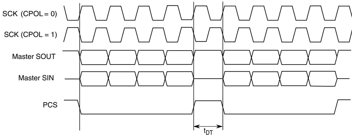
**Figure 51-15. Continuous SCK Timing Diagram (CONT=0)**
