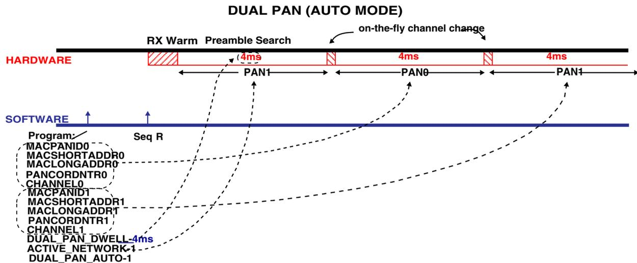
Figure 5-4. MKW2xD Dual PAN Auto mode diagram
