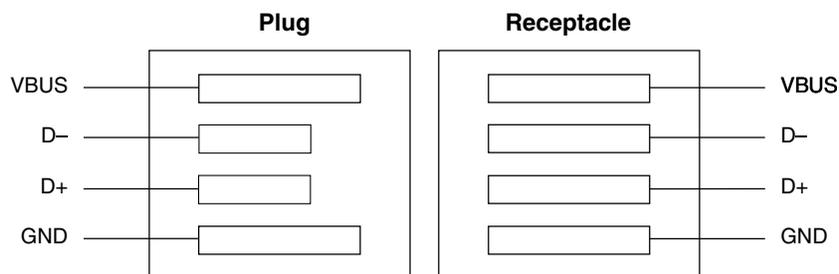
**Figure 49-4. Relative pin positions in USB plugs and receptacles**
