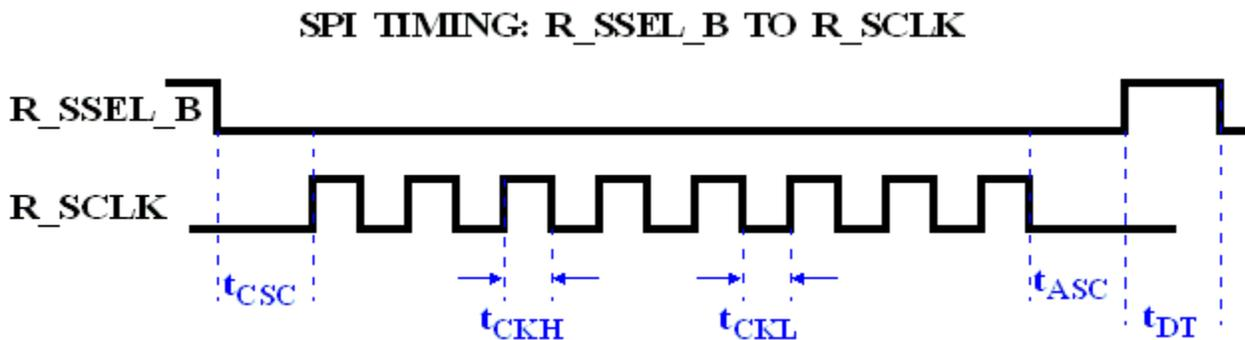
Figure 8-3. SPI Timing of R\_SSEL to R\_SCLK
