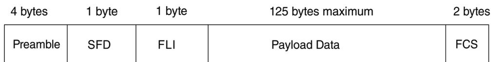
**Figure 2-3. MKW2xD Packet Structure**
