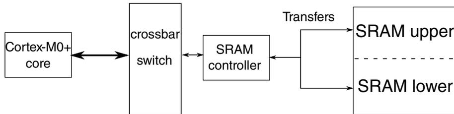
Figure 1-19. SRAM configuration
