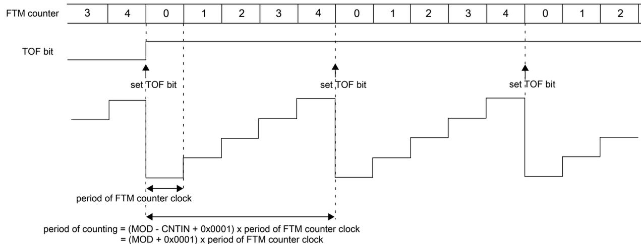
**Figure 43-5. Example of FTM up counting with CNTIN = 0x0000**
