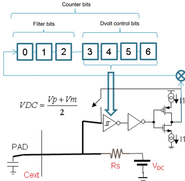
**Figure 35-10. Block diagram automatic noise threshold operation**
