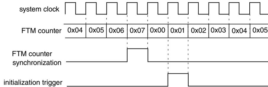
**Figure 43-78. Initialization trigger is generated when there is the FTM counter synchronization**
