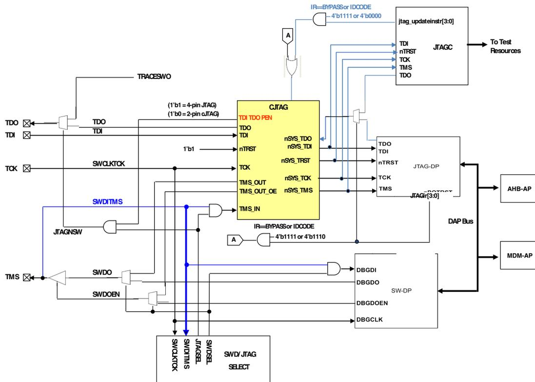
Figure 16-2. Modified Debug Port
