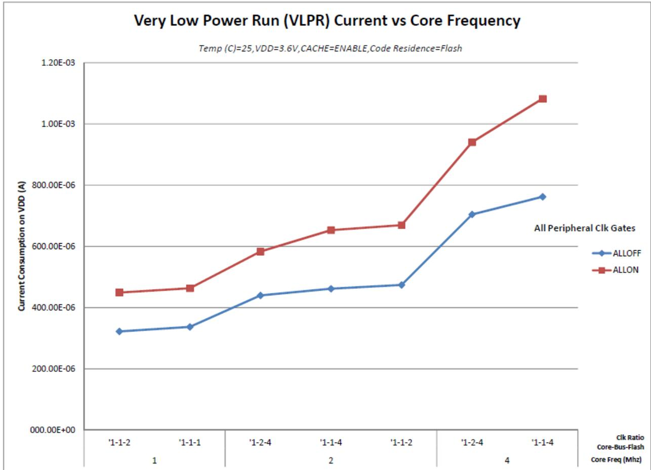
Figure 6. VLPR mode supply current vs. core frequency
