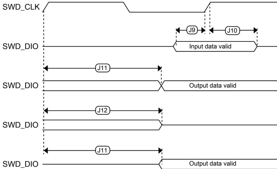
**Figure 4. Serial wire data timing**
