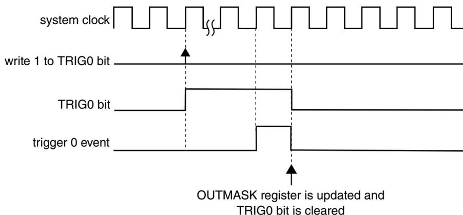
**Figure 43-54. OUTMASK synchronization with (SYNCMODE = 0), (HWTRIGMODE = 0), (SYNCHOM = 1), (PWMSYNC = 1), and a hardware trigger was used**
