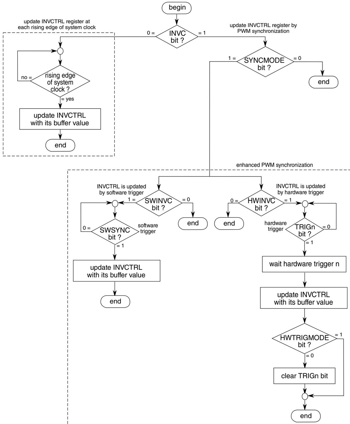
Figure 43-55. INVCTRL register synchronization flowchart
