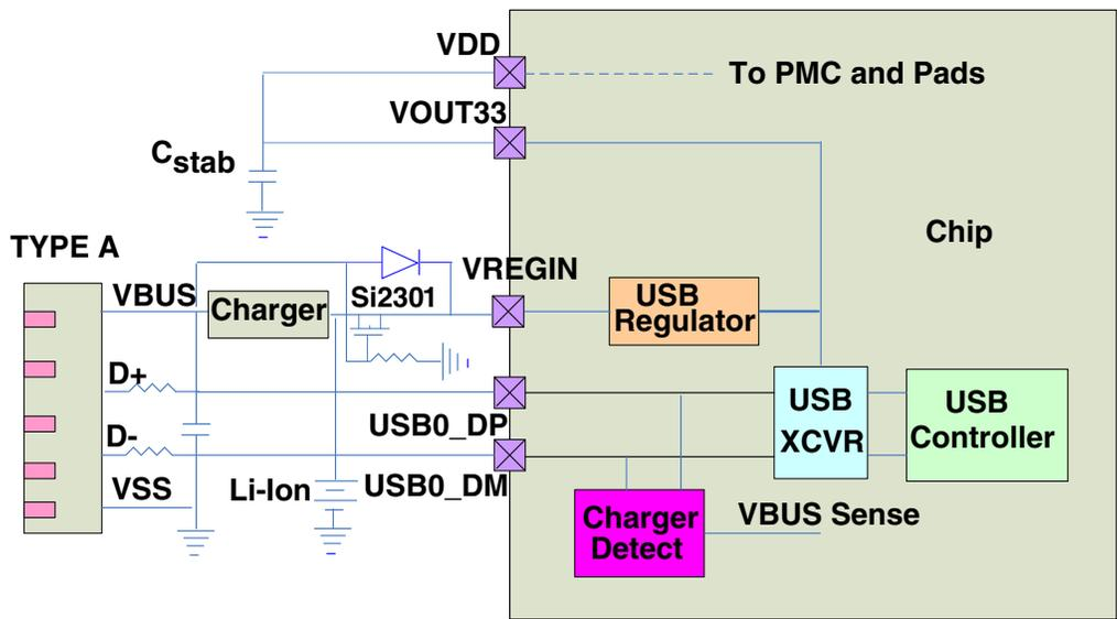
Figure 10-44. USB regulator Li-ion usecase
