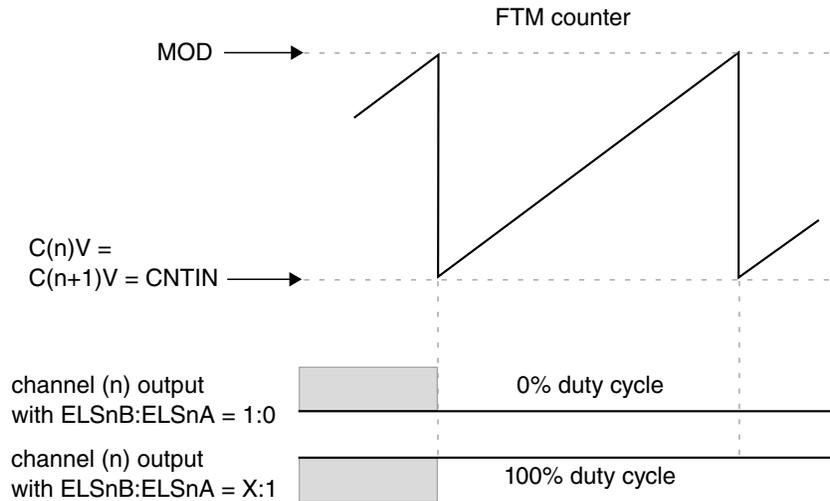
**Figure 43-32. Channel (n) output if  $(C(n)V = C(n+1)V = CNTIN)$**
