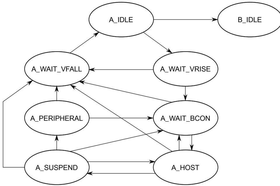
Figure 48-7. Dual role A device flow diagram
