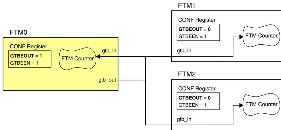
Figure 10-36. FTM Global Time Base Configuration
