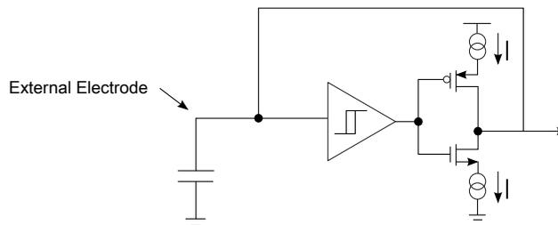
**Figure 35-2. TSI electrode oscillator circuit**
