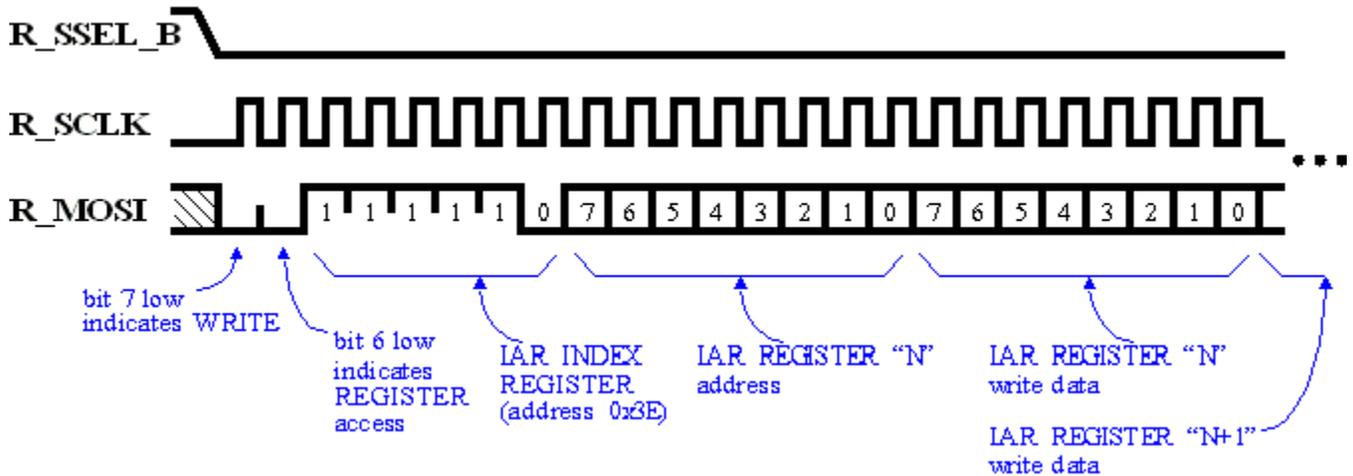
Figure 8-9. Multi-Byte Write Access to an Indirect Register Space
