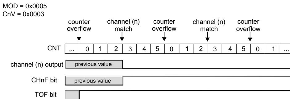
**Figure 27-7. Example of the output compare mode when the match clears the channel output**
