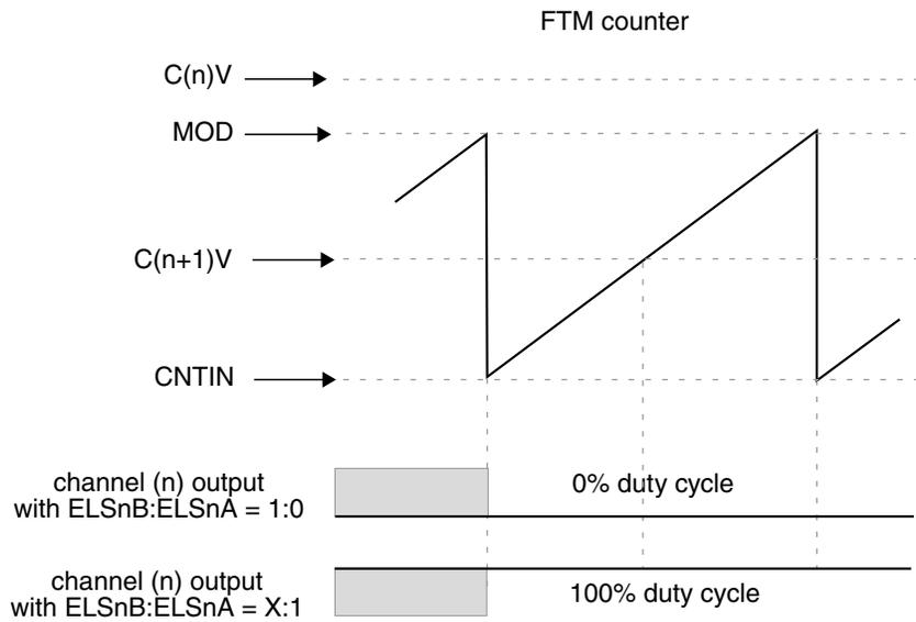
**Figure 43-37. Channel (n) output if  $(C(n)V > MOD)$  and  $(CNTIN < C(n+1)V < MOD)$**
