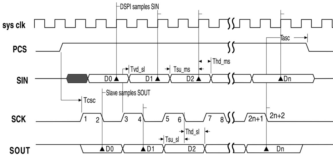
Figure 51-10. DSPI Modified Transfer Format (MTFE=1, CPHA=1,  $f_{sck} = f_{sys}/2$ )
