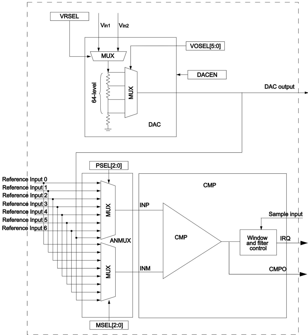
Figure 25-1. CMP, DAC and ANMUX block diagram
