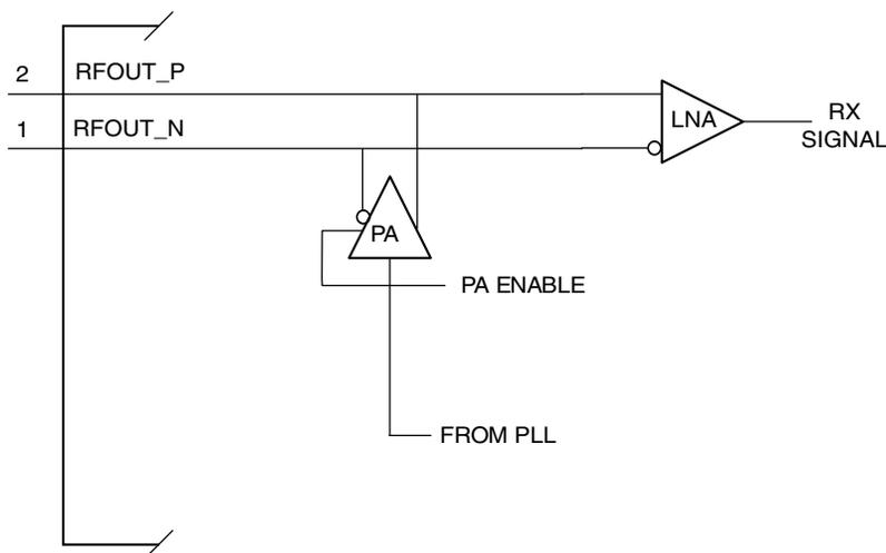
Figure 4-5. RF Interface Pins
