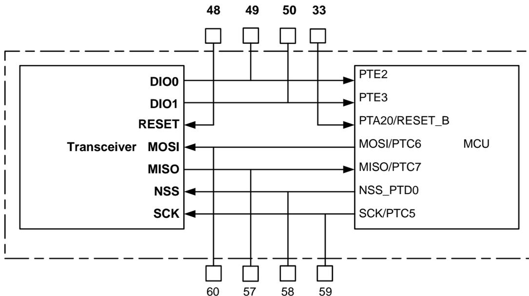
**Figure 8-1. MKW01 Internal Interconnects Highlighting SPI Bus**
