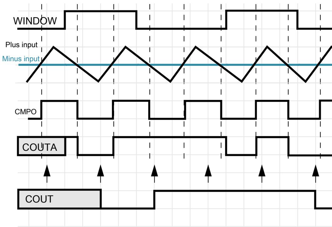
Figure 41-10. Windowed/resampled mode operation
