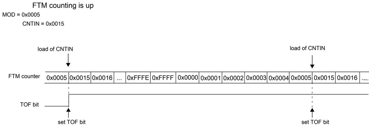
**Figure 43-6. Example of up counting when the value of CNTIN is greater than the value of MOD**
