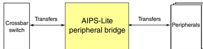
**Figure 10-11. Peripheral bridge configuration**
