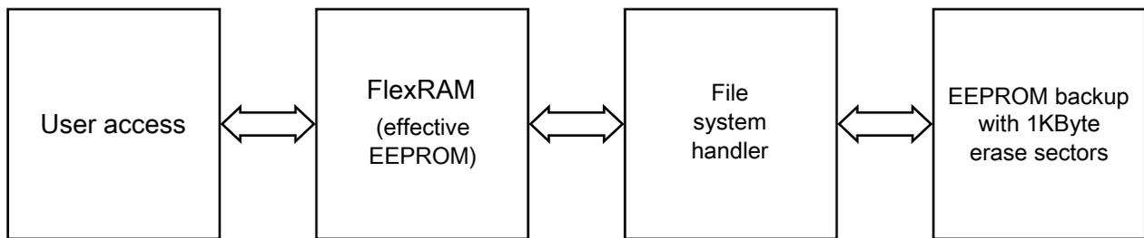
**Figure 35-6. Top Level EEPROM Architecture**
