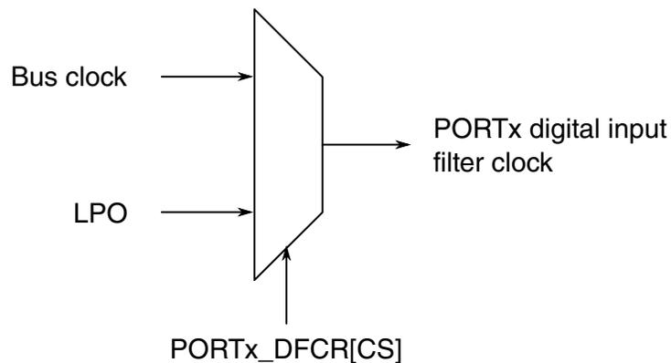
**Figure 12-4. PORT<sub>x</sub> digital input filter clock generation**
