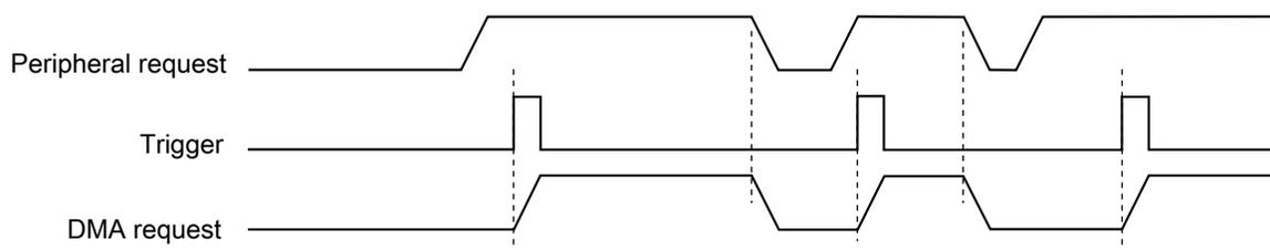
**Figure 27-3. DMAMUX channel triggering: normal operation**
