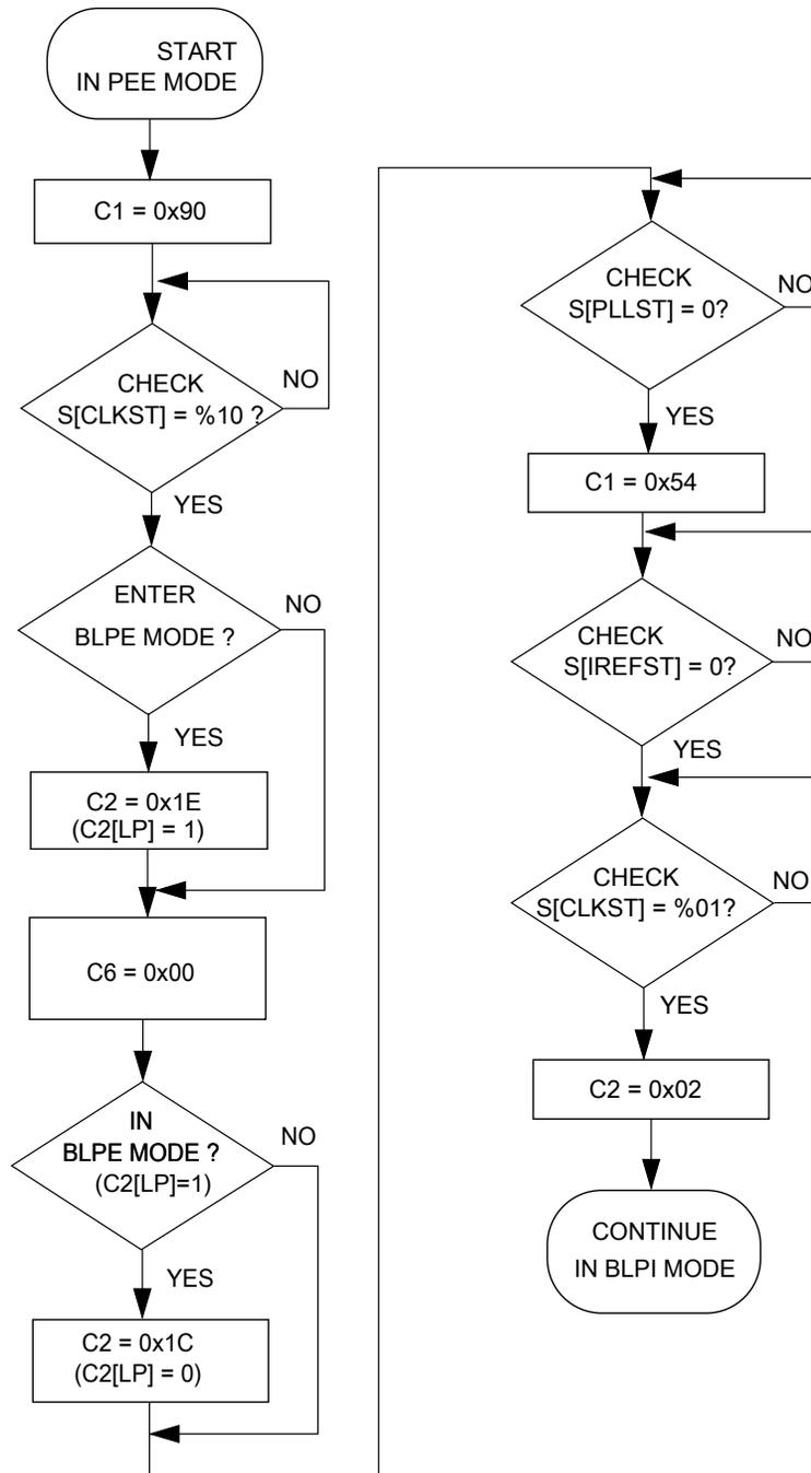
Figure 31-4. Flowchart of PEE to BLPI mode transition using an 4 MHz crystal
