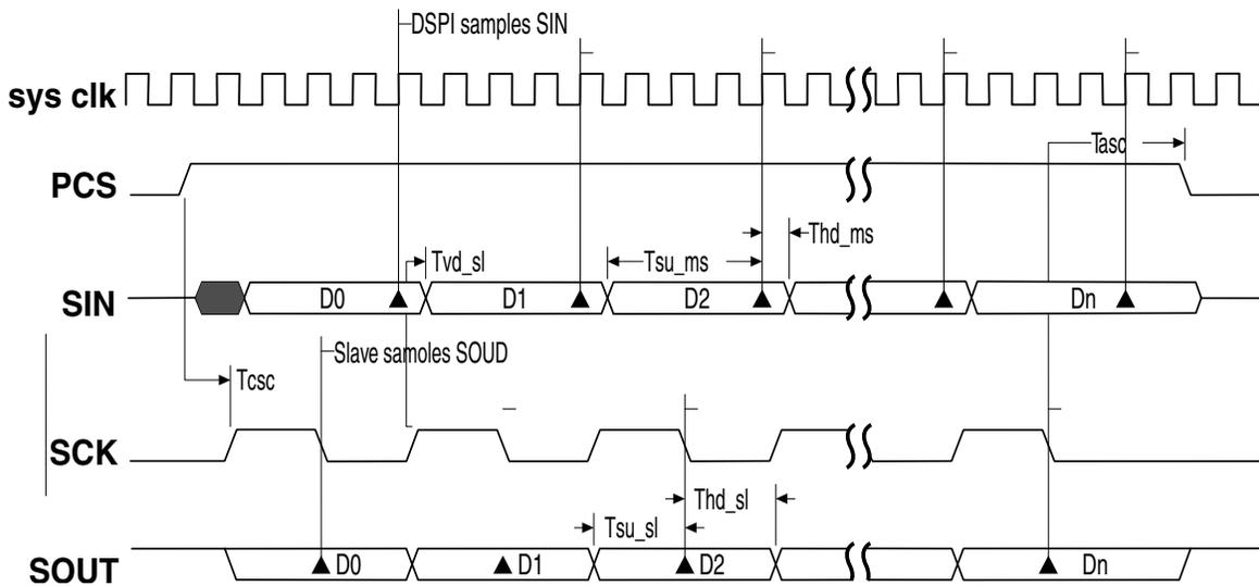
Figure 51-12. DSPI Modified Transfer Format (MTFE=1, CPHA=1,  $f_{sck} = f_{sys}/4$ )
