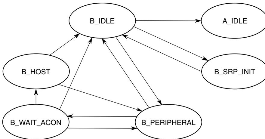
**Figure 48-8. Dual role B device flow diagram**
