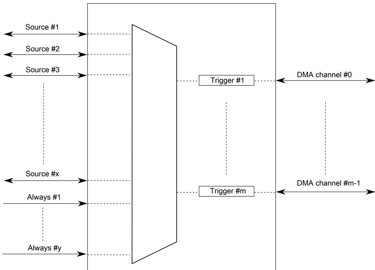
**Figure 18-2. DMAMUX triggered channels**
