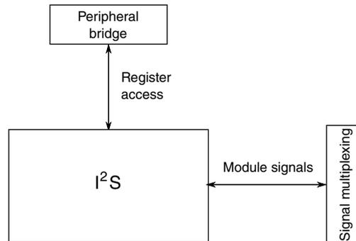
Figure 10-52. I<sup>2</sup>S configuration
