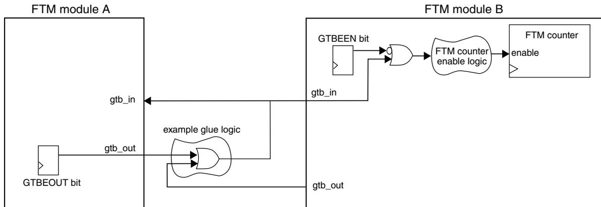
**Figure 43-95. Global time base (GTB) block diagram**
