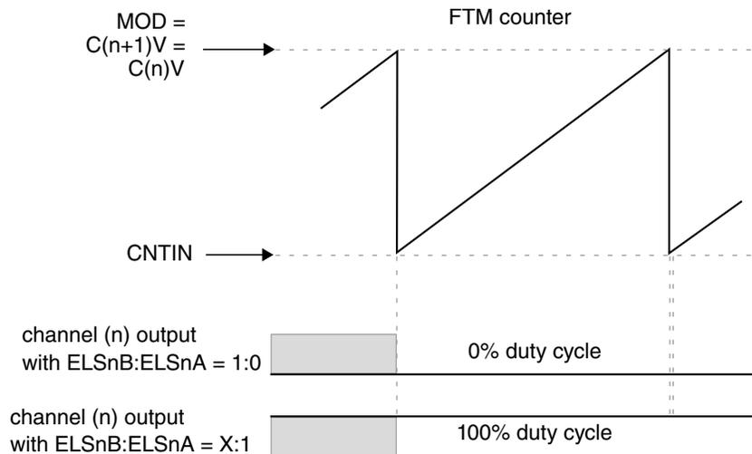
**Figure 43-33. Channel (n) output if  $(C(n)V = C(n+1)V = MOD)$**
