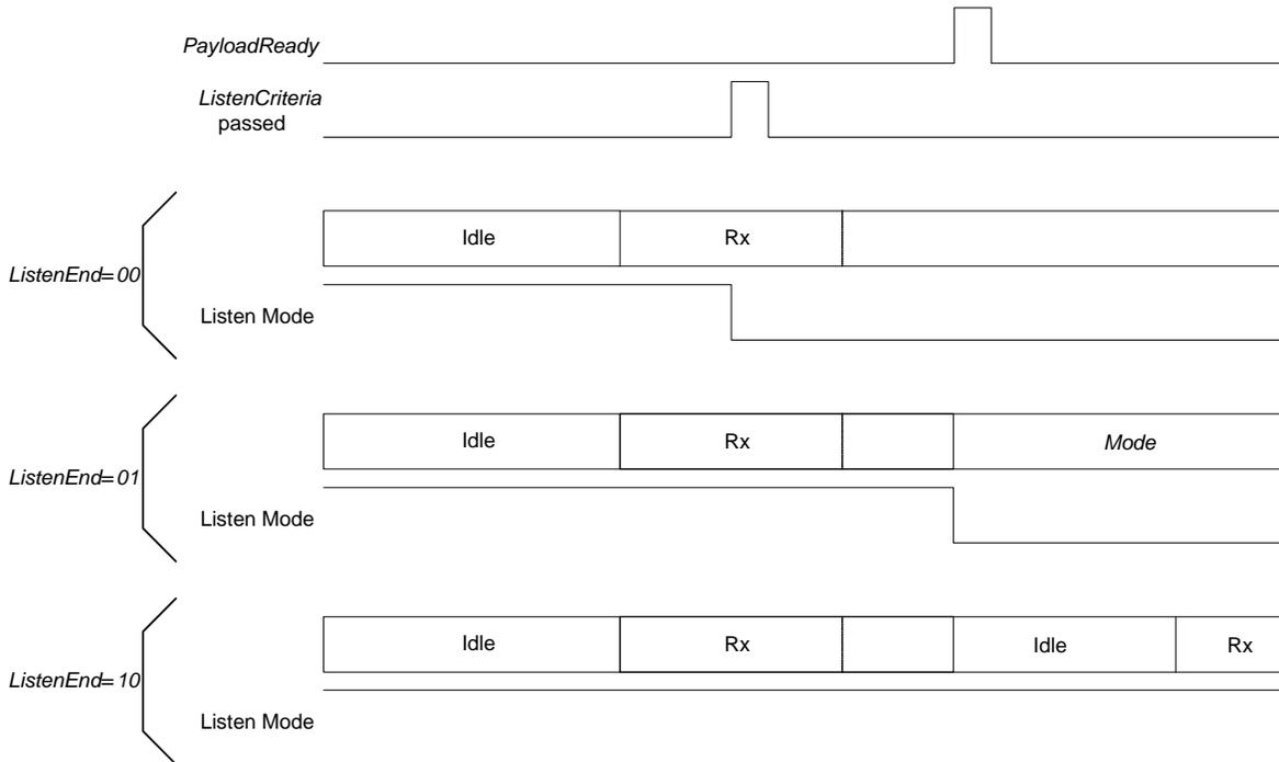
**Figure 6-6. Listen Mode Sequence (wanted signal is received)**
