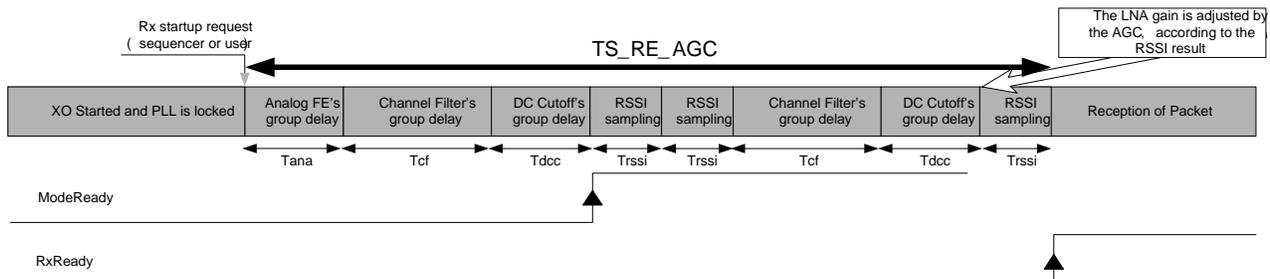
Figure 6-3. RX Startup - AGC, no AFC
