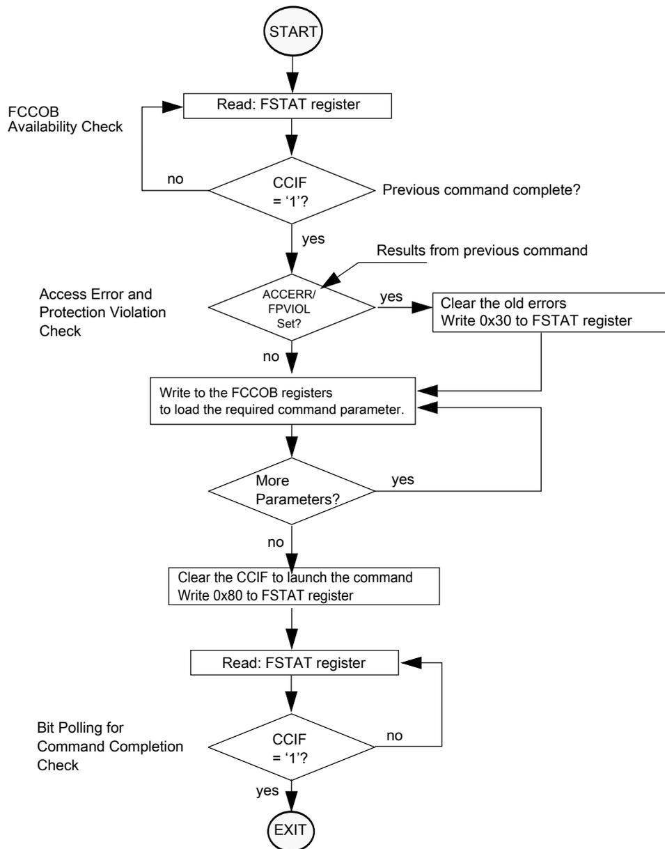
**Figure 35-9. Generic flash command write sequence flowchart**
