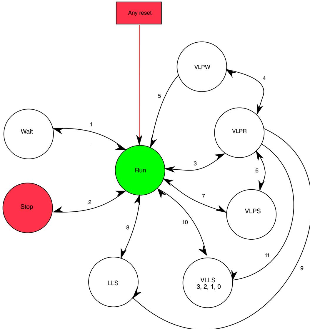
Figure 14-1. Power mode state transition diagram
