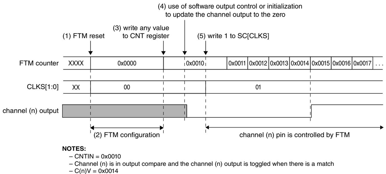
Figure 43-97. FTM behavior after reset when the channel (n) is in Output Compare mode
