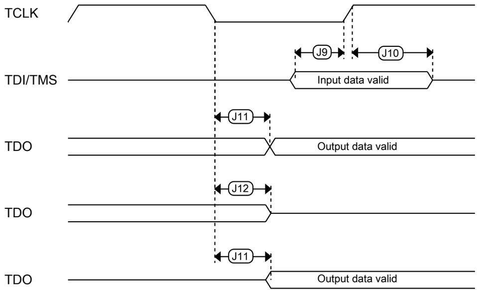
Figure 9. Test Access Port timing
