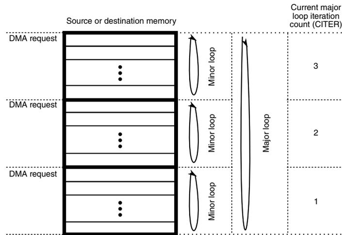
Figure 28-5. Example of multiple loop iterations
