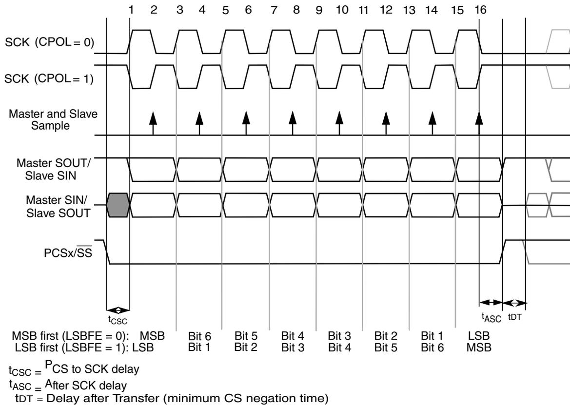
**Figure 51-6. Module transfer timing diagram (MTFE=0, CPHA=1, FMSZ=8)**
