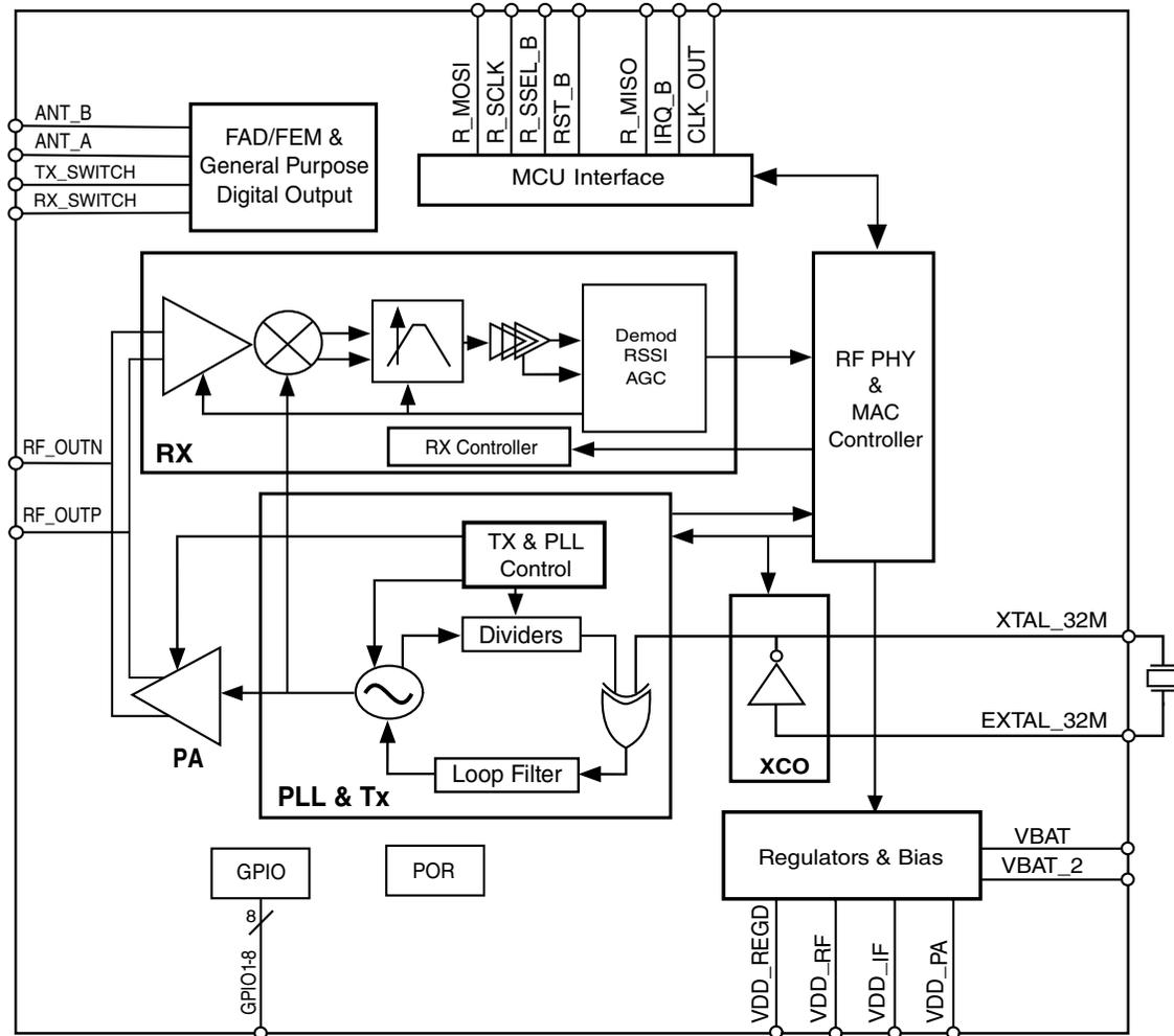
**Figure 2-2. Modem Simplified Block Diagram**
