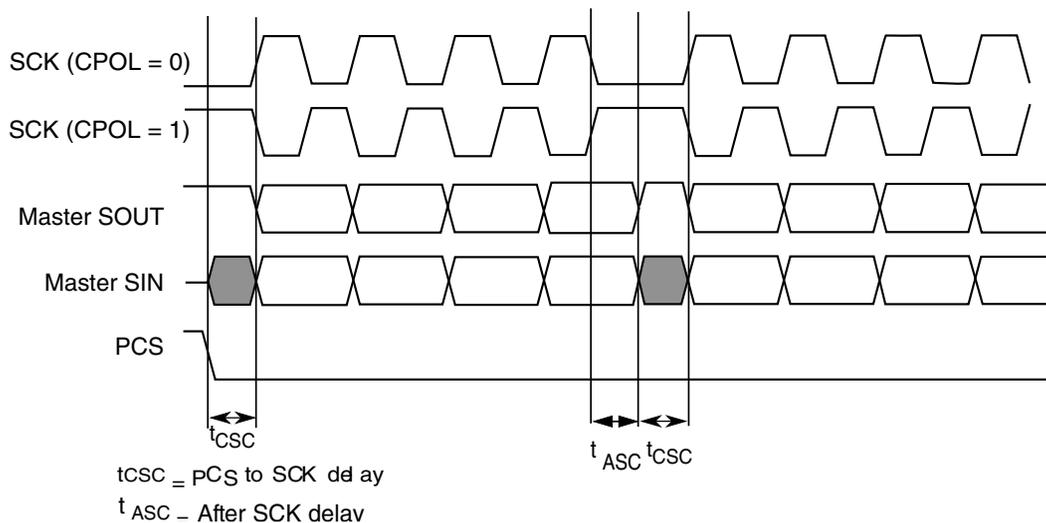
**Figure 51-14. Example of continuous transfer (CPHA=1, CONT=1)**
