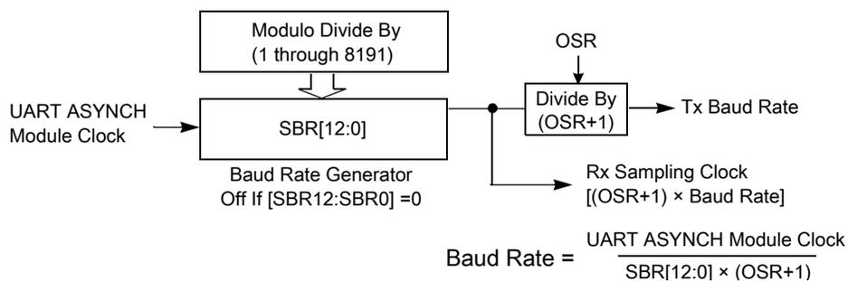
**Figure 32-3. UART baud rate generation**
