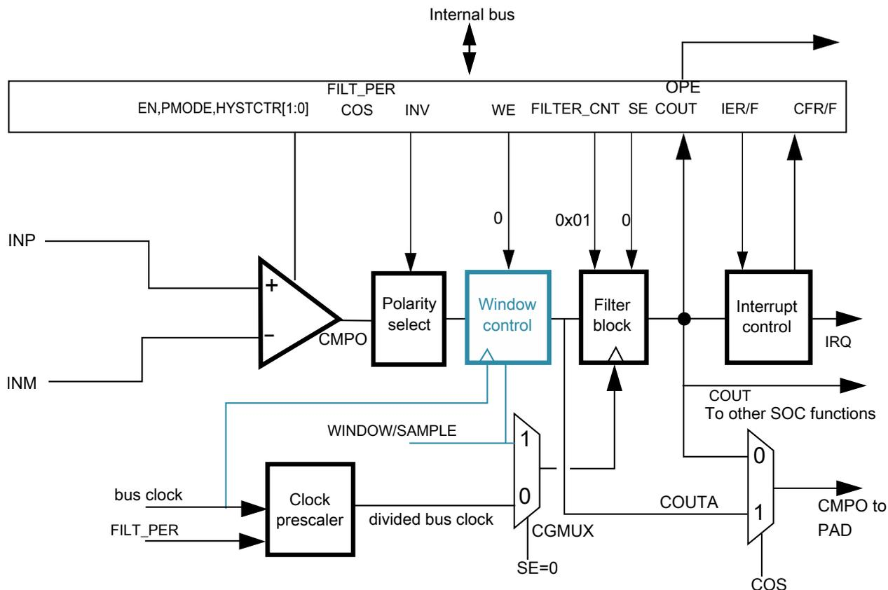
**Figure 41-5. Sampled, Non-Filtered (# 3B): sampling interval internally derived**
