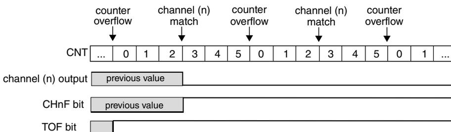
**Figure 43-16. Example of the Output Compare mode when the match clears the channel output**
