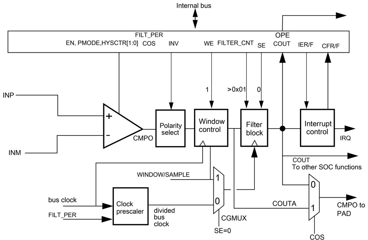
Figure 41-11. Windowed/Filtered mode
