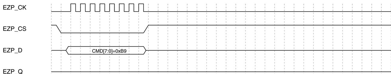
**Figure 36-10. Reset Chip command sequence**
