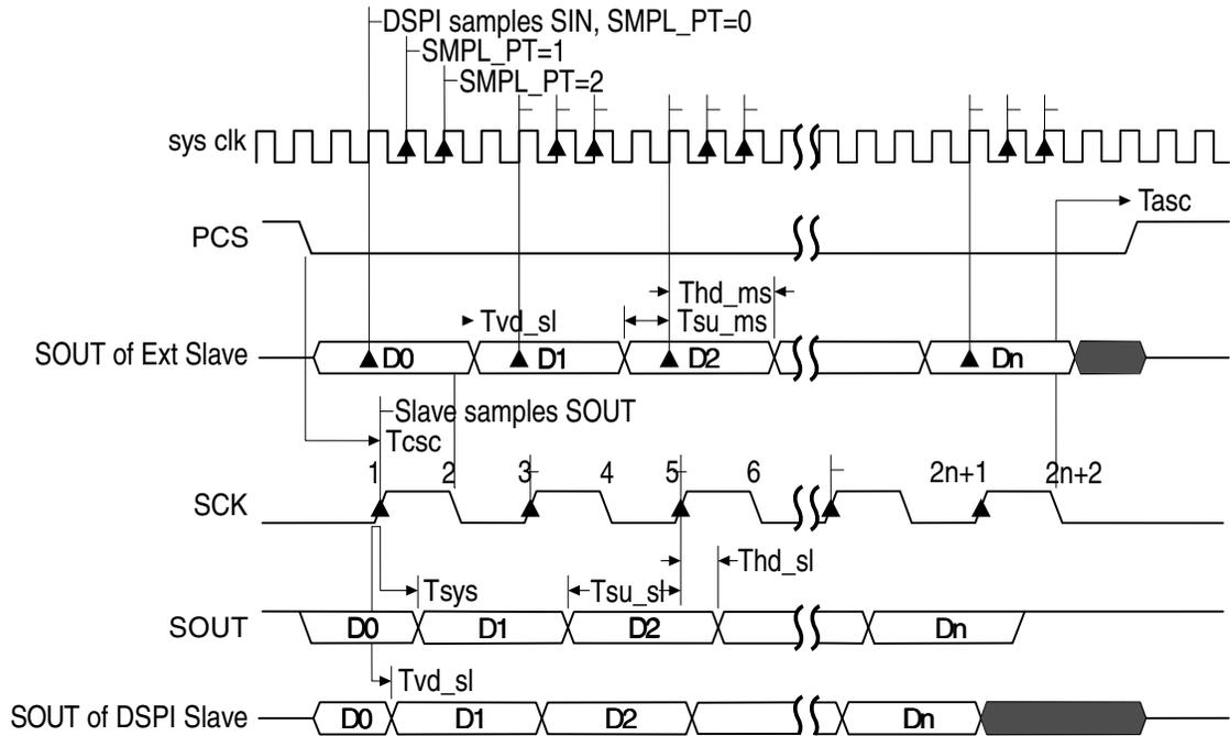
**Figure 51-7. DSPI Modified Transfer Format (MTFE=1, CPHA=0,  $f_{sck} = f_{sys}/4$ )**
