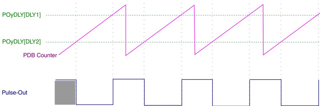
Figure 42-3. How Pulse Out is generated
