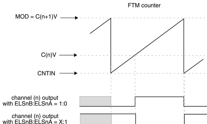
**Figure 43-26. Channel (n) output if  $(CNTIN < C(n)V < MOD)$  and  $(C(n+1)V = MOD)$**
