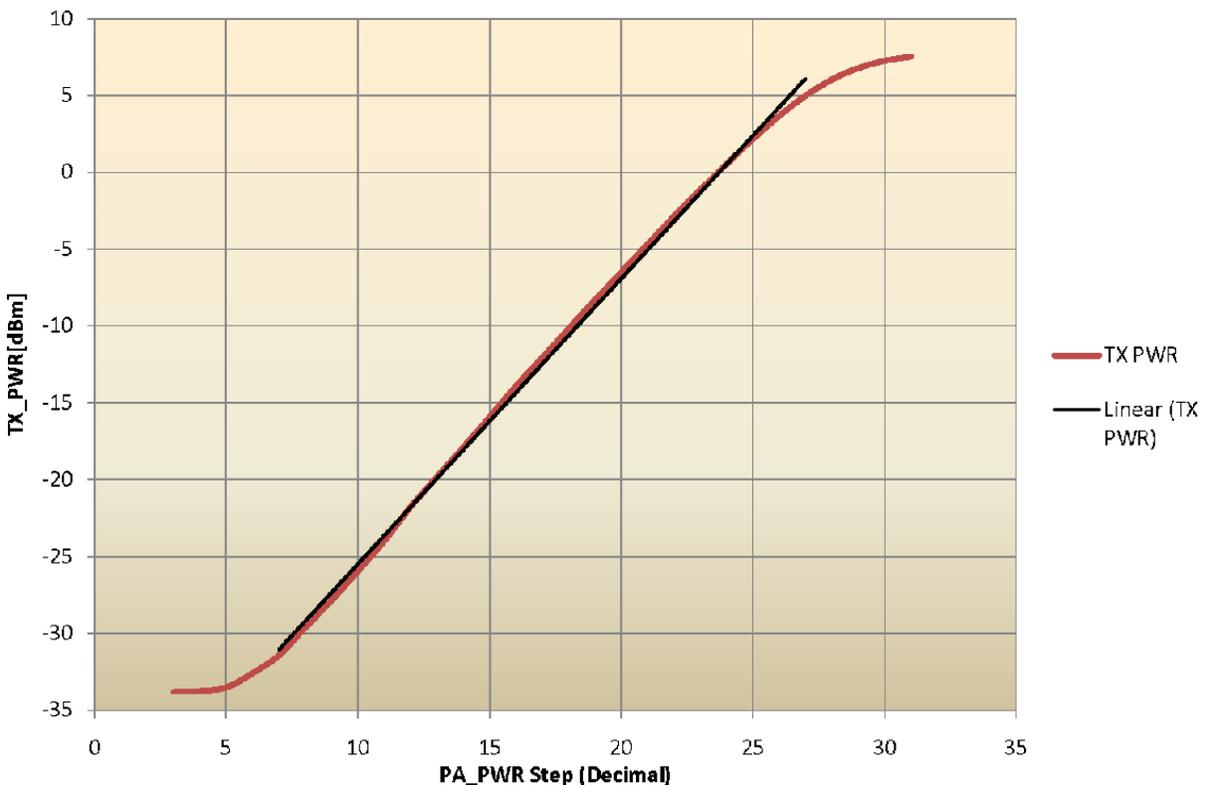
Figure 4-11. MKW2xD TX power vs. PA\_PWR step
