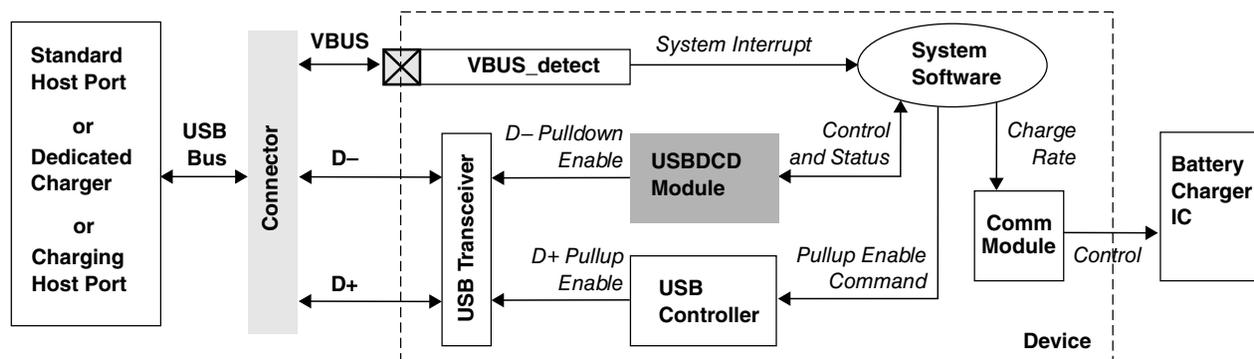
Figure 49-2. USB battery charging subsystem
