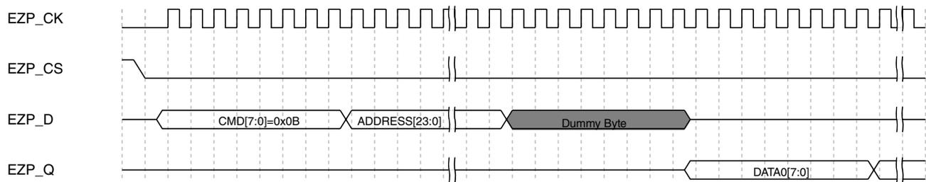
**Figure 36-6. Read Data at High Speed command sequence**
