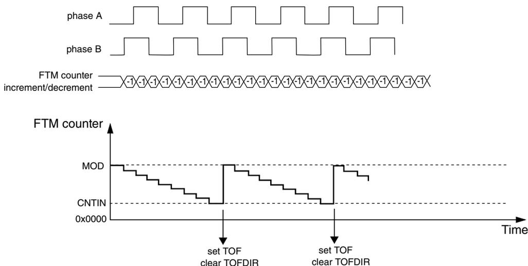
**Figure 43-91. FTM counter overflow in down counting for Quadrature Decoder mode**
