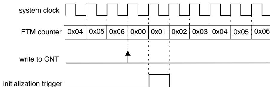
**Figure 43-77. Initialization trigger is generated when there is a write to CNT register**
