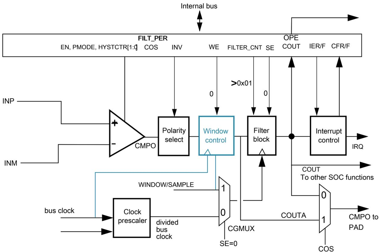
**Figure 41-7. Sampled, Filtered (# 4B): sampling point internally derived**
