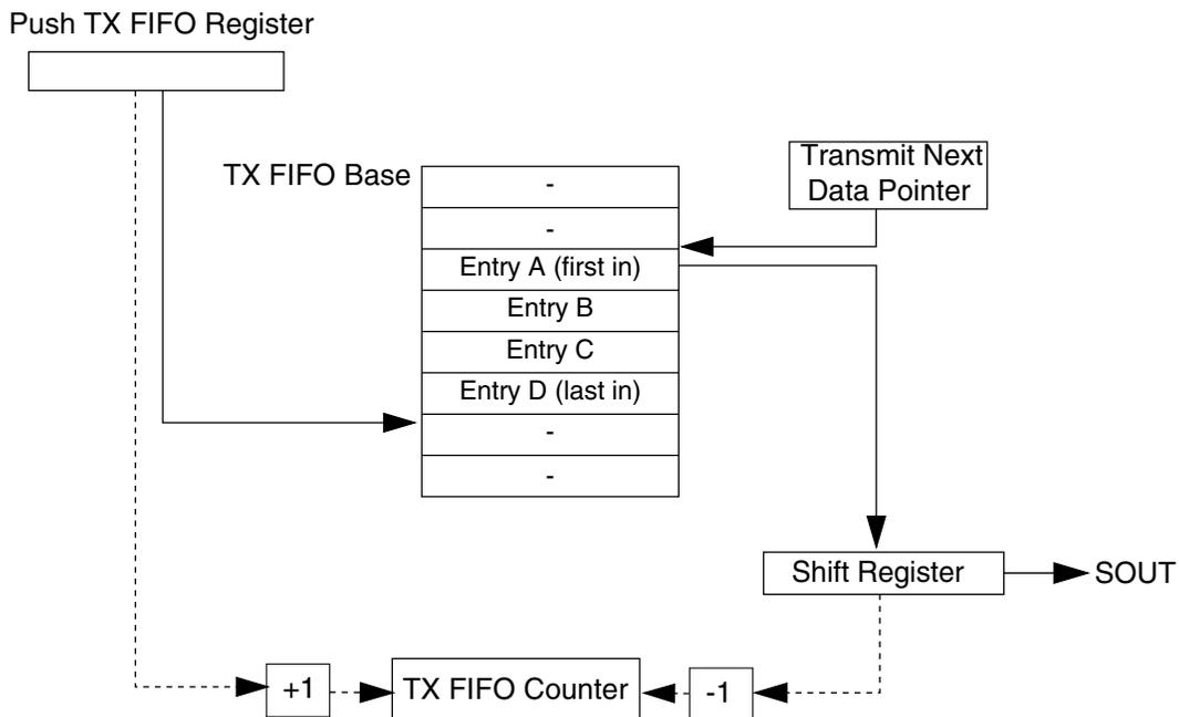
Figure 51-17. TX FIFO pointers and counter
