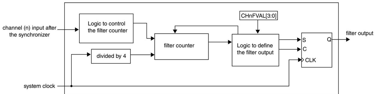
**Figure 43-12. Channel input filter**
