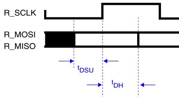
**Figure 26. SPI timing: R\_SCLK to R\_MOSI and R\_MISO**
