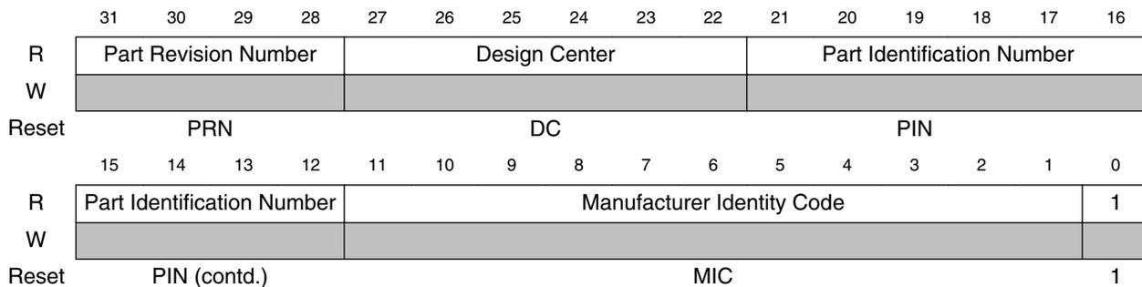
The following table describes the device identification register functions.
