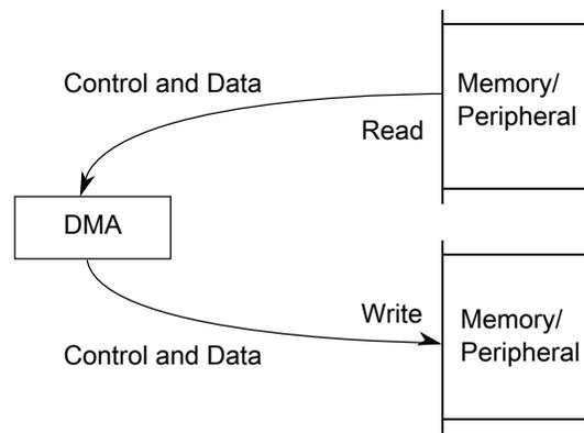
**Figure 19-2. Dual-Address Transfer**
