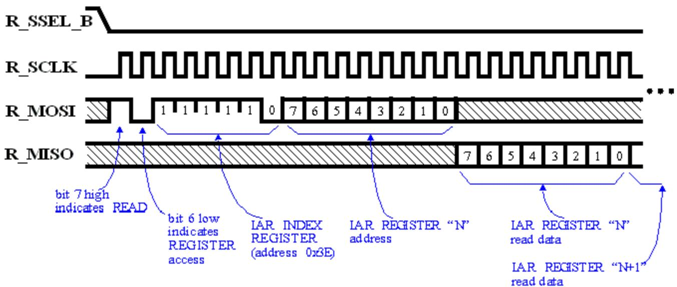
Figure 8-10. Multi-Byte Read Access to an Indirect Register Space
