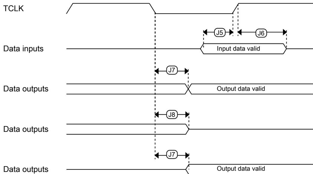
**Figure 8. Boundary scan (JTAG) timing**
