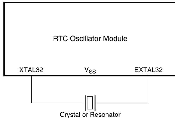
**Figure 33-2. Crystal Connections**
