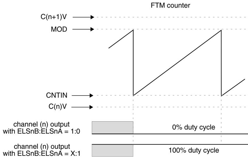
**Figure 43-30. Channel (n) output if  $C(n)V$  and  $C(n+1)V$  are not between  $CNTIN$  and  $MOD$**
