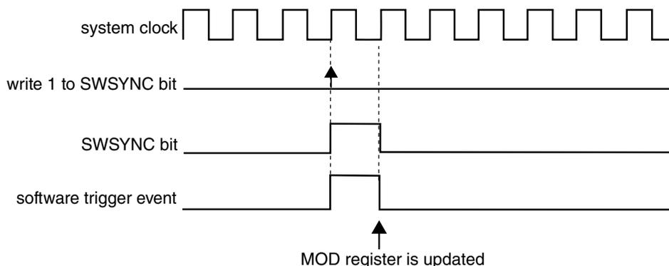
**Figure 43-48. MOD synchronization with (SYNCMODE = 0), (PWMSYNC = 0), (REINIT = 1), and software trigger was used**
