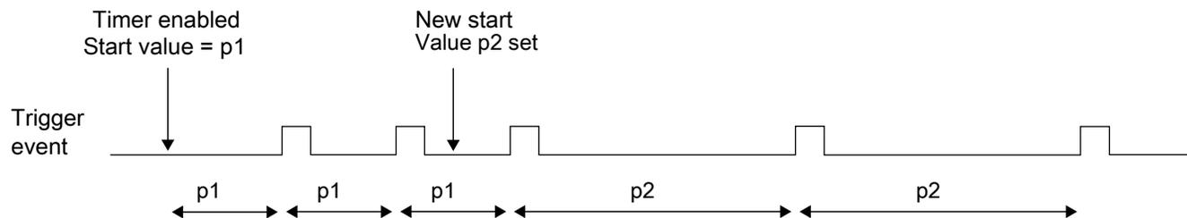
**Figure 44-4. Dynamically setting a new load value**
