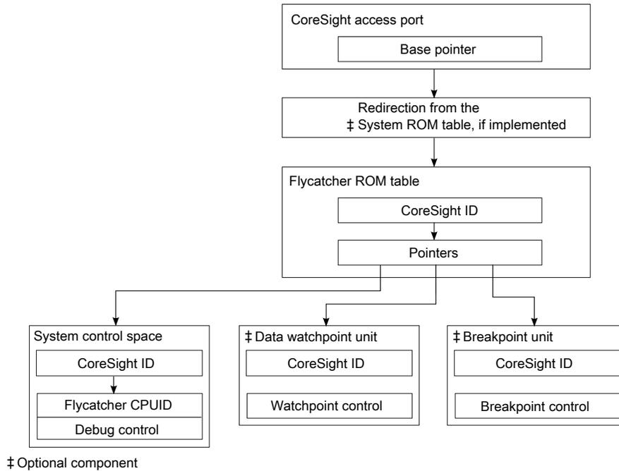
**Figure 15-3. CoreSight discovery process**
