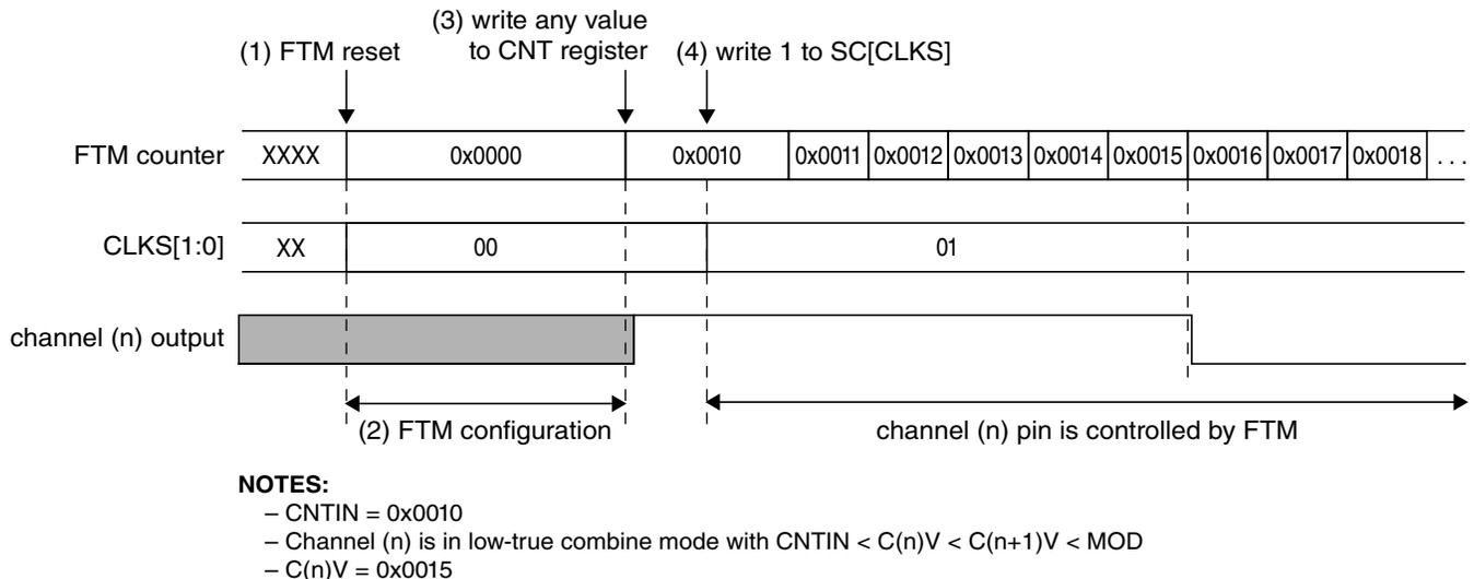
**Figure 43-96. FTM behavior after reset when the channel (n) is in Combine mode**
