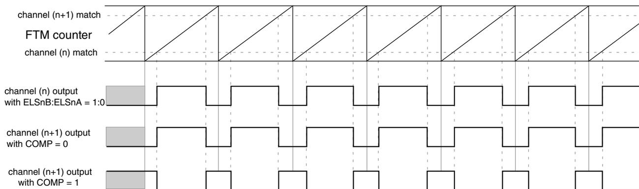
**Figure 43-40. Channel (n+1) output in Complementary mode with (ELSnB:ELSnA = 1:0)**
