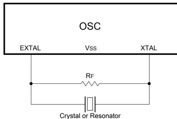
**Figure 32-3. Crystal/Ceramic Resonator Connections - Connection 2****NOTE**
