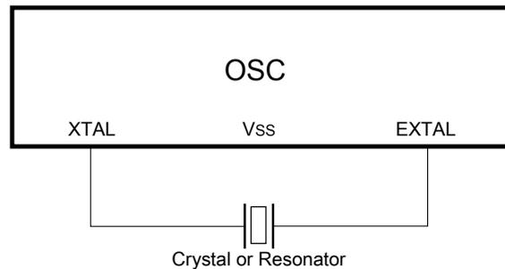
**Figure 32-2. Crystal/Ceramic Resonator Connections - Connection 1**
