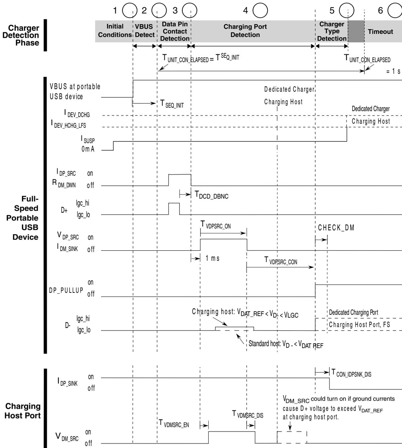
**Figure 49-3. Full speed charger detection timing**
