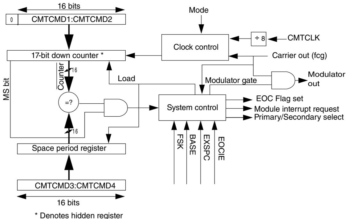
**Figure 46-4. Modulator block diagram**
