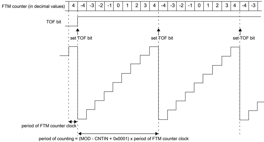
**Figure 43-4. Example of FTM up and signed counting**
