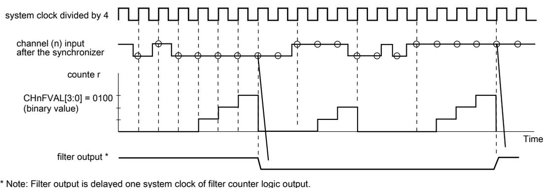
**Figure 43-13. Channel input filter example**
