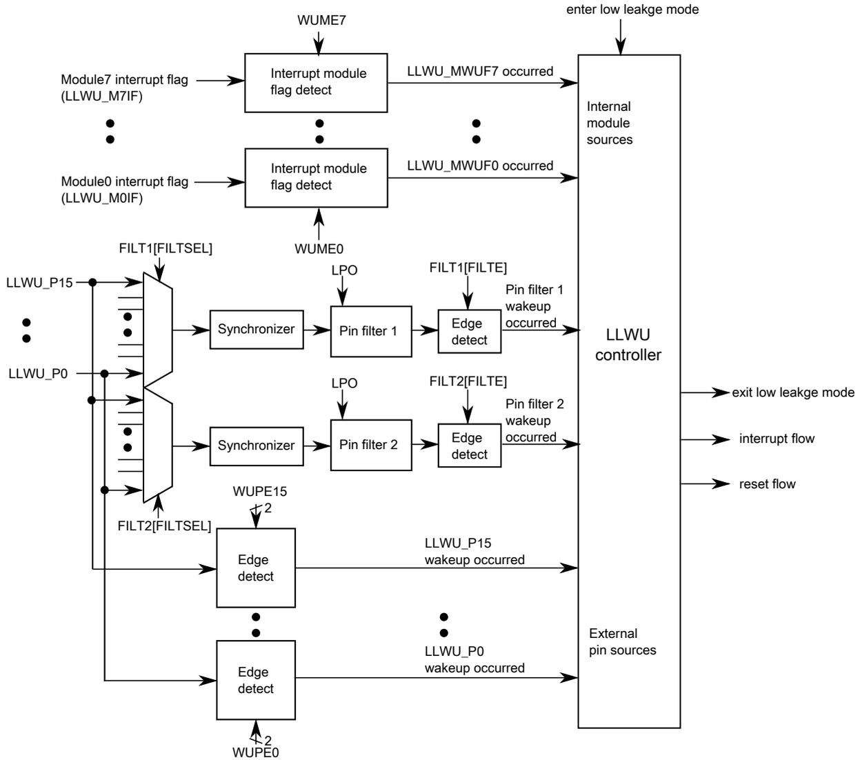
Figure 11-1. LLWU block diagram
