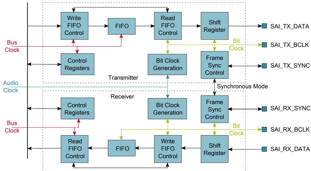
Figure 54-1. I<sup>2</sup>S/SAI block diagram
