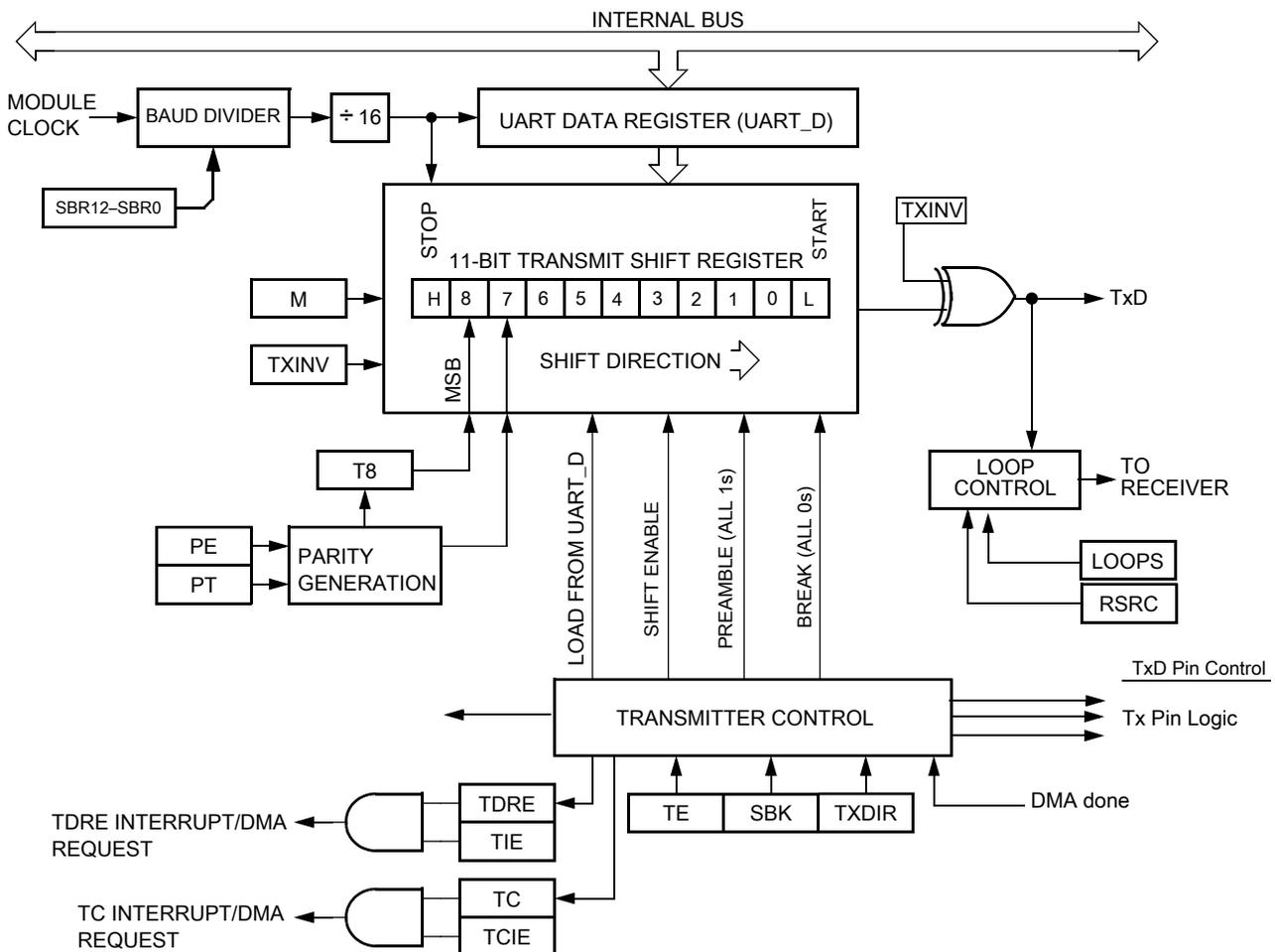
**Figure 33-1. UART transmitter block diagram**
