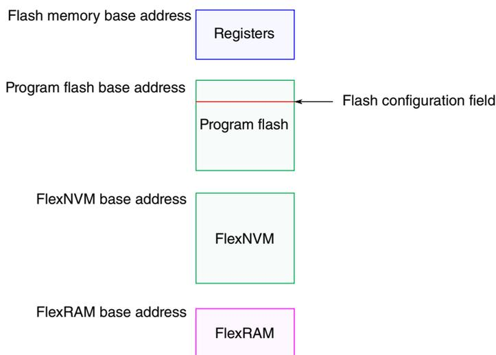
**Figure 10-21. Flash memory map for devices containing FlexNVM**
