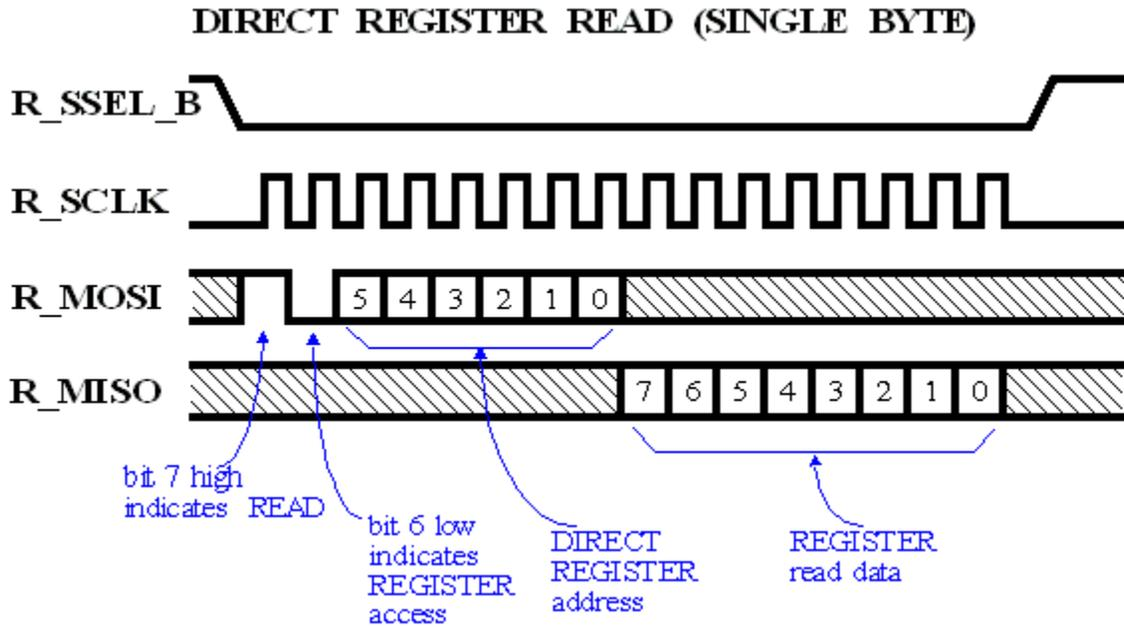
Figure 8-6. Single-Byte read Access to a Direct Register
