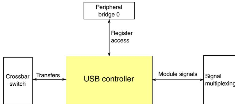
**Figure 10-46. USB controller configuration**
