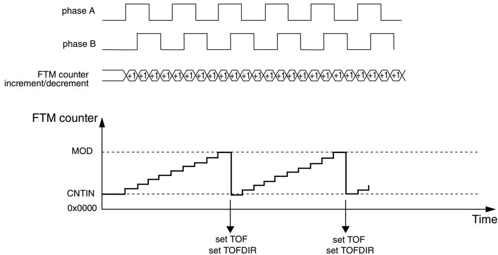
**Figure 43-90. FTM Counter overflow in up counting for Quadrature Decoder mode**
