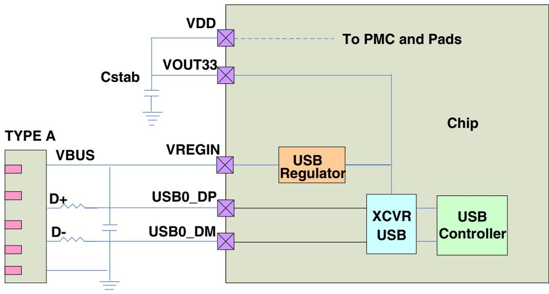
Figure 10-45. USB regulator bus supply
