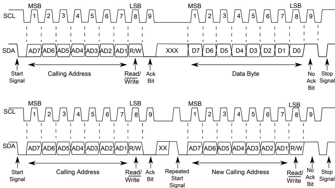
Figure 52-2. I2C bus transmission signals
