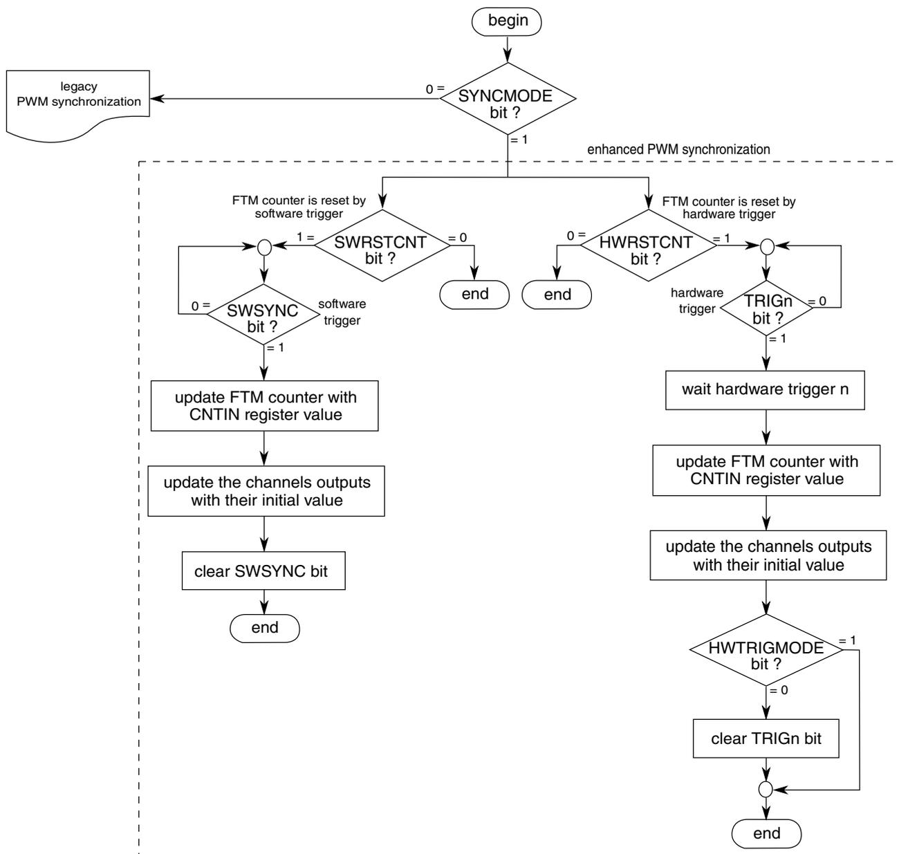
Figure 43-58. FTM counter synchronization flowchart
