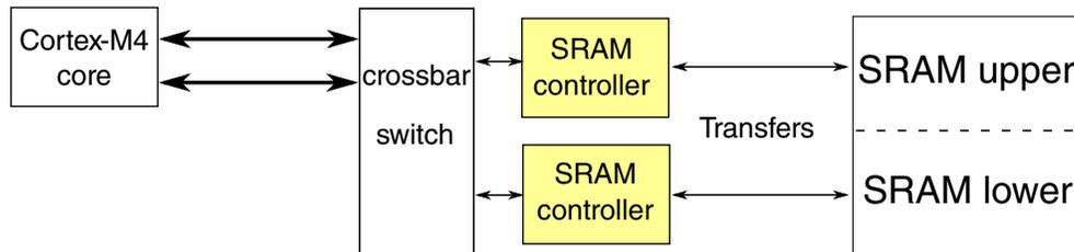
Figure 10-23. SRAM configuration
