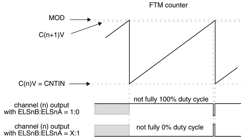
**Figure 43-29. Channel (n) output if  $C(n)V = CNTIN$  and  $CNTIN < C(n+1)V < MOD$  and  $C(n+1)V$  is Almost Equal to MOD**
