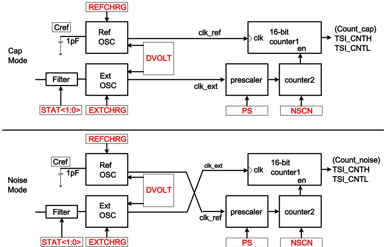
Figure 35-5. TSI noise detection mode block diagram
