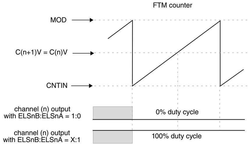
**Figure 43-31. Channel (n) output if  $(CNTIN < C(n)V < MOD)$  and  $(CNTIN < C(n+1)V < MOD)$  and  $(C(n)V = C(n+1)V)$**
