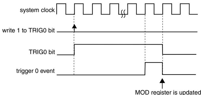
**Figure 43-49. MOD synchronization with (SYNCMODE = 0), (HWTRIGMODE = 0), (PWMSYNC = 0), (REINIT = 1), and a hardware trigger was used**
