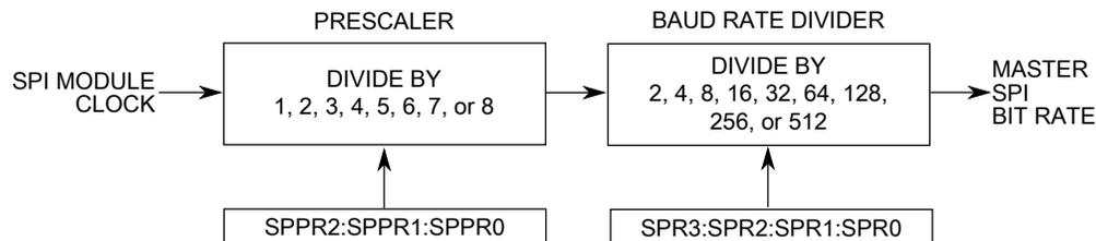
Figure 31-8. SPI baud rate generation
