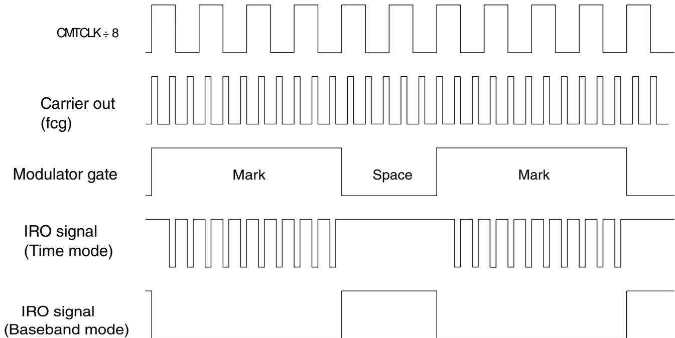
**Figure 46-5. Example: CMT output in Time and Baseband modes with  $\text{OC}[\text{CMTPOL}] = 0$**
