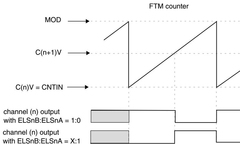
**Figure 43-27. Channel (n) output if  $(C(n)V = CNTIN)$  and  $(CNTIN < C(n+1)V < MOD)$**
