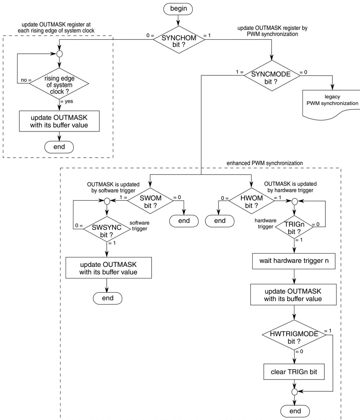
Figure 43-51. OUTMASK register synchronization flowchart
