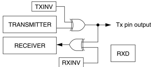
**Figure 53-25. Loop operation ( $C1[LOOPS] = 1$ ,  $C1[RSRC] = 0$ )**
