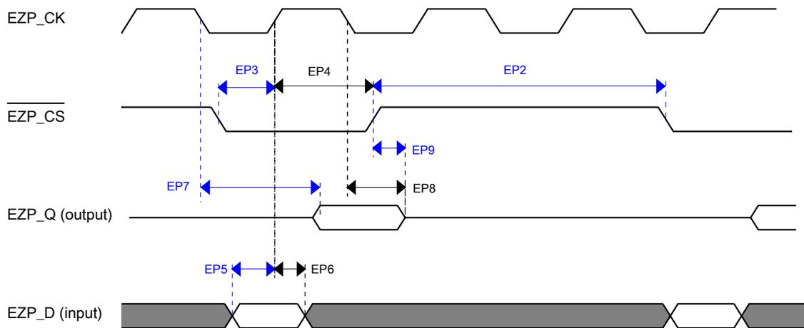
Figure 11. EzPort Timing Diagram
