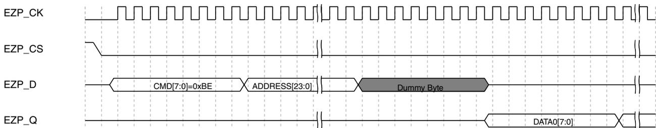
**Figure 36-15. Read FlexRAM at High Speed command sequence**
