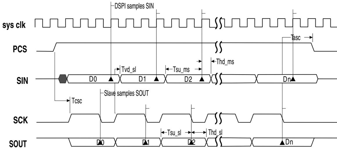
Figure 51-11. DSPI Modified Transfer Format (MTFE=1, CPHA=1,  $f_{sck} = f_{sys}/3$ )
