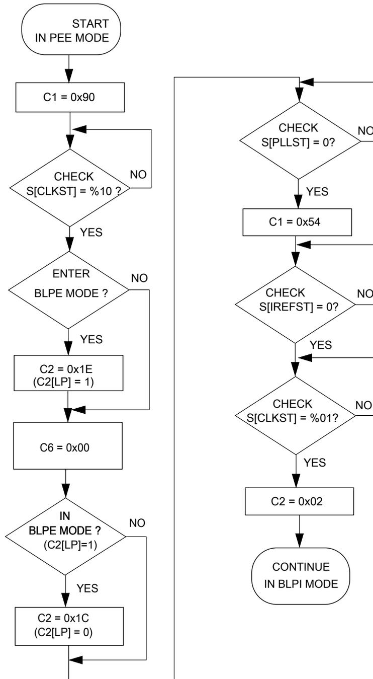
Figure 20-4. Flowchart of PEE to BLPI mode transition using an 4 MHz crystal
