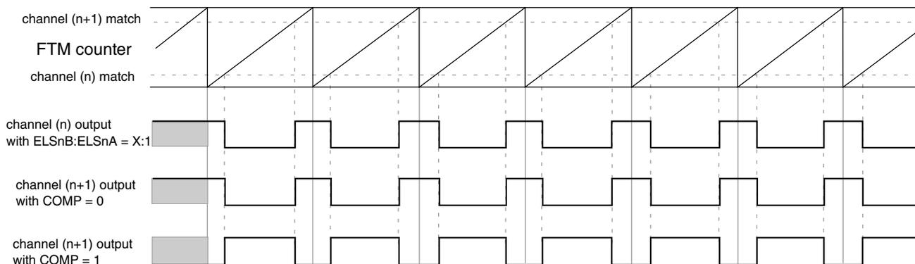
**Figure 43-41. Channel (n+1) output in Complementary mode with (ELSnB:ELSnA = X:1)**
