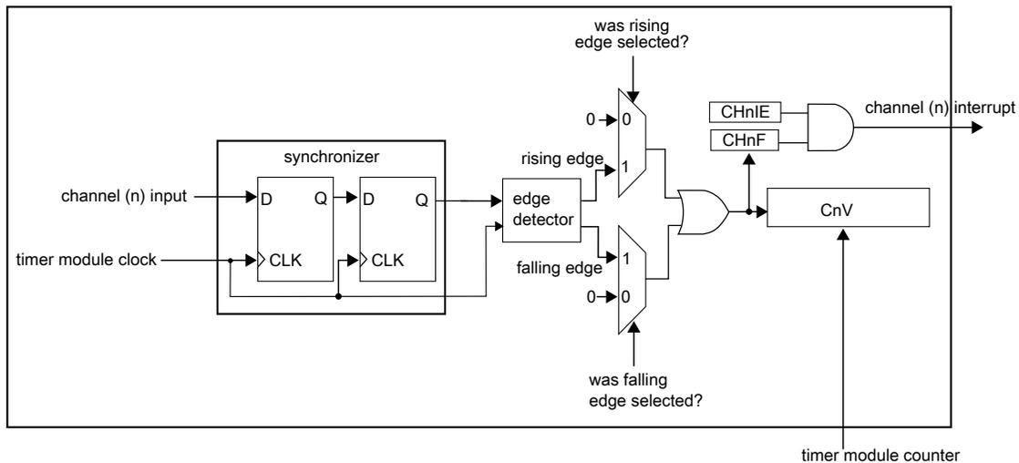
Figure 27-5. Input capture mode
