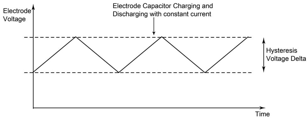
**Figure 35-3. TSI electrode oscillator chart**
