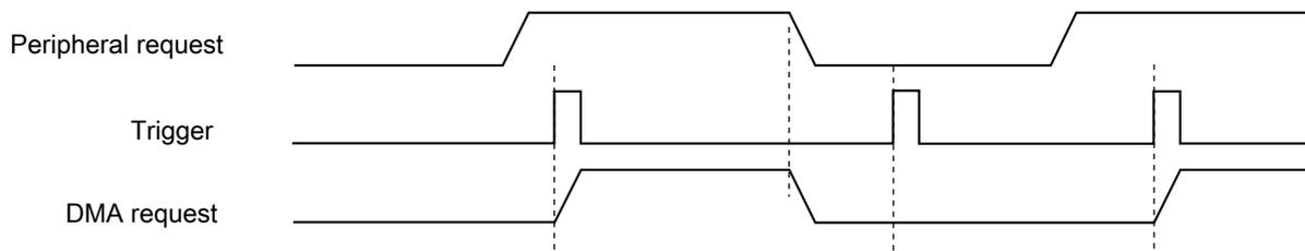
**Figure 18-4. DMAMUX channel triggering: ignored trigger**
