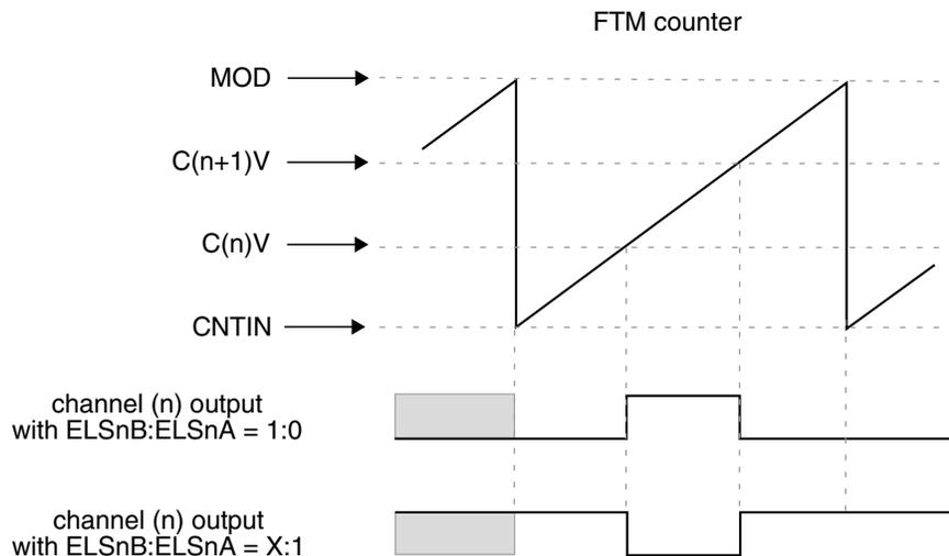
**Figure 43-25. Channel (n) output if (CNTIN < C(n)V < MOD) and (CNTIN < C(n+1)V < MOD) and (C(n)V < C(n+1)V)**
