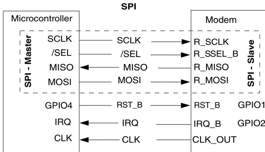
**Figure 2-4. Microcontroller to modem interface block diagram**
