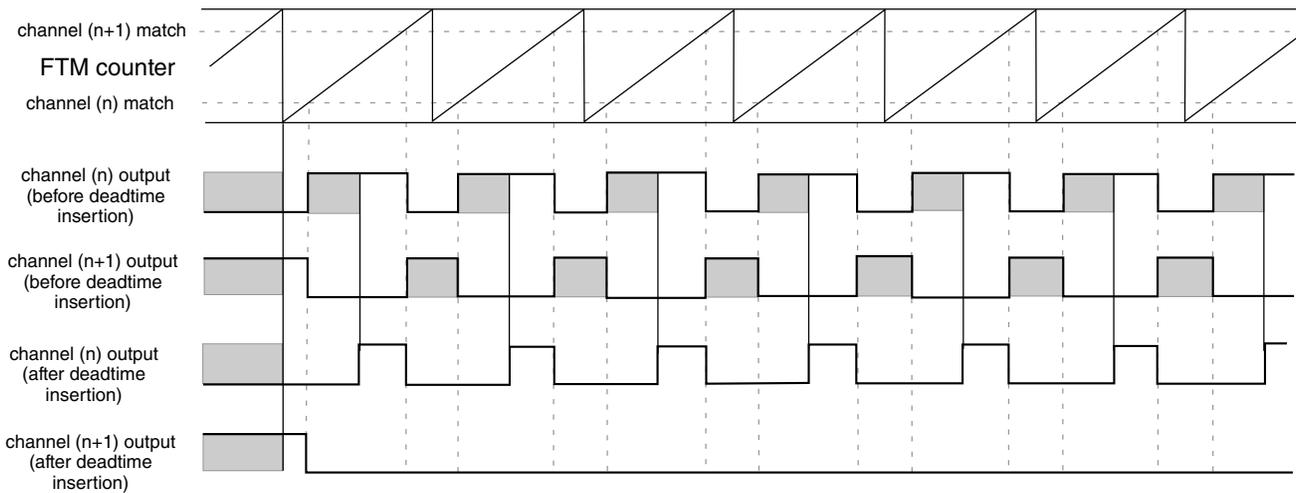
**Figure 43-67. Example of the deadtime insertion (ELSnB:ELSnA = 1:0, POL(n) = 0, and POL(n+1) = 0) when the deadtime delay is comparable to channel (n+1) duty cycle**
