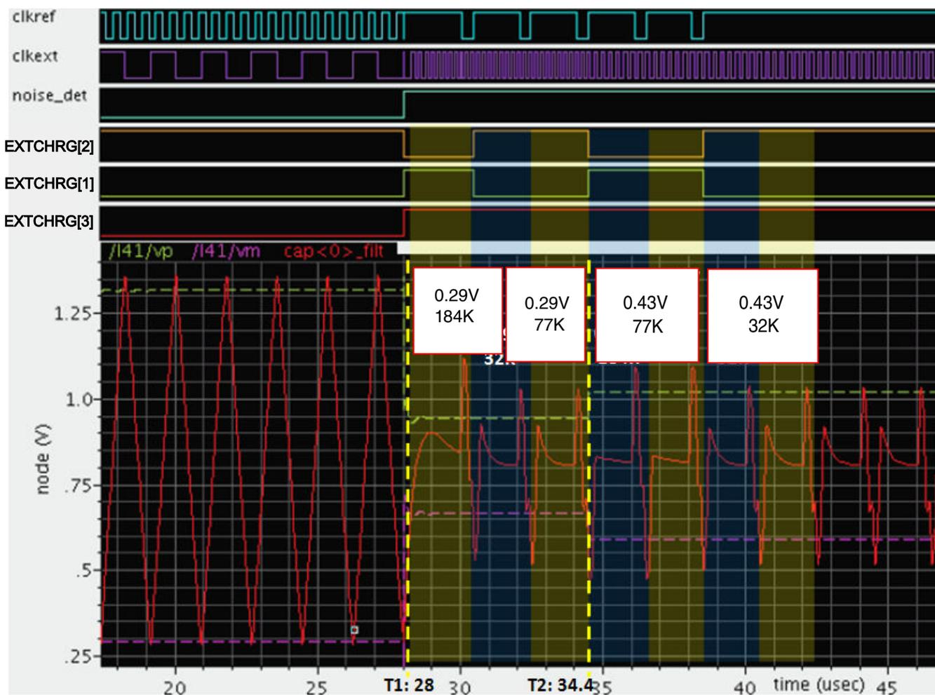
Figure 35-9. TSI noise detection mode waveform
