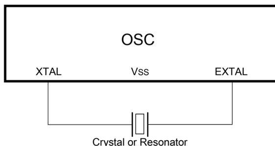
**Figure 21-2. Crystal/Ceramic Resonator Connections - Connection 1**
