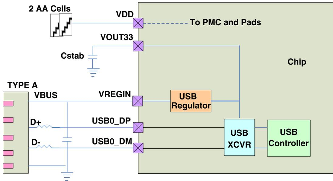
Figure 10-43. USB regulator AA cell usecase
