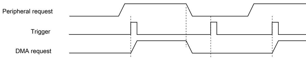
**Figure 27-4. DMAMUX channel triggering: ignored trigger**
