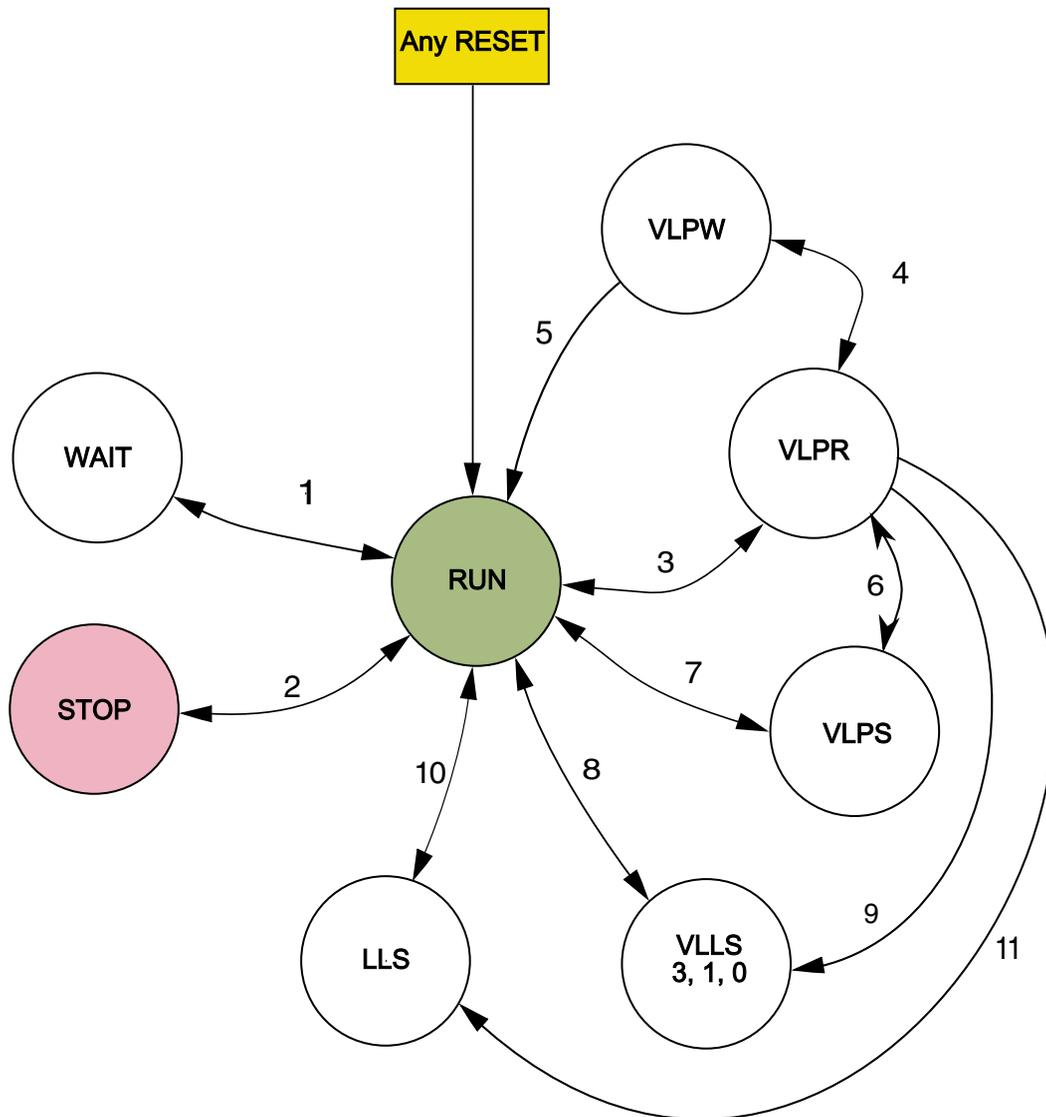
**Figure 9-1. Power mode state diagram**
