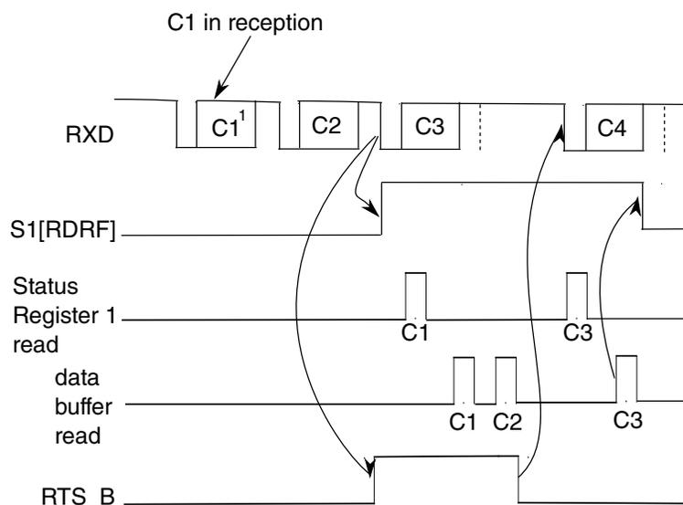
**Figure 53-11. Receiver hardware flow control timing diagram**
