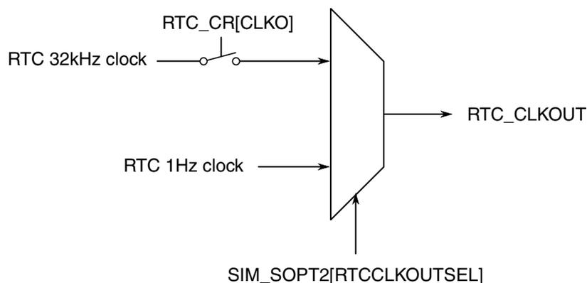
Figure 10-41. RTC\_CLKOUT generation
