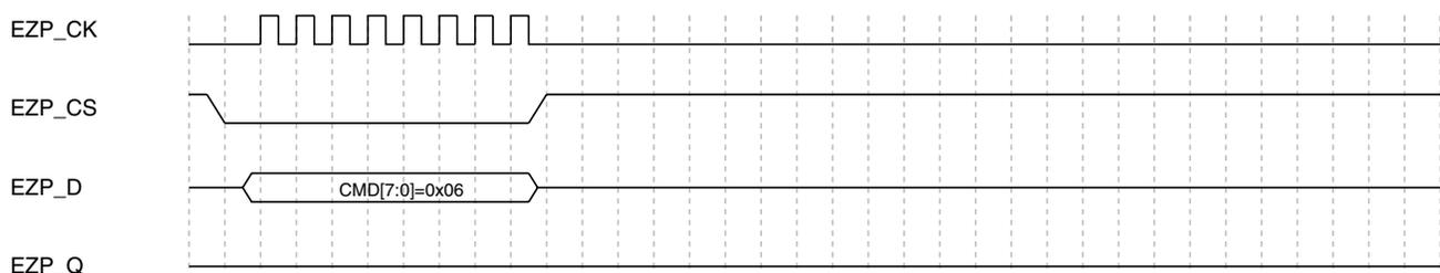
**Figure 36-2. Write Enable command sequence**
