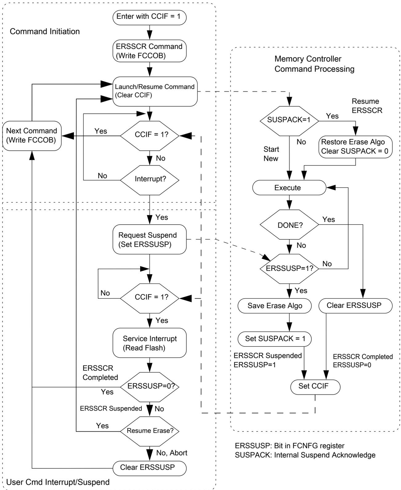
Figure 35-10. Suspend and Resume of Erase Flash Sector Operation
