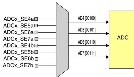
Figure 10-32. ADCx\_SEn channels a and b selection
