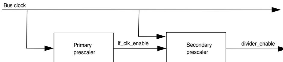
**Figure 46-2. Clock divider block diagram**
