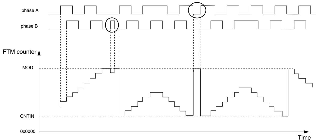
**Figure 43-93. Motor position jittering near maximum and minimum count value**
