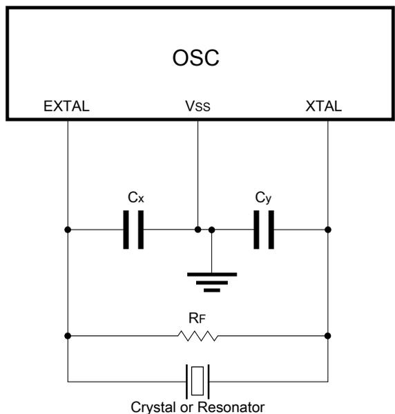
Figure 32-4. Crystal/Ceramic Resonator Connections - Connection 3
