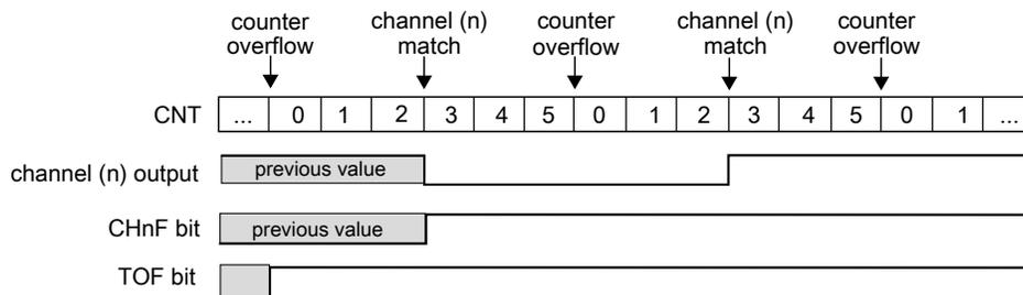
**Figure 43-15. Example of the Output Compare mode when the match toggles the channel output**
