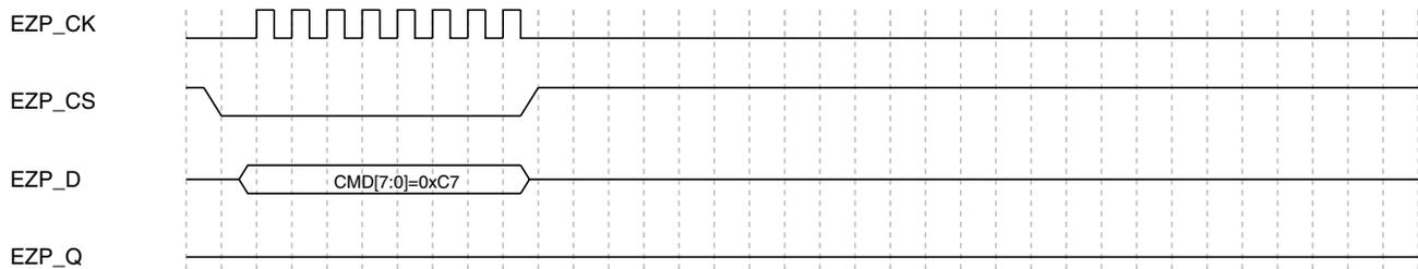
**Figure 36-9. Bulk Erase command sequence**
