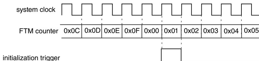
**Figure 43-76. Initialization trigger is generated when the FTM counting achieves the CNTIN register value**
