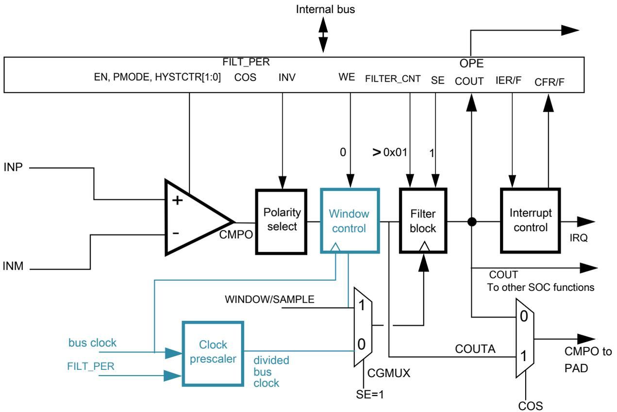
Figure 41-6. Sampled, Filtered (# 4A): sampling point externally driven
