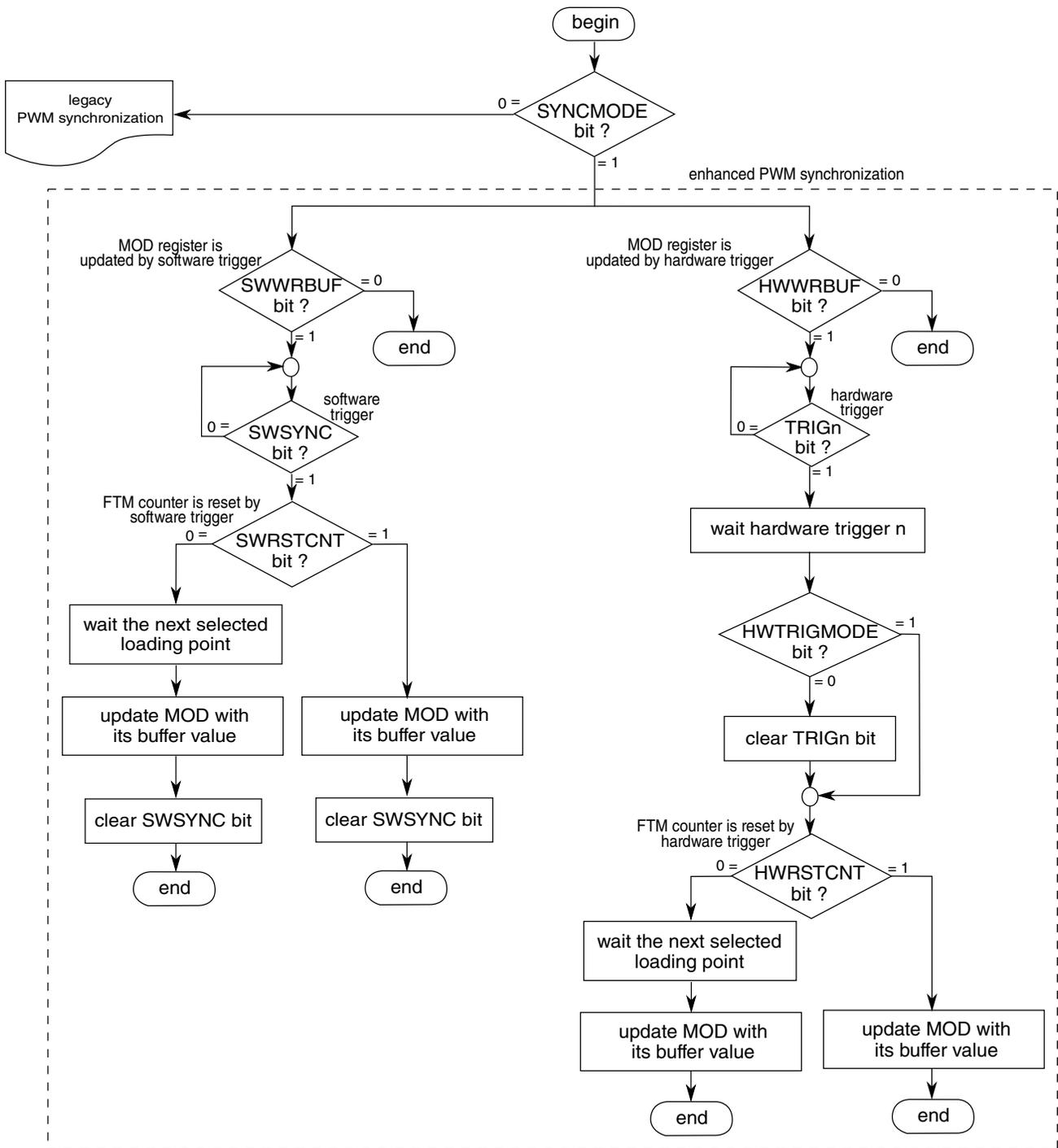
**Figure 43-45. MOD register synchronization flowchart**
