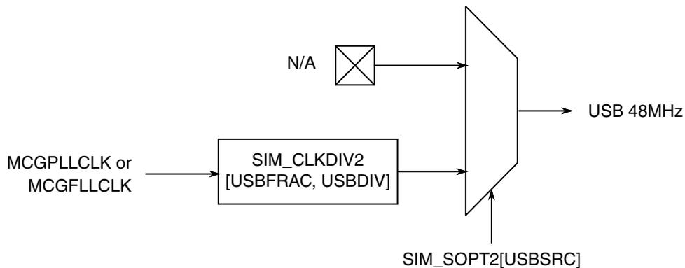
Figure 12-6. USB 48 MHz clock source
