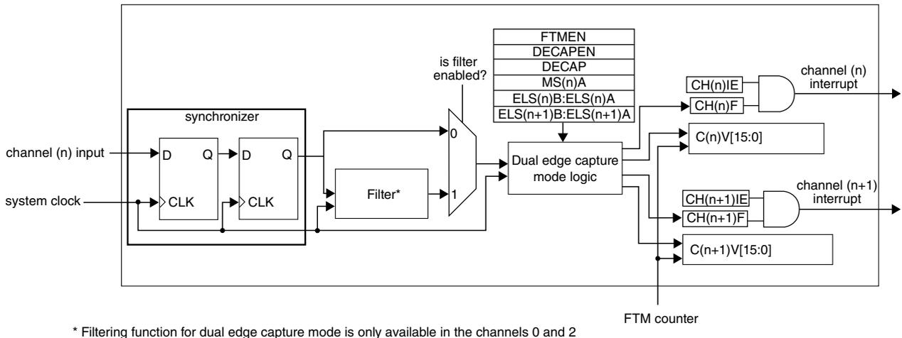
**Figure 43-81. Dual Edge Capture mode block diagram**
