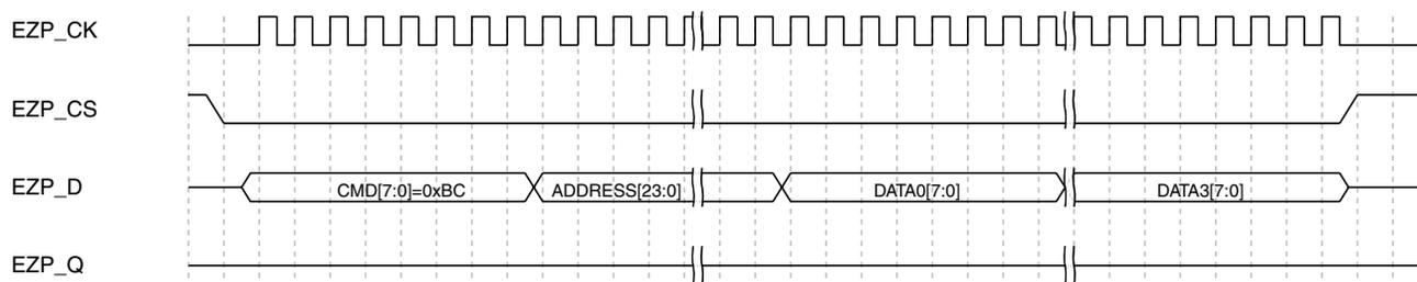
**Figure 36-13. Write FlexRAM command sequence**
