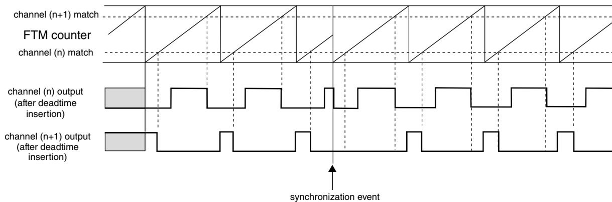
**Figure 43-57. FTM counter synchronization**
