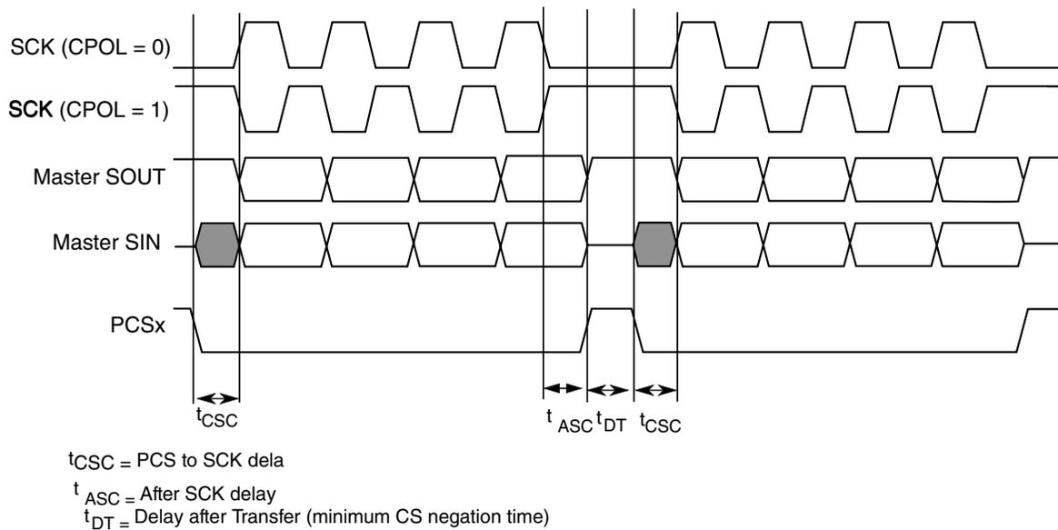
**Figure 51-13. Example of non-continuous format (CPHA=1, CONT=0)**
