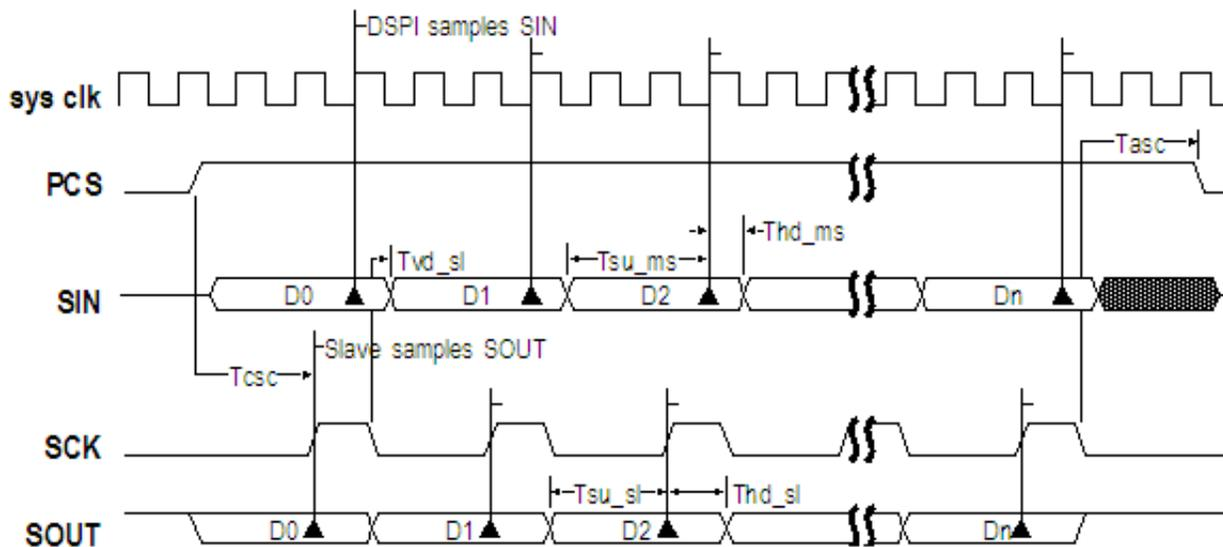
Figure 51-9. DSPI Modified Transfer Format (MTFE=1, CPHA=0,  $f_{sck} = f_{sys}/3$ )
