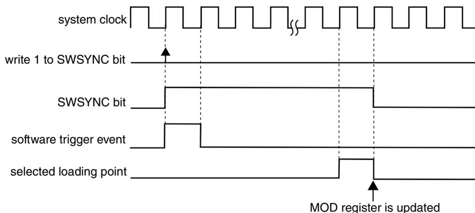
**Figure 43-50. MOD synchronization with (SYNCMODE = 0) and (PWMSYNC = 1)**
