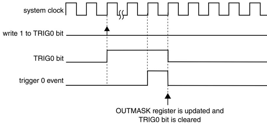
**Figure 43-53. OUTMASK synchronization with ( $\text{SYNCMODE} = 0$ ), ( $\text{HWTRIGMODE} = 0$ ), ( $\text{SYNCHOM} = 1$ ), ( $\text{PWMSYNC} = 0$ ), and a hardware trigger was used**
