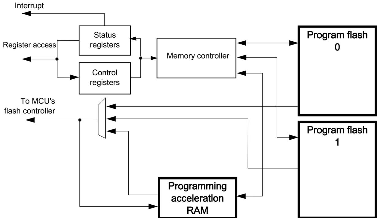
Figure 35-2. Flash Block Diagram
