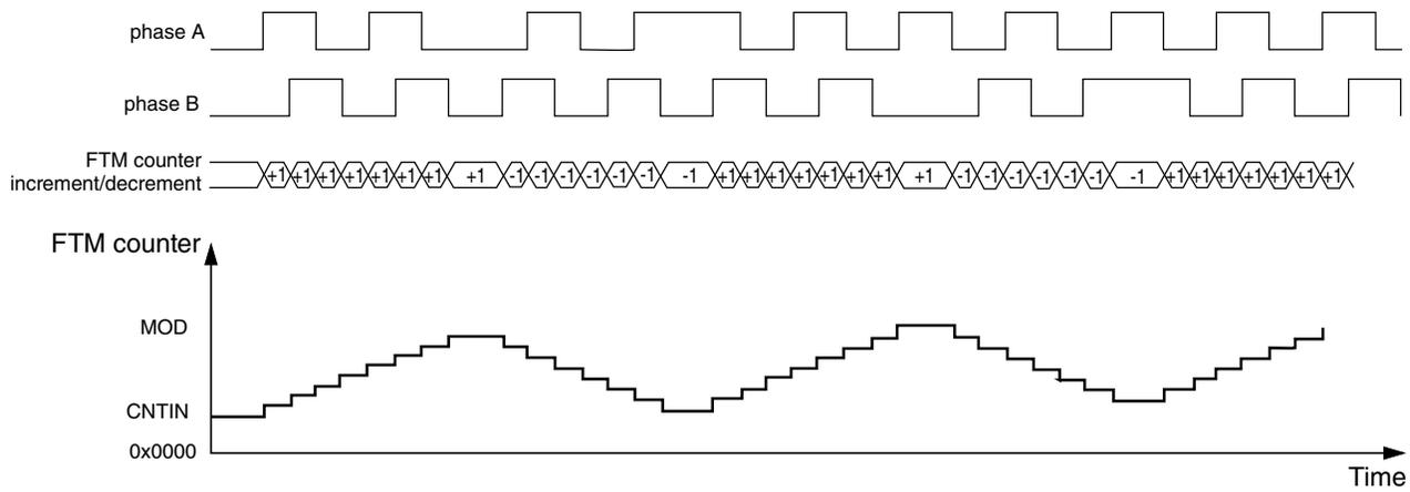
**Figure 43-89. Quadrature Decoder – Phase A and Phase B Encoding mode**
