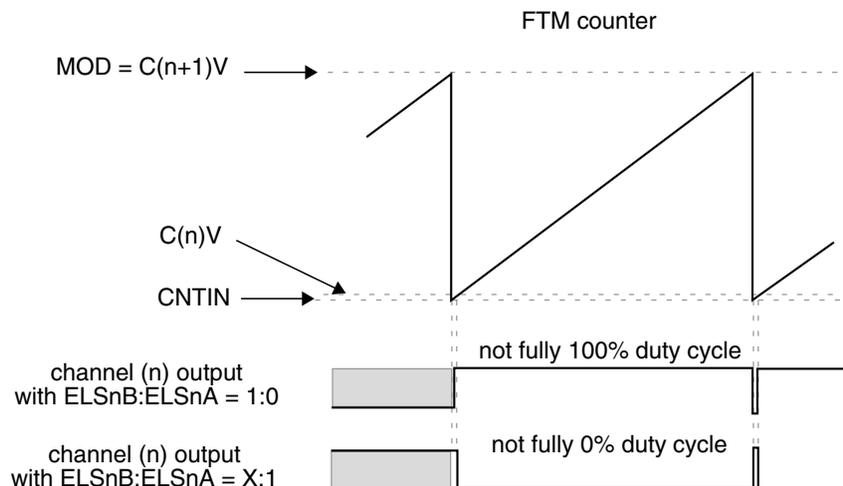
**Figure 43-28. Channel (n) output if  $(CNTIN < C(n)V < MOD)$  and  $(C(n)V$  is Almost Equal to  $CNTIN)$  and  $(C(n+1)V = MOD)$**
