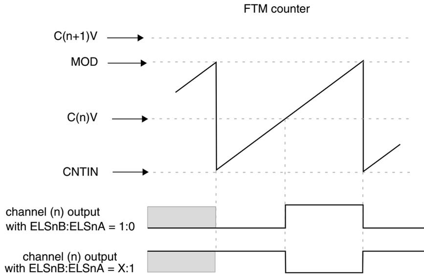
**Figure 43-38. Channel (n) output if  $(C(n+1)V > MOD$  and  $(CNTIN < C(n)V < MOD)$**
