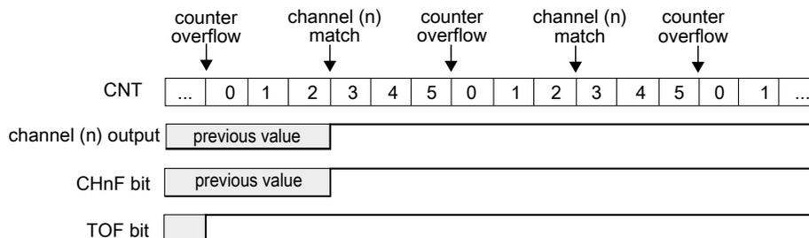
**Figure 43-17. Example of the Output Compare mode when the match sets the channel output**
