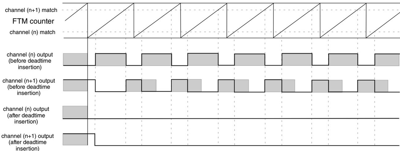
**Figure 43-68. Example of the deadtime insertion (ELSnB:ELSnA = 1:0, POL(n) = 0, and POL(n+1) = 0) when the deadtime delay is comparable to channels (n) and (n+1) duty cycle**
