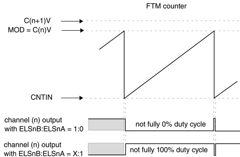
**Figure 43-39. Channel (n) output if  $(C(n+1)V > MOD$  and  $(CNTIN < C(n)V = MOD)$**
