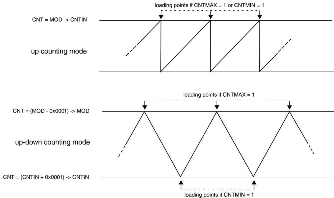
**Figure 43-44. Boundary cycles and loading points**
