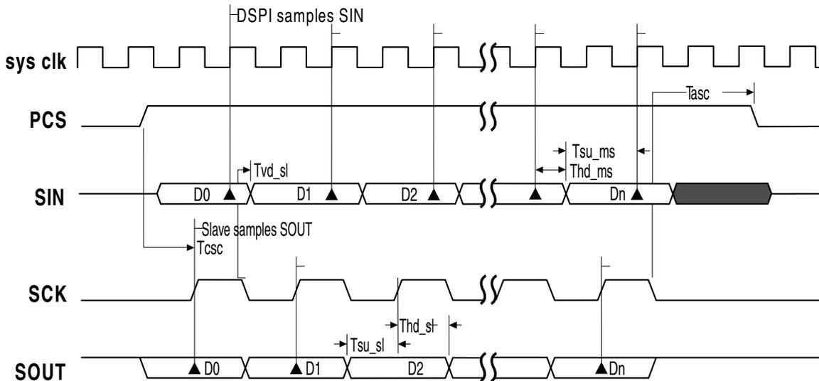
**Figure 51-8. DSPI Modified Transfer Format (MTFE=1, CPHA=0,  $f_{sck} = f_{sys}/2$ )**
