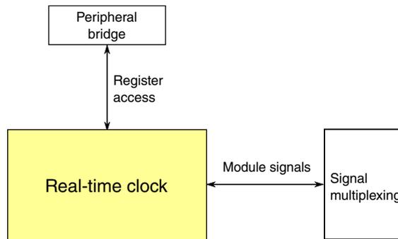
Figure 10-40. RTC configuration
