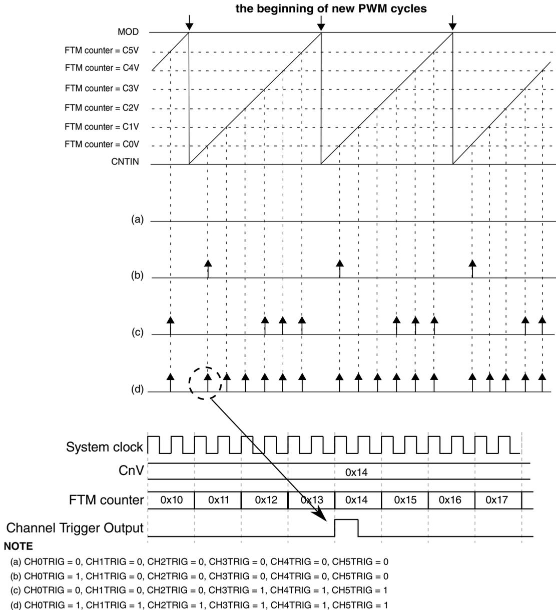
**Figure 43-75. Channel match trigger**
