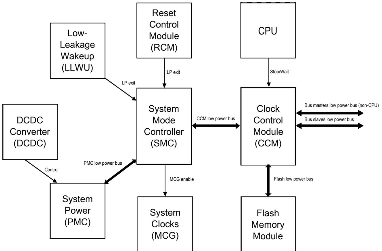
**Figure 9-2. Low-power system components and connections**
