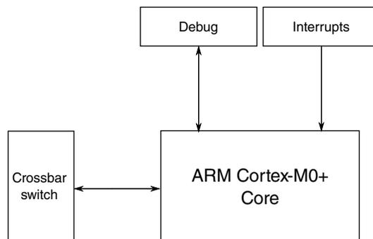
Figure 1-1. Core configuration
