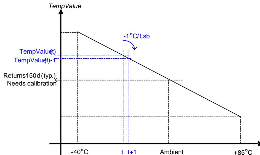
Figure 5-12. Temperature Sensor Response
