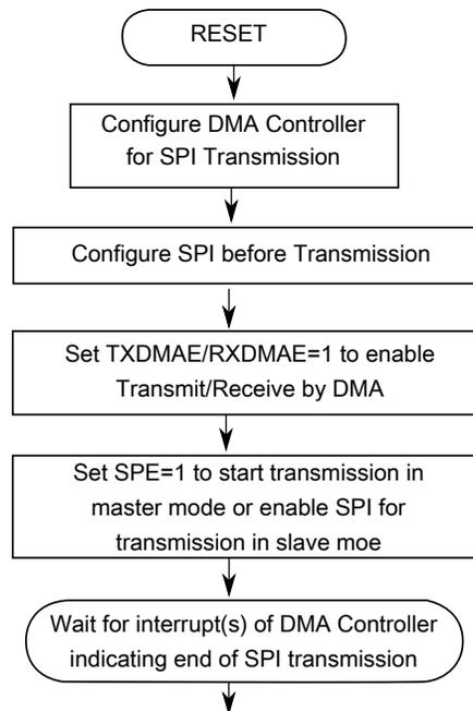
Figure 31-5. Basic Flow of SPI Transmission by DMA
