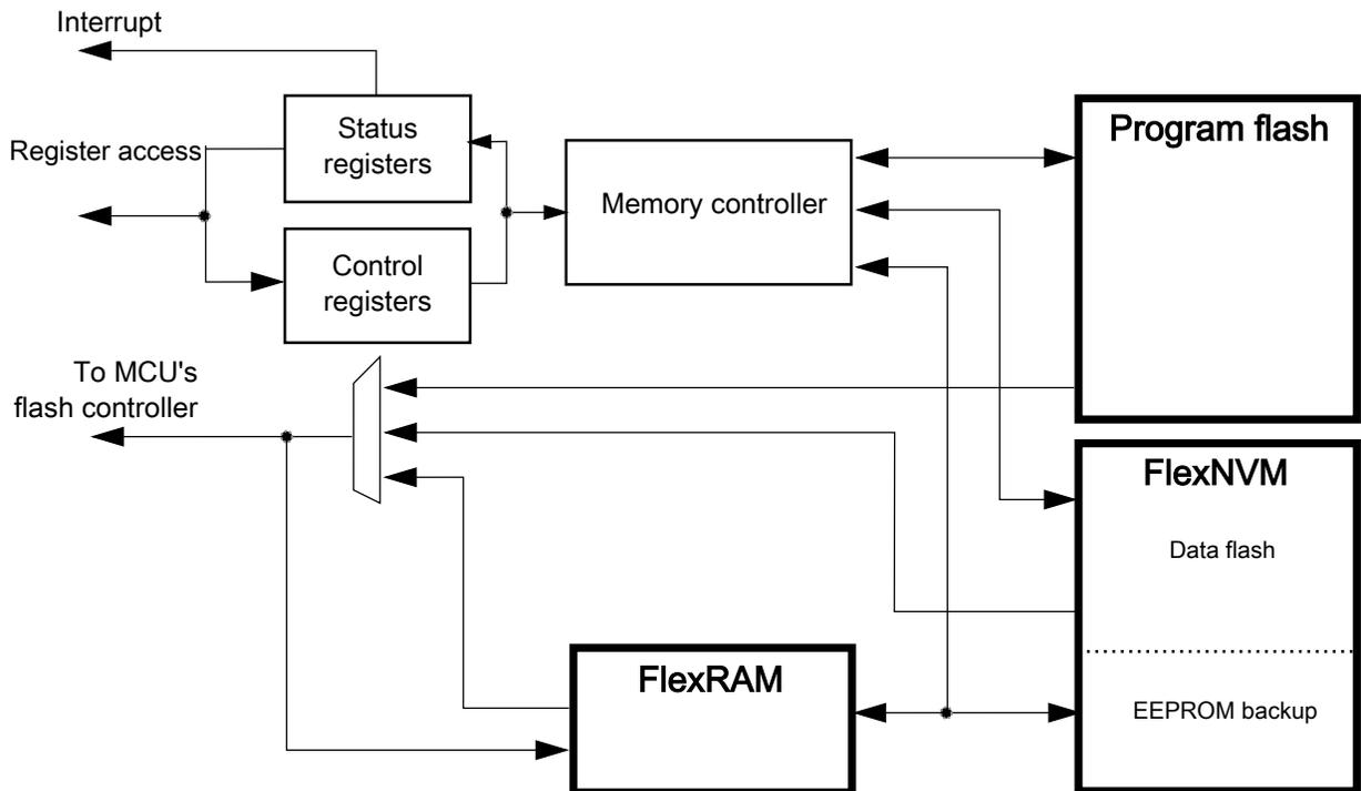
Figure 35-1. Flash Block Diagram
