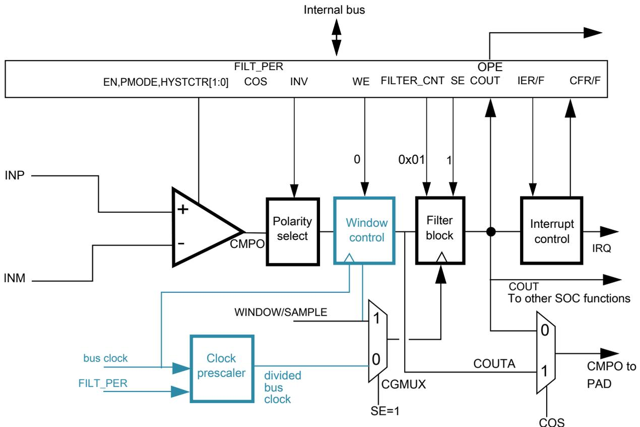
**Figure 41-4. Sampled, Non-Filtered (# 3A): sampling point externally driven**
