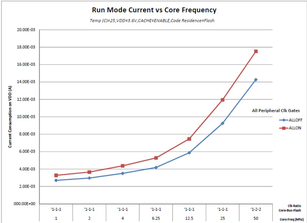
Figure 5. Run mode supply current vs. core frequency
