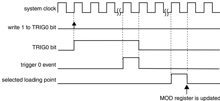
**Figure 43-47. MOD synchronization with (SYNCMODE = 0), (HWTRIGMODE = 0), (PWMSYNC = 0), (REINIT = 0), and a hardware trigger was used**
