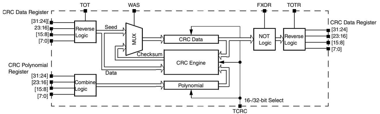
Figure 37-1. Programmable cyclic redundancy check (CRC) block diagram
