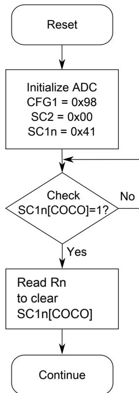
Figure 40-2. Initialization flowchart example
