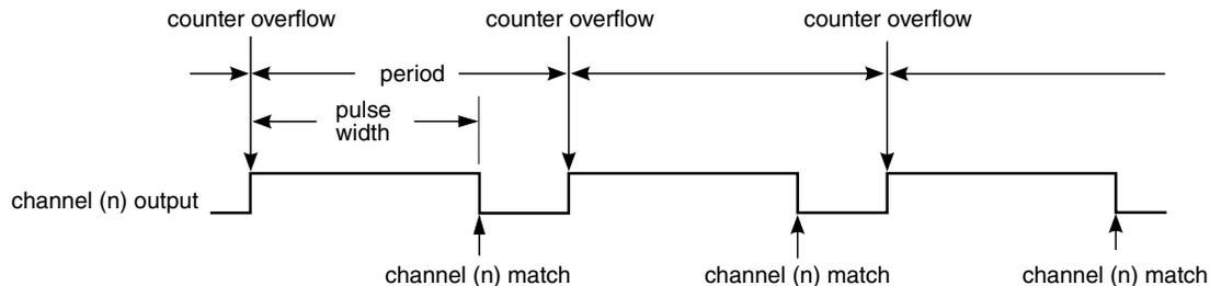
**Figure 43-18. EPWM period and pulse width with  $ELSnB:ELSnA = 1:0$**
