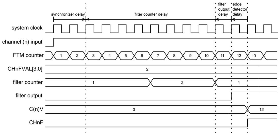
Figure 43-14. Input capture example
