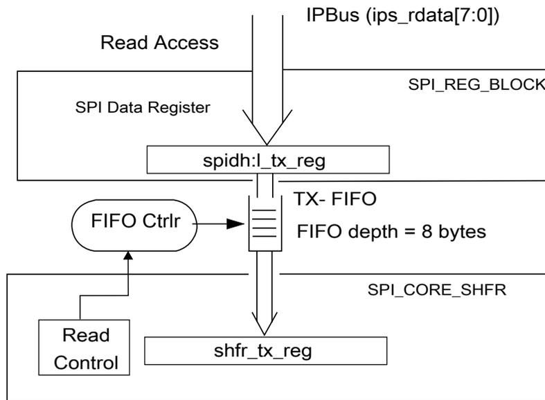
Figure 31-4. SPIH:L write side structural overview in FIFO mode
