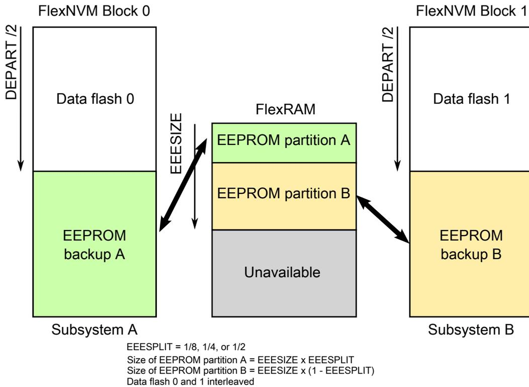
**Figure 35-7. FlexRAM to FlexNVM Memory Mapping with 2 Sub-systems**
