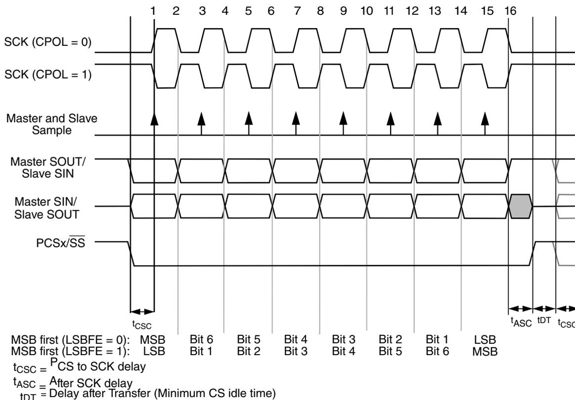
**Figure 51-5. Module transfer timing diagram (MTFE=0, CPHA=0, FMSZ=8)**
