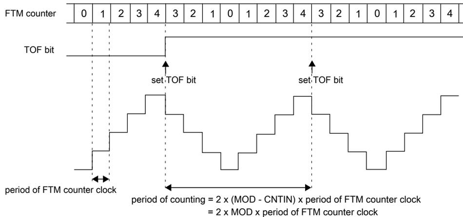
**Figure 43-7. Example of up-down counting when CNTIN = 0x0000**
