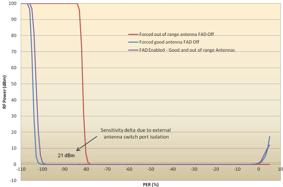
**Figure 4-10. Sensitivity FAD mode at 2450 MHz**
