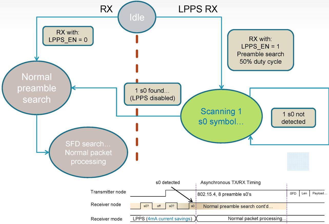
Figure 4-13. LPPS flow diagram
