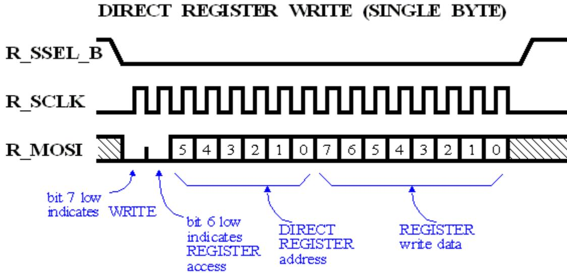
Figure 8-5. Single-Byte Write Access to a Direct Register
