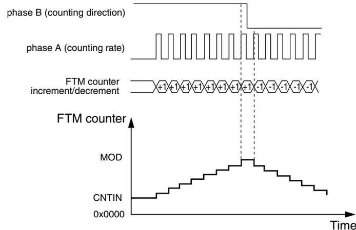
**Figure 43-88. Quadrature Decoder – Count and Direction Encoding mode**
