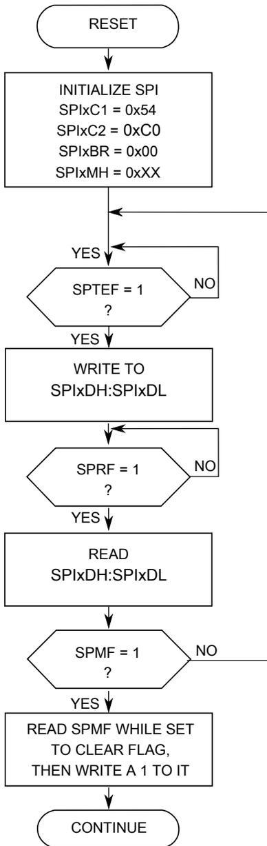
**Figure 31-9. Initialization Flowchart Example for SPI Master Device in 16-bit Mode for FIFOMODE = 0**
