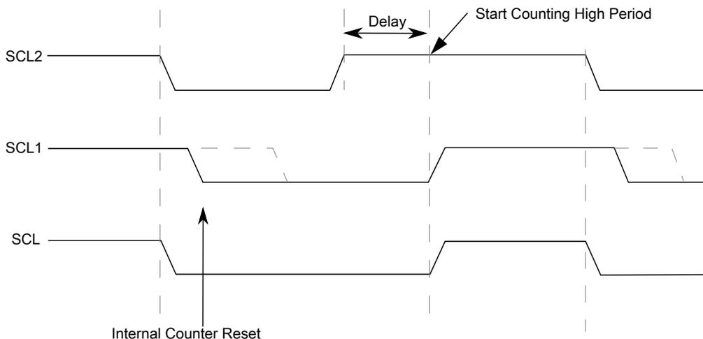
**Figure 36-3. I2C clock synchronization**
