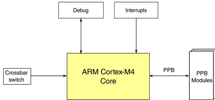
Figure 10-1. Core configuration
