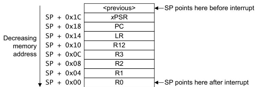
Immediately after stacking, the stack pointer indicates the lowest address in the stack frame. The stack frame is aligned to a double-word address.
