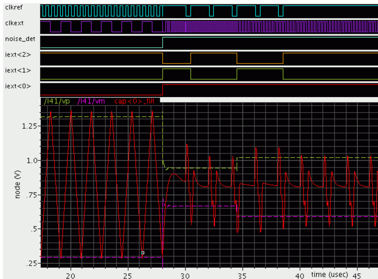
Figure 41-16. TSI noise detection mode waveform
