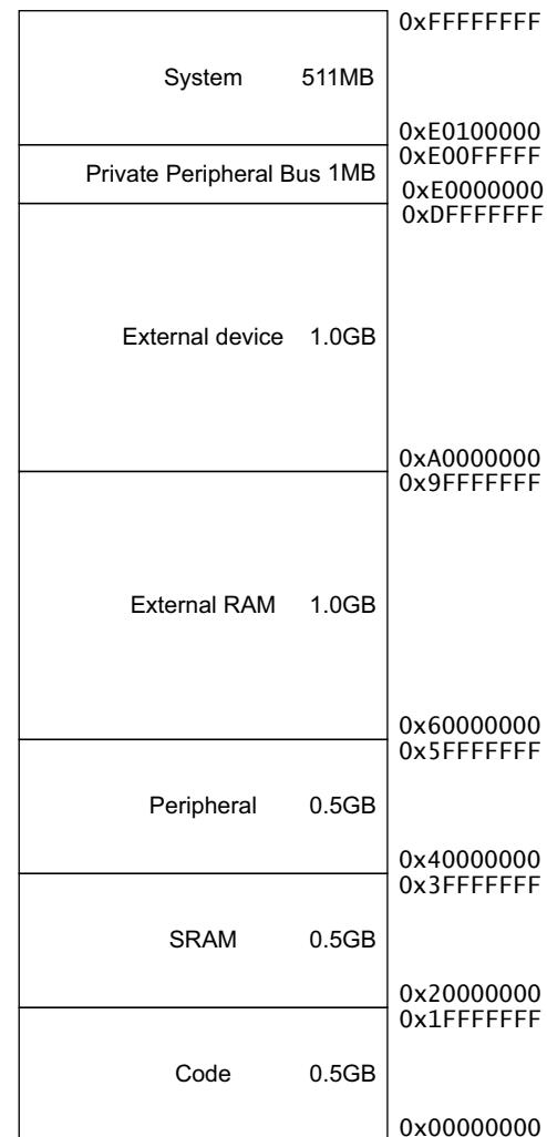
The processor reserves regions of the *Private Peripheral Bus* (PPB) address range for core peripheral registers, see [About the Cortex-M0+ processor and core peripherals](#) on page 1-2.
