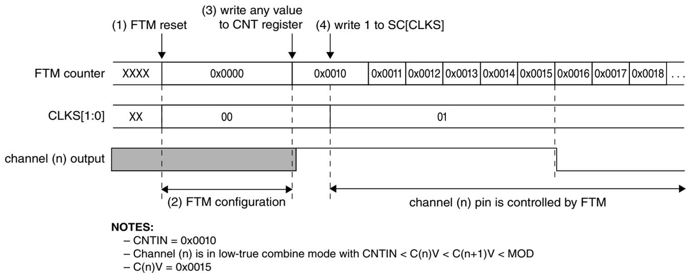
**Figure 26-88. FTM behavior after reset when the channel (n) is in Combine mode**
