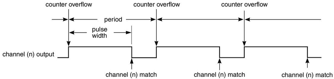
**Figure 26-17. EPWM period and pulse width with ELSnB:ELSnA = 1:0**
