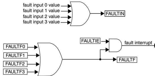
**Figure 26-70. FAULTF and FAULTIN bits and fault interrupt**
