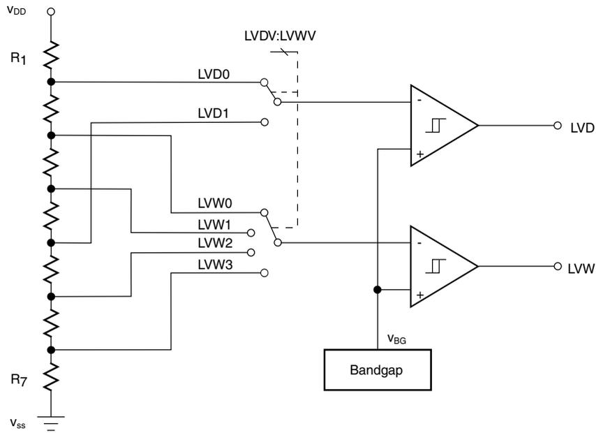
Figure 13-1. Low voltage detect (LVD) block diagram
