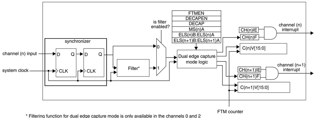
**Figure 26-80. Dual Edge Capture mode block diagram**
