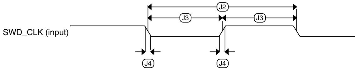
**Figure 13. Serial wire clock input timing**
