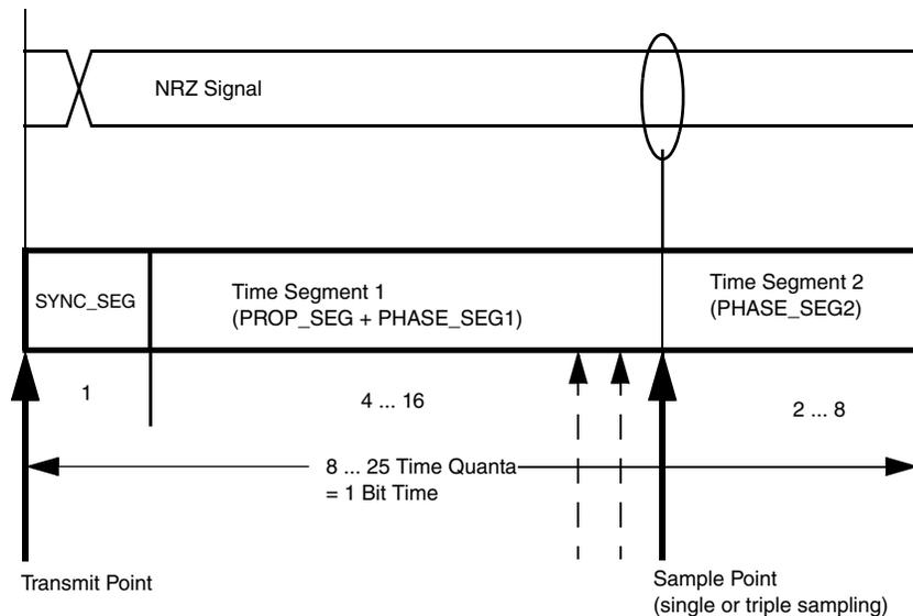
**Figure 32-9. Segments within the bit time**
