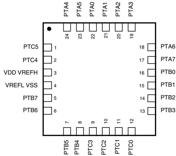
**Figure 21. 24-pin QFN package**
