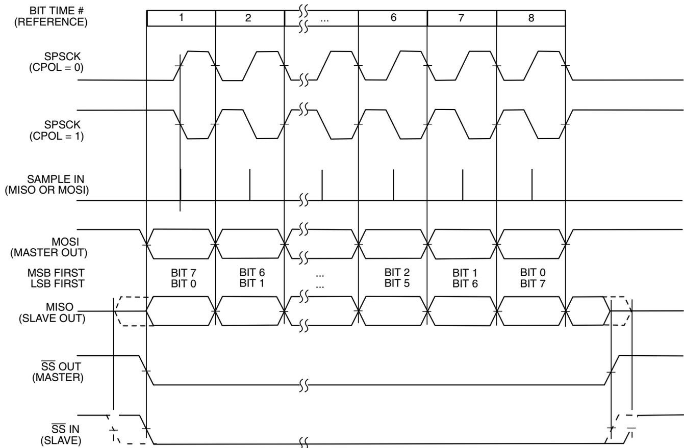
**Figure 30-4. SPI clock formats (CPHA = 0)**
