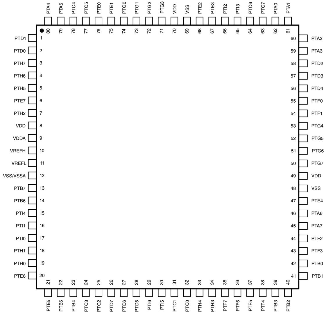
Figure 21. 80-pin LQFP package
