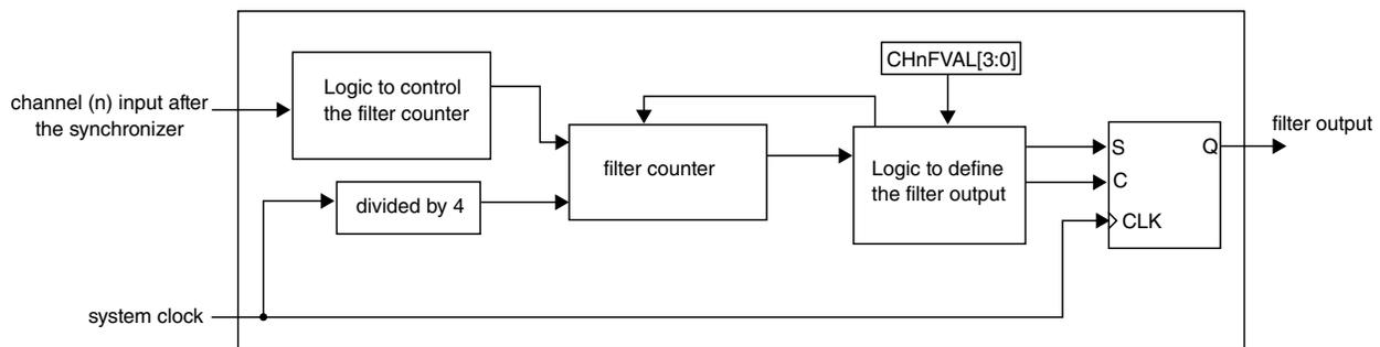
**Figure 26-12. Channel input filter**
