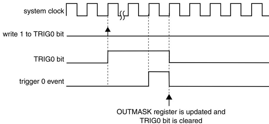
**Figure 26-52. OUTMASK synchronization with ( $\text{SYNCMODE} = 0$ ), ( $\text{HWTRIGMODE} = 0$ ), ( $\text{SYNCHOM} = 1$ ), ( $\text{PWMSYNC} = 0$ ), and a hardware trigger was used**
