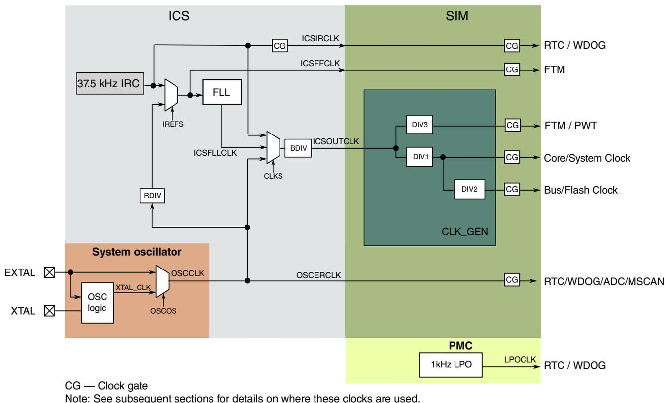
**Figure 5-1. Clocking diagram**
