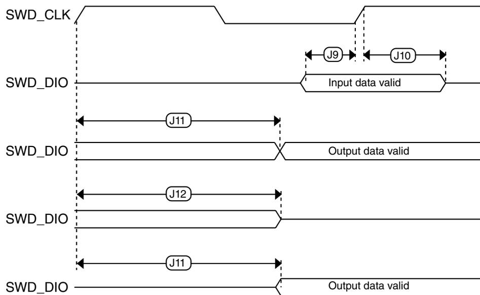
**Figure 14. Serial wire data timing**
