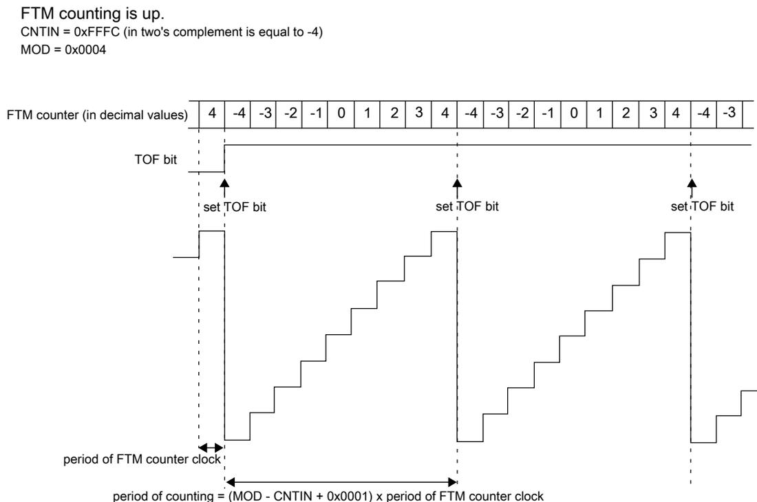
**Figure 26-4. Example of FTM up and signed counting**
