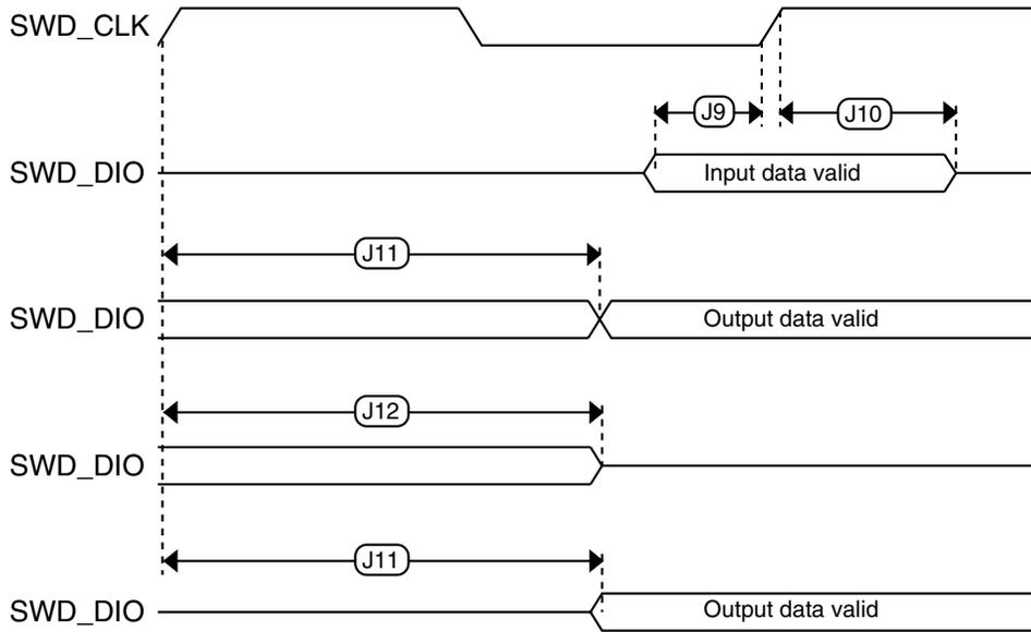
Figure 14. Serial wire data timing
