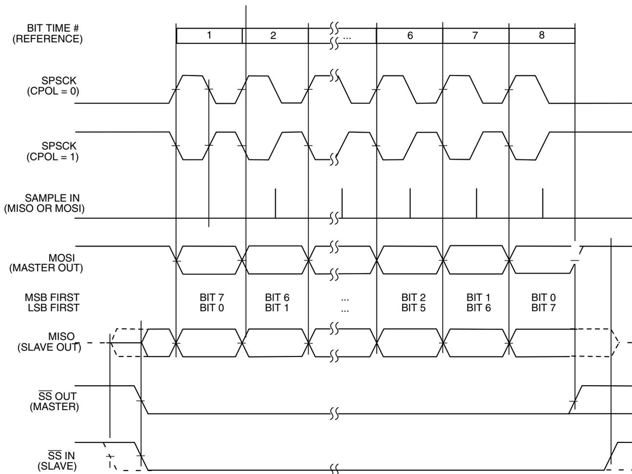
**Figure 30-3. SPI clock formats (CPHA = 1)**
