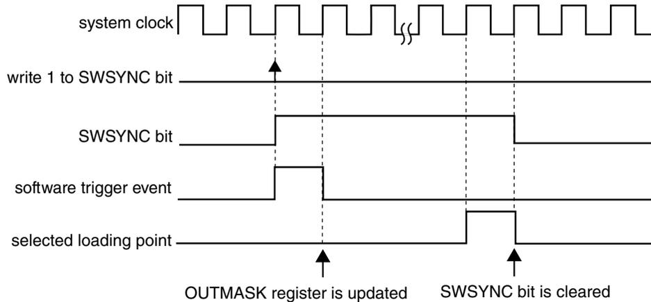
**Figure 26-51. OUTMASK synchronization with ( $\text{SYNCMODE} = 0$ ), ( $\text{SYNCHOM} = 1$ ), ( $\text{PWMSYNC} = 0$ ) and software trigger was used**
