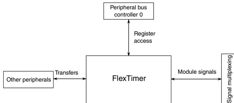
Figure 3-27. FlexTimer configuration
