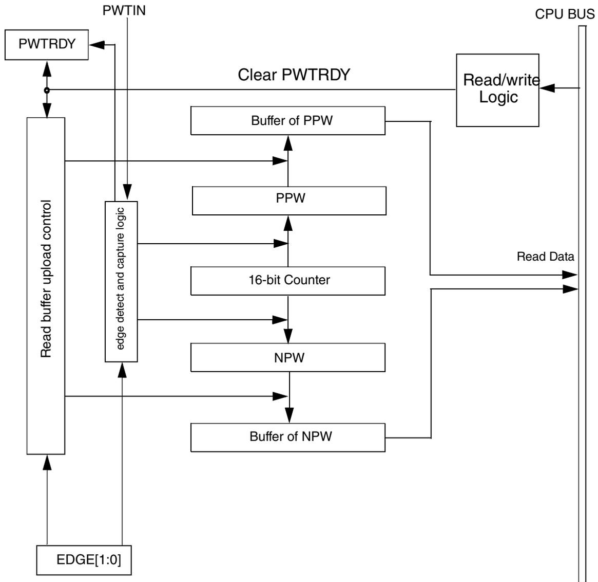
**Figure 27-3. Buffering mechanism of Pulse Width register**
