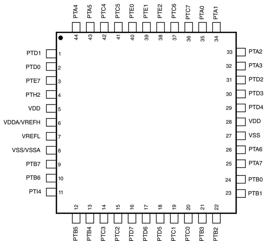
Figure 10-3. 44-pin LQFP package
