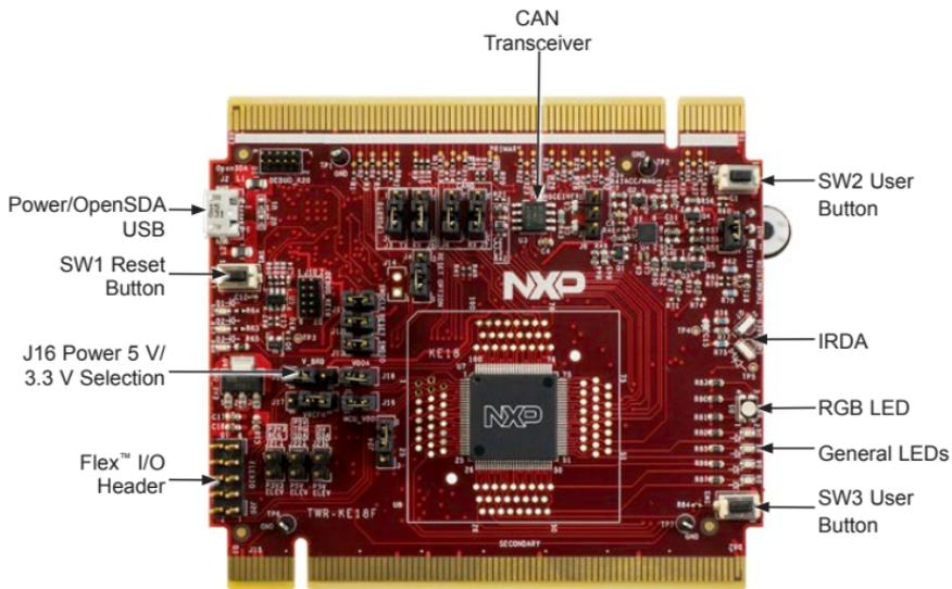
Figure 1: Front Side of TWR-KE18F
