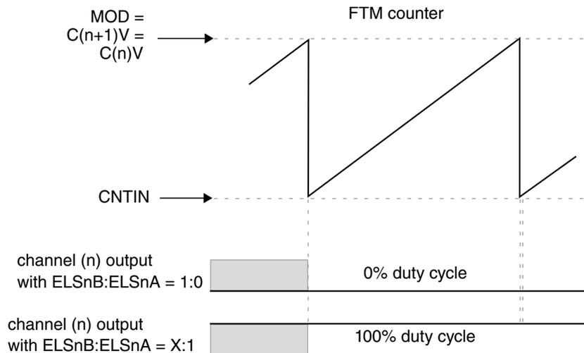
**Figure 26-32. Channel (n) output if  $(C(n)V = C(n+1)V = MOD)$**
