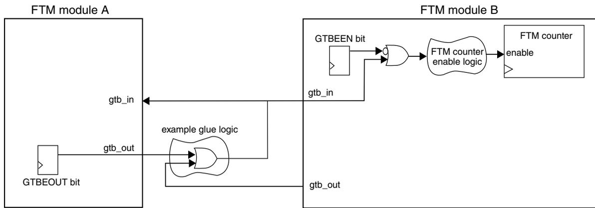
**Figure 26-87. Global time base (GTB) block diagram**
