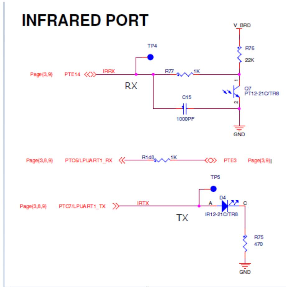
Figure 9. Infrared port
