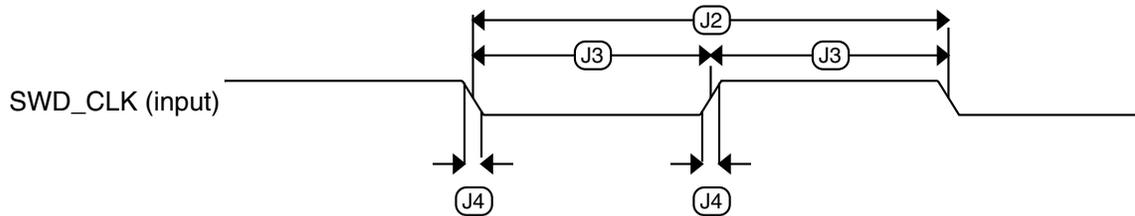
**Figure 13. Serial wire clock input timing**
