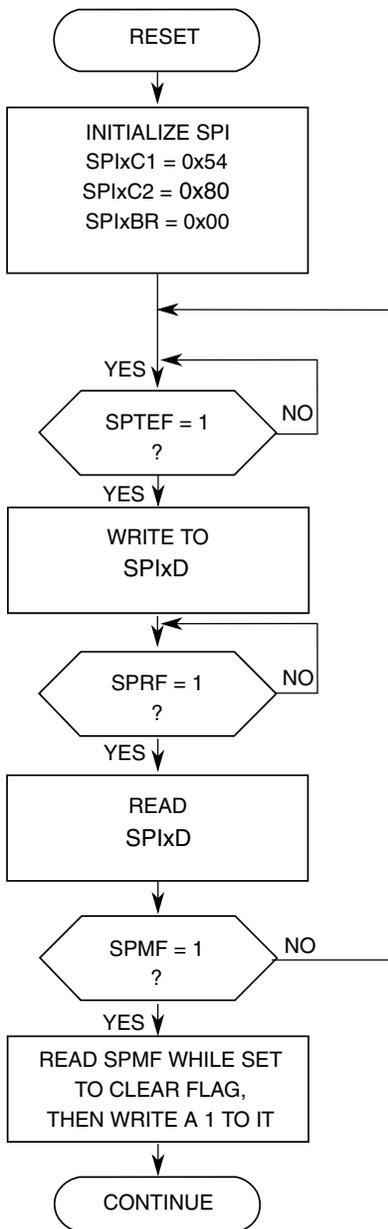
**Figure 30-6. Initialization Flowchart Example for SPI Master Device**
