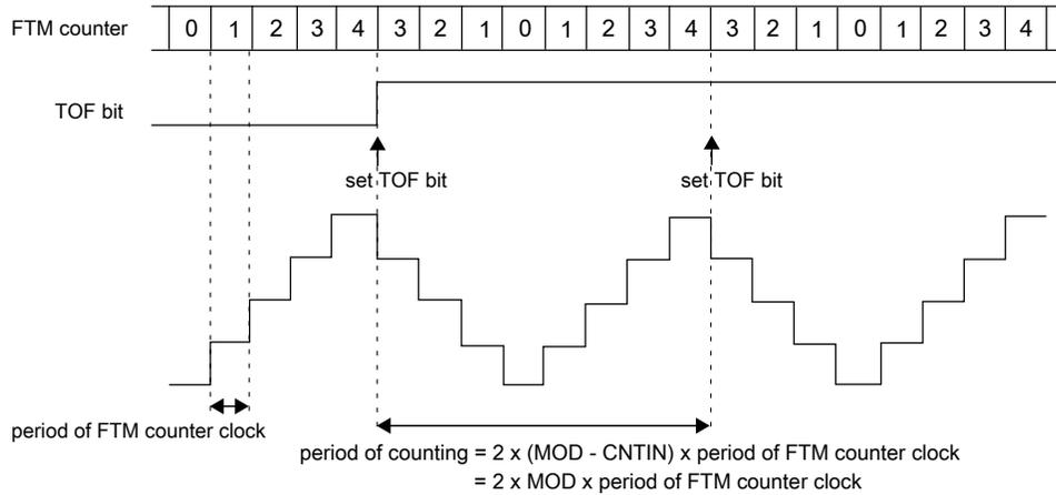
**Figure 26-7. Example of up-down counting when CNTIN = 0x0000**
