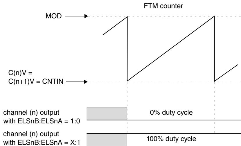
**Figure 26-31. Channel (n) output if  $(C(n)V = C(n+1)V = CNTIN)$**
