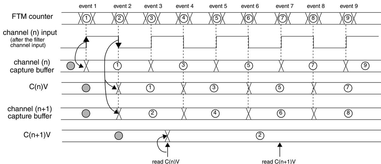
**Figure 26-85. Dual Edge Capture mode read coherency mechanism**
