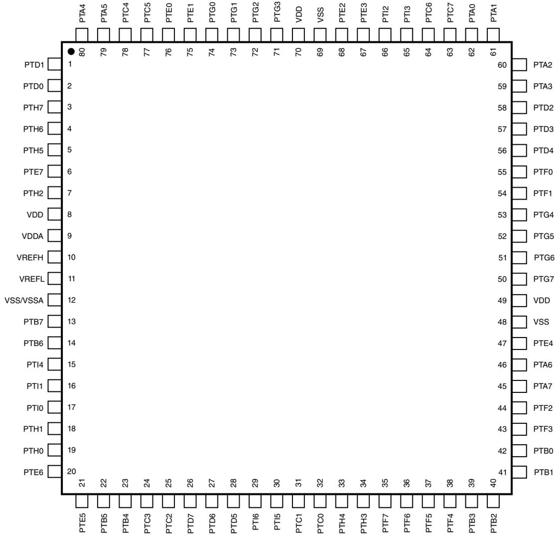
Figure 10-1. 80-pin LQFP package
