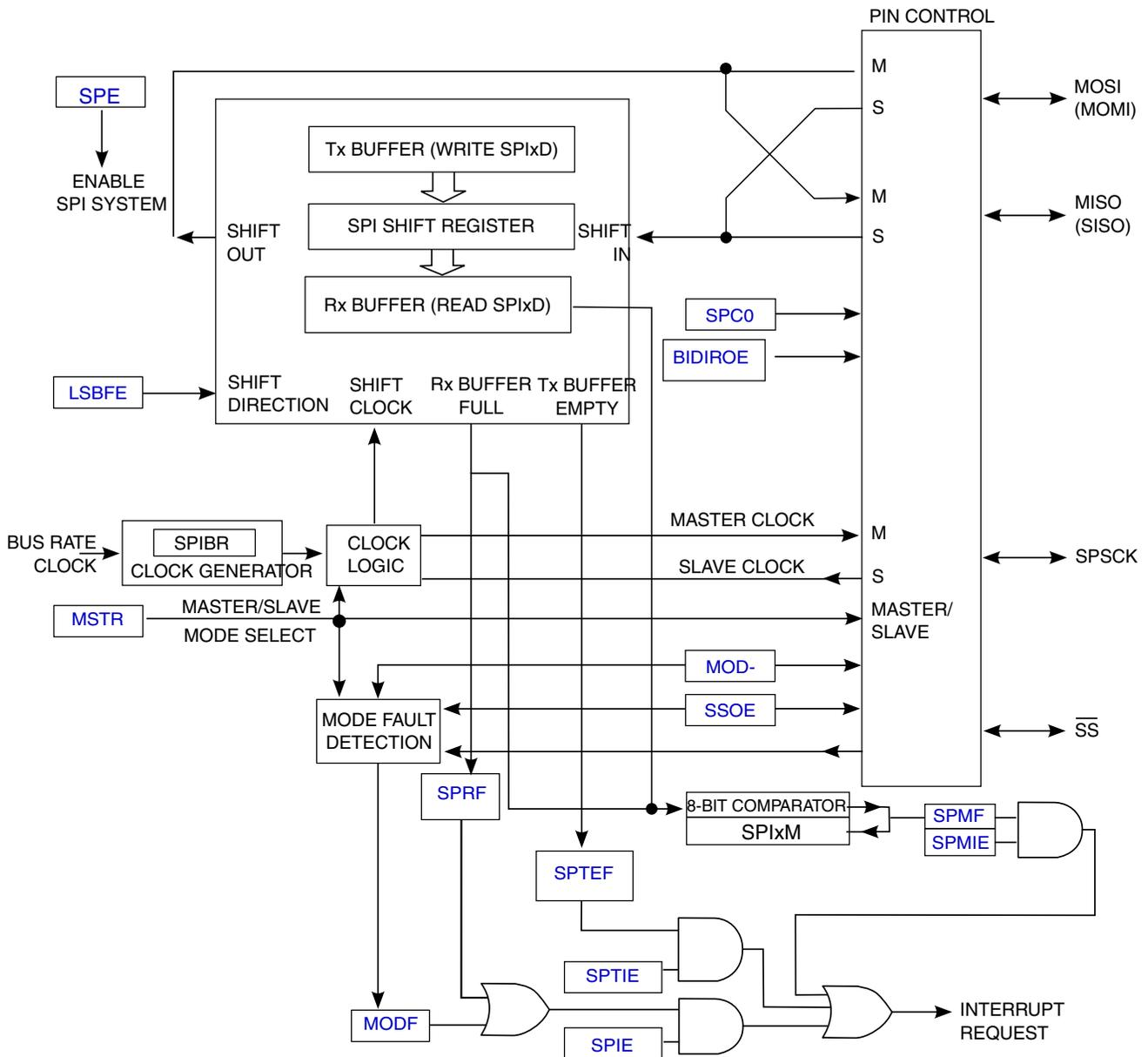
Figure 30-2. SPI module block diagram without FIFO
