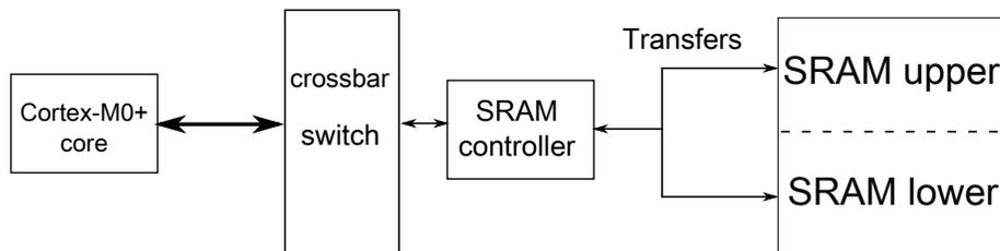
Figure 3-23. SRAM configuration
