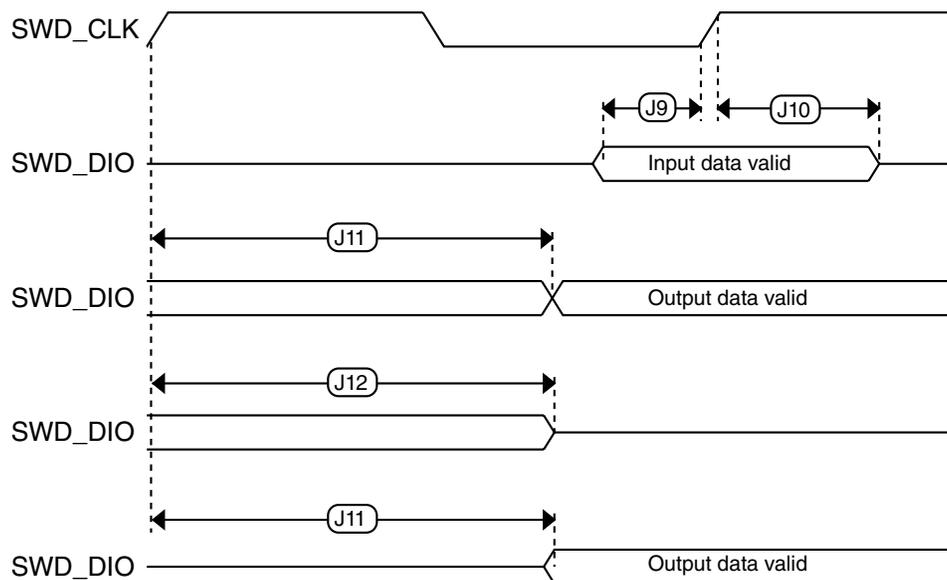
**Figure 14. Serial wire data timing**
