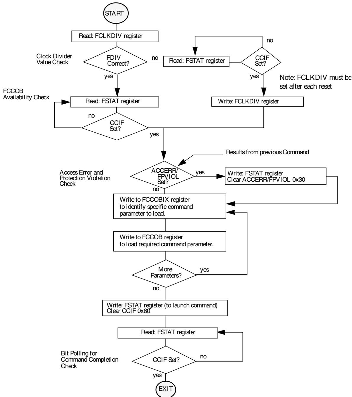
**Figure 18-1. Generic flash command write sequence flowchart**
