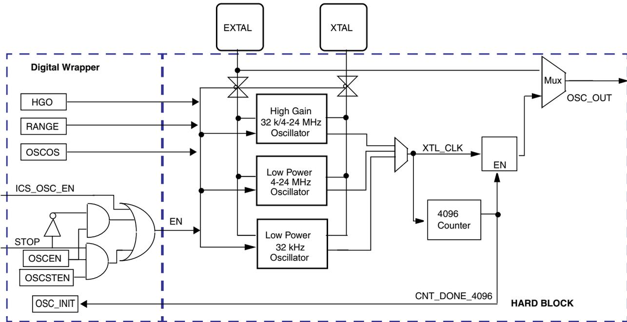
Figure 21-1. OSC module block diagram
