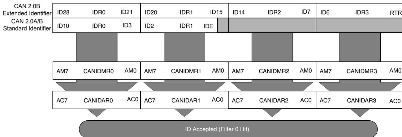
**Figure 32-5. 32-bit maskable identifier acceptance filter**
