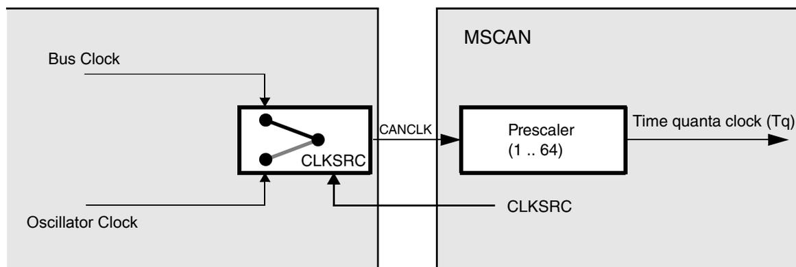
Figure 32-8. MSCAN clocking scheme
