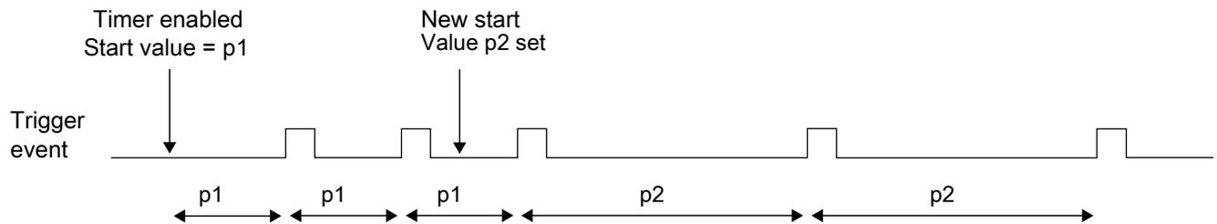
**Figure 28-4. Dynamically setting a new load value**
