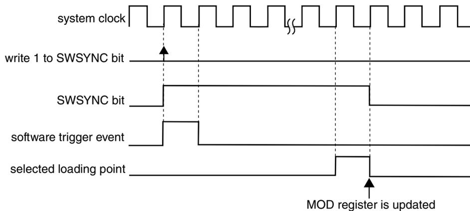
**Figure 26-49. MOD synchronization with (SYNCMODE = 0) and (PWMSYNC = 1)**
