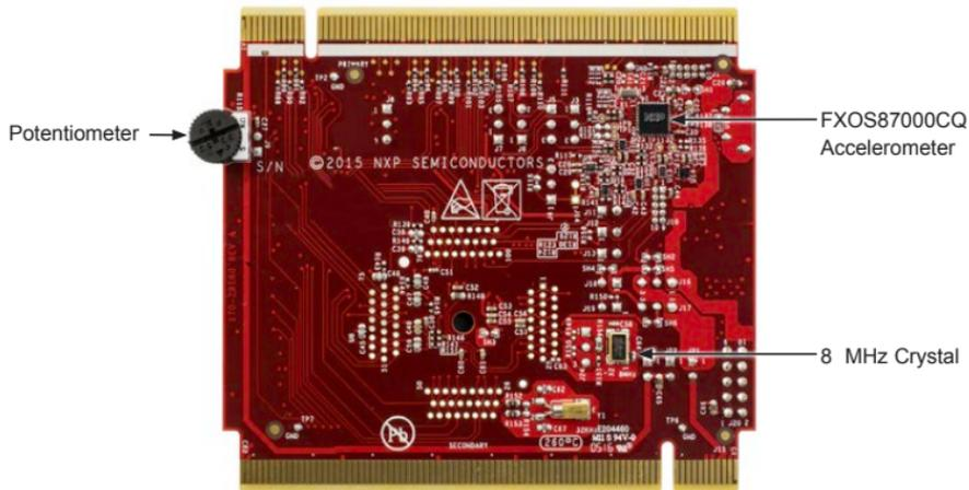
Figure 2: Back Side of TWR-KE18F
