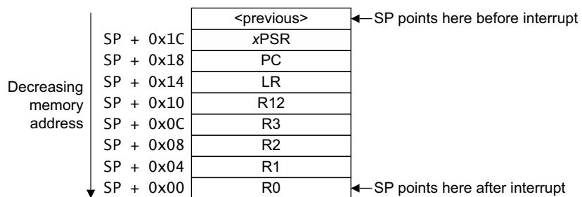
Immediately after stacking, the stack pointer indicates the lowest address in the stack frame. The stack frame is aligned to a double-word address.
