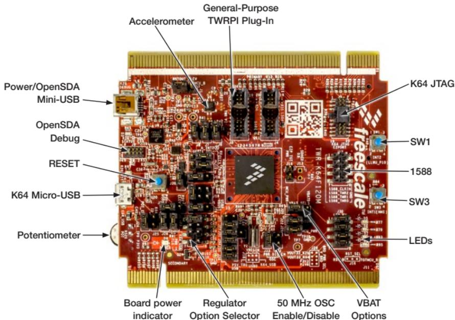
Figure 1: Front side of TWR-K64F120M
