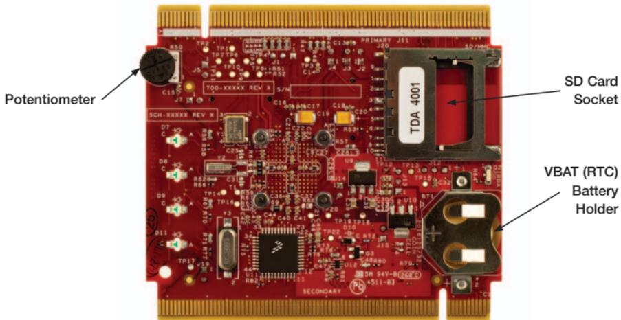
Figure 2: Back side of TWR-K60D100M module.
