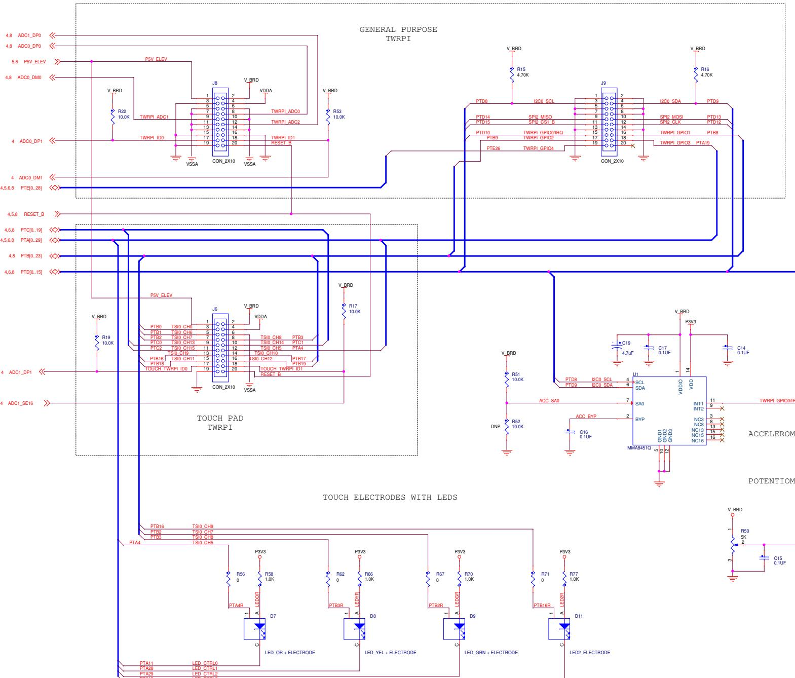
Note: The TWRPI connectors are powered by V\_BRD which may be 1.8V or 3.3V.
