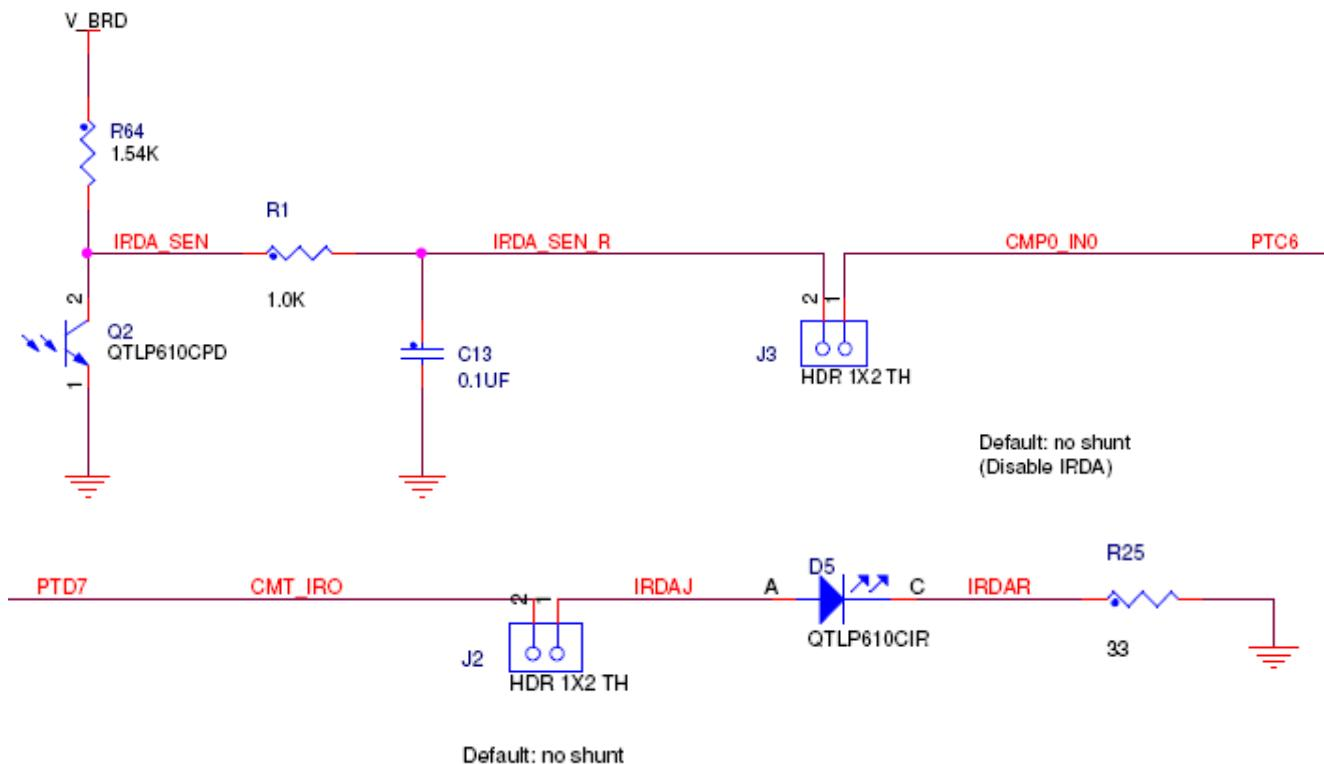
Figure 5. Infrared Port Implementation
