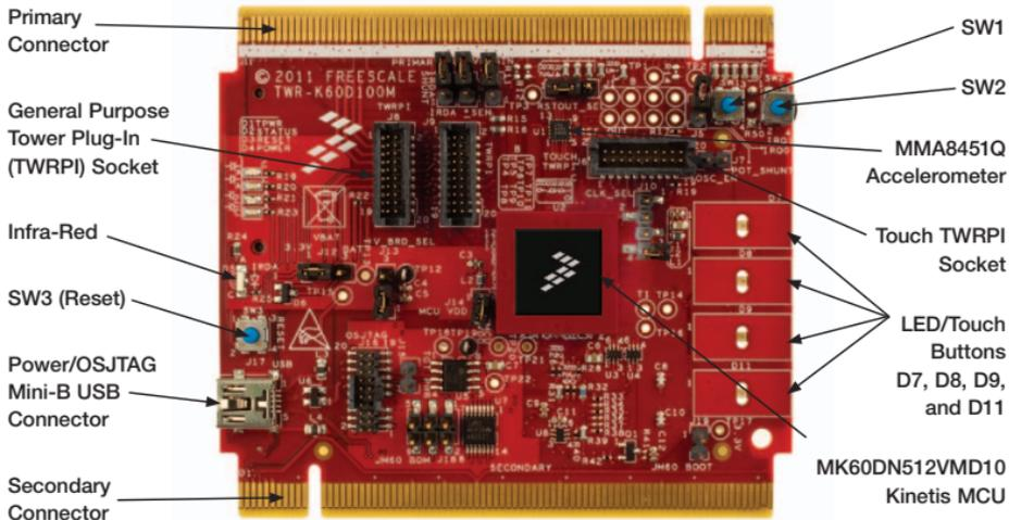
Figure 1: Front side of TWR-K60D100M module.
