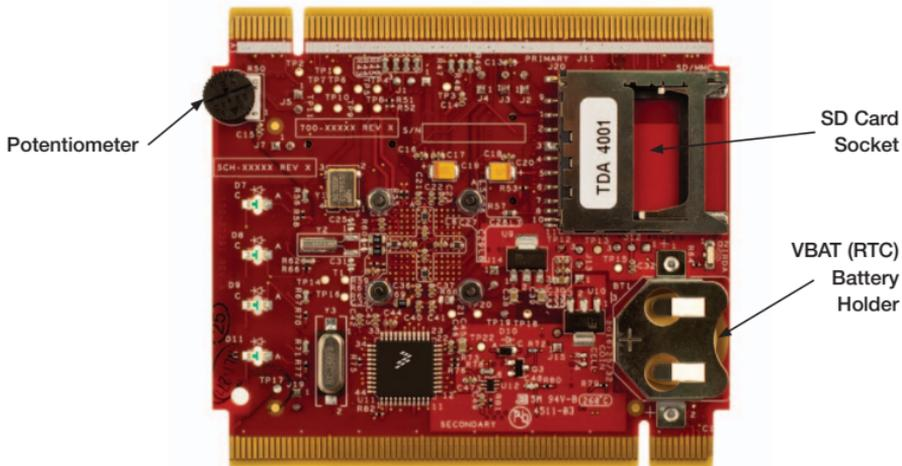
Figure 2: Back side of TWR-K60D100M module.
