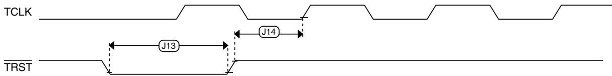
Figure 8.  $\overline{\text{TRST}}$  timing
