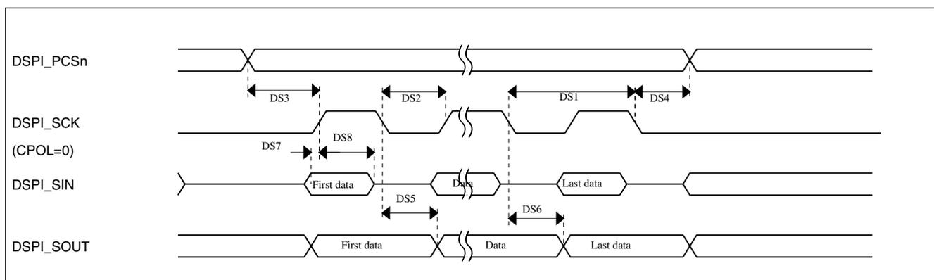
**Figure 22. DSPI classic SPI timing — master mode**
