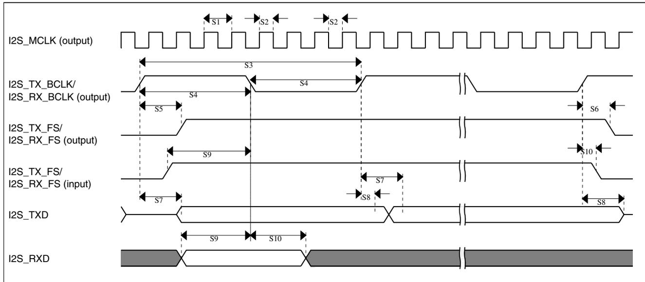
**Figure 32. I2S/SAI timing — master modes****Table 53. I2S/SAI slave mode timing in VLPR, VLPW, and VLPS modes (full voltage range)**
