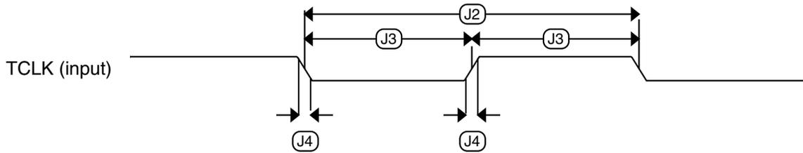
**Figure 5. Test clock input timing**
