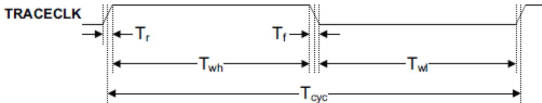
Figure 3. TRACE\_CLKOUT specifications
