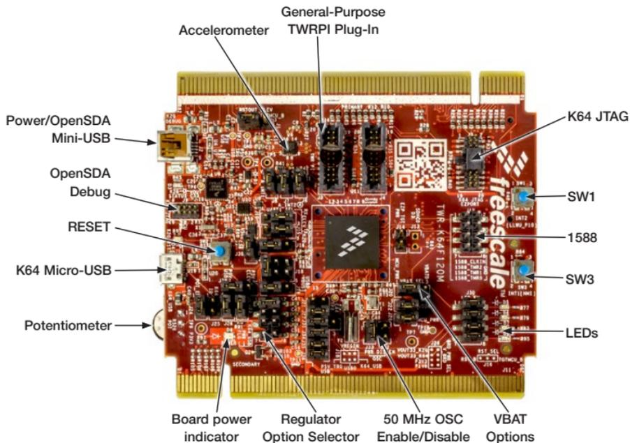
Figure 1: Front side of TWR-K64F120M
