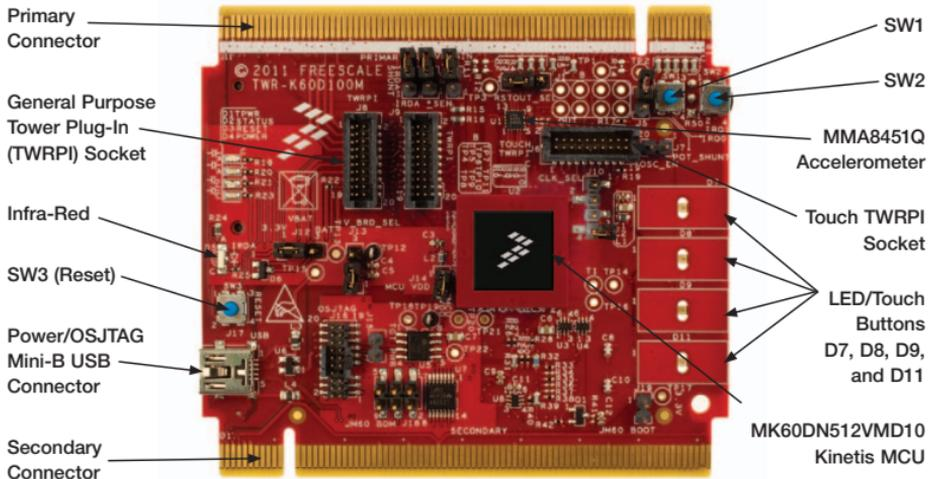
Figure 1: Front side of TWR-K60D100M module.
