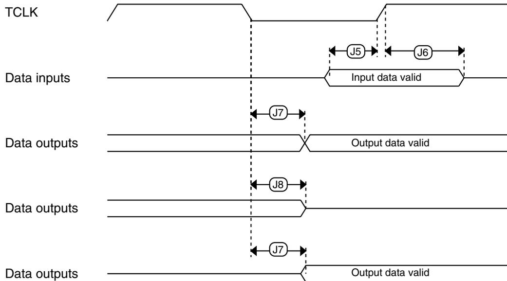
**Figure 6. Boundary scan (JTAG) timing**
