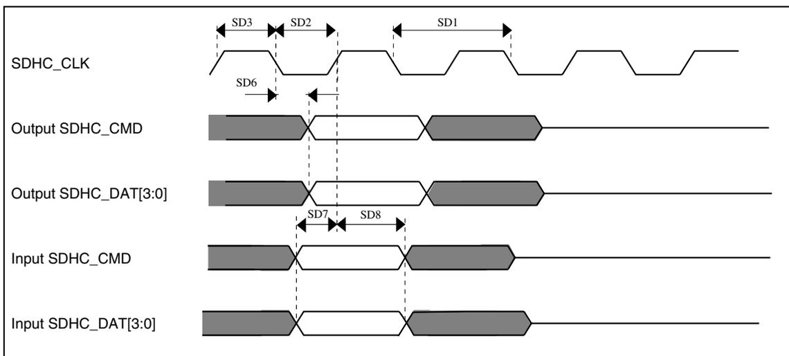
Figure 27. SDHC timing
