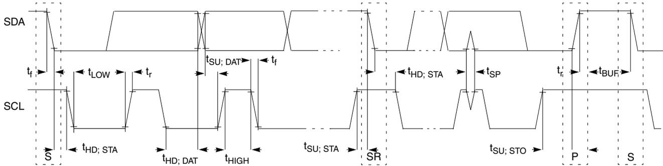
Figure 26. Timing definition for fast and standard mode devices on the I<sup>2</sup>C bus
