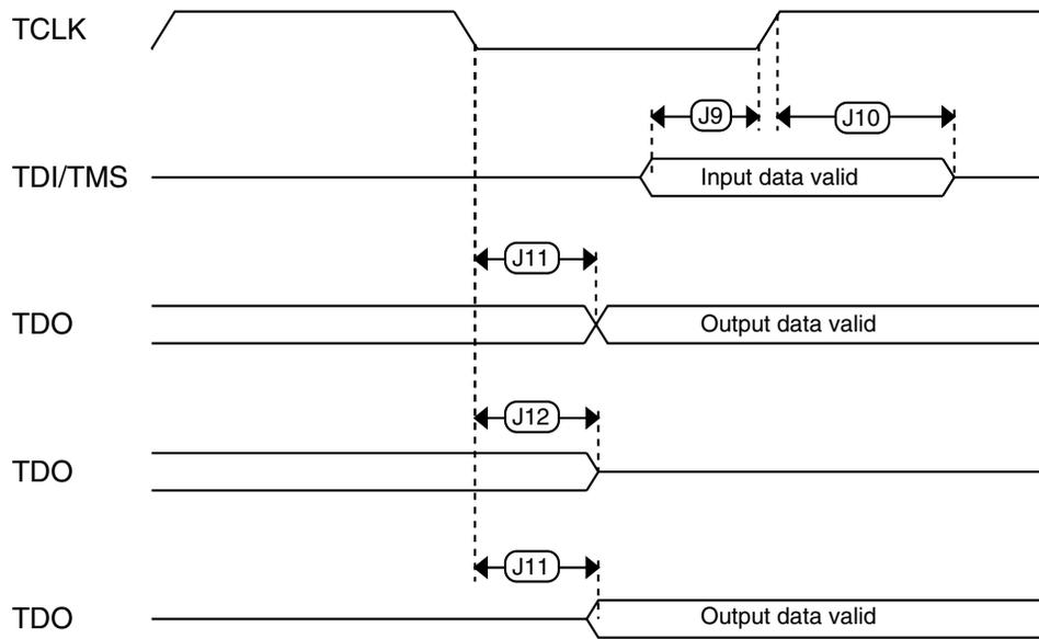
Figure 7. Test Access Port timing
