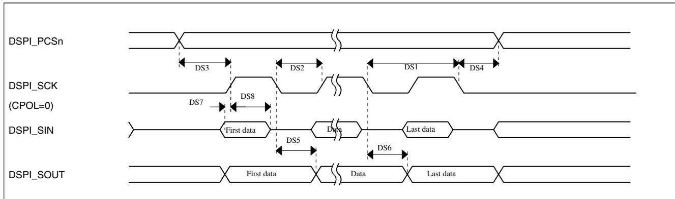
**Figure 24. DSPI classic SPI timing — master mode****Table 45. Slave mode DSPI timing (full voltage range)**
