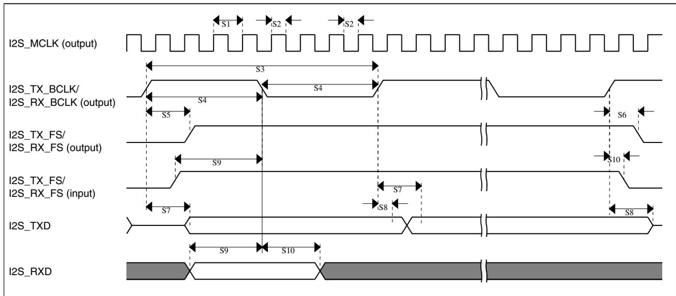
**Figure 28. I2S/SAI timing — master modes****Table 49. I2S/SAI slave mode timing in Normal Run, Wait and Stop modes (limited voltage range)**
