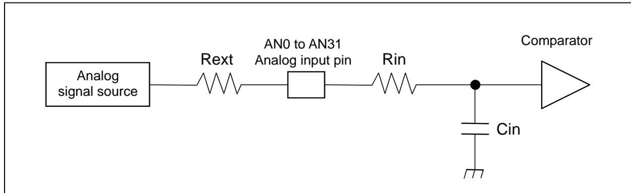
$$\text{(Equation 1) } T_s \geq (R_{in} + R_{ext}) \times C_{in} \times 9$$
