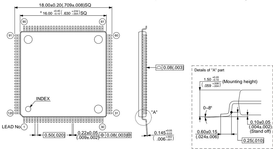
Note 1) \*: These dimensions do not include resin protrusion. Resin protrusion is +0.25(.010) MAX(each side).
