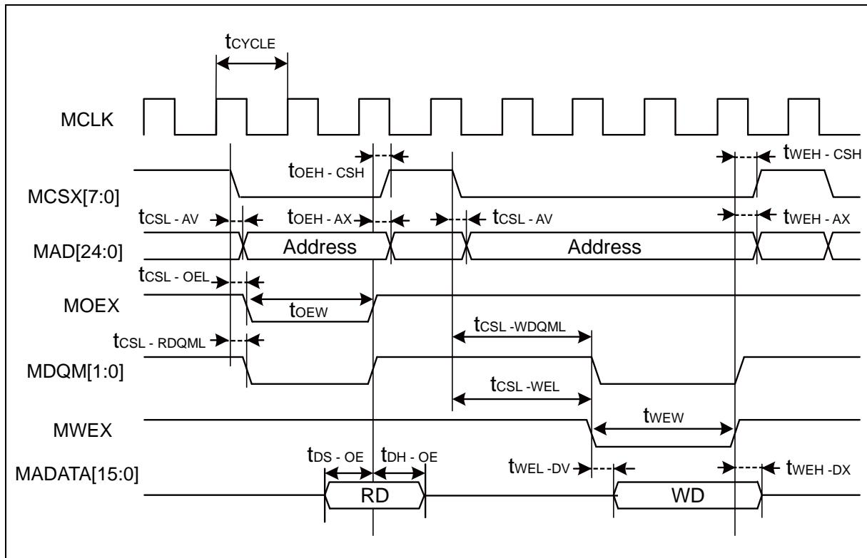
· Separate Bus Access Synchronous SRAM Mode
