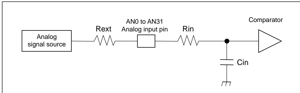
$$(Equation 1) \quad Ts \geq (Rin + Rext) \times Cin \times 9$$
