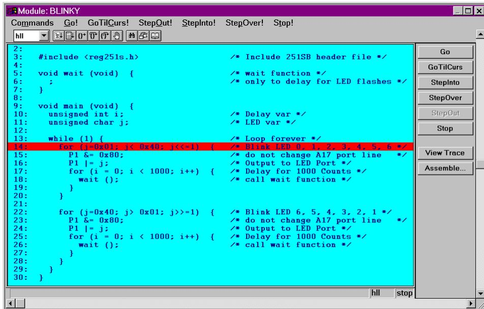
You may now single step through the BLINKY program by clicking on the StepOver button on the right side of the module window. As you step through the program, you should see the LEDs on the MCB251 changing.
