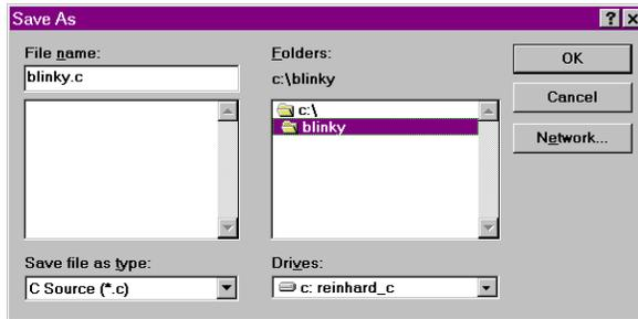
To save the program as BLINKY.C, enter BLINKY.C in the File Name text box at the top of the Save As dialog box. You may want to save the flash program and the other files you create in a separate directory. This example uses C:\BLINKY for the source files and project files.
