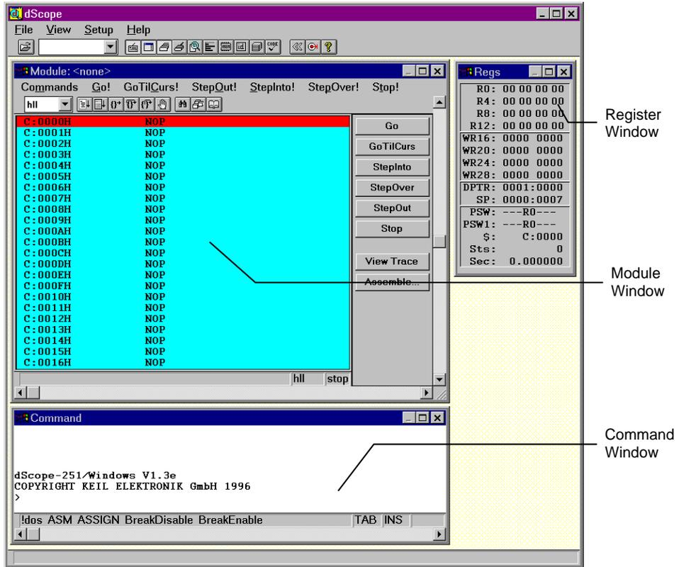
To load the MON251.DLL CPU driver, type the following in the command window.
