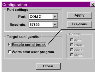
Set Enable serial break to let dScope stop programs running on the MCB251.
