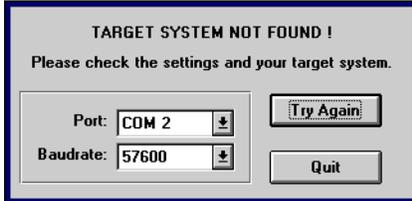
When using the MCB251 evaluation board, the baud rate should be set for 57,600 baud. You must determine which COM port you use.
