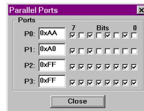
As you step through the BLINKY program, you will see how the Parallel Ports dialog box mirrors the LEDs on the MCB251 evaluation board.
