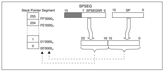
Figure 2-20 Addressing via the Stack Pointer
