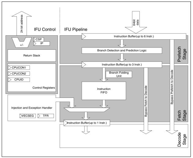
Figure 2-2 IFU Block Diagram
