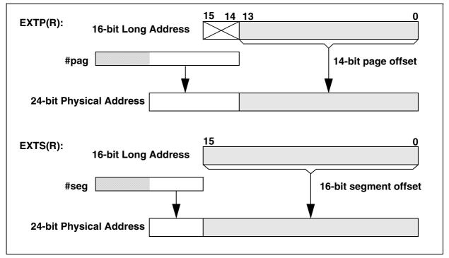
Figure 2-16 Overriding the DPP Mechanism
