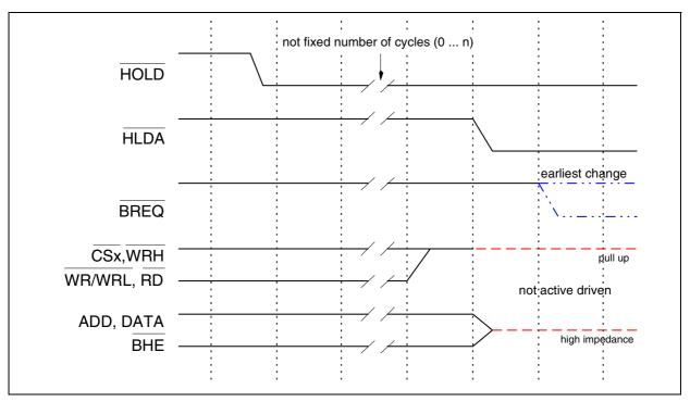
Figure 6-8 Releasing the Bus by the Arbitration Master
