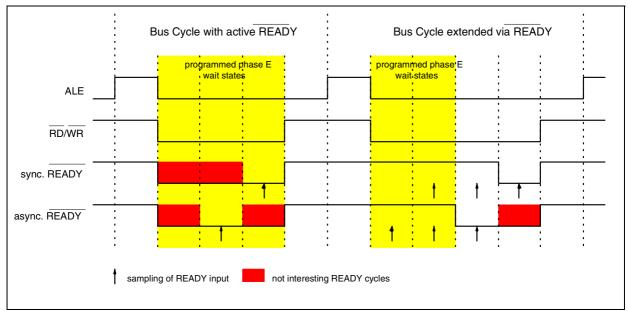
Figure 6-7 Ready controlled bus cycles
