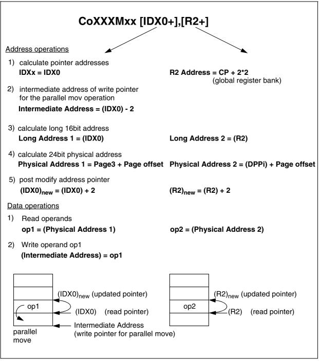
Figure 2-19 Arithmetic MAC Operations with Parallel Move
