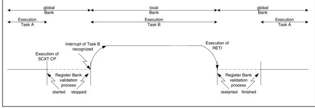
Note: Validation Process and Hardware Interrupts using a Local Register Bank
