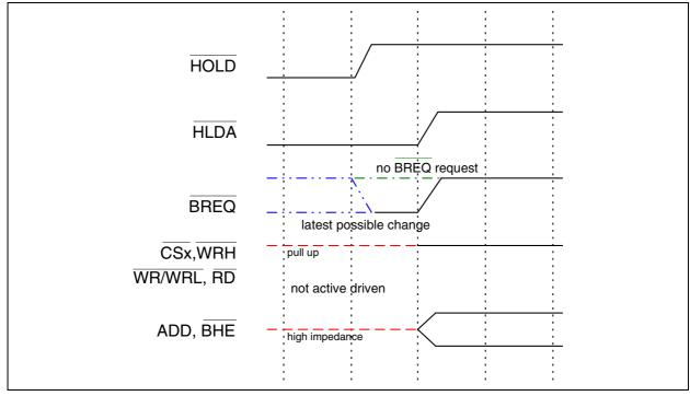
Figure 6-9 Regaining the Bus by the Arbitration Master
