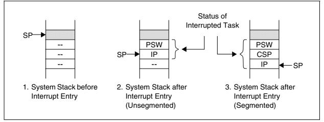
Figure 5-3 Task Status Saved on the System Stack
