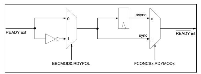
Figure 6-6 External to internal READY conversion
