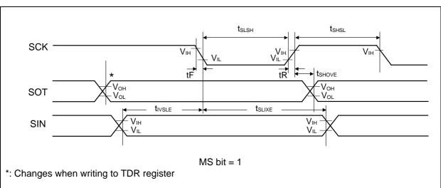
• Synchronous serial (SPI = 1, SCINV = 1)
