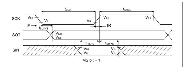
• Synchronous serial (SPI = 0, SCINV = 1)
