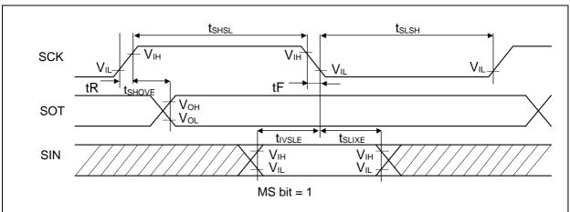
• Synchronous serial (SPI = 1, SCINV = 0)
