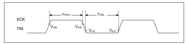
· Trigger input timing
