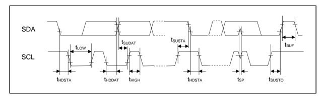
$<sup>*2:</sup> The \ maximum \ t_{HDDAT} \ must \ satisfy \ that \ it \ does \ not \ extend \ at \ least \ "L" \ period \ (t_{LOW}) \ of \ device's \ SCL \ signal.$
