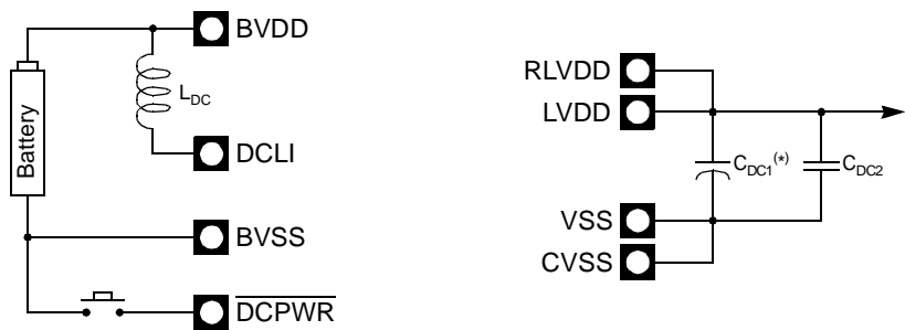
Figure 8. Battery DC-DC Connection
