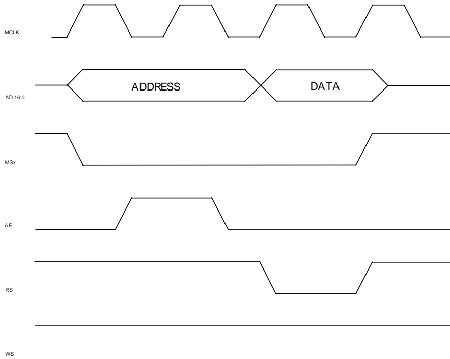
Figure 34: External Memory Read Cycle
