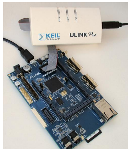
The SAMV71 Xplained Ultra board connected to a Keil ULINK pro . This lab uses the onboard Atmel EDBG.
