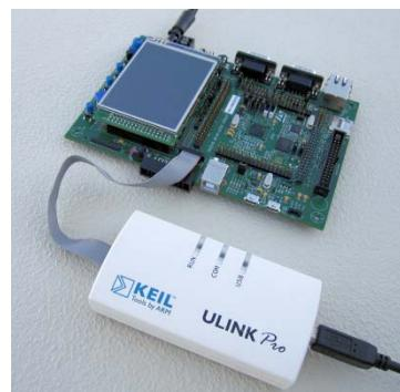
A STM3240G-EVAL board connected to a ULINKpro using the special CoreSight 20 pin ETM connector:
