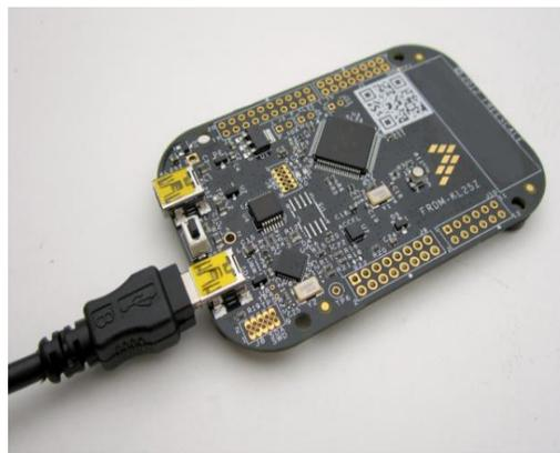
The Freedom KL25Z board connected to run OpenSDA (CMSIS-DAP) and MDK.
