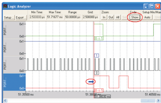
Logic Analyzer window showing signals after glitch correction
