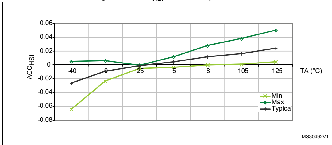
Figure 26. ACC HSI versus temperature
