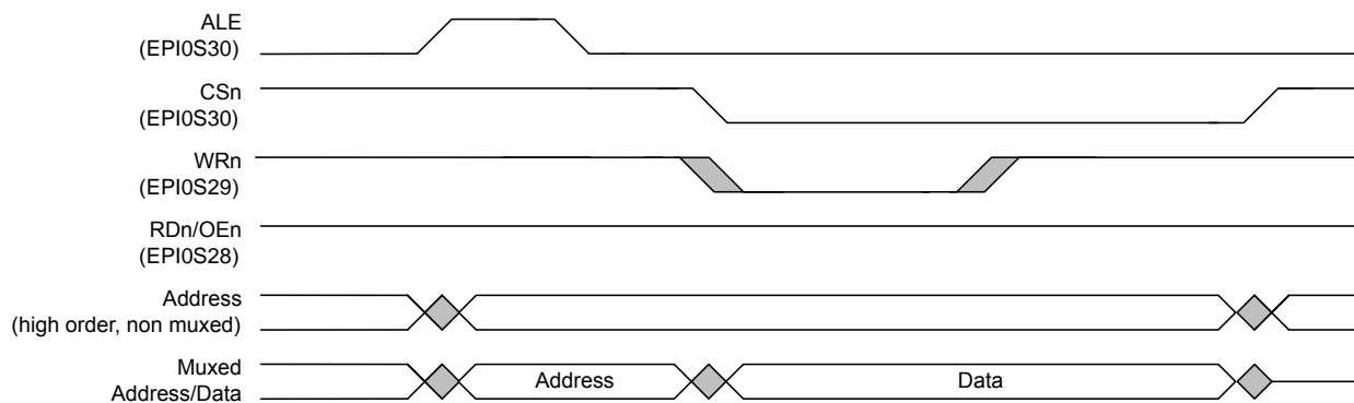
Figure 11-7. Host-Bus Write Cycle with Multiplexed Address and Data, MODE = 0x0, WRHIGH = 1, RDHIGH = 1
