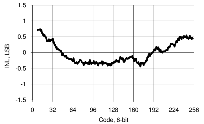
Figure 11-26. IDAC INL vs Input Code, Range = 255 \mu A, Sink Mode
