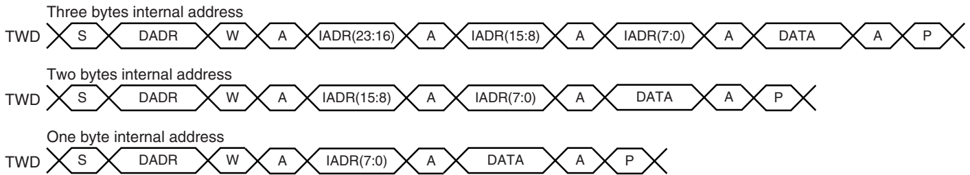
Figure 23-5. Master Write with One, Two or Three Bytes Internal Address and One Data Byte
