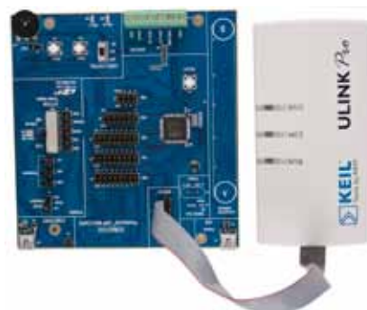
ULINKpro connects to SiLab UDP MCU card via ETM
