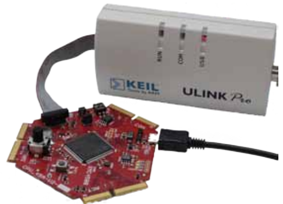
ULINKpro supports the XMC4000 family and enables instruction trace via ETM.
