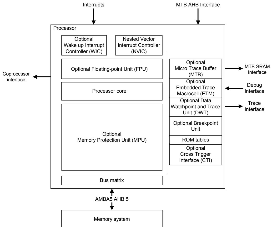
Figure 1-1 Cortex-M33 processor implementation without the Security Extension
