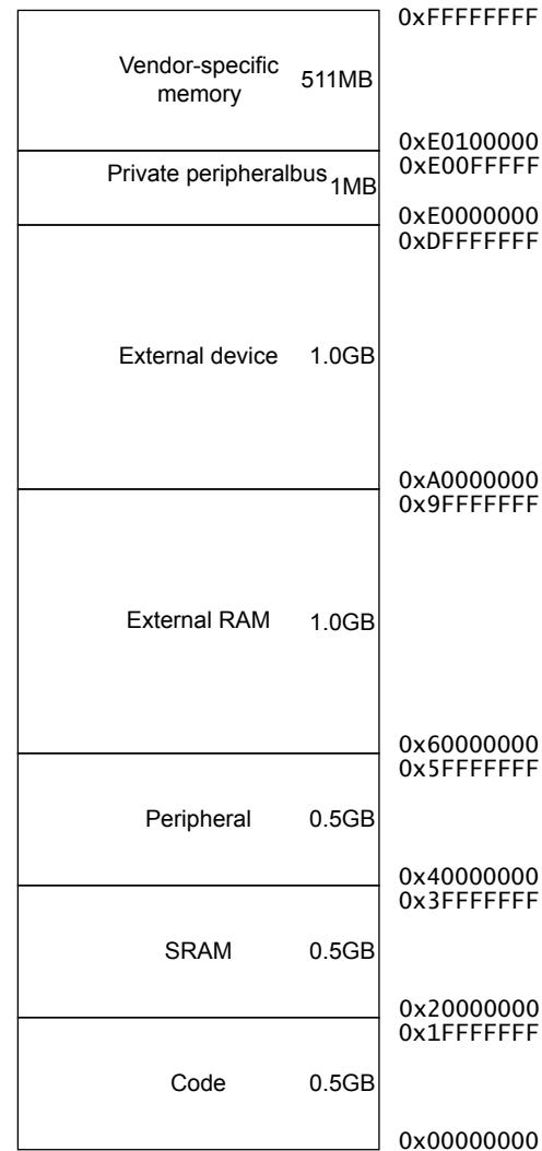
**Figure 2-3 Cortex-M33 processor memory map**
