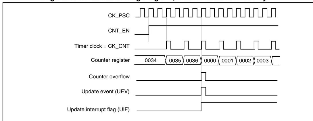
Figure 135. Counter timing diagram, internal clock divided by 4
