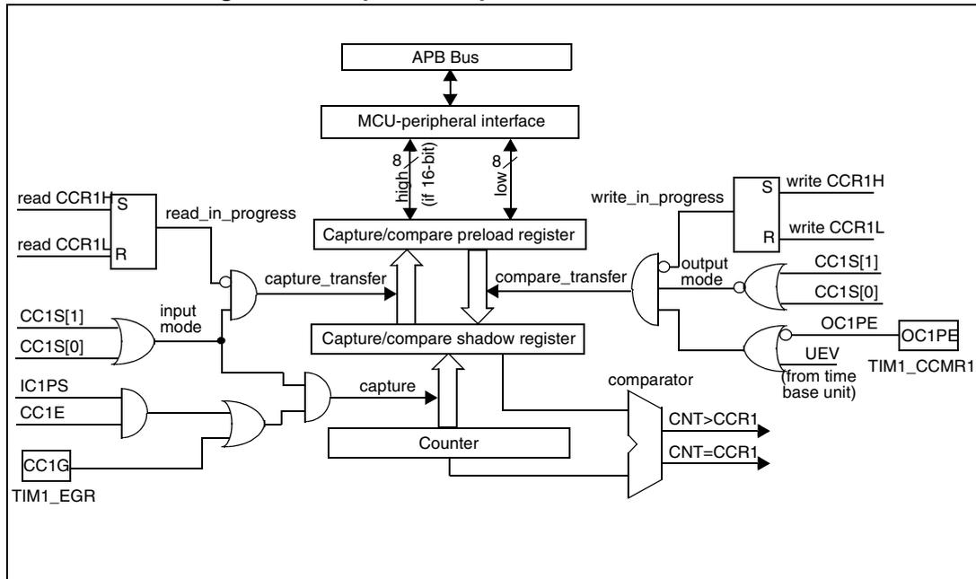
Figure 144. Output stage of capture/compare channel (channel 1)
