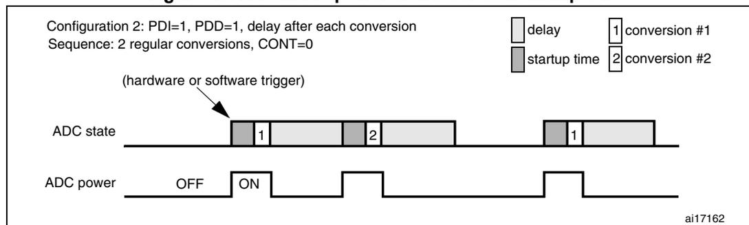
Figure 49. Automatic power-down control: example 3
