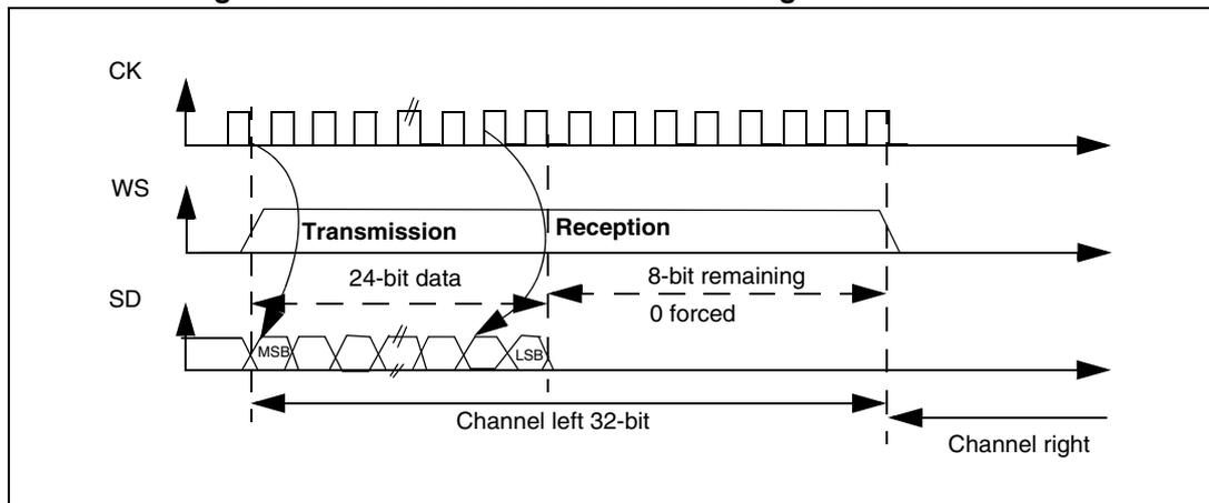
Figure 263. MSB Justified 16-bit extended to 32-bit packet frame with CPOL = 0
