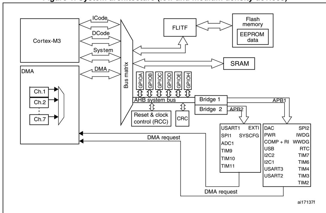
Figure 2. System architecture (medium+ density devices)
