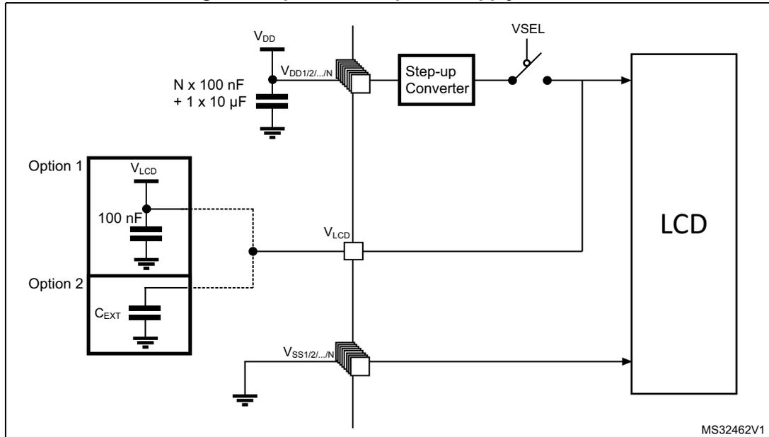
1. Option 1: LCD power supply is provided by a dedicated VLCD supply source, VSEL switch is open.
