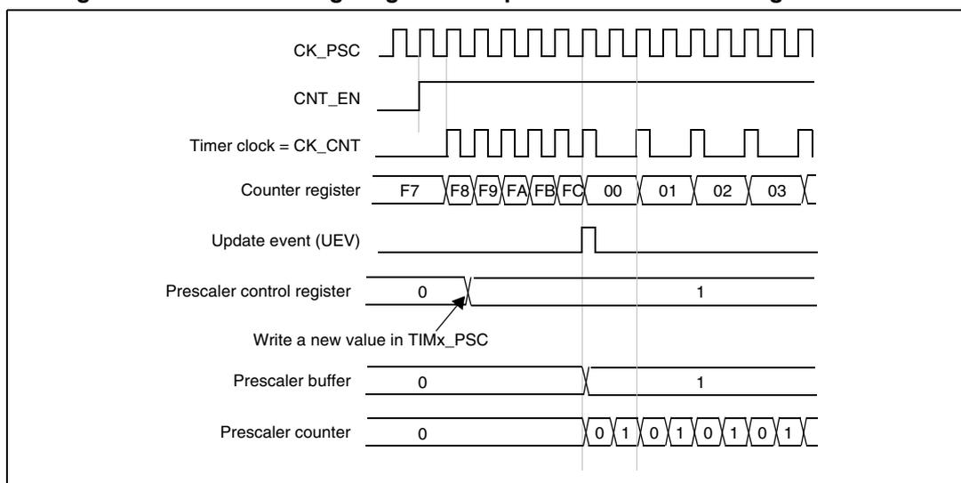
Figure 84. Counter timing diagram with prescaler division change from 1 to 4
