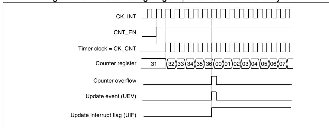
**Figure 156. Counter timing diagram, internal clock divided by 2**
