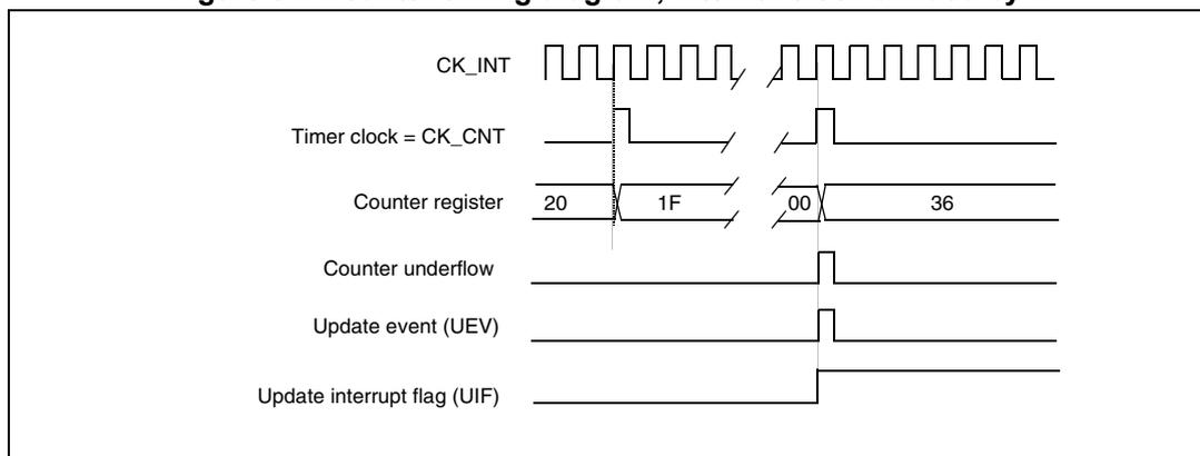
**Figure 95. Counter timing diagram, Update event**
