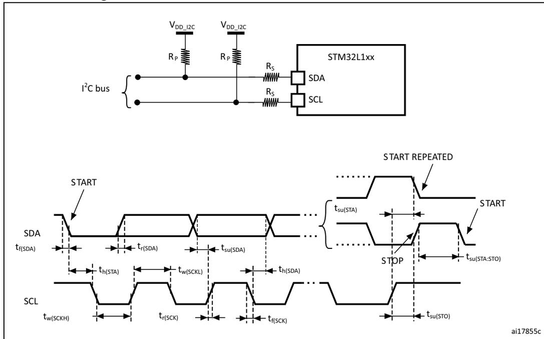
1.  $R_S$  = series protection resistor.
