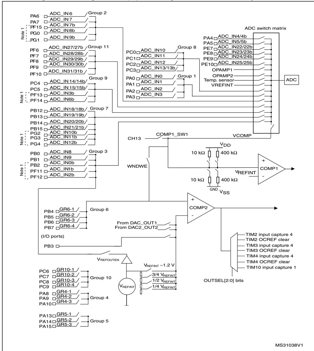
Figure 24. Routing interface (RI) block diagram for high-density devices
