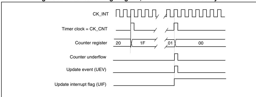
**Figure 100. Counter timing diagram, Update event with ARPE=1 (counter underflow)**
