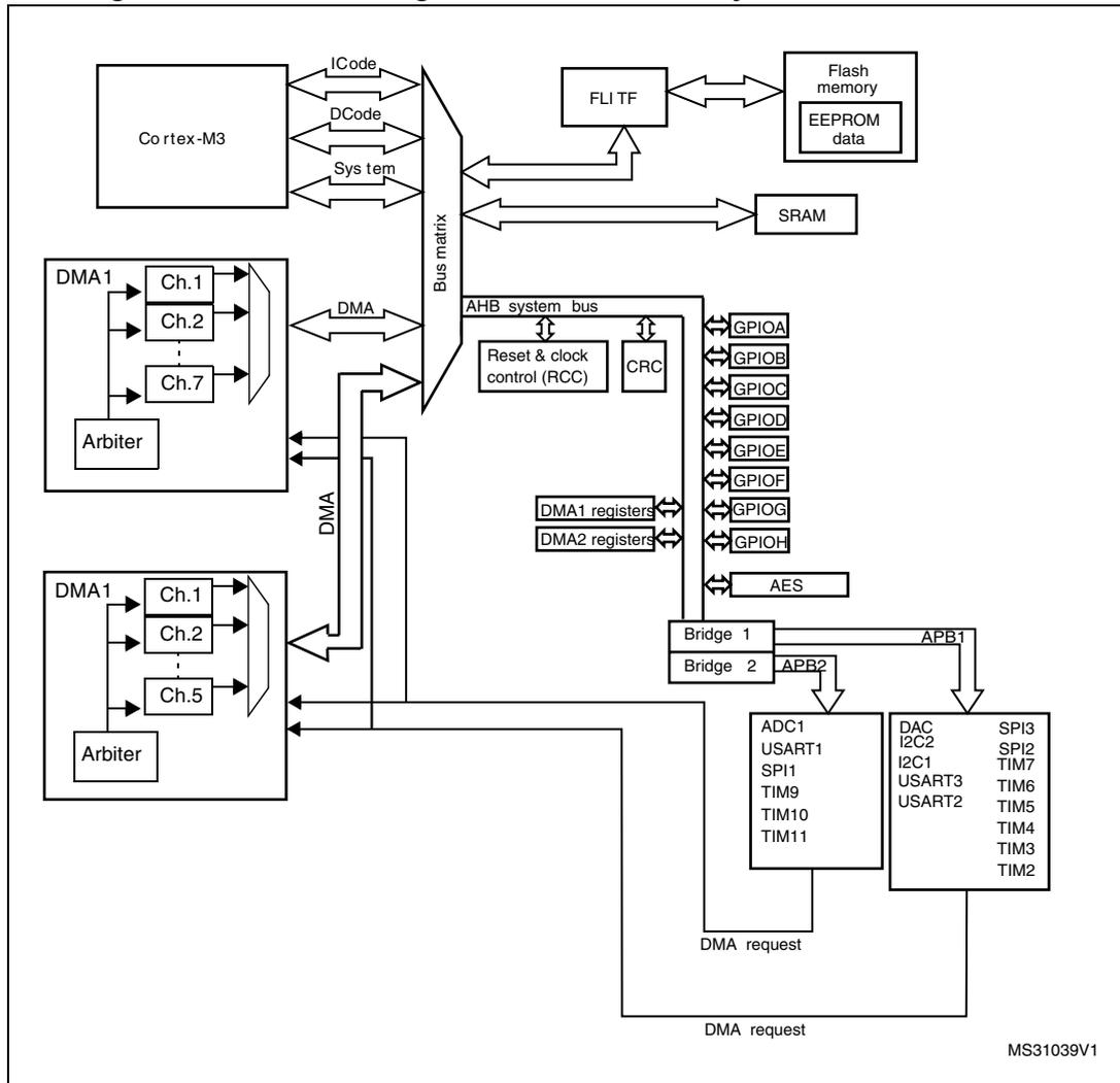
Figure 33. DMA block diagram in high-density STM32L1xxx devices
