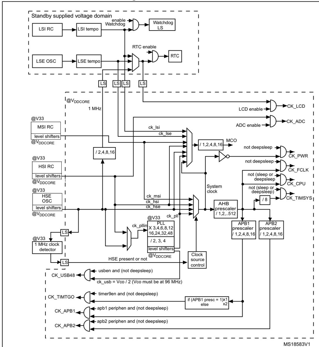
1. For the USB function to be available, both HSE and PLL must be enabled, with the CPU running at either 24 MHz or 32 MHz.
