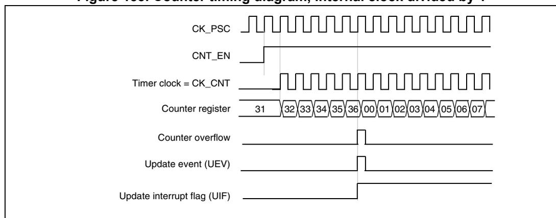
**Figure 134. Counter timing diagram, internal clock divided by 2**
