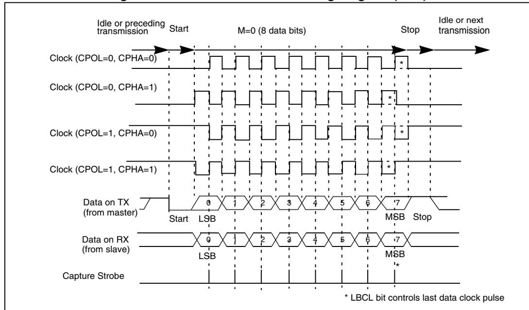
Figure 226. USART data clock timing diagram (M=1)
