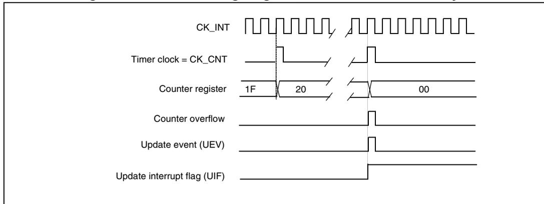
Figure 89. Counter timing diagram, Update event when ARPE=0 (TIMx\_ARR not preloaded)
