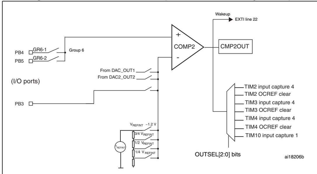
**Figure 64. COMP2 interconnections (high and medium+ density devices)**
