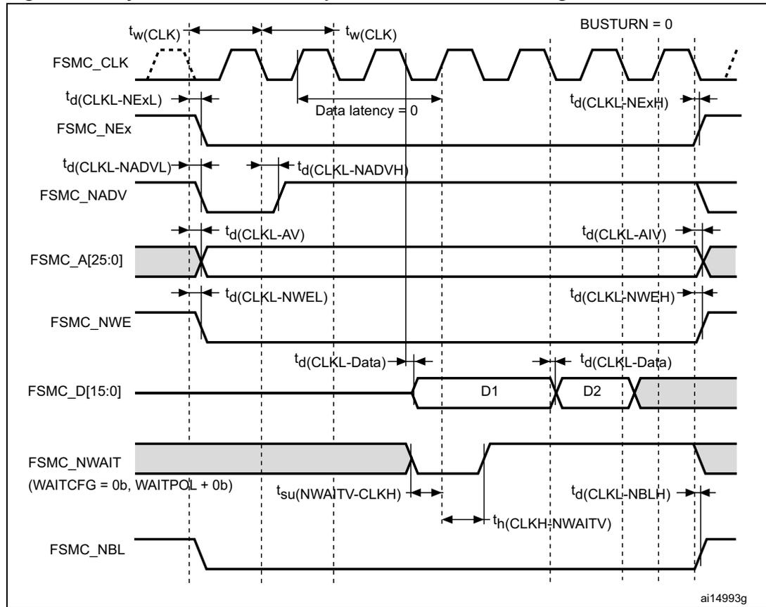
Table 44. Synchronous non-multiplexed PSRAM write timings<sup>(1)</sup>
