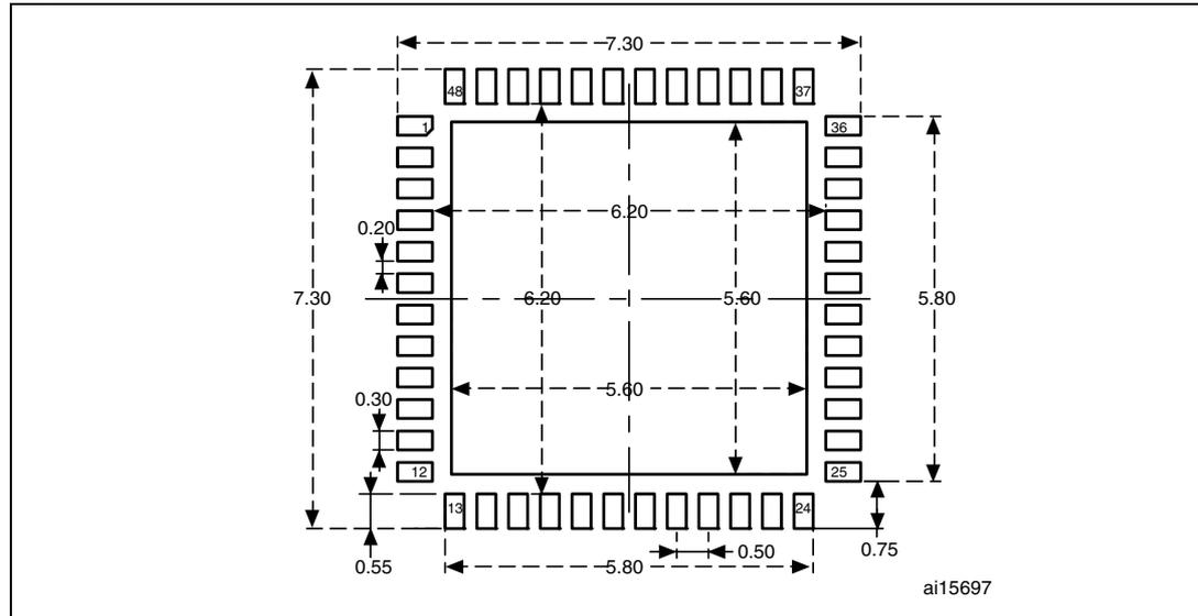
1. Dimensions are in millimeters.
