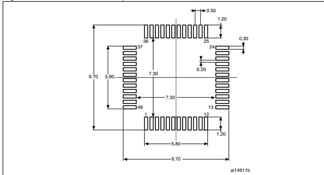
1. Dimensions are in millimeters.
