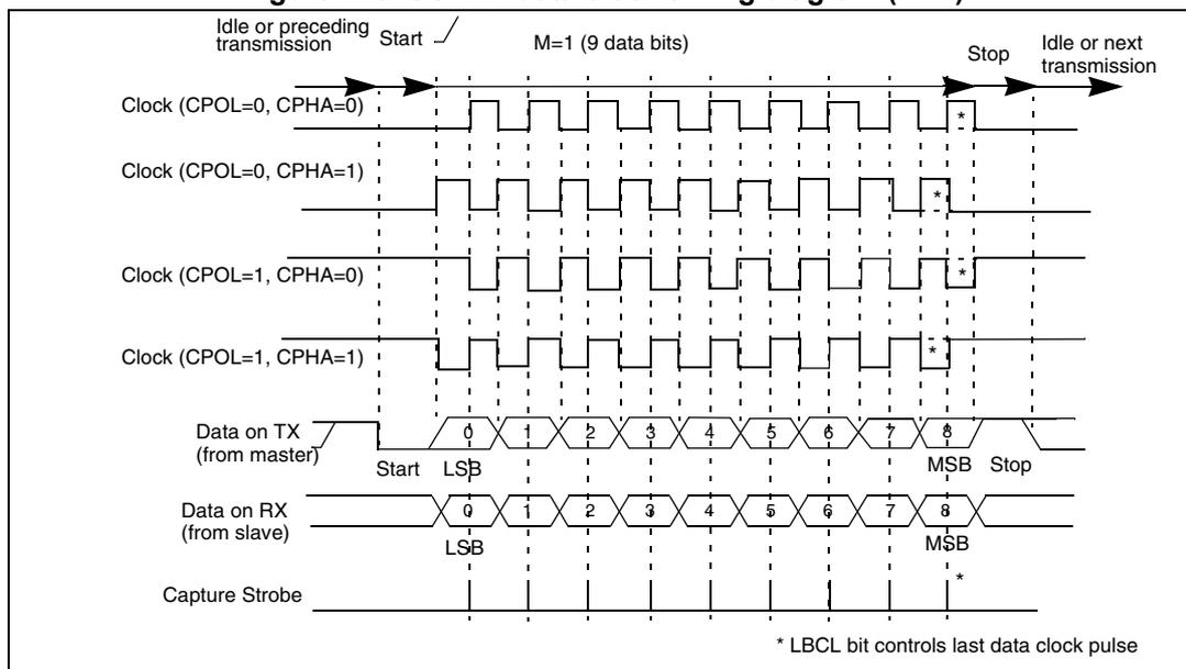
Figure 227. RX data setup/hold time
