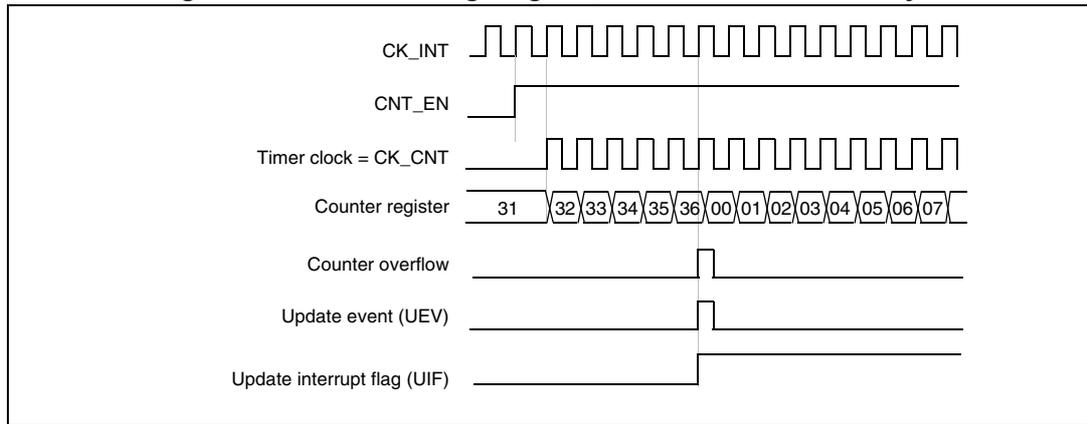
**Figure 86. Counter timing diagram, internal clock divided by 2**
