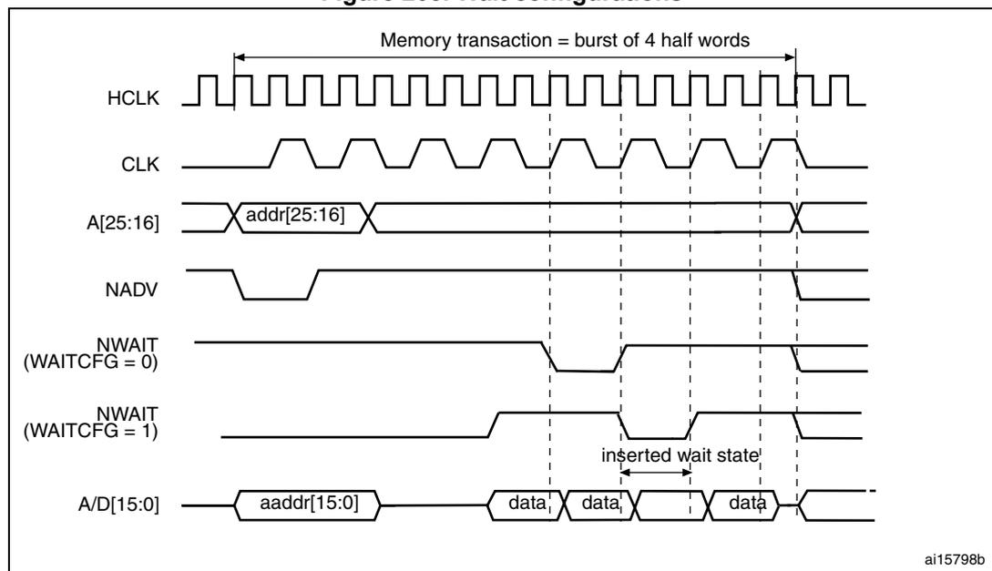
Figure 204. Synchronous multiplexed read mode - NOR, PSRAM (CRAM)
