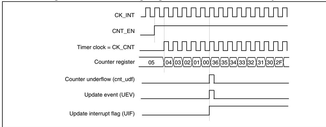
**Figure 92. Counter timing diagram, internal clock divided by 2**
