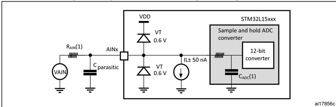
1. Refer to [Table 56: RAIN max for fADC = 16 MHz](#) for the value of  $R_{\text{AIN}}$  and [Table 54: ADC characteristics](#) for the value of  $C_{\text{ADC}}$ .
