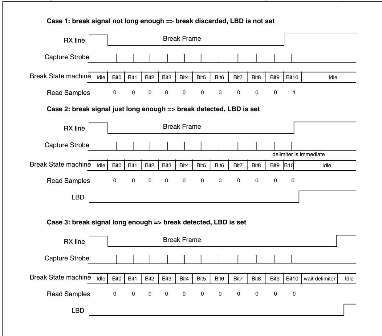
**Figure 223. Break detection in LIN mode vs. Framing error detection**
