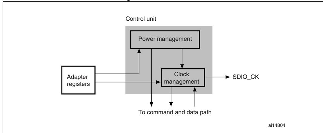
The control unit is illustrated in [Figure 281](#). It consists of a power management subunit and a clock management subunit.
