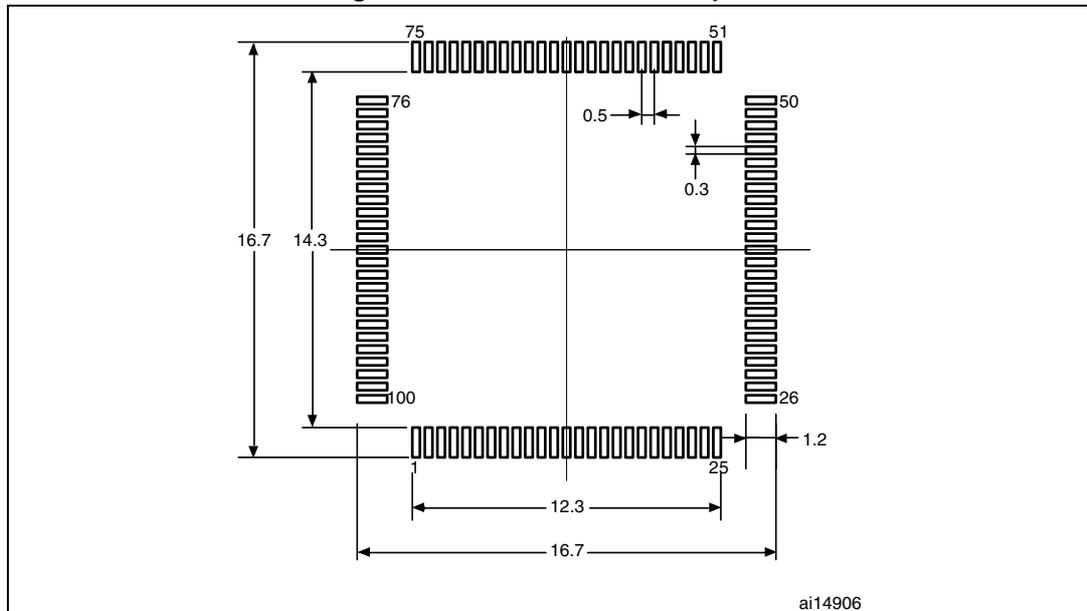
1. Dimensions are in millimeters.
