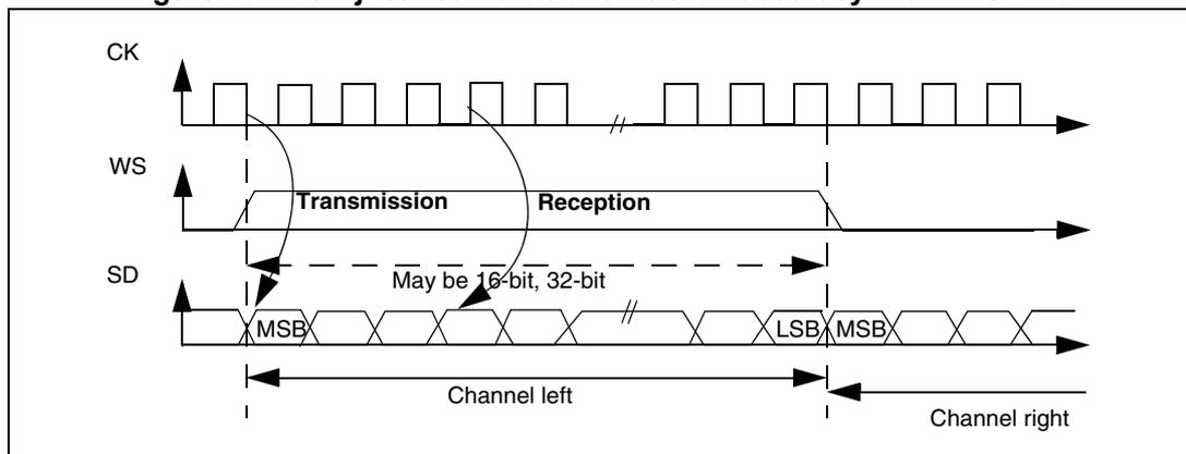
Figure 265. LSB Justified 24-bit frame length with CPOL = 0
