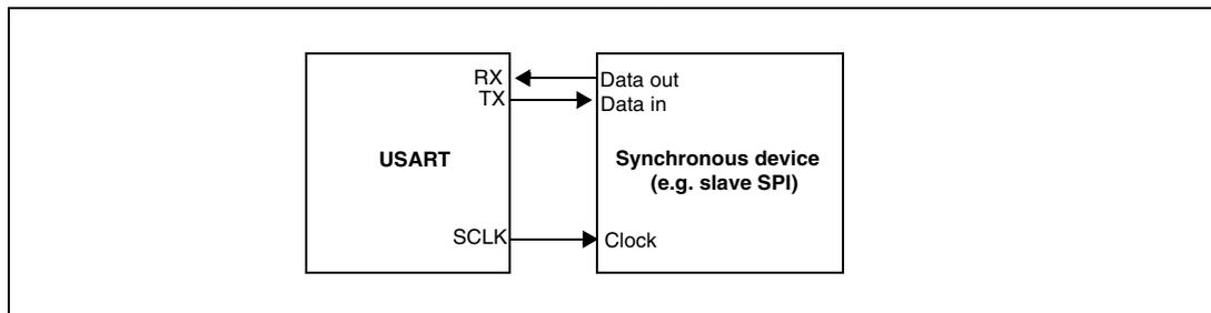
Figure 225. USART data clock timing diagram (M=0)
