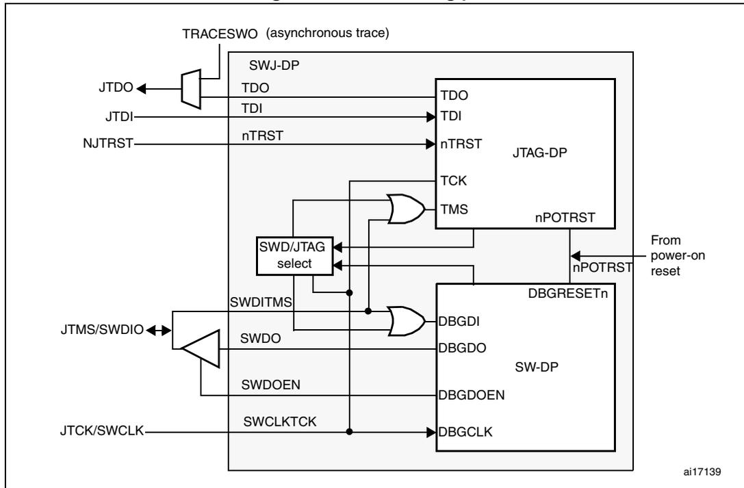
Figure 288 shows that the asynchronous TRACE output (TRACESWO) is multiplexed with TDO. This means that the asynchronous trace can only be used with SW-DP, not JTAG-DP.
