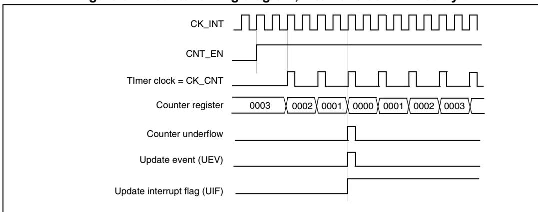
**Figure 98. Counter timing diagram, internal clock divided by 4, TIMx\_ARR=0x36**
