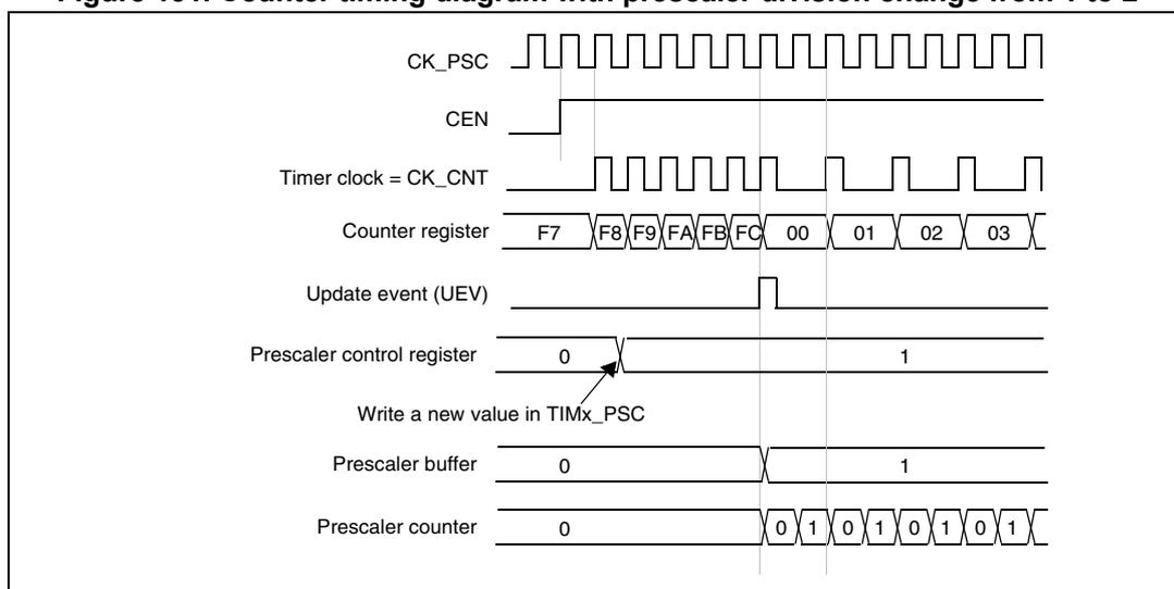
**Figure 132. Counter timing diagram with prescaler division change from 1 to 4**
