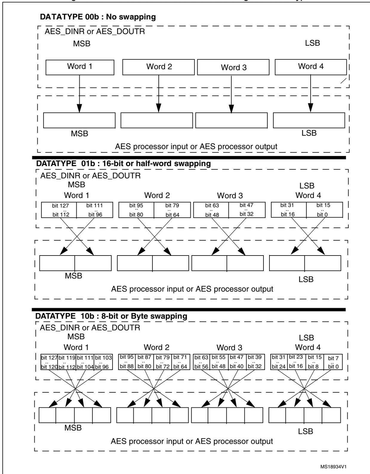
Figure 177. 128-bit block construction according to the data type (continued)
