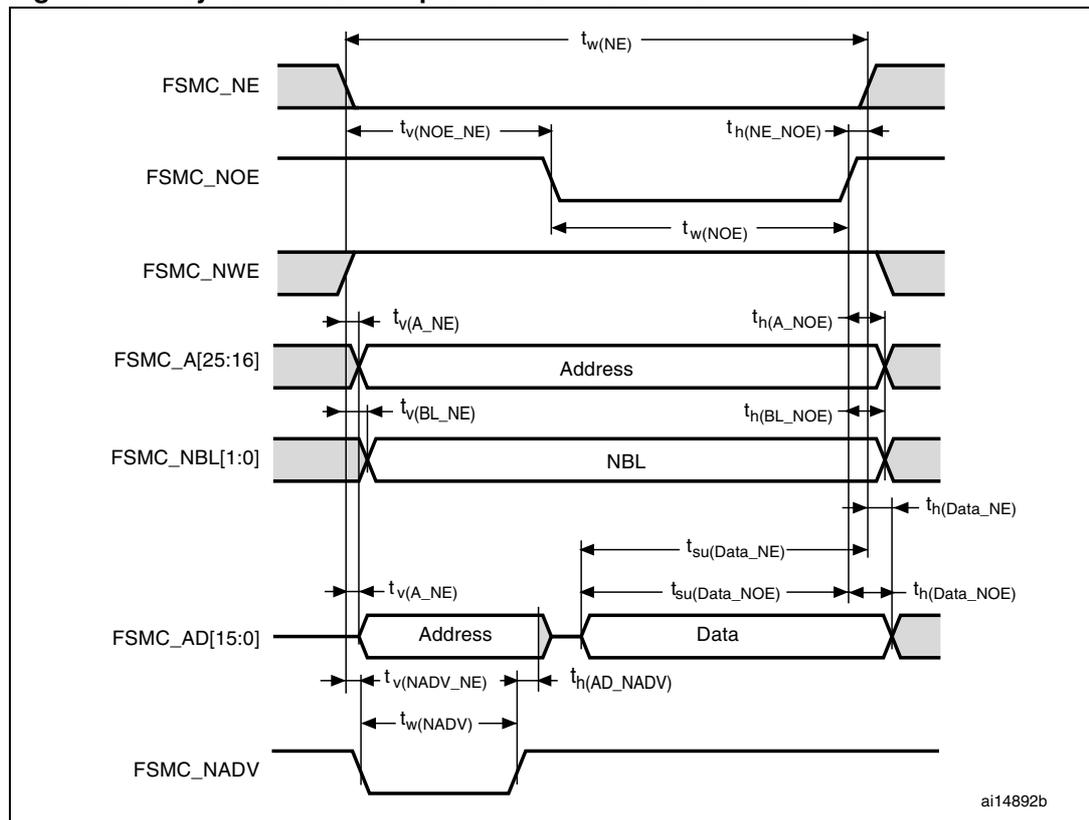
**Table 39. Asynchronous multiplexed PSRAM/NOR read timings<sup>(1)</sup>**
