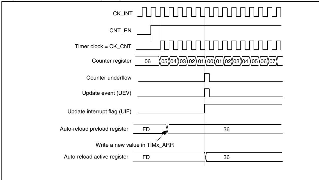
**Figure 101. Counter timing diagram, Update event with ARPE=1 (counter overflow)**
