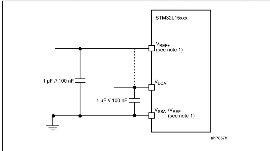
1.  $V_{REF+}$  and  $V_{REF-}$  inputs are available only on 100-pin packages.
