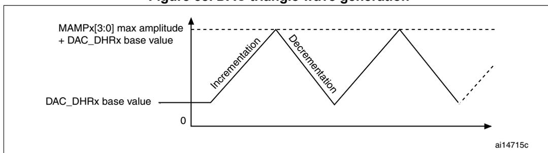
Figure 59. DAC conversion (SW trigger enabled) with triangle wave generation
