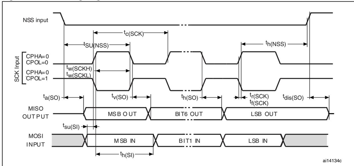
Figure 22. SPI timing diagram - slave mode and CPHA = 1<sup>(1)</sup>
