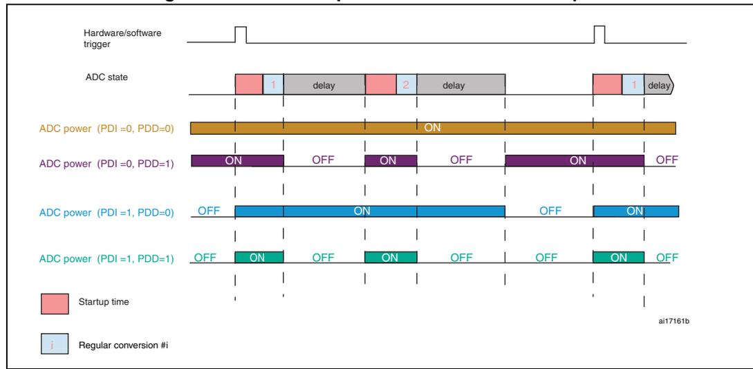
**Figure 48. Automatic power-down control: example 2**
