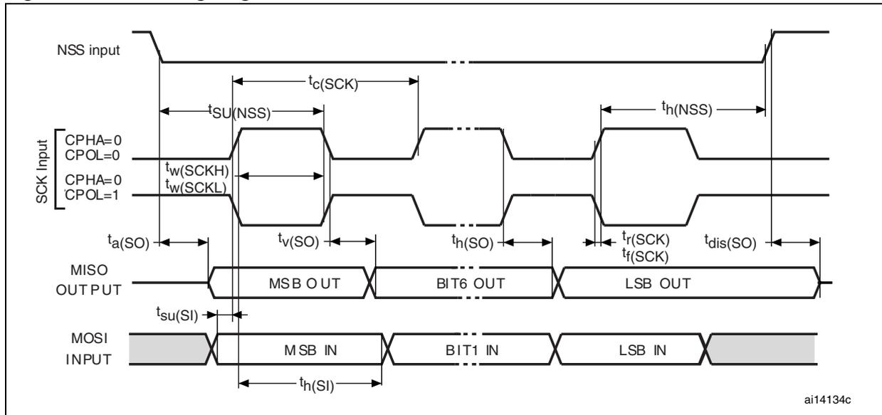
Figure 25. SPI timing diagram - slave mode and CPHA = 1<sup>(1)</sup>
