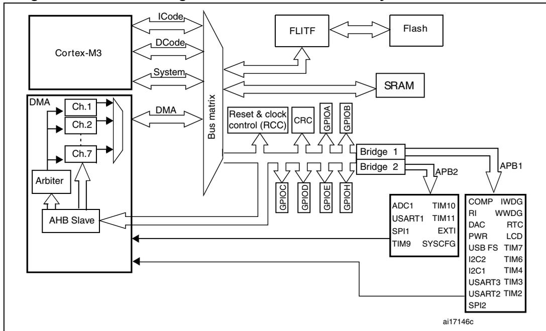
Figure 32. DMA block diagram in medium+ density STM32L1xxx devices
