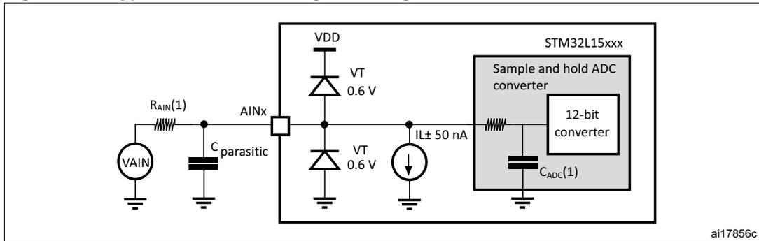
1. Refer to [Table 56:  \$R\_{\text{AIN}}\$  max for  \$f\_{\text{ADC}} = 16 \text{ MHz}\$](#)  for the value of  $R_{\text{AIN}}$  and [Table 54: ADC characteristics](#) for the value of  $C_{\text{ADC}}$
