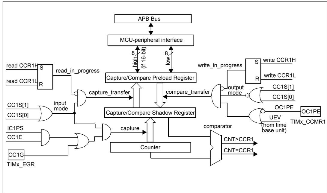
Figure 109. Output stage of capture/compare channel (channel 1)
