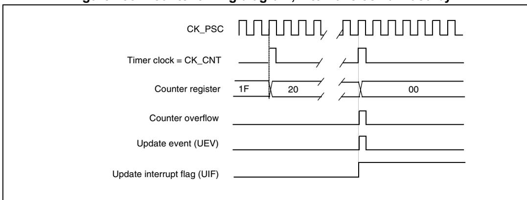
Figure 137. Counter timing diagram, update event when ARPE=0 (TIMx\_ARR not preloaded)
