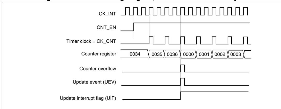
**Figure 87. Counter timing diagram, internal clock divided by 4**
