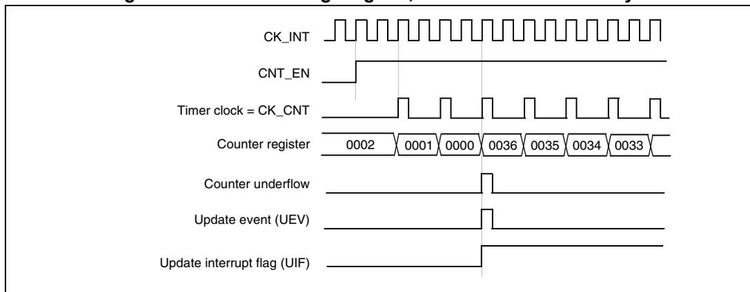
**Figure 93. Counter timing diagram, internal clock divided by 4**
