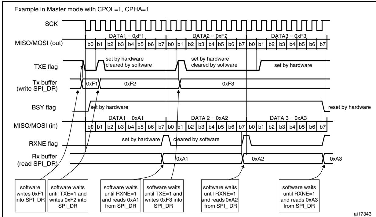
**Figure 246. TXE/RXNE/BSY behavior in Slave / full-duplex mode (BIDIMODE=0, RXONLY=0) in the case of continuous transfers**
