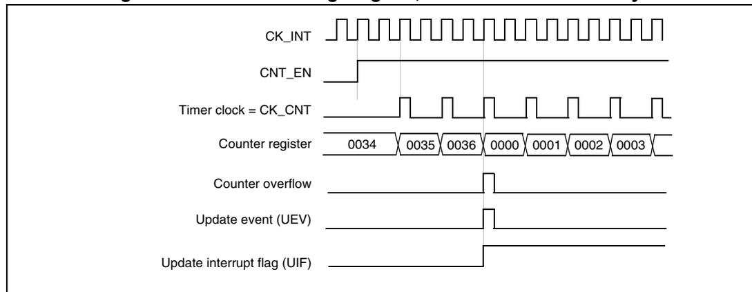
**Figure 157. Counter timing diagram, internal clock divided by 4**
