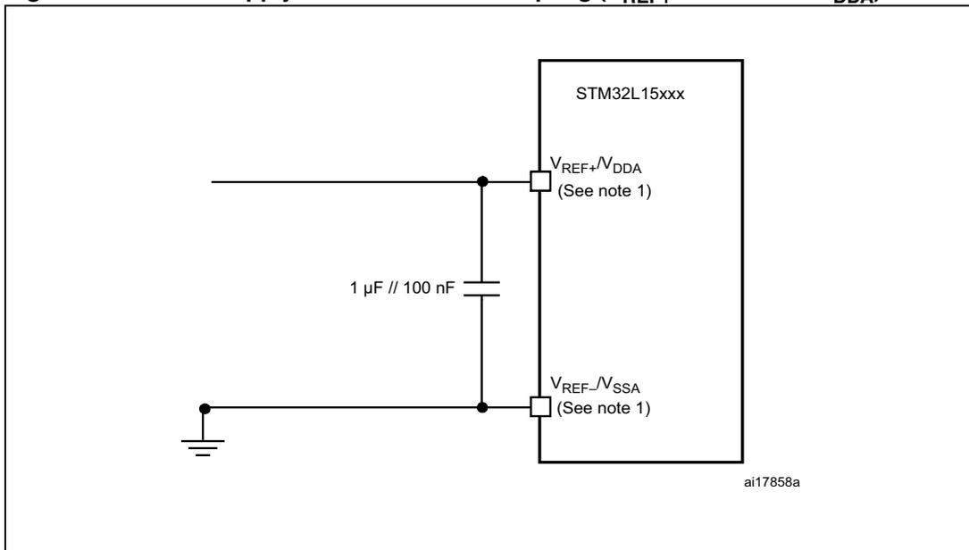
1.  $V_{REF+}$  and  $V_{REF-}$  inputs are available only on 100-pin packages.
