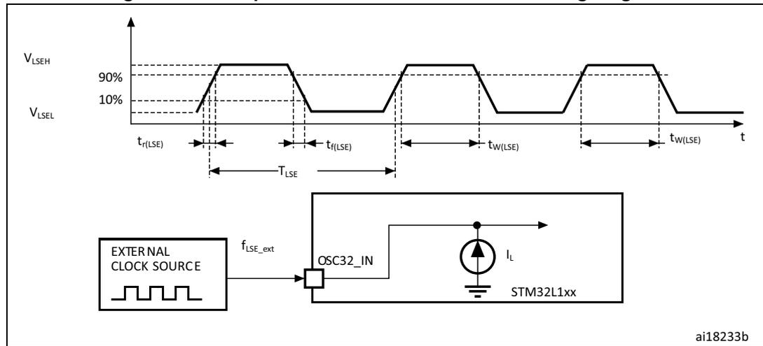
Figure 12. High-speed external clock source AC timing diagram
