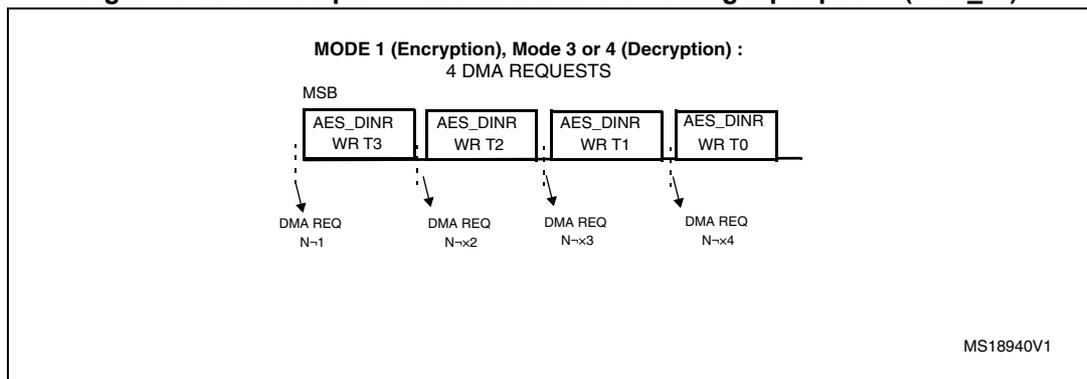
**Figure 183. DMA requests during Output phase (AES\_OUT)**
