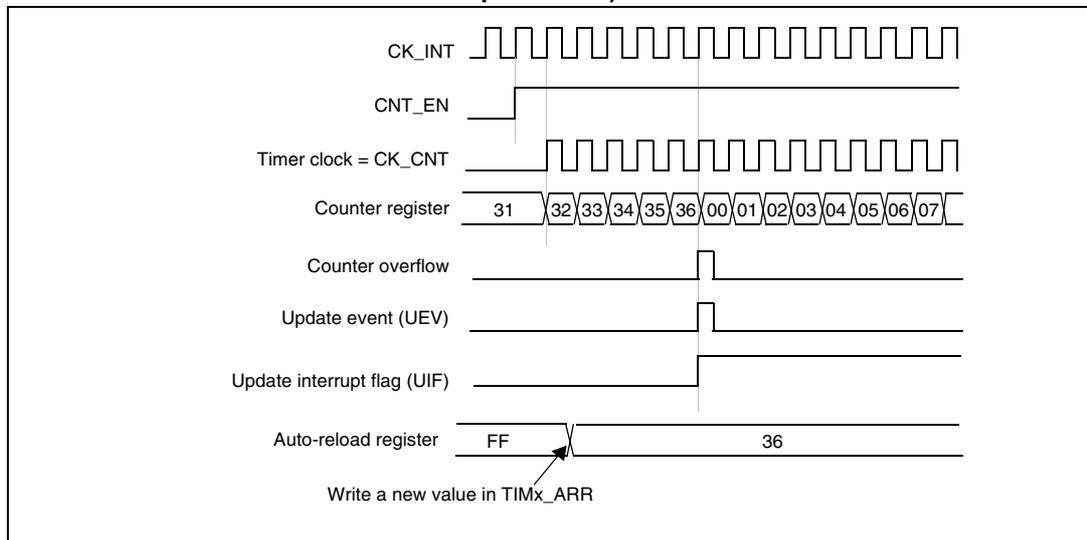
**Figure 90. Counter timing diagram, Update event when ARPE=1 (TIMx\_ARR preloaded)**
