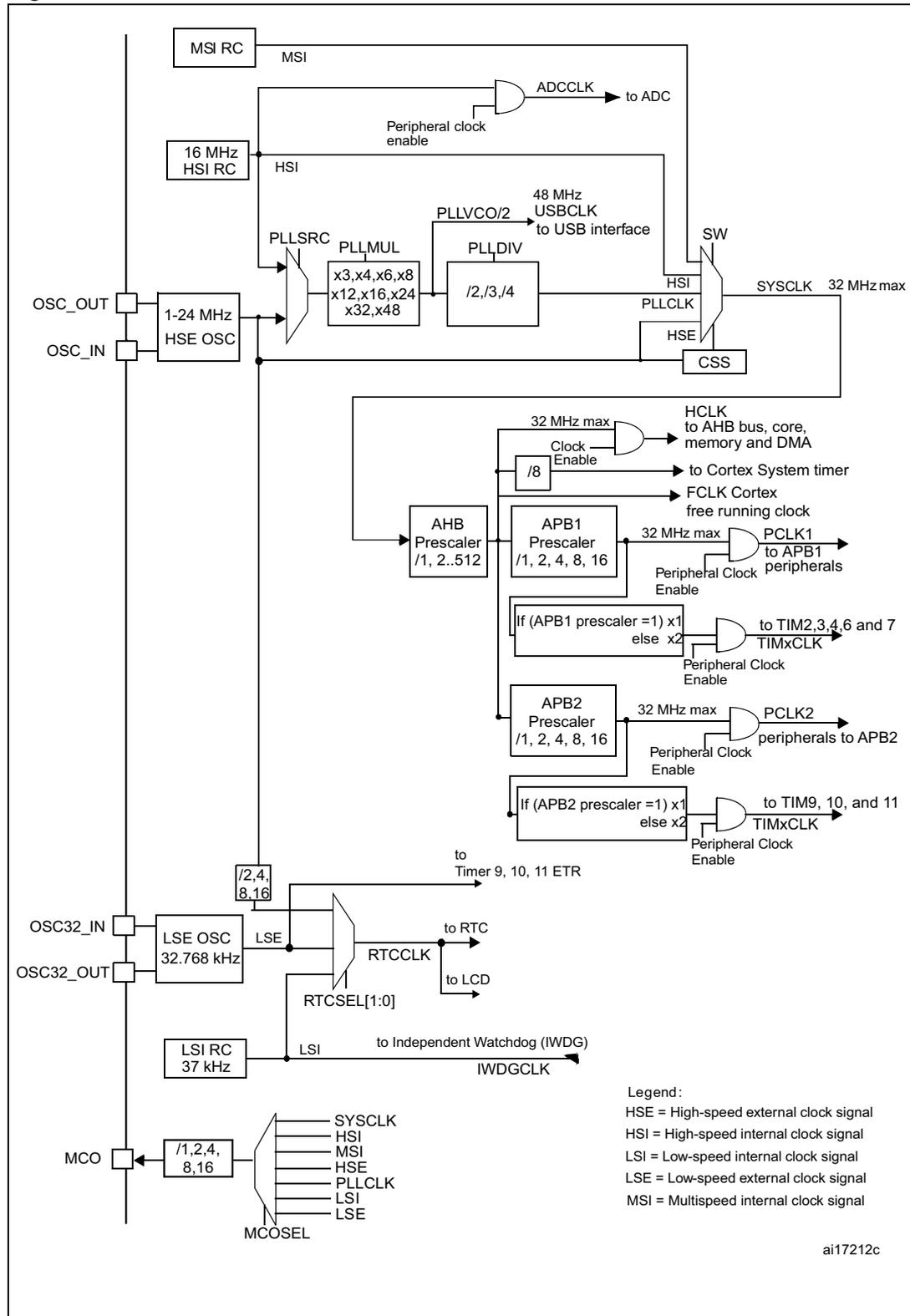
2. For the USB function to be available, both HSE and PLL must be enabled, with the CPU running at either 24 MHz or 32 MHz.
