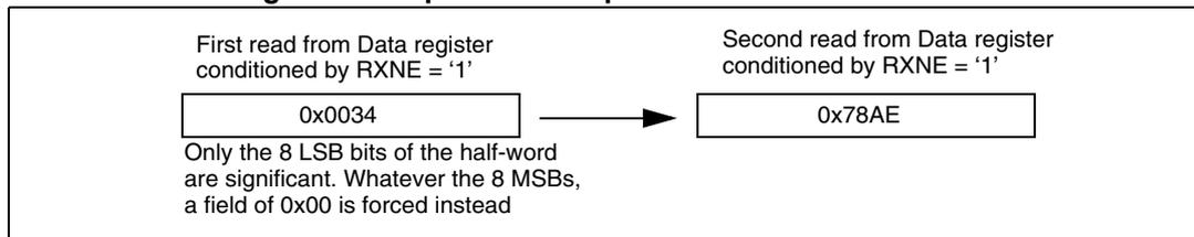
**Figure 268. LSB justified 16-bit extended to 32-bit packet frame with CPOL = 0**
