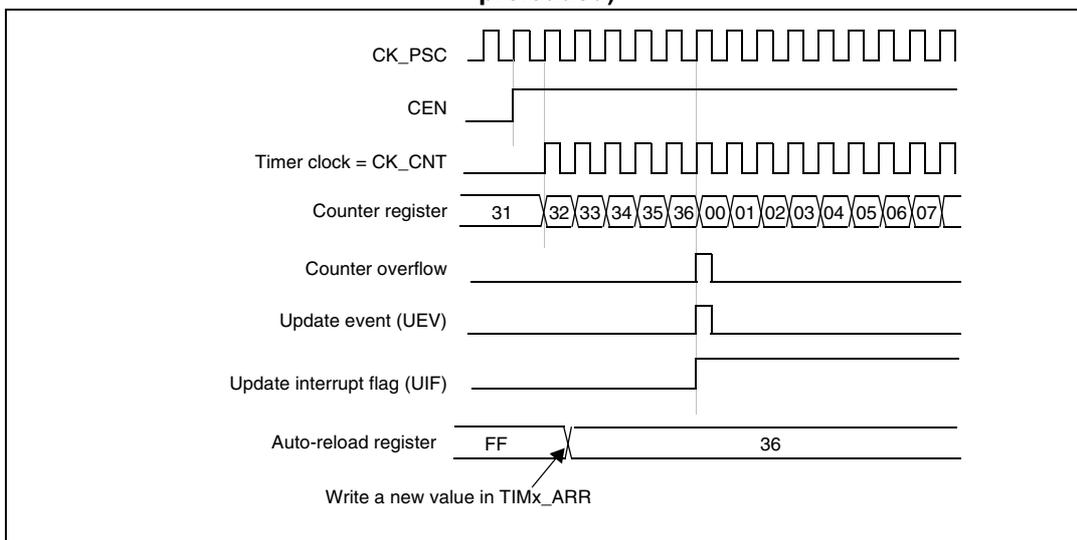
**Figure 138. Counter timing diagram, update event when ARPE=1 (TIMx\_ARR preloaded)**
