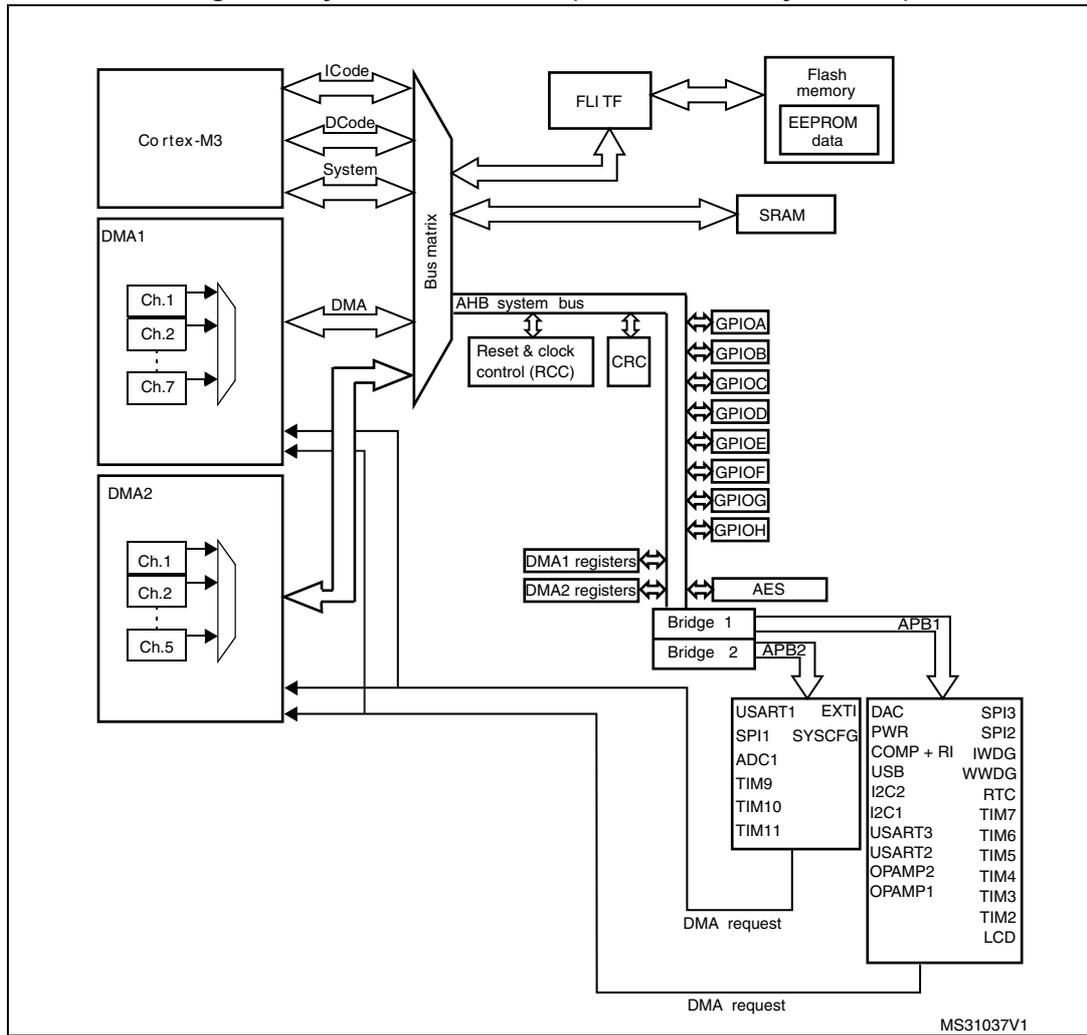
Figure 3. System architecture (high density devices)
