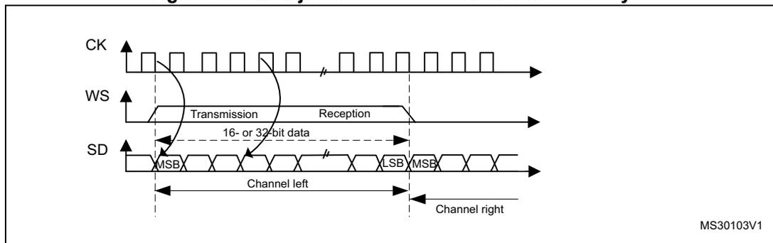
**Figure 376. LSB justified 24-bit frame length**
