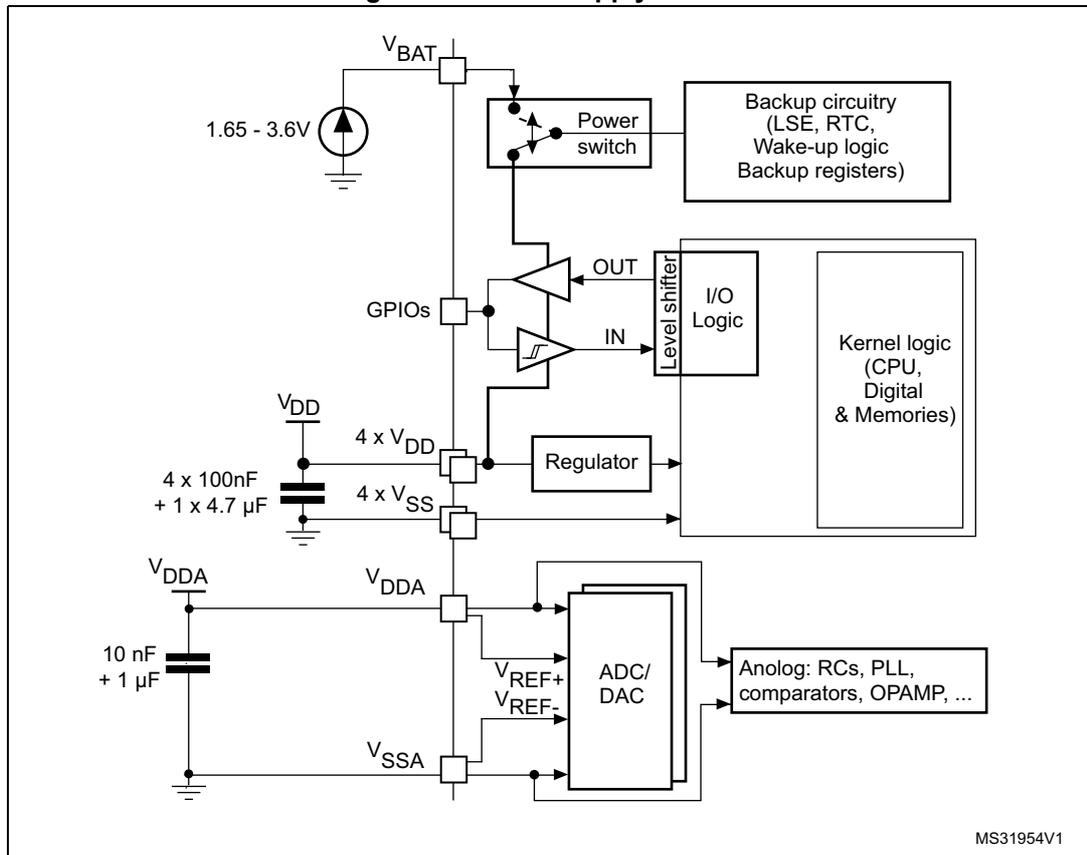
**Caution:** Each power supply pair (V<sub>DD</sub>/V<sub>SS</sub>, V<sub>DDA</sub>/V<sub>SSA</sub> etc..) must be decoupled with filtering ceramic capacitors as shown above. These capacitors must be placed as close as possible to, or below the appropriate pins on the underside of the PCB to ensure the good functionality of the device.
