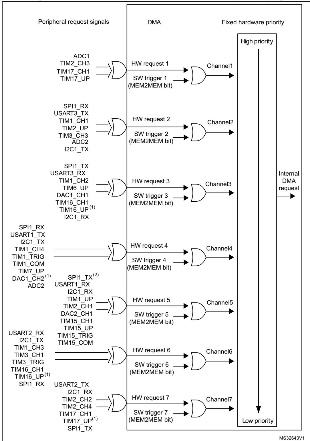
1. TIM6\_UP, DAC1\_CH1, TIM7\_UP, DAC1\_CH2, TIM16\_CH1, TIM16\_UP, TIM17\_CH1, TIM17\_UP, DAC2\_CH1, I2C1, SPI1 and DMA request are mapped on this DMA channel only if the corresponding remapping bit is set in the SYSCFG\_CFGR1 or SYSCFG\_CFGR3 register. For more details, please refer to [Section 12.1.1: SYSCFG configuration register 1 \(SYSCFG\\_CFGR1\)](#) on page 245 and [Section 12.1.8:](#)
