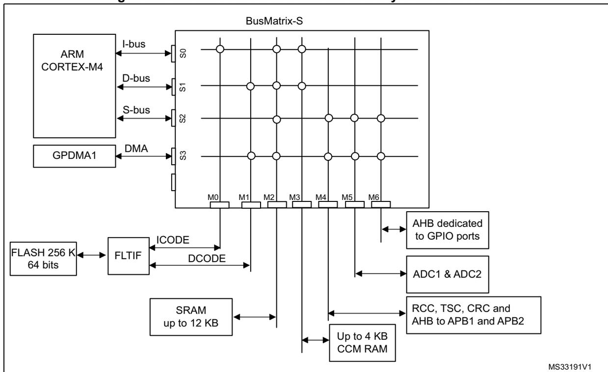
Figure 3. STM32F303xDxE and STM32F398xE system architecture
