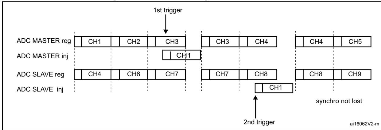
If a trigger occurs during an injected conversion that has interrupted a regular conversion, the alternate trigger is served. [Figure 106](#) shows the behavior in this case (note that the 6th trigger is ignored because the associated alternate conversion is not complete).
