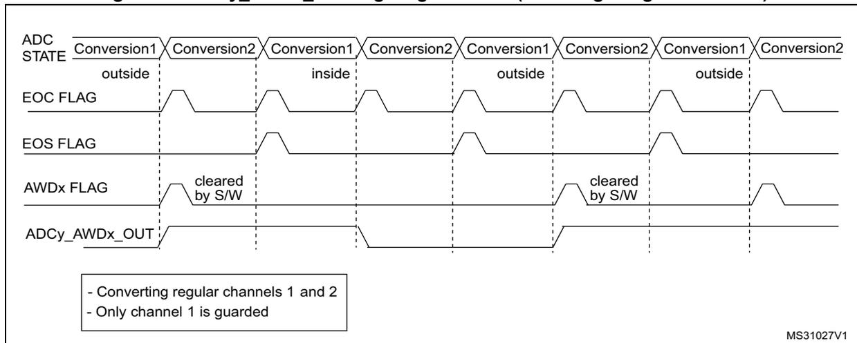
Figure 96. ADCy\_AWDx\_OUT signal generation (on all injected channels)
