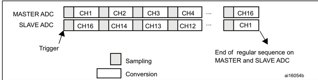
If  $DISCEN=1$  then each “n” simultaneous conversions of the regular sequence require a regular trigger event to occur (“n” is defined by  $DISCNUM$ ).
