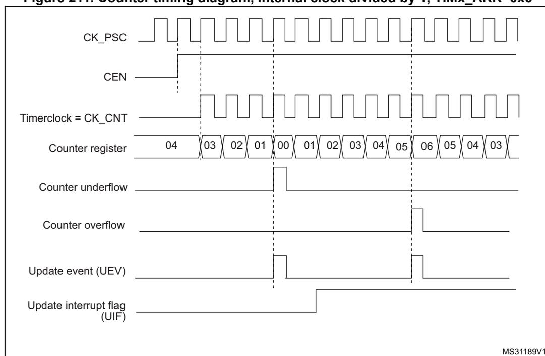
1. Here, center-aligned mode 1 is used (for more details refer to [Section 21.4.1: TIMx control register 1 \(TIMx\\_CR1\) on page 649](#)).
