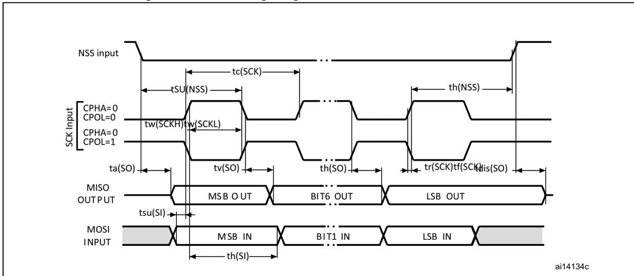
Figure 26. SPI timing diagram - slave mode and CPHA = 1<sup>(1)</sup>
