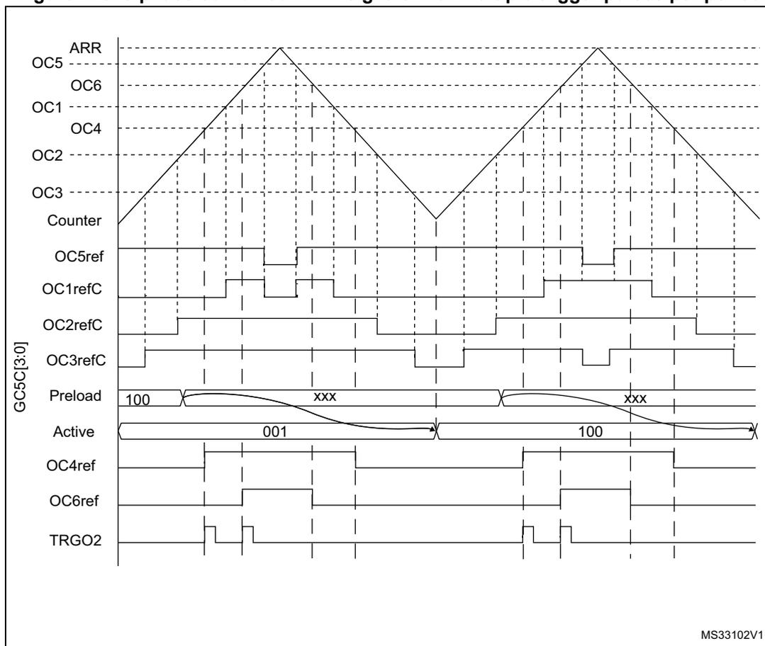
The TRGO2 waveform shows how the ADC can be synchronized on given 3-phase PWM signals. Please refer to [Section 20.3.26: ADC synchronization](#) for more details.
