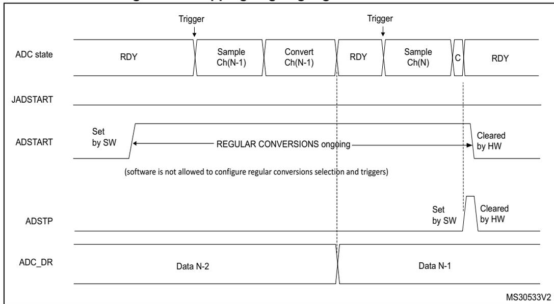
Figure 62. Stopping ongoing regular and injected conversions
