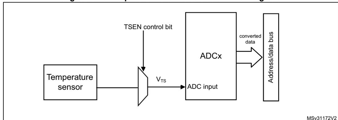
*Note:* The TSEN bit must be set to enable the conversion of the temperature sensor voltage  $V_{TS}$ .
