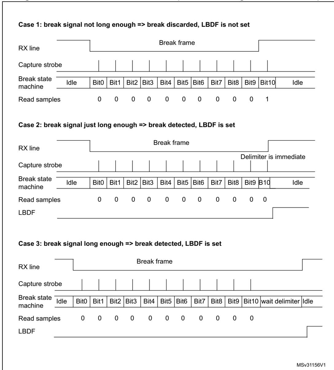
Figure 333. Break detection in LIN mode vs. Framing error detection
