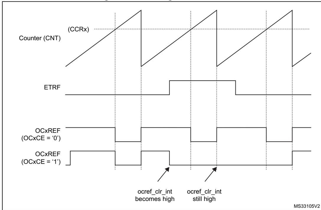
Note: In case of a PWM with a 100% duty cycle (if  $CCR_x > ARR$ ), then OCxREF is enabled again at the next counter overflow.
