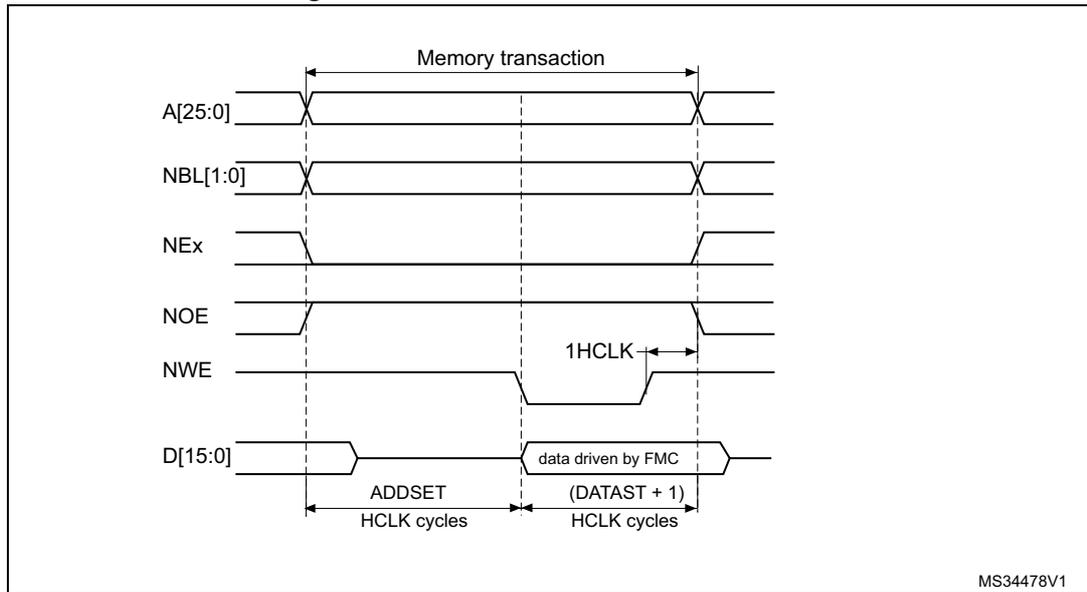
The one HCLK cycle at the end of the write transaction helps guarantee the address and data hold time after the NWE rising edge. Due to the presence of this HCLK cycle, the DATAST value must be greater than zero (DATAST > 0).
