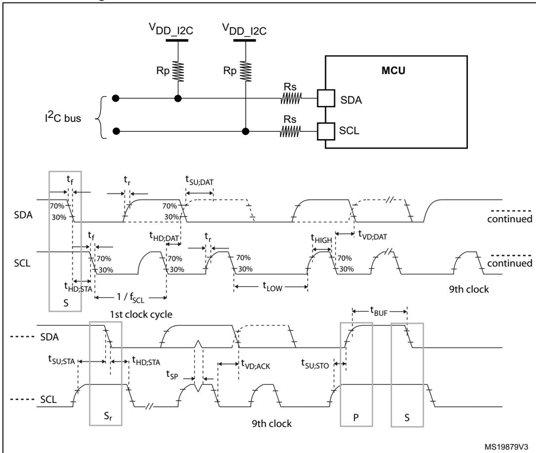
1. Rs: Series protection resistors, Rp: Pull-up resistors, VDD\_I2C: I2C bus supply.
