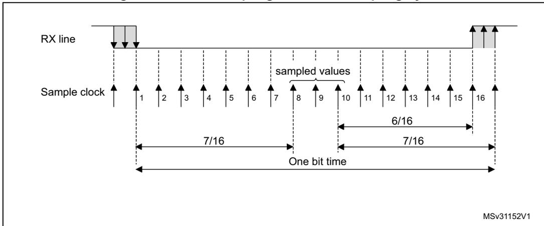
Figure 329. Data sampling when oversampling by 8
