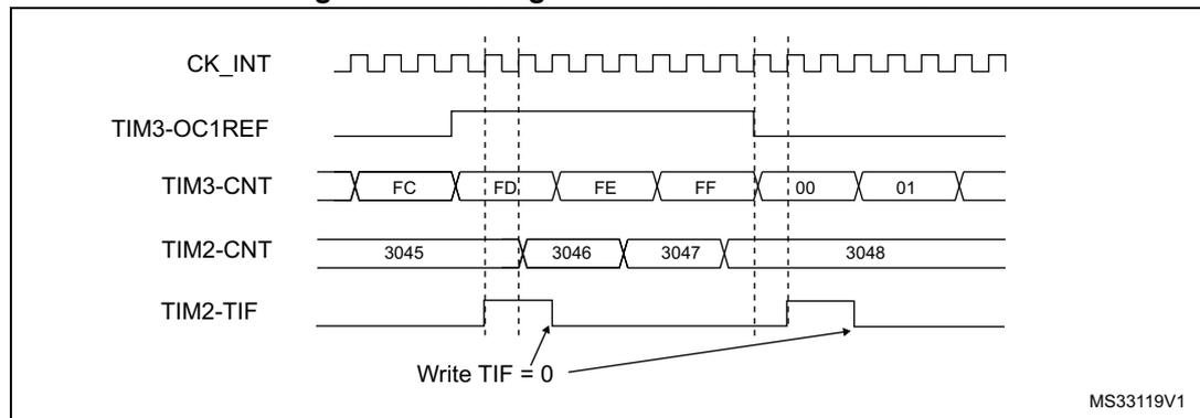
In the example in [Figure 241](#), the TIM2 counter and prescaler are not initialized before being started. So they start counting from their current value. It is possible to start from a given value by resetting both timers before starting TIM3. You can then write any value you want in the timer counters. The timers can easily be reset by software using the UG bit in the TIMx\_EGR registers.
