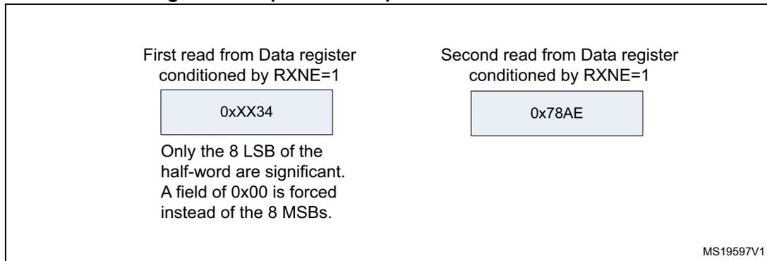
**Figure 379. LSB justified 16-bit extended to 32-bit packet frame**
