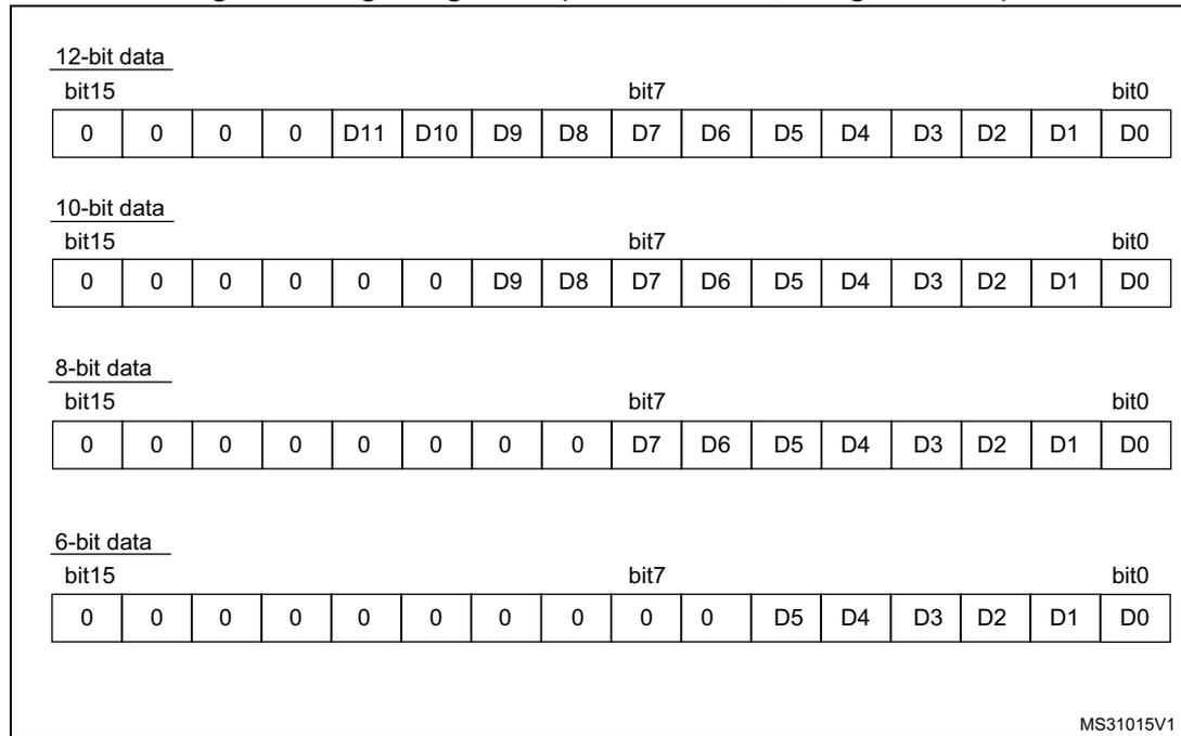
**Figure 83. Right alignment (offset enabled, signed value)**
