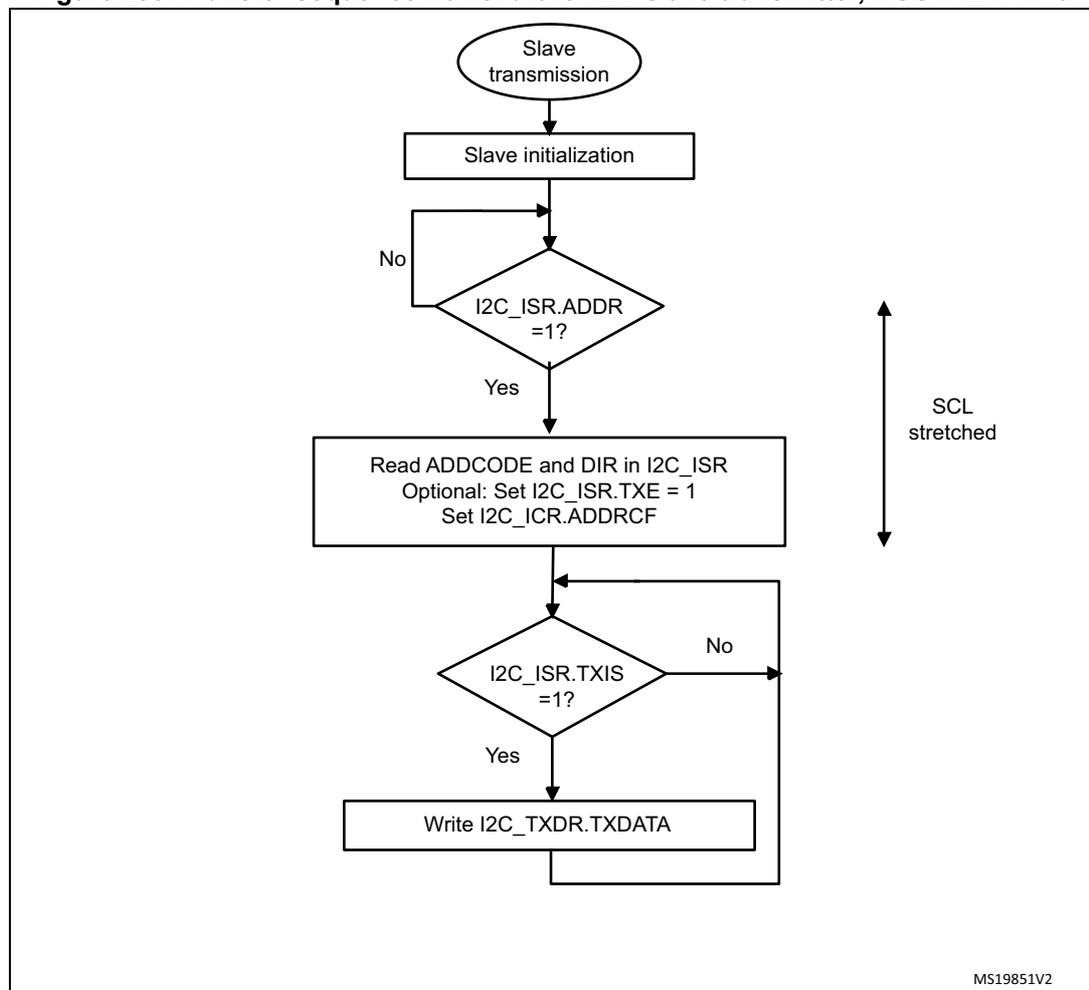
Figure 300. Transfer sequence flowchart for I2C slave transmitter, NOSTRETCH=1
