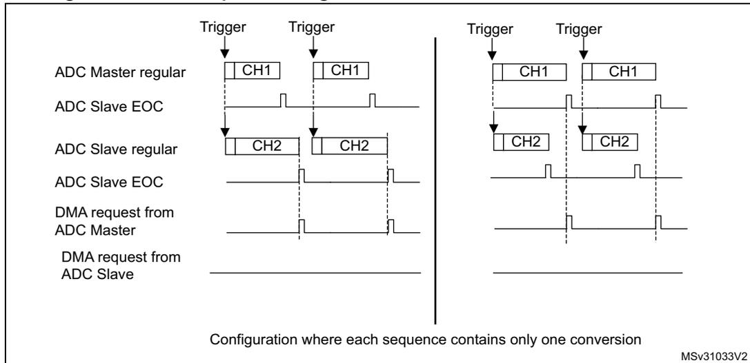
**Figure 109. DMA requests in interleaved mode when MDMA=0b10**
