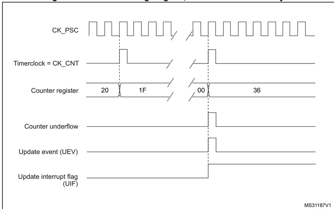
**Figure 153. Counter timing diagram, update event when repetition counter is not used**
