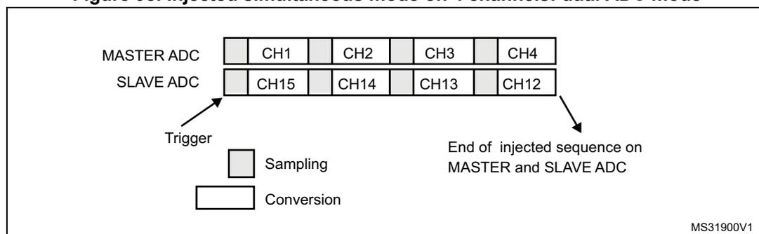
If JDISCEN=1, each simultaneous conversion of the injected sequence requires an injected trigger event to occur.
