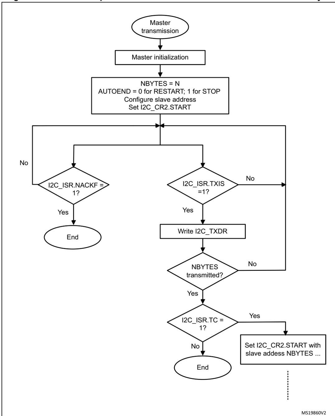
Figure 310. Transfer sequence flowchart for I2C master transmitter for N>255 bytes
