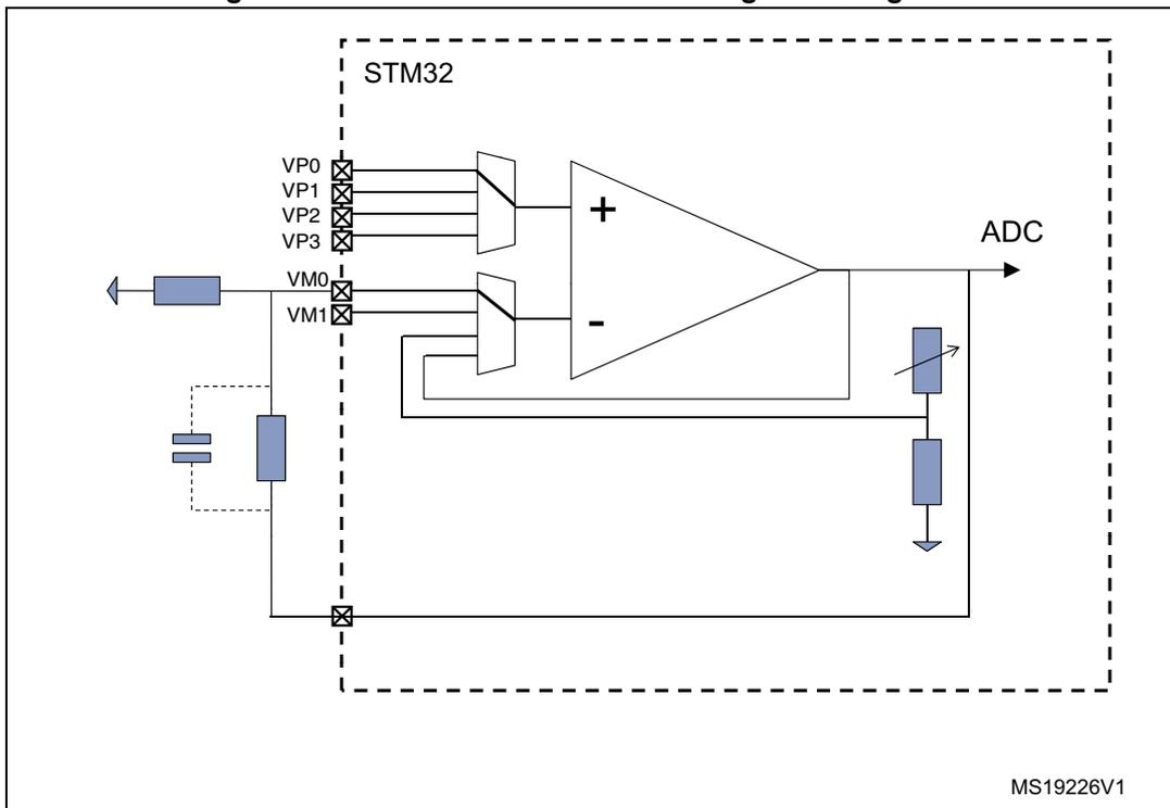
1. This figure gives an example in an inverting configuration. Any other option is possible, including comparator mode.
