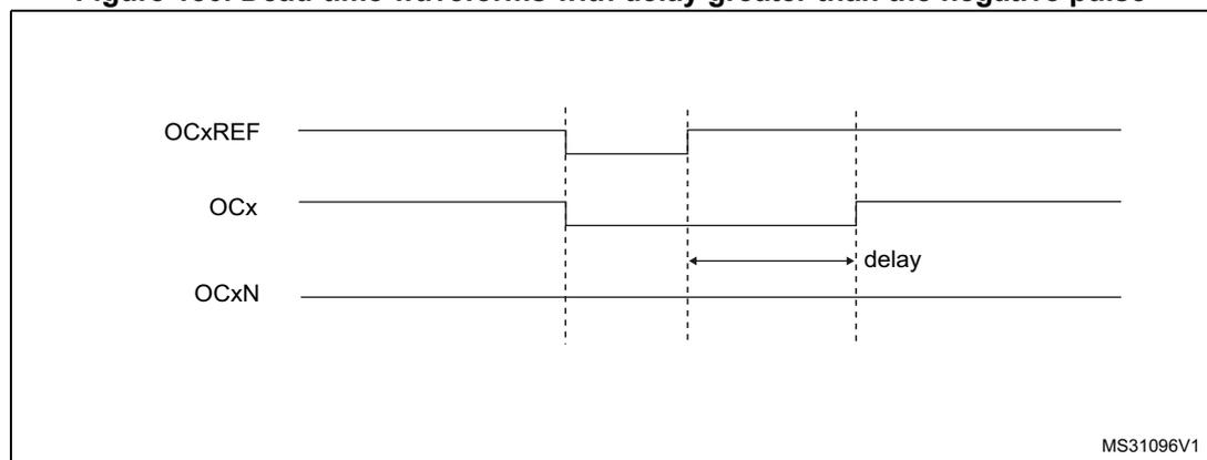
**Figure 181. Dead-time waveforms with delay greater than the positive pulse**
