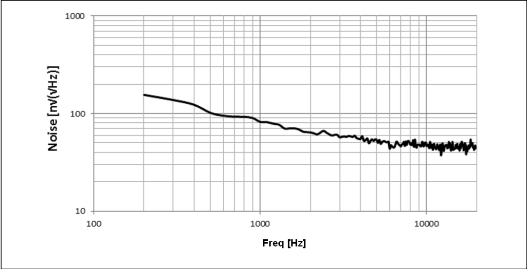
Figure 53. OPAMP voltage noise versus frequency
