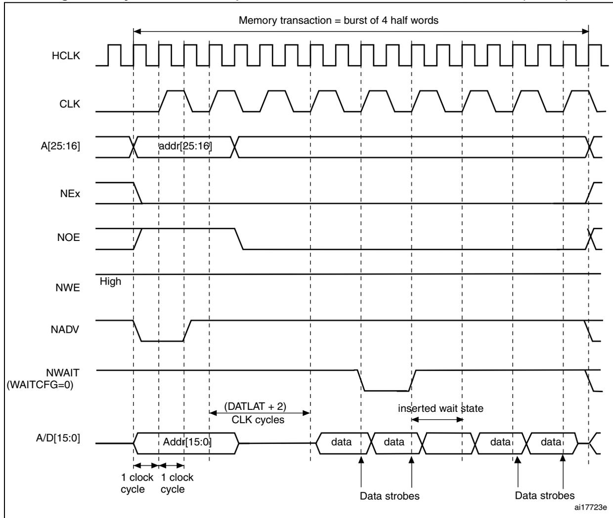
1. Byte lane outputs (NBL are not shown; for NOR access, they are held high, and, for PSRAM (CRAM) access, they are held low.
