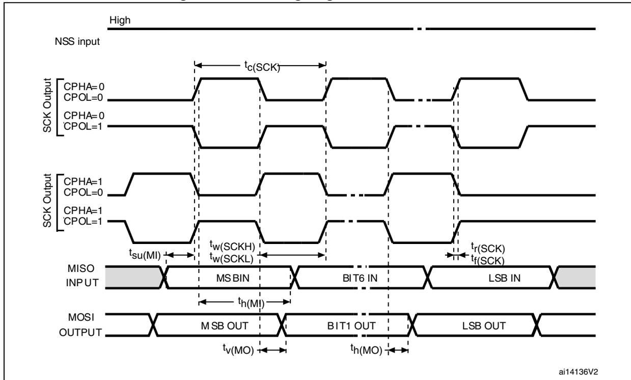
1. Measurement points are done at  $0.5V_{DD}$  and with external  $C_L = 30 \text{ pF}$ .
