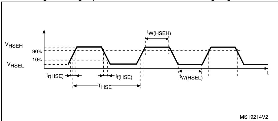
**Low-speed external user clock generated from an external source**
