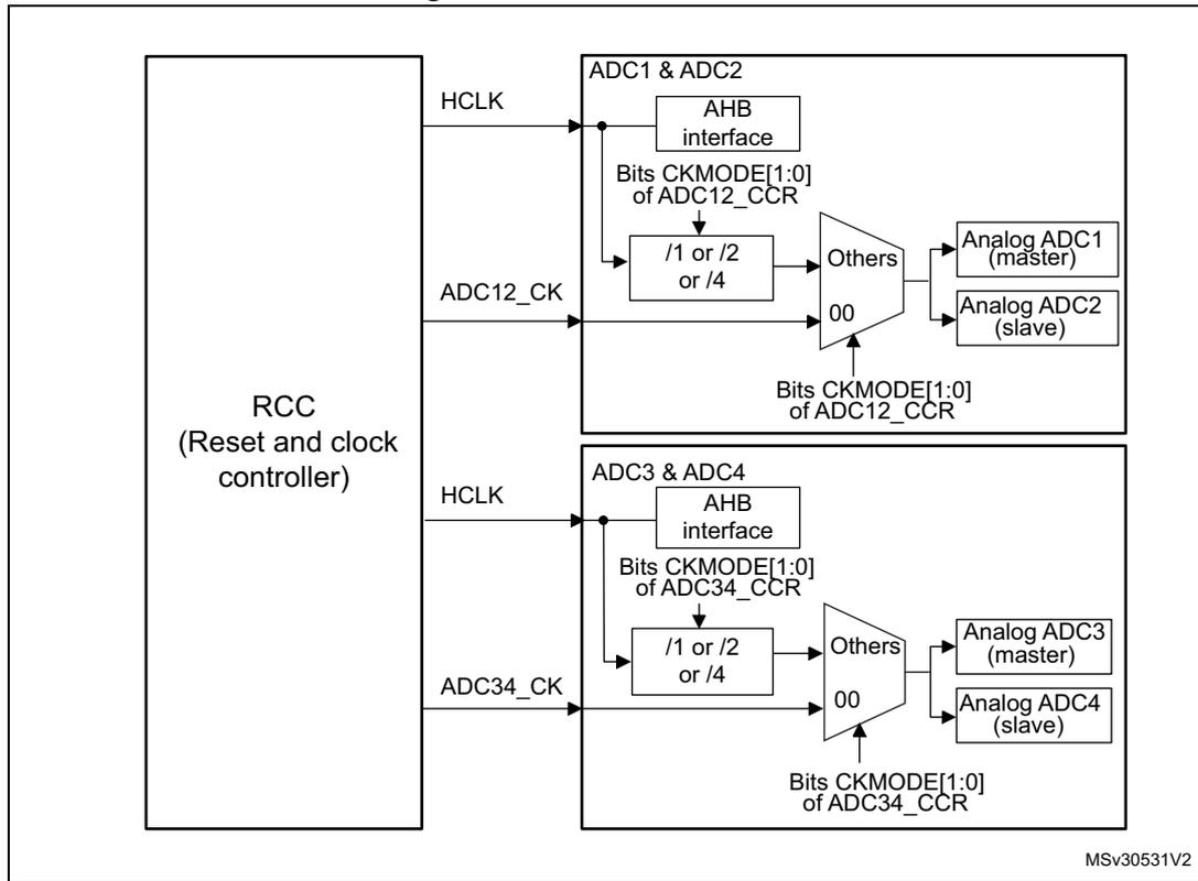
1. Refer to the RCC section to see how HCLK, ADC12\_CK, and ADC34\_CK can be generated.
