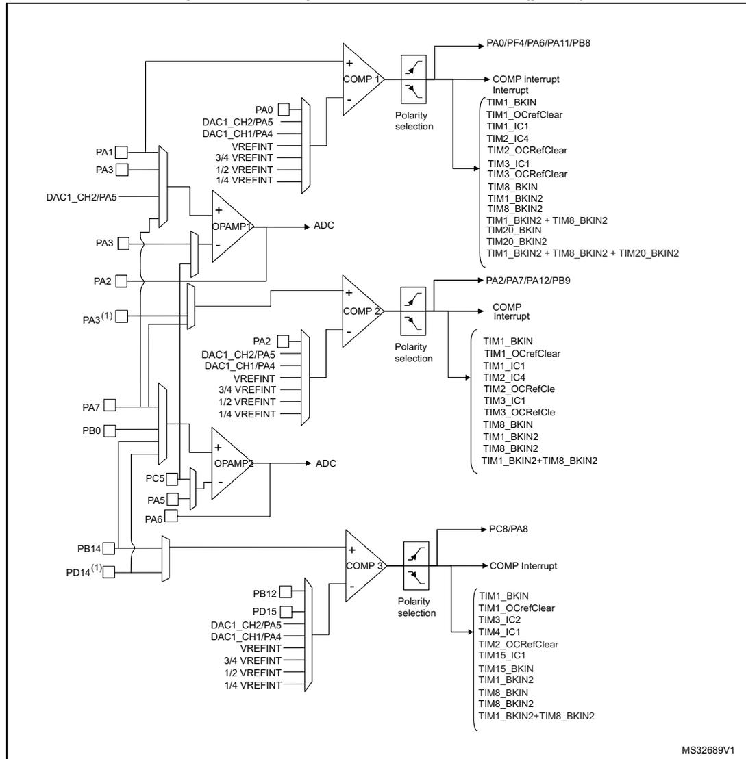
Figure 128. STM32F303xB/C/D/E and STM32F358xC comparators and operational amplifiers interconnections (part 2)
