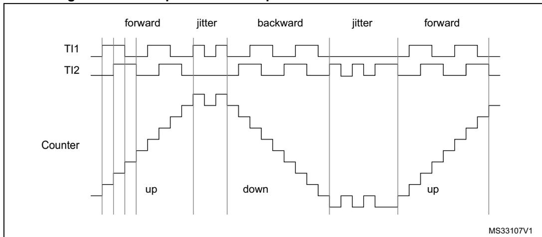
Figure 190 gives an example of counter behavior when TI1FP1 polarity is inverted (same configuration as above except CC1P='1').
