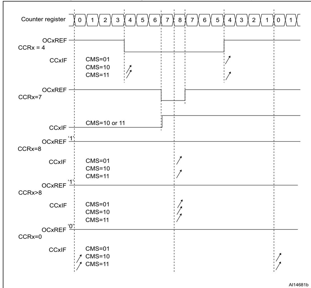
Hints on using center-aligned mode
