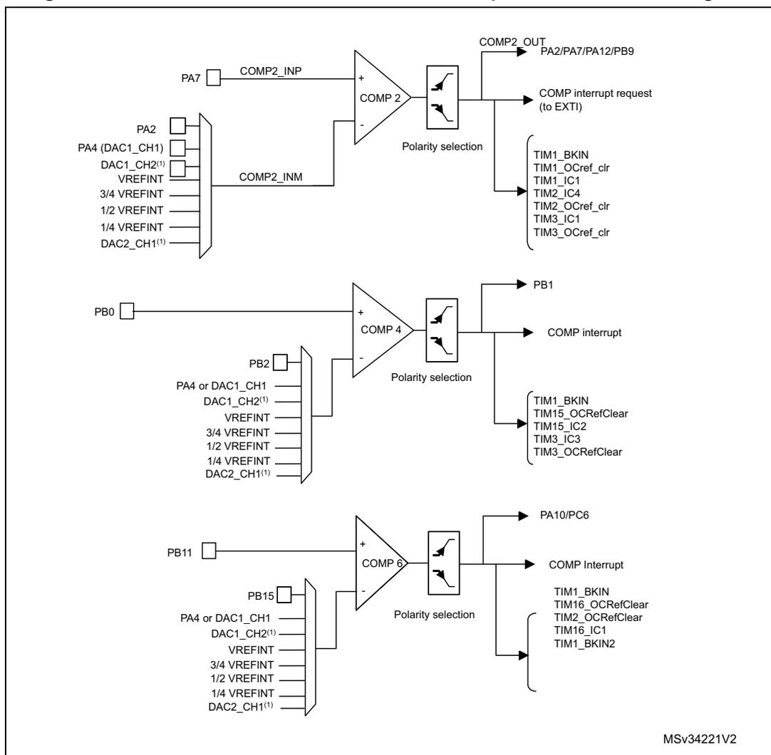
1. In STM32F303x6/8 and STM32F328x8 devices, DAC1\_CH2 and DAC2\_CH1 outputs are connected directly, thus PA5 and PA6 are not available as COMPx\_INM (x = 2,4,6) inputs. When DAC1\_OUT2 and DAC2\_OUT1 are connected internally to comparator non inverting input, the I/Os on which the DAC1\_OUT and DAC2\_OUT1 are mapped (PA5 and PA6) can be used as GPIOs.
