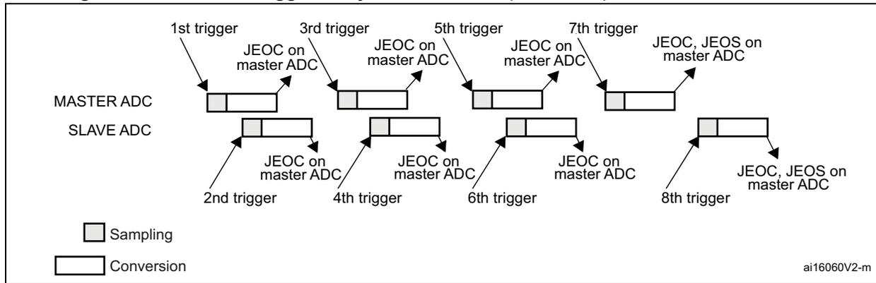
**Combined regular/injected simultaneous mode**
