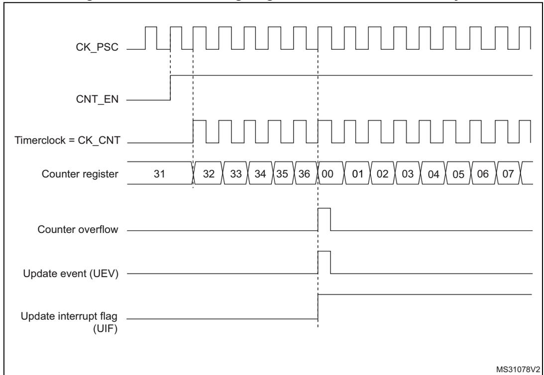
**Figure 144. Counter timing diagram, internal clock divided by 2**
