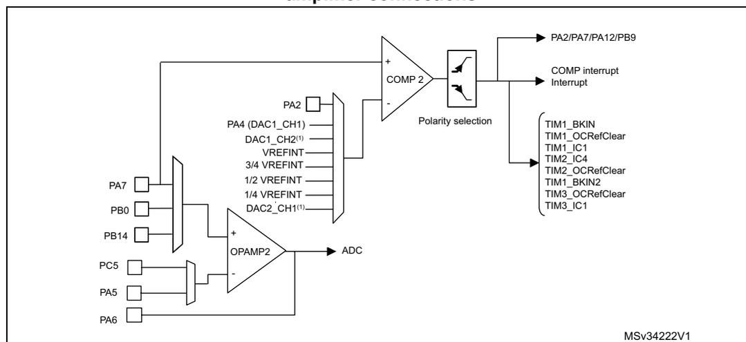
1. DAC1\_CH2 and DAC2\_CH1 outputs are connected directly, thus PA5 and PA6 are not available as inputs for COMP2\_INM. They can be used as GPIOs.
