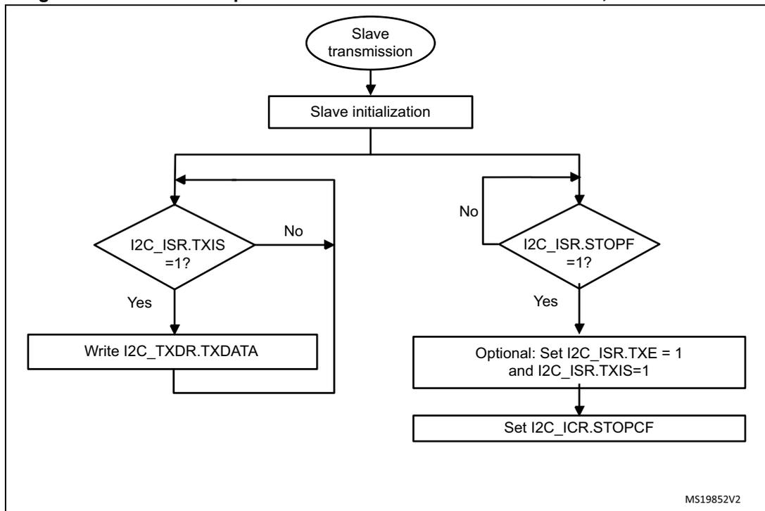
Figure 301. Transfer bus diagrams for I2C slave transmitter
