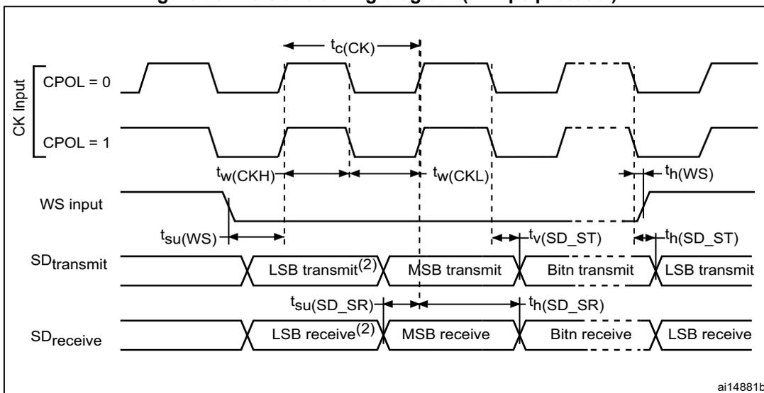
1. Measurement points are done at 0.5V<sub>DD</sub> and with external C<sub>L</sub>=30 pF.
