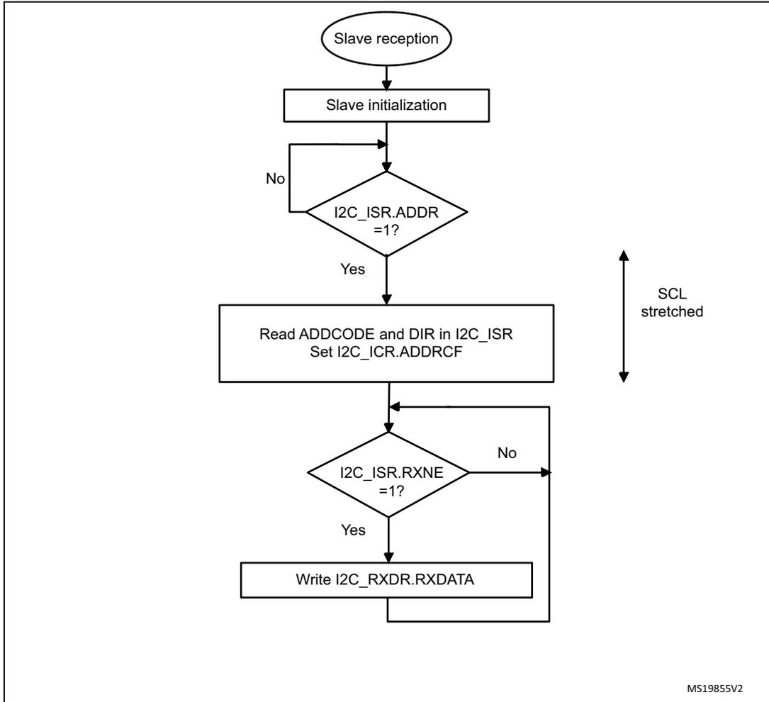
Figure 303. Transfer sequence flowchart for slave receiver with NOSTRETCH=1
