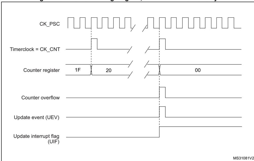
**Figure 264. Counter timing diagram, update event when ARPE=0 (TIMx\_ARR not preloaded)**
