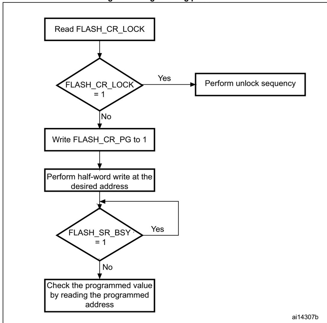
The Flash memory interface preliminarily reads the value at the addressed main Flash memory location and checks that it has been erased. If not, the program operation is skipped and a warning is issued by the PGERR bit in FLASH\_SR register (the only exception to this is when 0x0000 is programmed. In this case, the location is correctly
