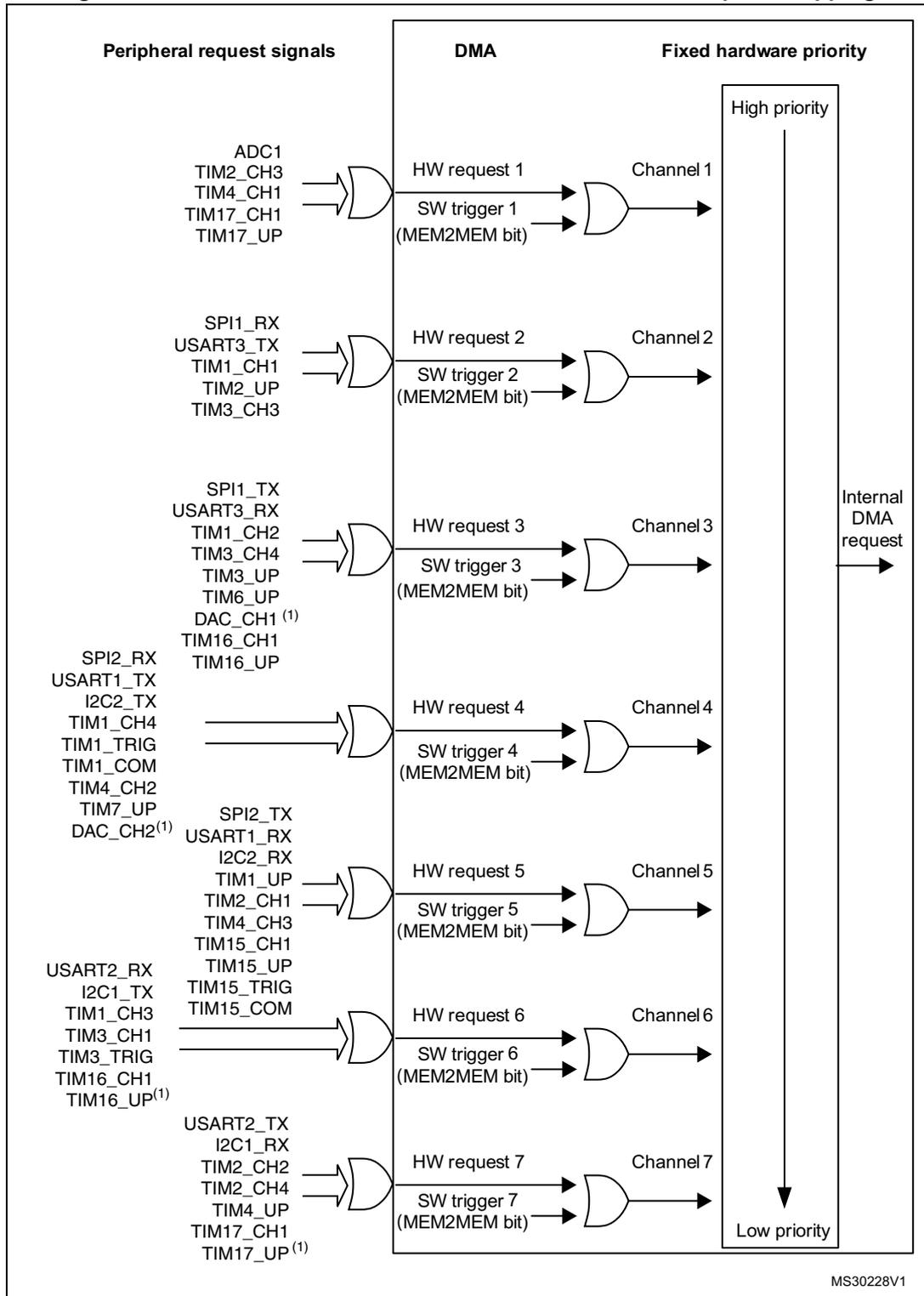
1. DMA requests are mapped on this DMA channel only if the corresponding remapping bit is set in the SYSCFG\_CFGR1 register. For more details, please refer to [Section 12.1.1: SYSCFG configuration register 1 \(SYSCFG\\_CFGR1\) on page 245](#).
