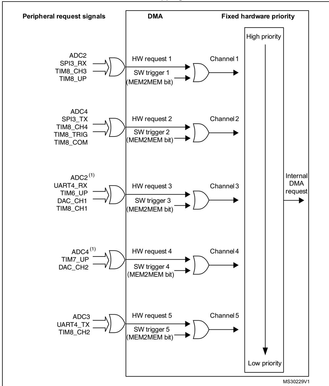
1. DMA request mapped on this DMA channel only if the corresponding remapping bit is set in the SYSCFG\_CFGR1 register. For more details, please refer to [Section 12.1.1: SYSCFG configuration register 1 \(SYSCFG\\_CFGR1\) on page 245](#).
