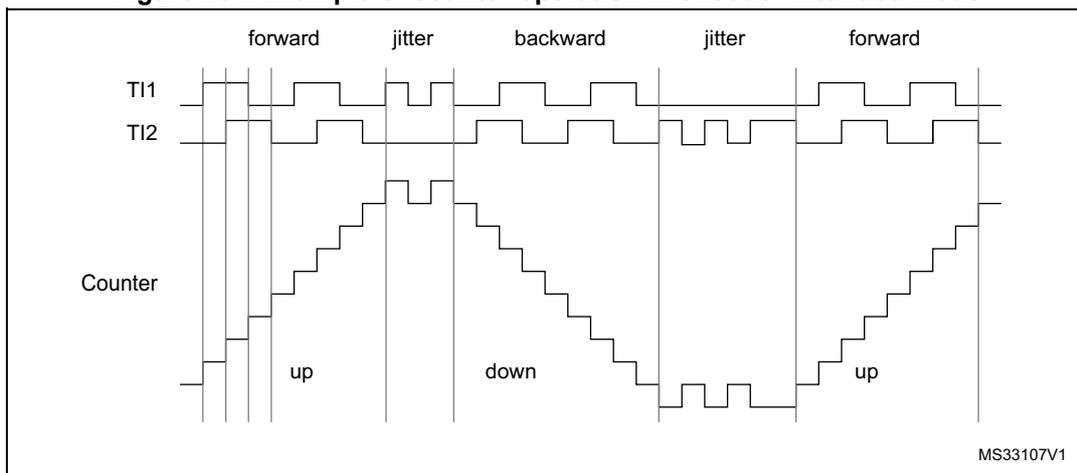
Figure 235 gives an example of counter behavior when TI1FP1 polarity is inverted (same configuration as above except CC1P=1).
