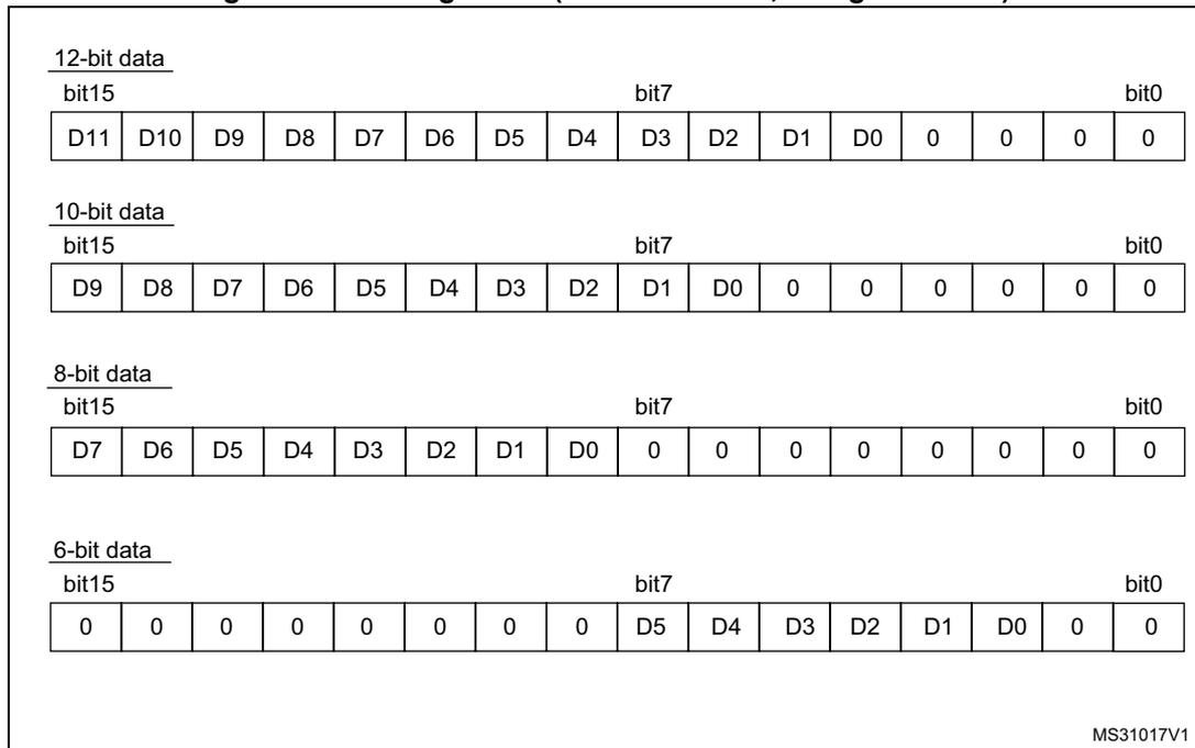
**Figure 85. Left alignment (offset enabled, signed value)**
