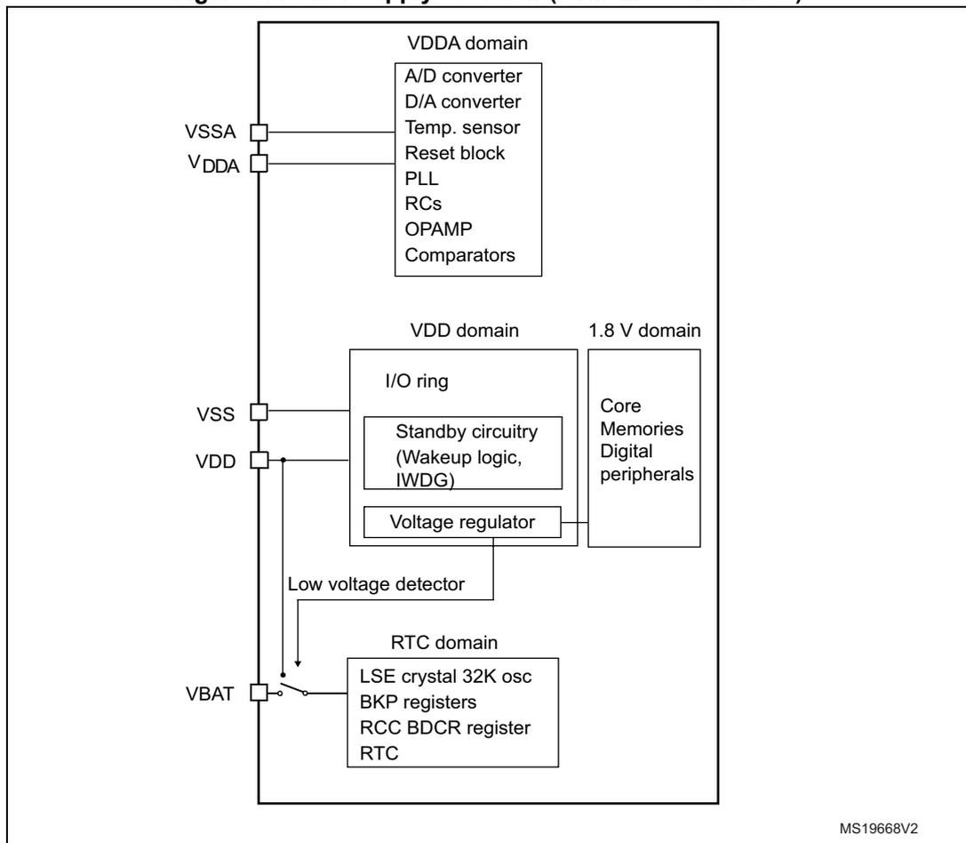
Figure 9. Power supply overview (STM32F3x8 devices)
