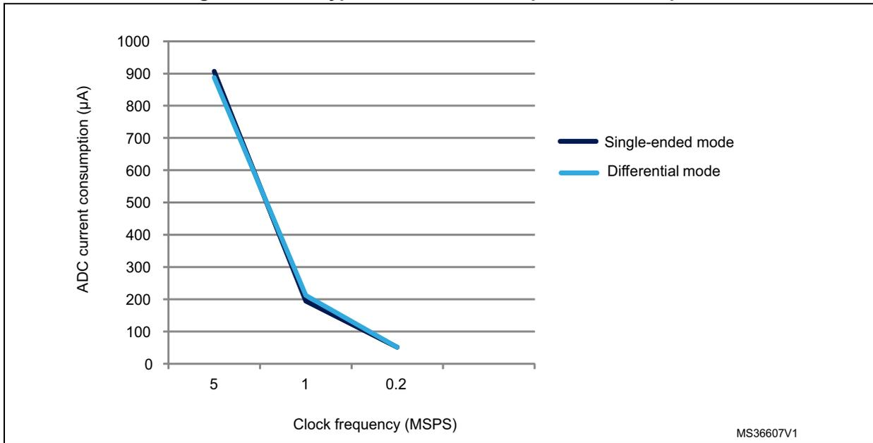
Figure 32. ADC typical current consumption on VREF+ pin
