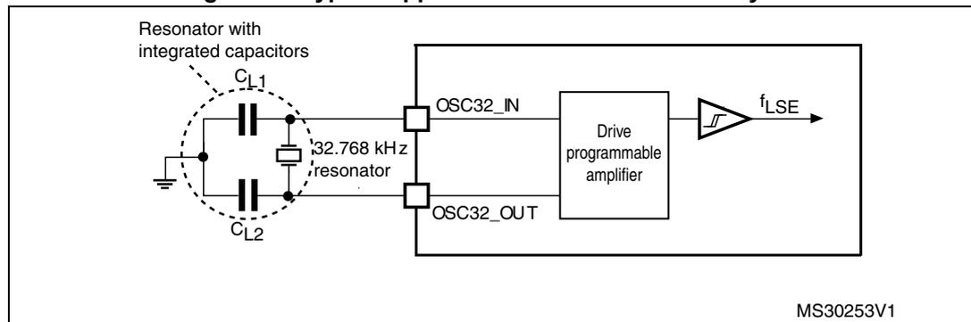
**Note:** An external resistor is not required between  $OSC32\_IN$  and  $OSC32\_OUT$  and it is forbidden to add one.
