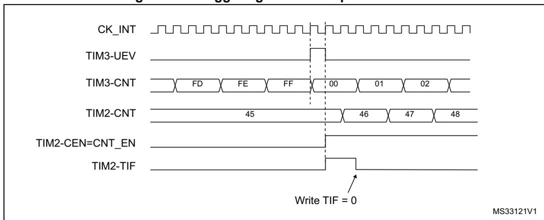
As in the previous example, you can initialize both counters before starting counting. [Figure 244](#) shows the behavior with the same configuration as in [Figure 243](#) but in trigger mode instead of gated mode (SMS=110 in the TIM2\_SMCR register).
