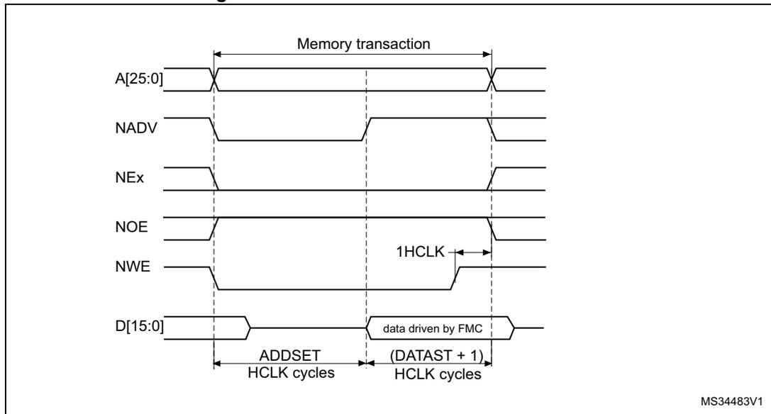
The differences with mode1 are the toggling of NWE and the independent read and write timings when extended mode is set (Mode B).
