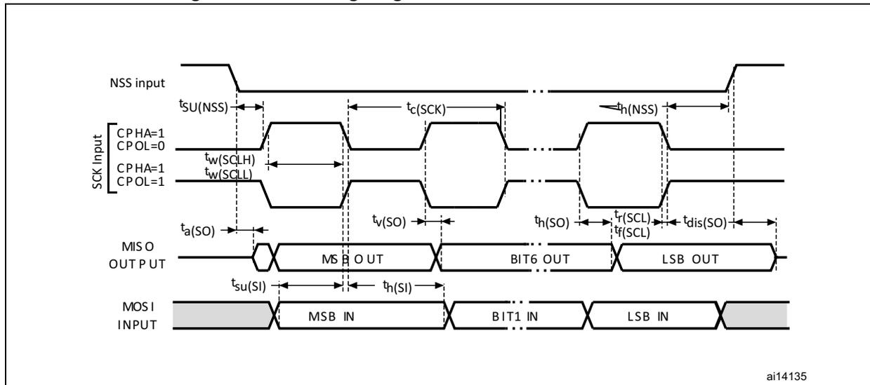
1. Measurement points are done at  $0.5V_{DD}$  and with external  $C_L = 30$  pF.
