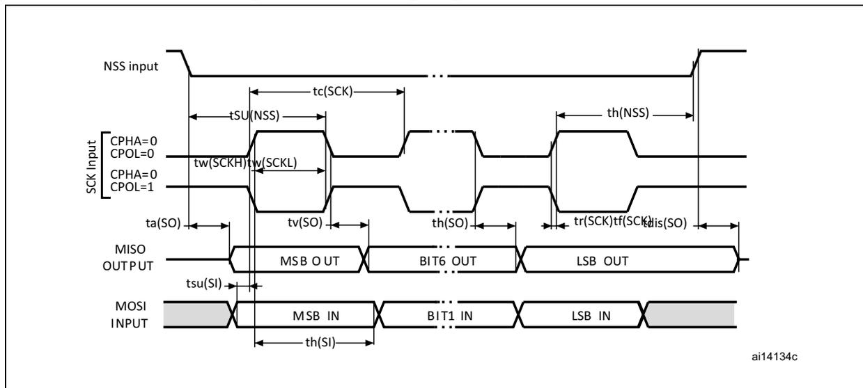
Figure 25. SPI timing diagram - slave mode and CPHA = 1<sup>(1)</sup>
