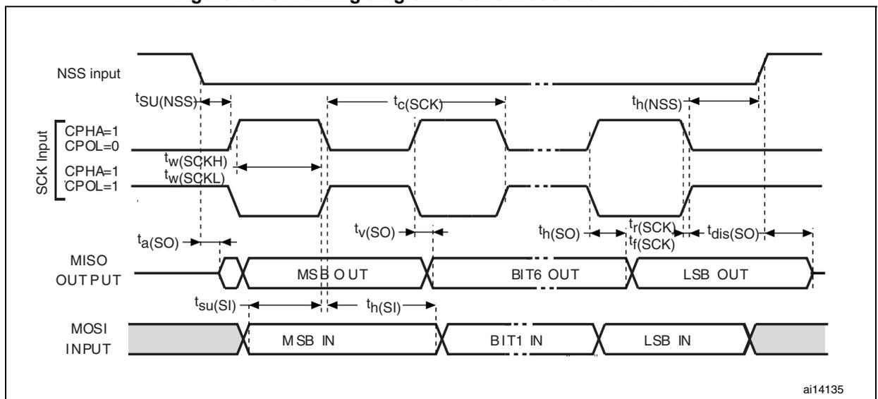
1. Measurement points are done at 0.5V<sub>DD</sub> and with external C<sub>L</sub> = 30 pF.
