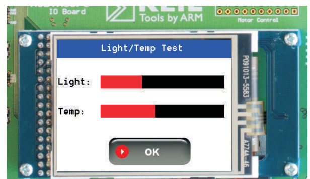
Light and Temperature sensors are provided on the I/O board and their level is shown on the LCD screen.
