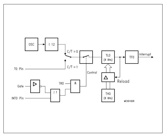
Figure 7-23 Timer/Counter 0/1, Mode 2: 8-Bit Timer/Counter with Auto-Reload
