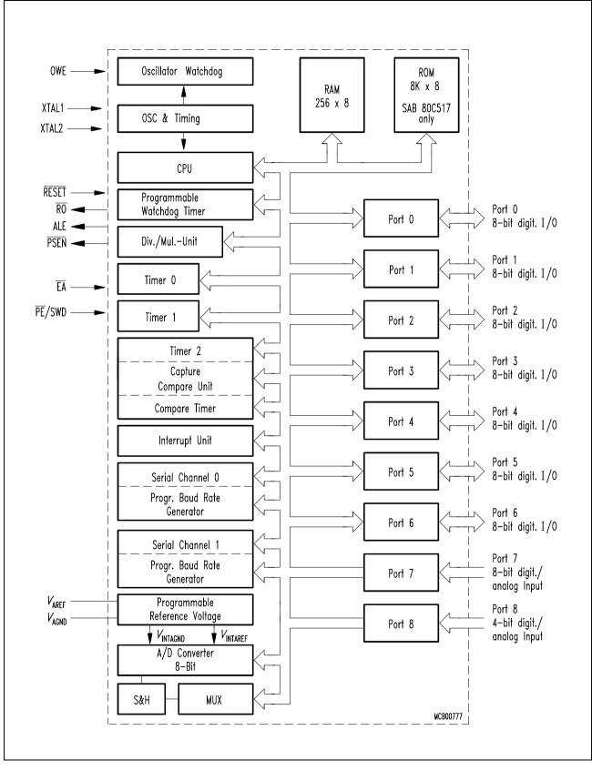
Figure 2-1 Functional Block Diagram
