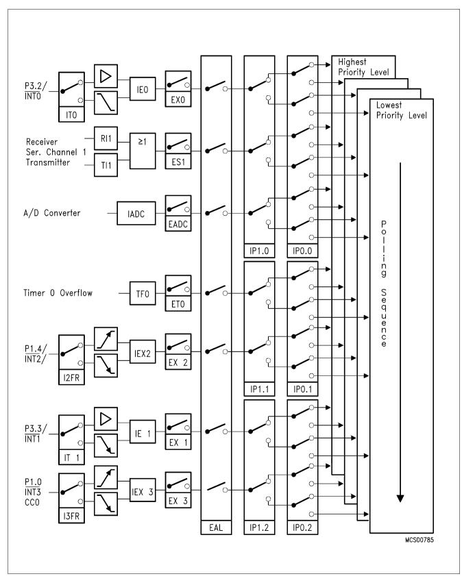
Figure 9 Interrupt Structure
