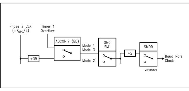
Figure 7-11 Generation of Baud Rates for Serial Channel 0
