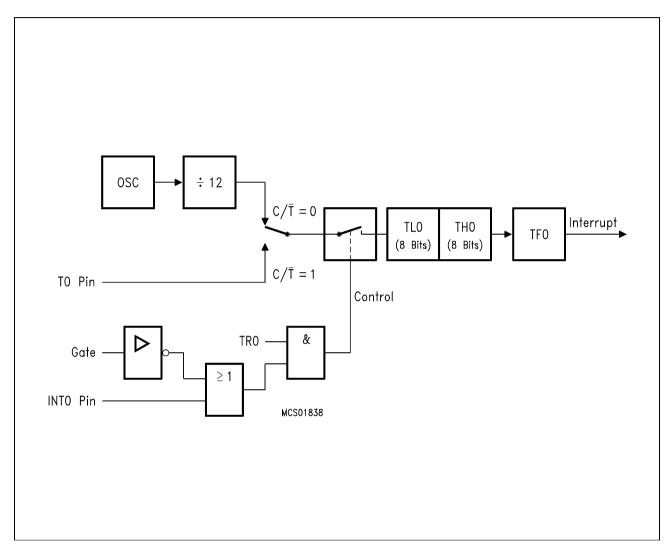
Figure 7-22 Timer/Counter 0/1, Mode 1: 16-Bit Timer/Counter
