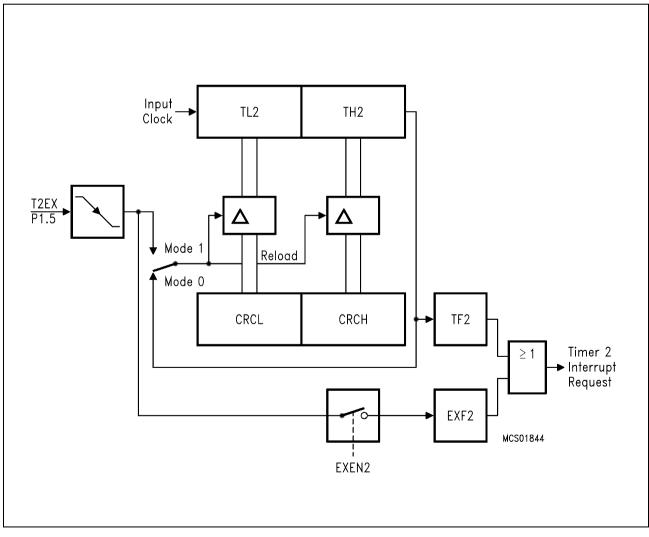
Figure 7-34 b) Timer 2 in Reload Mode
