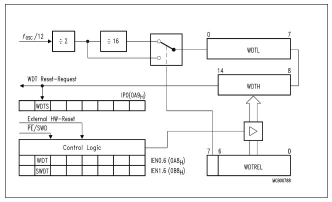
Figure 7-58 Block Diagram of the Programmable Watchdog Timer
