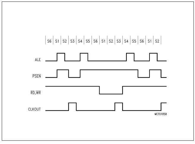
Figure 7-69 Timing Diagram - System Clock Output
