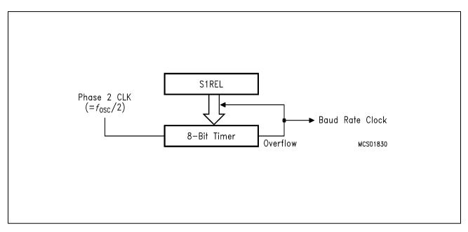
Figure 7-14 Baud Rate Generator for Serial Interface 1
