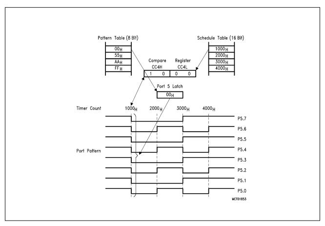
Figure 7-46 Example for a "Concurrent Compare" at Port 5
