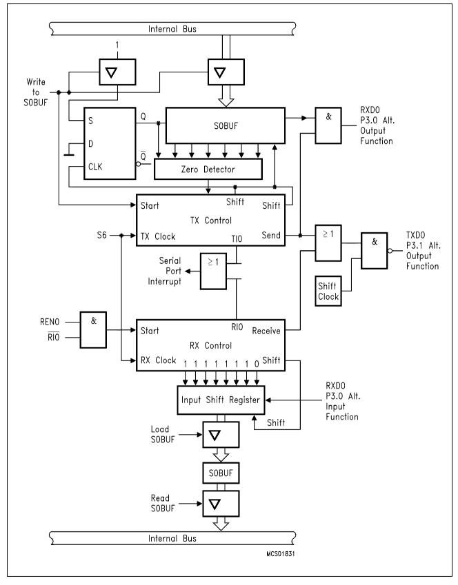
Figure 7-16 a) Functional Diagram - Serial Interface 0, Mode 0
