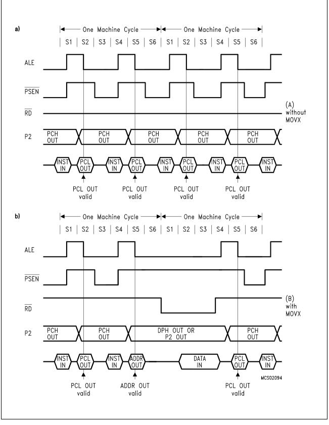
Figure 5-2 a) and b) External Program Memory Execution
