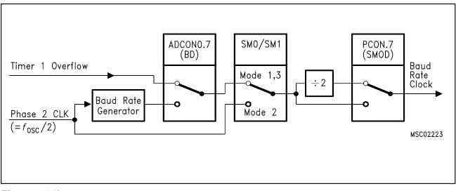
Figure 7-11b Block Diagram of Baud Rate Generation for Serial Interface 0
