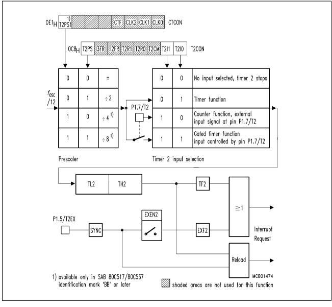
Figure 7-34 a) Block Diagram of Timer 2
