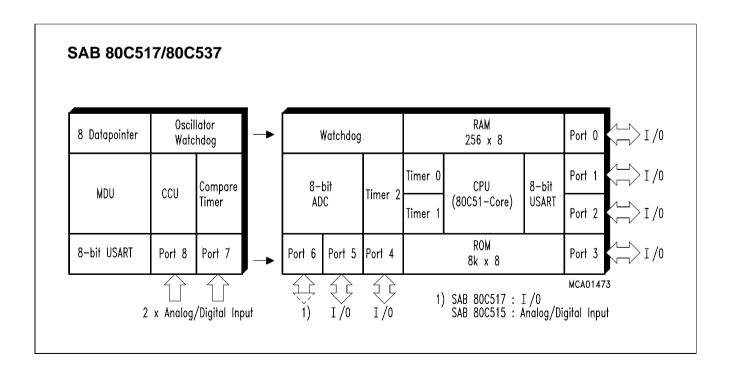
The SAB 80C517/80C537 is a high-end member of the Siemens SAB 8051 family of microcontrollers. It is designed in Siemens ACMOS technology and based on the SAB 8051 architecture. ACMOS is a technology which combines high-speed and density characteristics with low-power consumption or dissipation.
