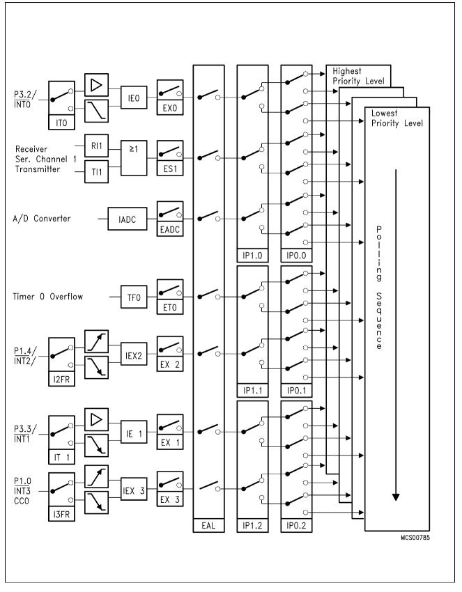
Figure 8-1 a) Interrupt Structure of the SAB 80C517
