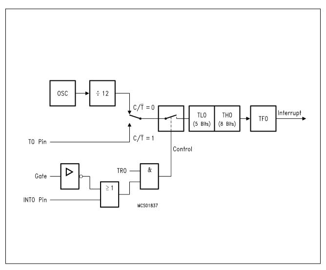
Figure 7-21 Timer/Counter 0/1, Mode 0: 13 Bit Timer/Counter
