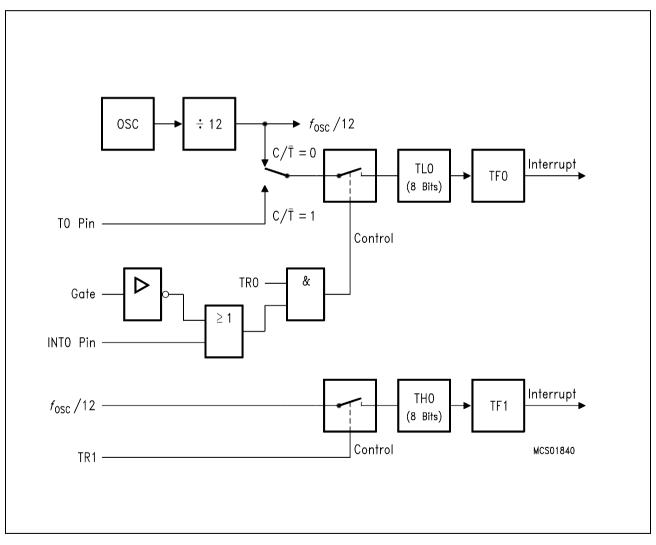
Figure 7-24 Timer/Counter 0, Mode 3: Two 8-Bit Timer/Counter
