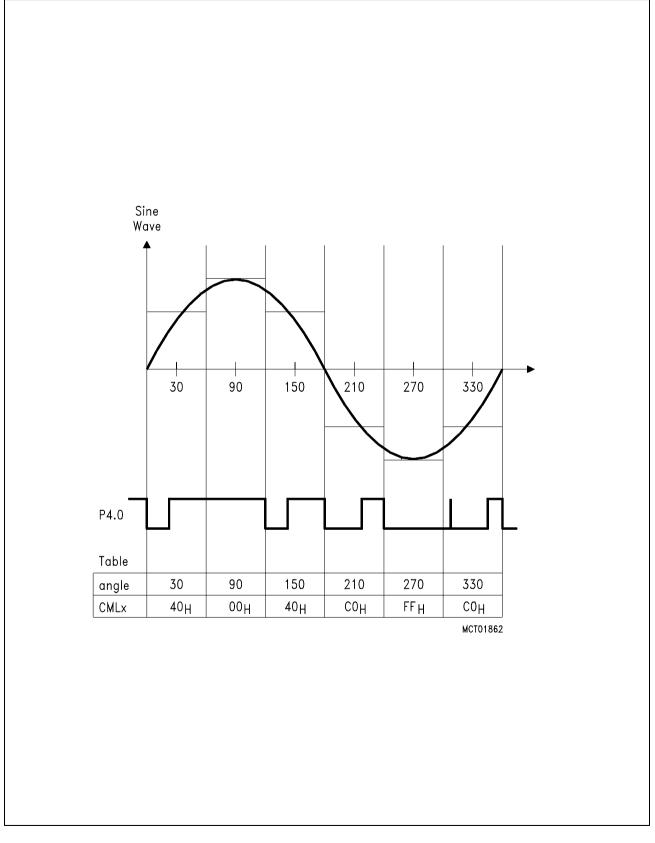
Figure 10-2 PWM Generation for Sine-Wave Synthesis
