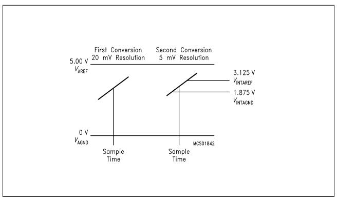
Figure 7-31 Increasing the Resolution by a Second Conversion
