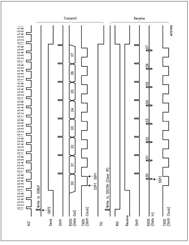
Figure 7-16 b) Timing Diagram - Serial Interface 0, Mode 0
