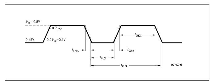
Clock of Waveform for  $I_{CC}$  Tests in Active, Idle Mode and Slow Down Mode
