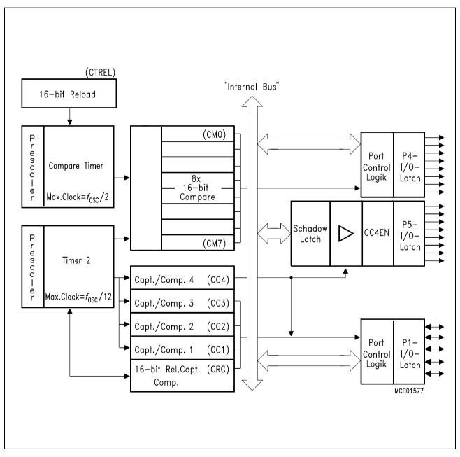
Figure 7-33 Block Diagram of the CCU
