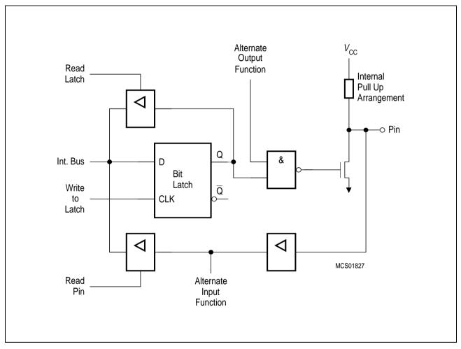
Figure 7-5 Circuitry of Ports 1, 3, 4, 5 and 6.0 through 6.2
