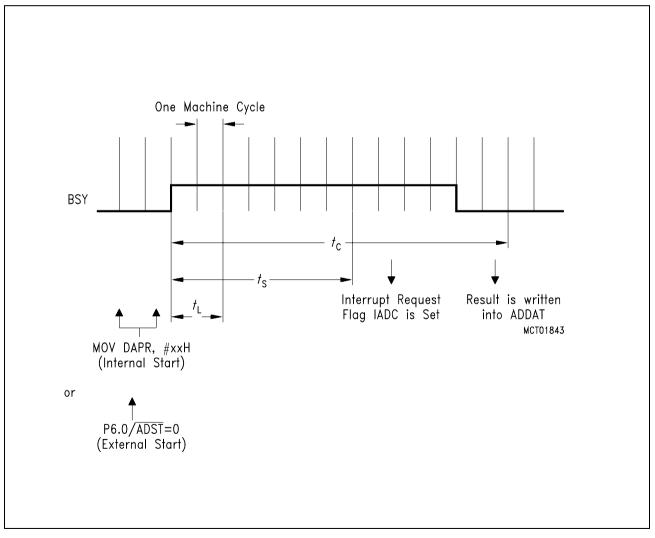
Figure 7-32 Timing Diagram of an A/D Converter
