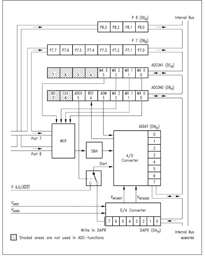
Figure 7-25 Block Diagram of the A/D Converter
