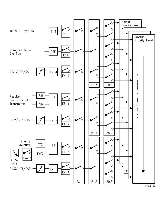
Figure 9 (cont'd) Interrupt Structure
