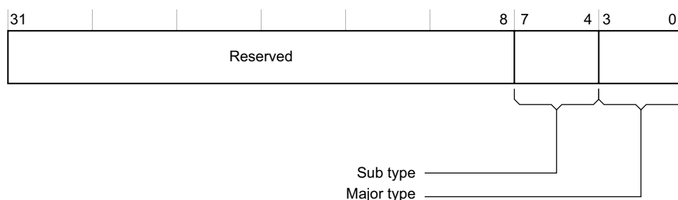
Figure 11-12 TPIU_DEVTYPE bit assignments
