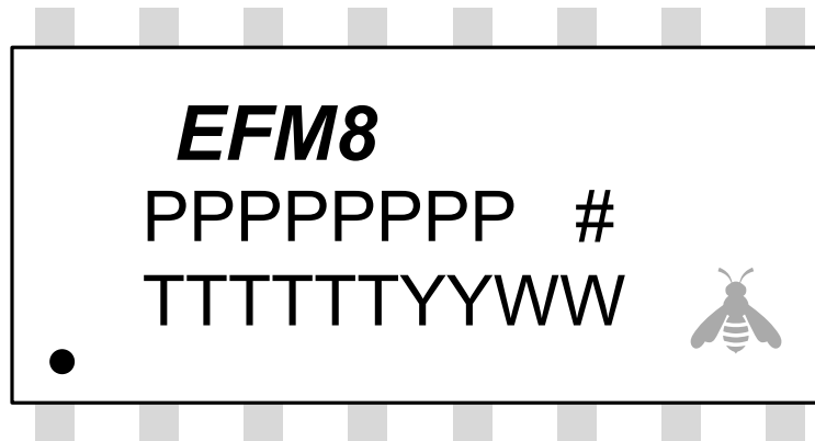
Figure 9.3. SOIC16 Package Marking
