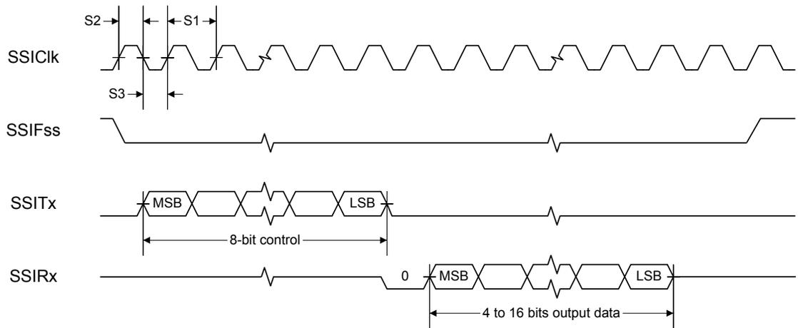
Figure 19-6. SSI Timing for SPI Frame Format (FRF=00), with SPH=1
