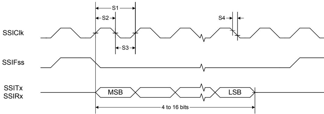
Figure 19-5. SSI Timing for MICROWIRE Frame Format (FRF=10), Single Transfer
