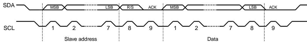
The first seven bits of the first byte make up the slave address (see Figure 13-5 on page 321). The eighth bit determines the direction of the message. A zero in the R/S position of the first byte means that the master will write (send) data to the selected slave, and a one in this position means that the master will receive data from the slave.
