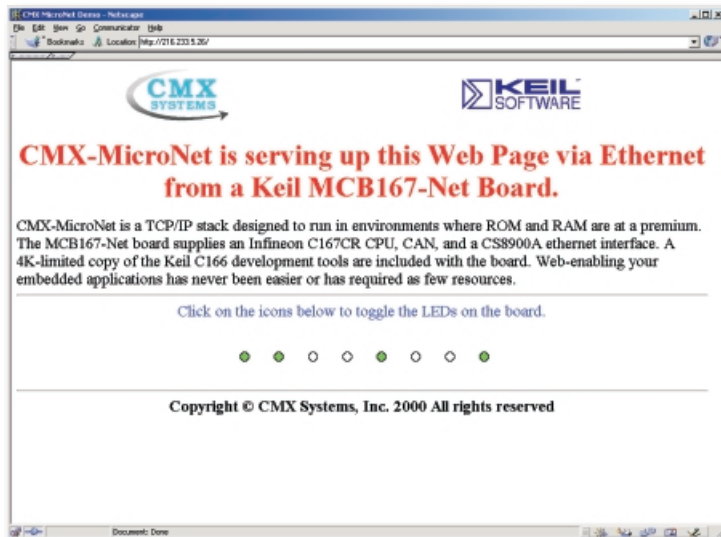
The CMX MicroNet TCP/IP stack allows you to create internet-ready applications for C16x/ST10 devices.
