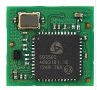
The ZM5202 module combines a Z-Wave® SD3502 SoC (with a built-in microcontroller and Z-Wave RF transceiver), crystal, and passive RF components. This makes the ZM5202 ideal for single microcontroller
