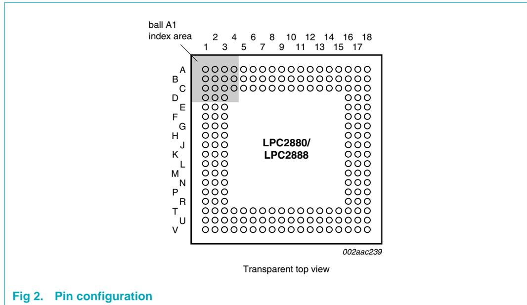
Fig 2. Pin configuration
