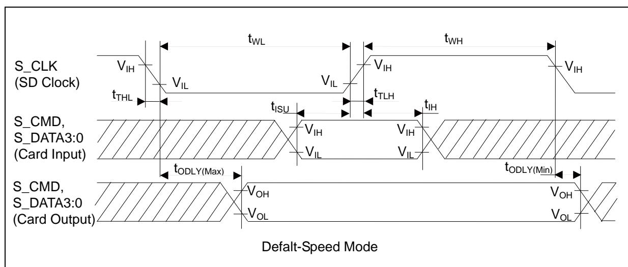
Note: The Card Input corresponds to the Host Output and the Card Output corresponds to the Host Input because this model is the Host.
