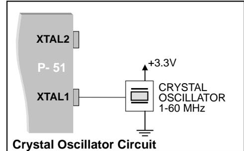
The frequency range for the Crystal circuit is 4 to 51 MHz. The circuitry differs for fundamental vs. third-overtone crystals. The boundary between the two types is approx 26 MHz (consult crystal manufacturer specs).
