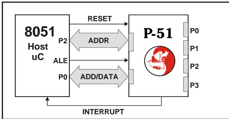
In this example a standard 8051 uses P0, P2, and control strobes to control a P-51, effectively doubling 8051 resources. The internal dual port RAM serves as a mailbox for communicating between the two and also can be used as 4K RAM data for a standard 8051. The standard 8051 can download code to the P51 while holding it in reset, then release the P51 to run the code. Think of the possibilities!
