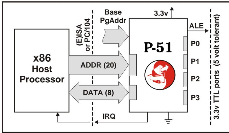
In the case of the 20-bit address presented by the EISA bus, the high order bits are compared to the Base Page address pins, and the P-51 is enabled when addresses match, thereby allowing the P-51 to be located at a specific range in x86 address space. By writing to a P-51 control register, the x86 can select (and enable) an IRQ signal (from IRQ3 to IRQ15).
