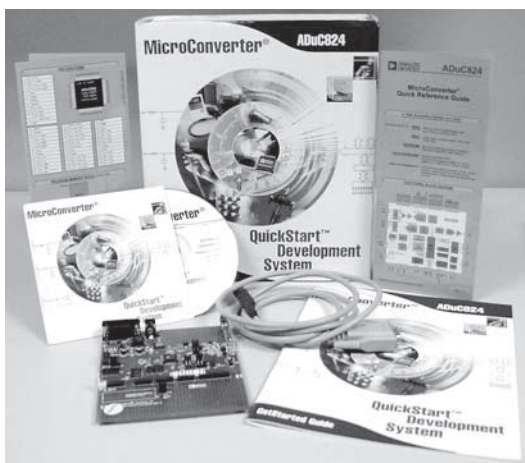
Figure 65. Components of the QuickStar Development System
